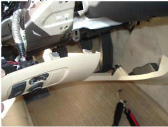
There are two screws (self-tapping) behind the loosened cover that need to be removed to free up the driver's side center console cover.
