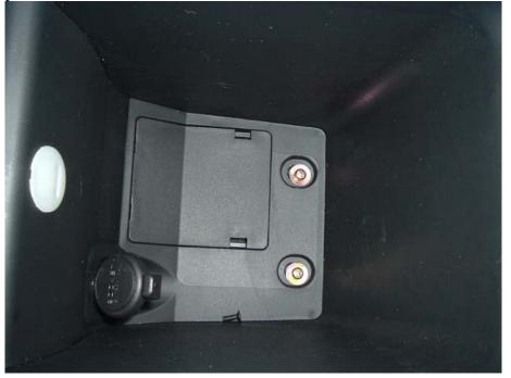
Remove self-tapping screws on driver side that were under removed trim.
