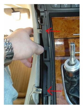
Fold down the carpeting from the side console (there are a couple of clips easily removed) to gain access to the back of the unit with the aux input.
