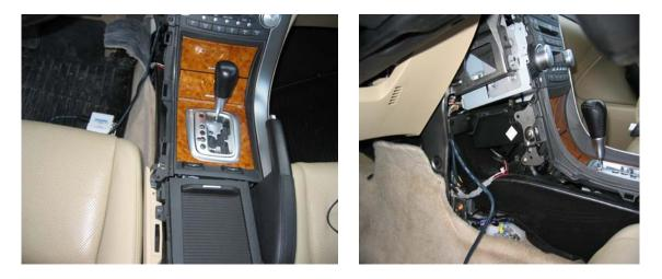
Now you have to decide where to run the cable, and where to put the 'box'. I decided to run the cable behind the drivers side console cover, have the box under the driver's seat (relatively easy access), and the cable for my ipod and Sirius run from under the driver's seat under the console, through the door at the bottom of the console box (used wire cutters to snip the corner off of the door to fit the wires - some have drilled a hole, wire cutters are simpler (2019) and reinstall panels.
