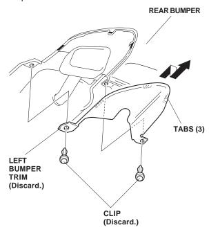
Remove the rear bumper (two covers, two bolts, six clips and six self-tapping screws).
