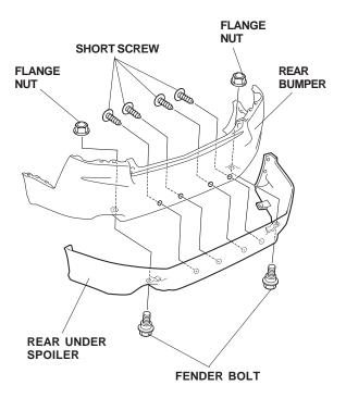
7. Using a tape measure and a felt-tip pen, measure and mark the rear under spoiler in the area shown.
