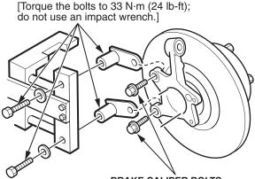
**BRAKE CALIPER BOLTS** [Torque to 54 N m (40 lb-ft); do not use an impact wrench.]
