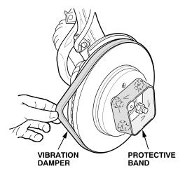
If you are not using the power drive system, use a fabric tie-down strap to secure the brake disc that is opposite to the one you are refinishing. If you are working on an Integra Type-R, do not use a tie-down strap; let both front wheels turn freely.
