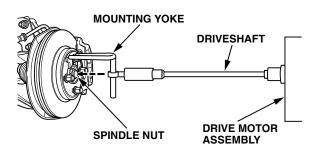
Set the lower toggle switch on the drive motor assembly to FWD (counterclockwise rotation) or REV (clockwise rotation).
