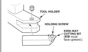
Before you use the brake lathe, inspect the tips of the cutting bits with a magnifying glass to make sure the tips are not worn out. Each bit has three tips. If a tip is worn, rotate the bit, and use a new tip. A worn tip produces a poor finish and may cause chattering.
