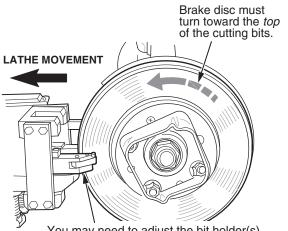
You may need to adjust the bit holder(s) for proper cutting of the brake disc.
