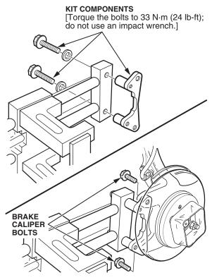
[Torque to 54 N·m (40 lb-ft); do not use an impact wrench.]
