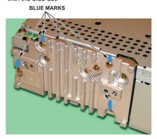
4. Using the orange marker, mark the four 2.6 x 16 mm screws on the heat sink as shown. Then remove the four screws, and place them in the section of the screw container marked with the orange dot.
