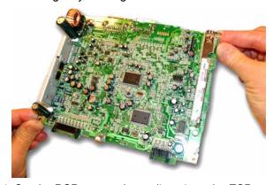
Set the PCB next to the audio unit on the ESD mat, and pull on the ribbon cable to disconnect it from the PCB.
