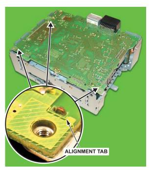
14. Carefully remove the protective cover from the gray thermal pad on the replacement PCB.
