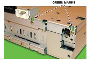
7. Using the green marker, mark the large screw on the front lower cover of the audio unit. Also, mark the small screw with the red marker. Then remove the two screws, and place them in the appropriate sections of the screw container marked with the green dot and the red dot.
