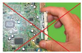
Never touch the electrical components of the PCB.
