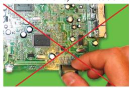
To prevent damage to the thermal pad, don't remove the protective cover until step 14.
