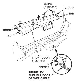
5. Remove the screw, then remove the opener assembly from the front door sill trim.
