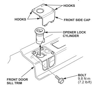
3. Remove the opener lock cylinder. Remove the bolt from the opener assembly.
