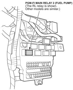
• If the name is **DENSO**, the relay is OK. Go to step 6.
