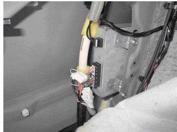
12. Connect the blue No. 1 connector of the AcuraLink reprogramming cable to the 5P connector (with male terminals) in the vehicle.
