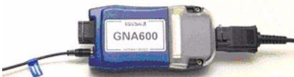
9. Connect the GNA600 power supply cord to the GNA600 and to the power supply. Connect the power supply to a power outlet. The GNA600 starts a self-check, and after about 30 seconds, the LEDs on the GNA600 flash green and yellow.
