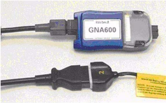
22. Within 30 seconds of the LEDs on the GNA600 flashing green and yellow, reconnect the yellow No. 3 connector of the AcuraLink reprogramming cable to the yellow connector of the reprogramming cable adapter.
