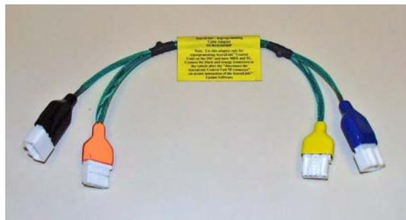
NOTE: The GNA kit and the AcuraLink reprogramming cable adapter are available through the Acura Tool and Equipment Program at **888-424-6857**.
