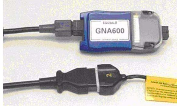
15. Connect the yellow No. 3 connector of the AcuraLink reprogramming cable to the yellow connector of the reprogramming cable adapter.
