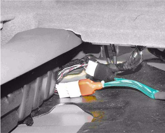
13. Connect the blue No. 1 connector of the AcuraLink reprogramming cable to the blue connector of the reprogramming cable adapter.
