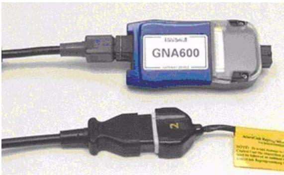
23. Within 30 seconds of the LEDs on the GNA600 flashing green and yellow, reconnect the yellow No. 3 connector of the AcuraLink reprogramming cable to the yellow connector of the reprogramming cable adapter.
