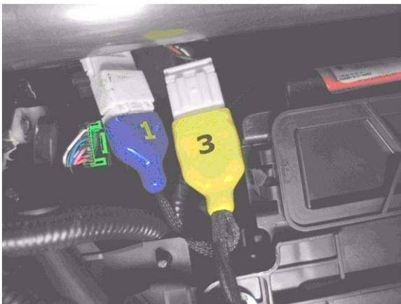
15. After the green LEDs on the GNA600 stay on, disconnect the DLC cable from the GNA600. The current program ID has been captured.
