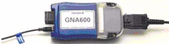
9. Connect the power supply cord to the GNA600 unit and to the power supply. Connect the power supply to a power outlet. The GNA600 unit starts a self-check, and after about 30 seconds, the LEDs on the GNA600 unit flash green and yellow.
