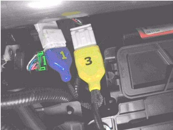
23. After the yellow LEDs on the GNA600 stay on, disconnect the DLC cable from the GNA600. The AcuraLink control unit has been updated.
