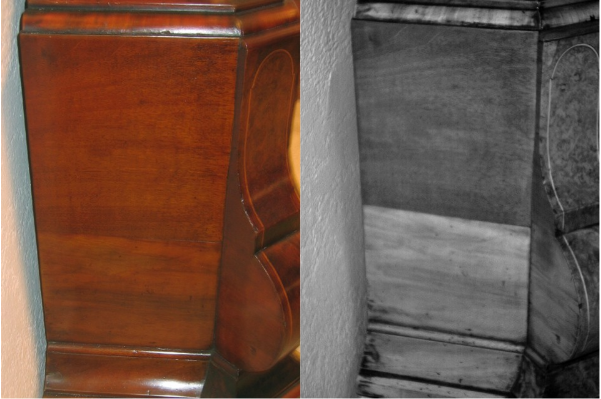
Longcase clock. This 18 th century longcase clock has had walnut veneers replaced recently. The replacement veneer appears much lighter in color, possibly because it contains more water.
