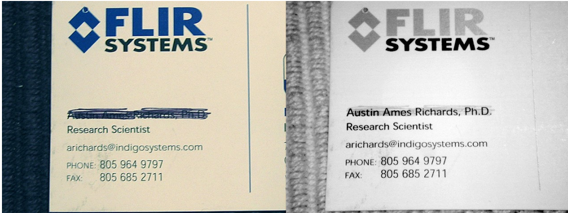
Business card. The aniline dyes used in ballpoint pen ink are transparent to NIR light.
