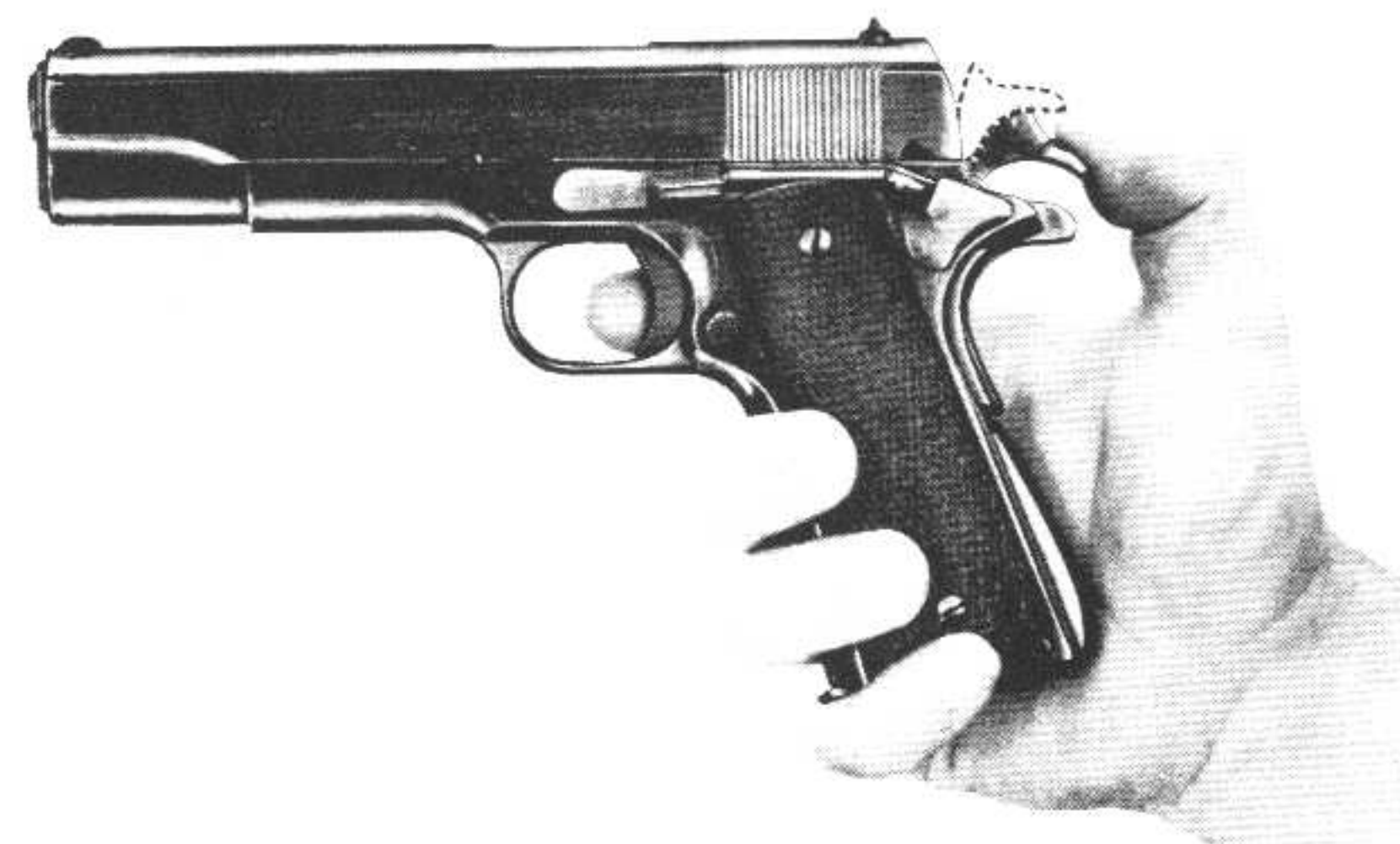
Figure 15 — Pistol M1911A1, Hammer at Half-Cock Notch, Finger Squeezing Trigger
