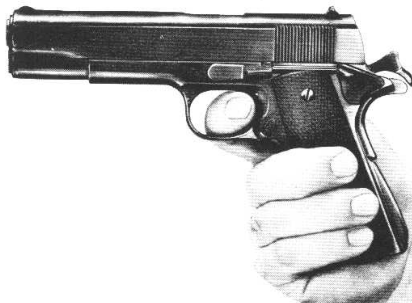
Figure 14 — Pistol M1911A1, Hammer Cocked, Grip Safety Not Depressed, Finger Squeezing Trigger
