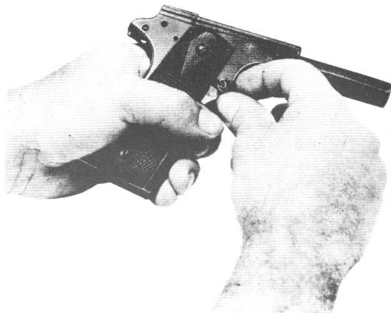
Figure 28 — Disassembling Old Design Magazine Catch from Pistol M1911
