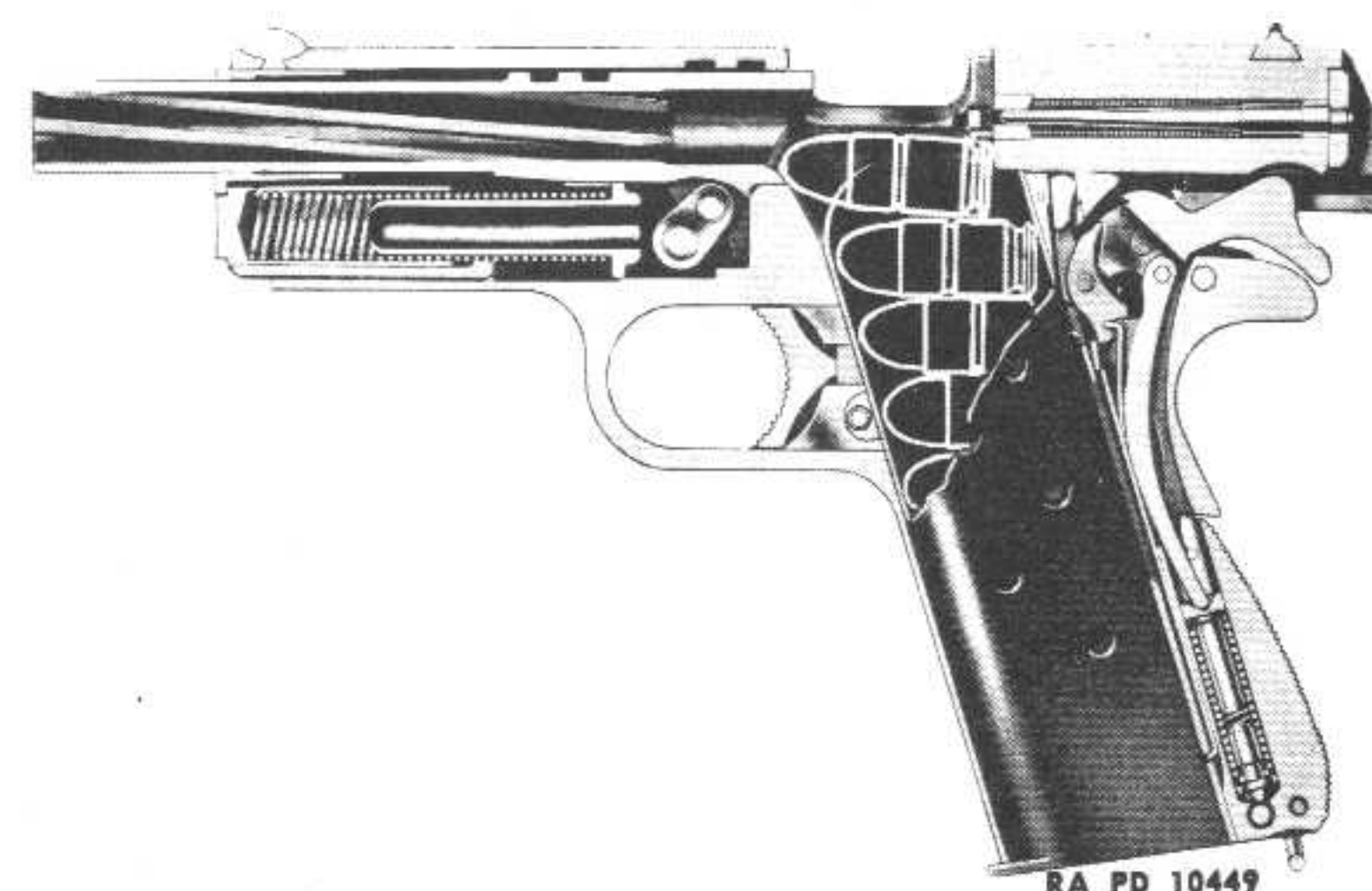
Figure 9 — Sectional View of Pistol M1911A1, Slide Partly Forward, Cartridge Entering Chamber, Hammer Back
