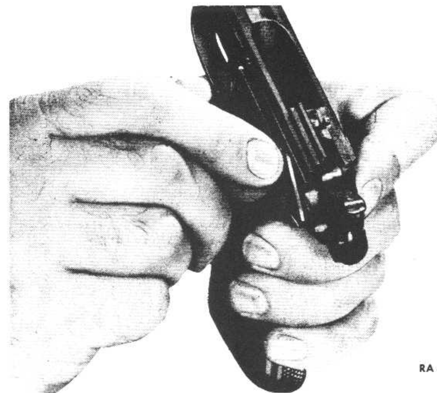
Figure 27 — Removing Safety Lock from Pistol M1911A1
