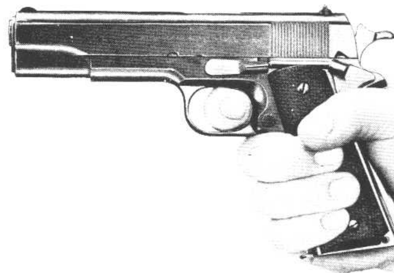
Figure 15 — Pistol M1911A1, Hammer at Half-Cock Notch, Finger Squeezing Trigger
