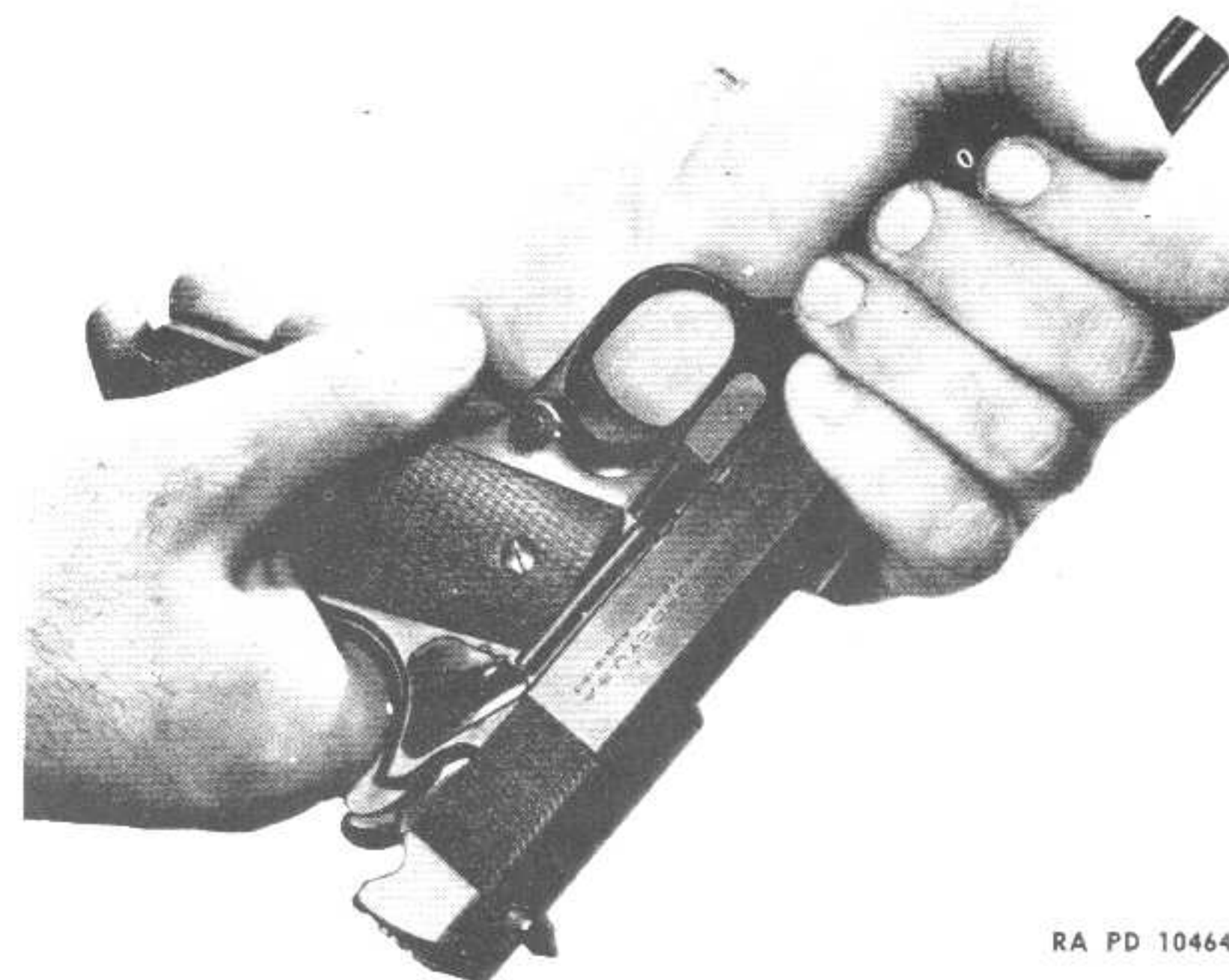
Figure 24 — Lining Up Slide Stop of Pistol M1911A1
