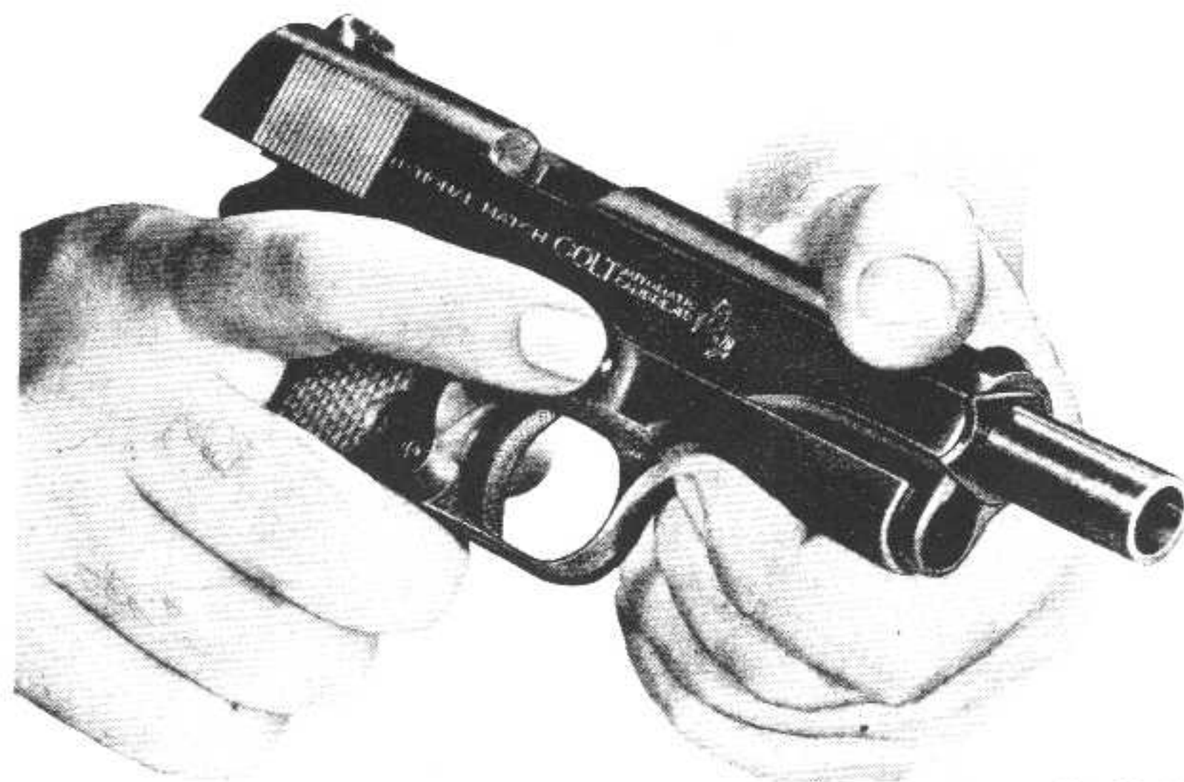
Figure 25 — Removing Slide Stop Pin from Pistol M1911A1
