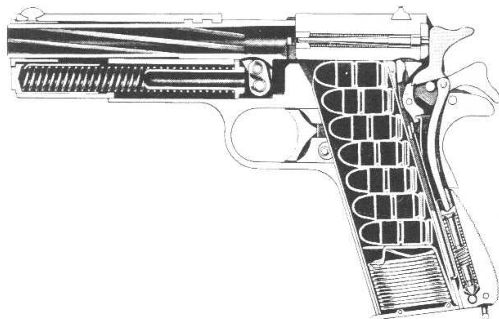
Figure 7 — Sectional View of Pistol M1911A1, Slide Forward, Magazine Loaded, Chamber Empty, Hammer Down
