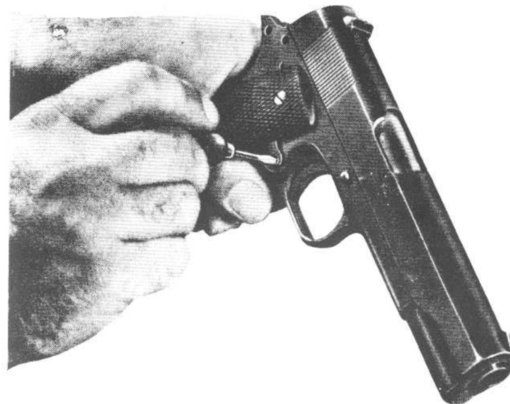
Figure 29 — Disassembling New Design Magazine Catch from Pistol M1911A1
