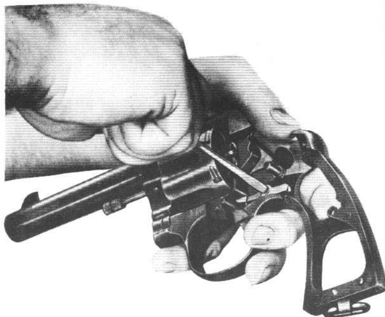
Figure 58 — Removing Bolt Screw from Colt Revolver M1917
