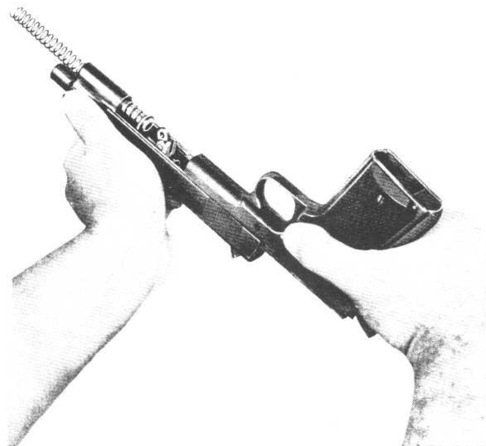
Figure 41 — Replacing Slide and Barrel on Receiver, Barrel Link Tilted Forward and Link Pin In Place On Pistol M1911A1
