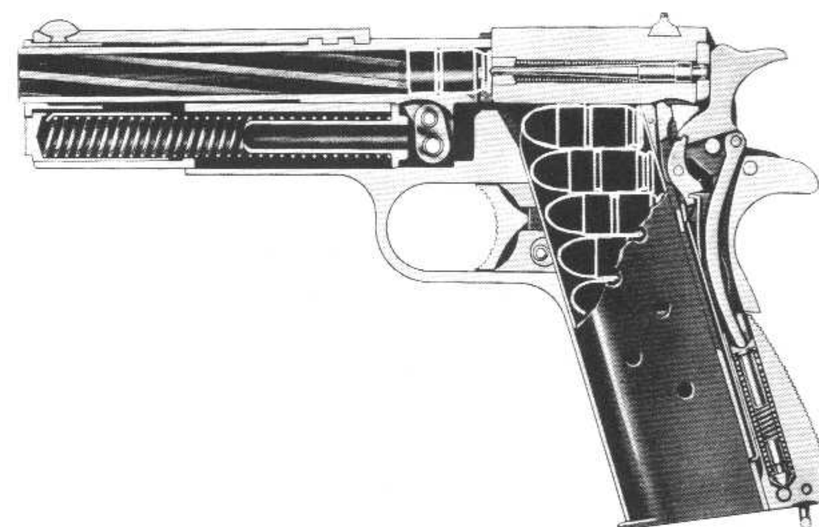
Figure 11 — Sectional View of Pistol M1911A1, Hammer Down, Firing Pin Striking Cartridge
