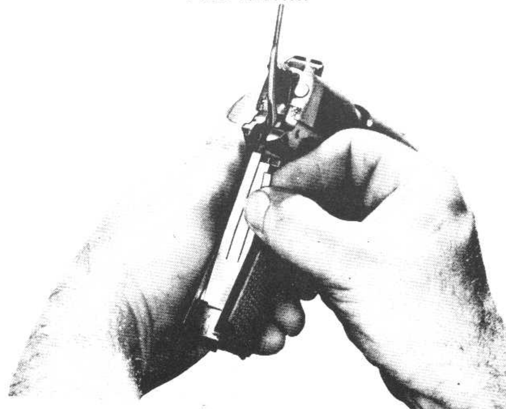
Figure 38 — Reassembling Sear and Disconnecter on Pistol M1911A1
