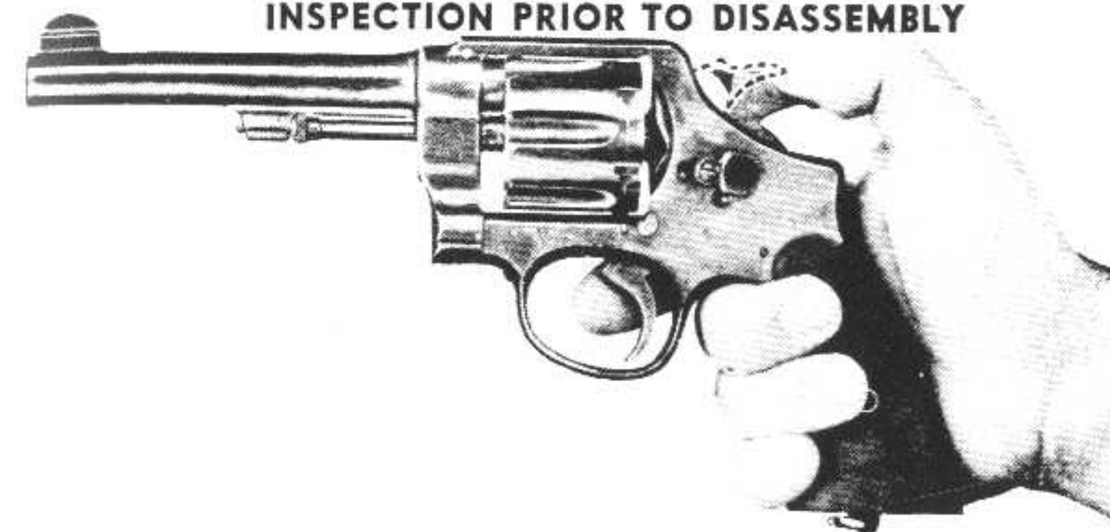
Figure 77 — Smith and Wesson Revolver M1917, Unloaded Cylinder Closed, Hammer Cocked, Thumb Holding Hammer Back
