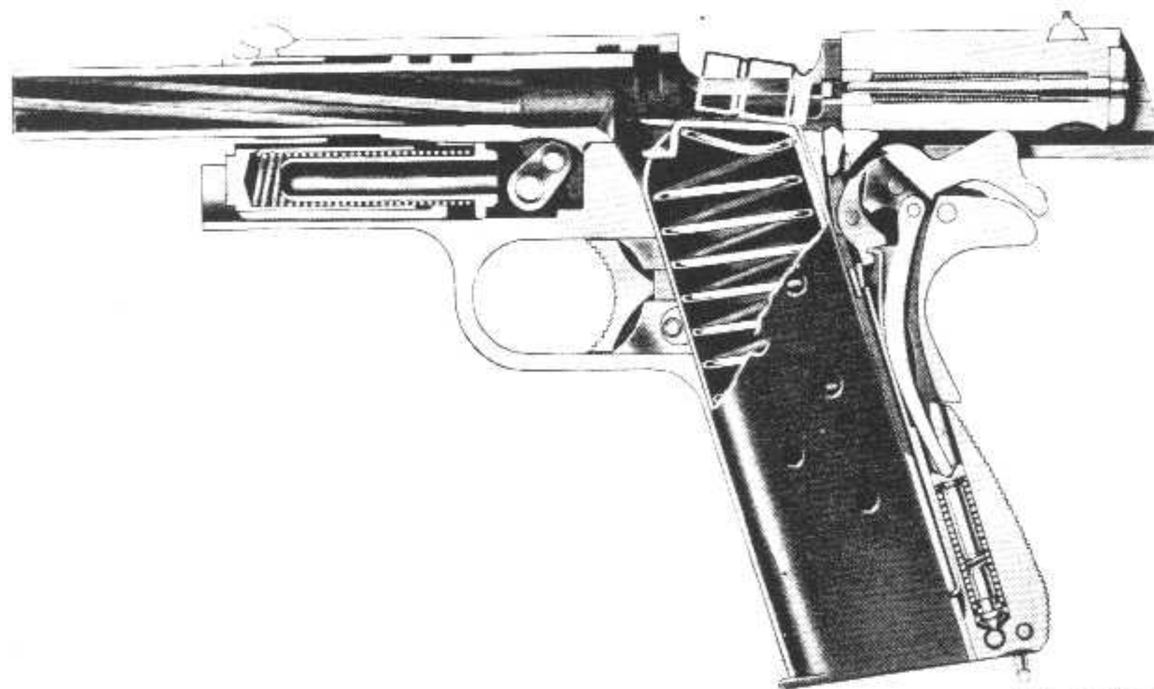
Figure 12 — Sectional View of Pistol M1911A1, Slide Back, Cartridge Being Ejected, Hammer Back, Magazine Empty
