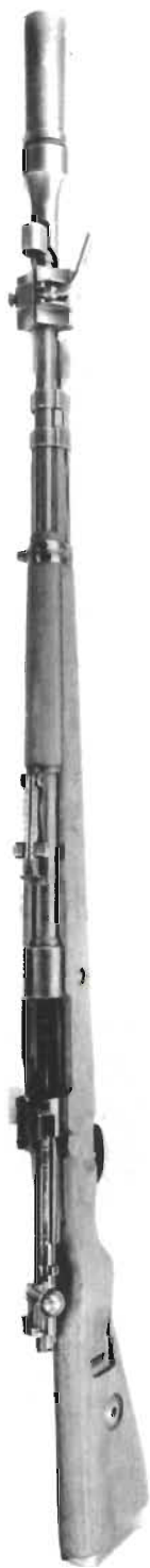
A WARTIME OPPONENT OF THE LEE-ENFIELD A German 7.92 SERVICE RIFLE fitted with Grenade Thrower.
