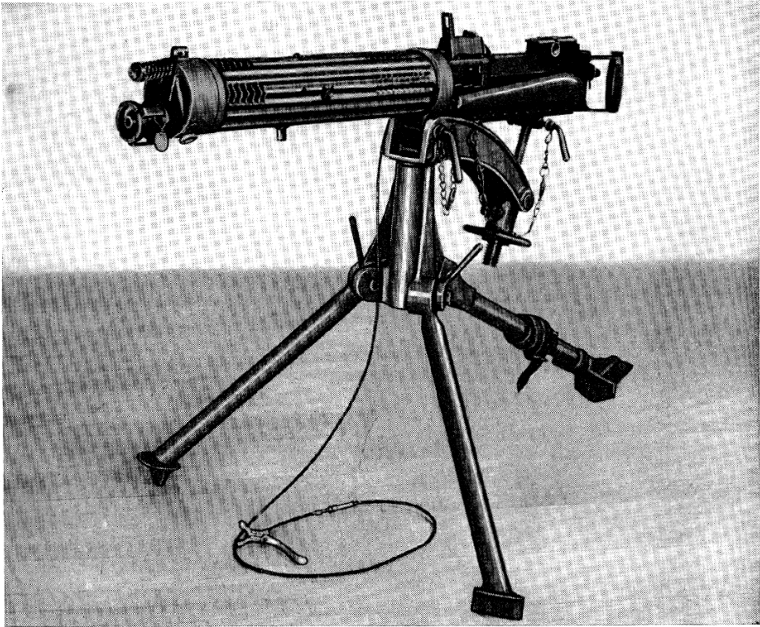
Vickers Aircraft Machine Gun, Model 1915, Equipped for Synchronizing. Mount is for Purposes of Photographing Only.
