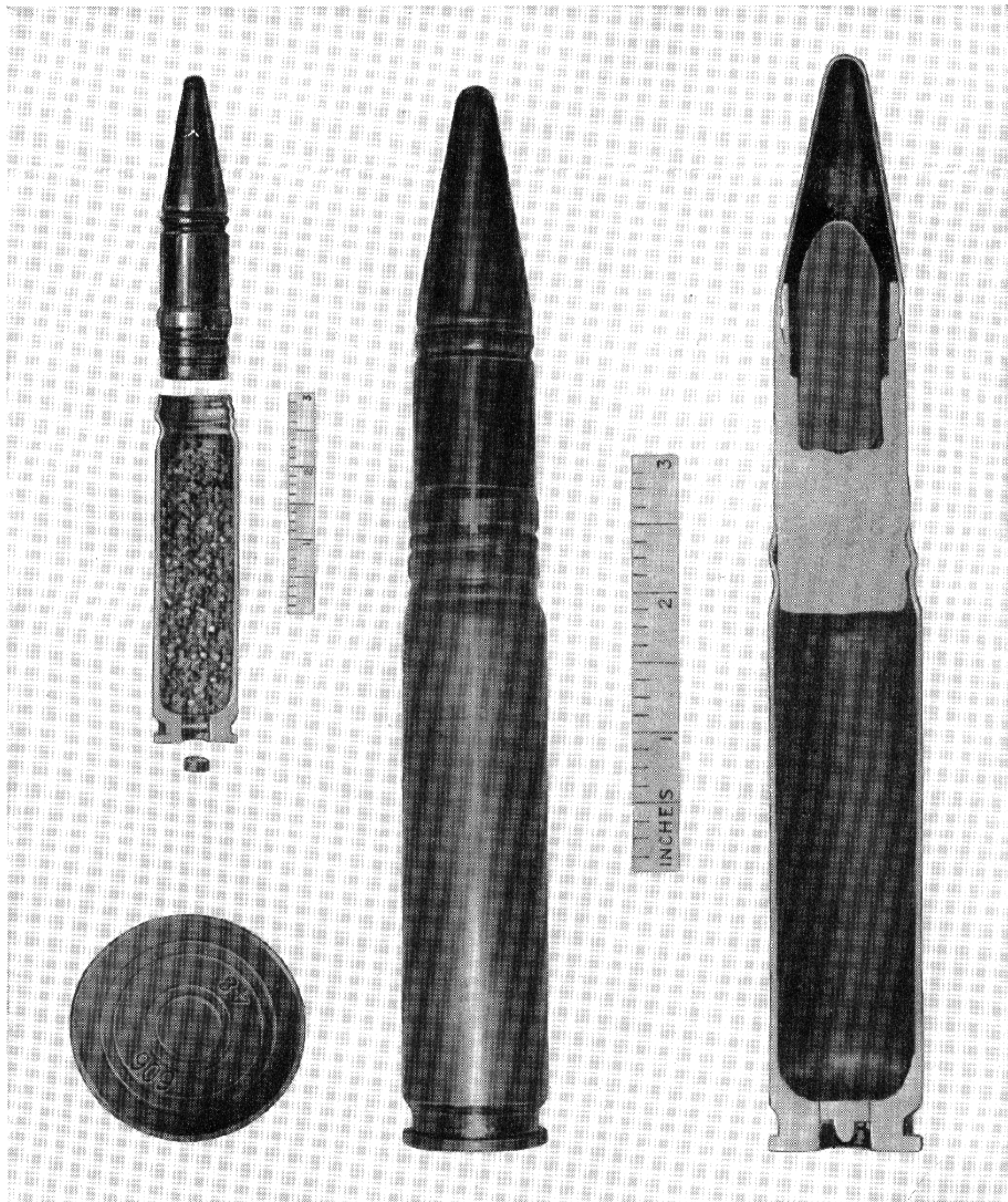
Figure 9-15. Study of a complete round for 23-mm NS cannon.
