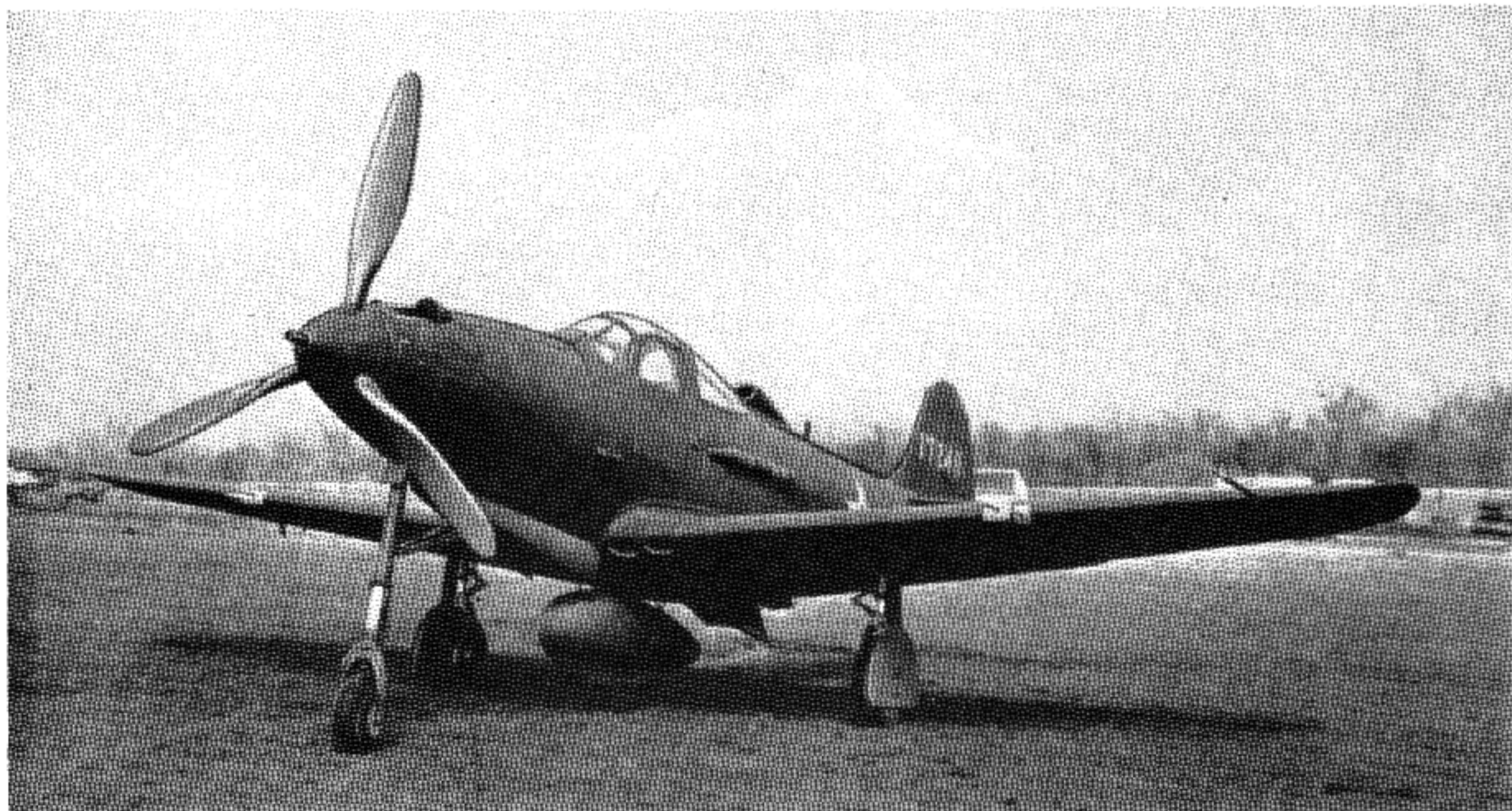
Figure 12-1. 37-mm Browning Gun M4 mounted in a P39F aircraft to fire through the propeller hub.
