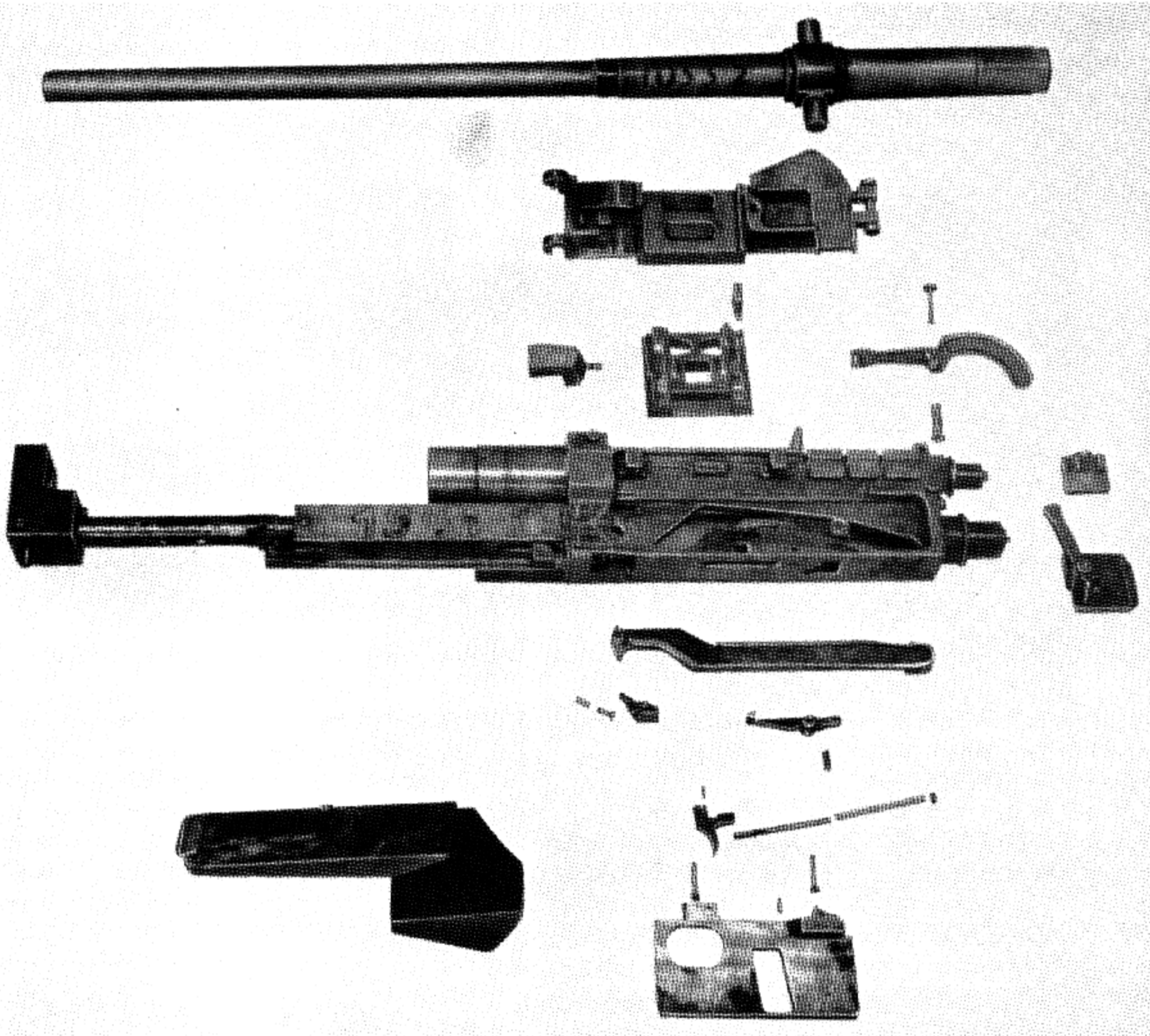
Figure 24-12. Second version of Krieghoff Experimental 20-mm Aircraft Cannon. Exploded view of feed elements.
