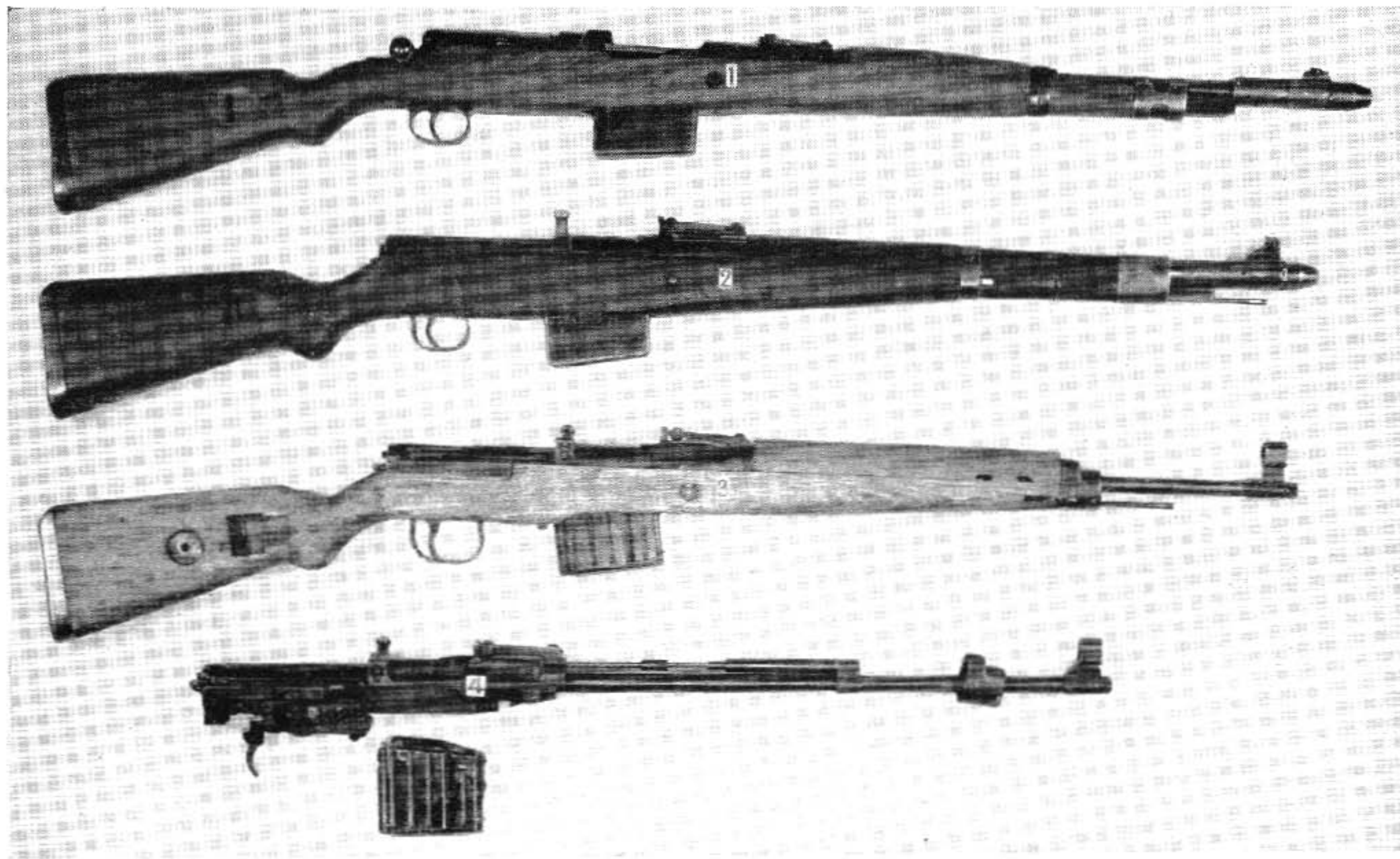
German semiautomatic rifles of World War II: 1. Gewehr 41M. 2. Gewehr 41W. 3. Gewehr 43. 4. Gewehr 43 with stock removed to show gas cylinder
