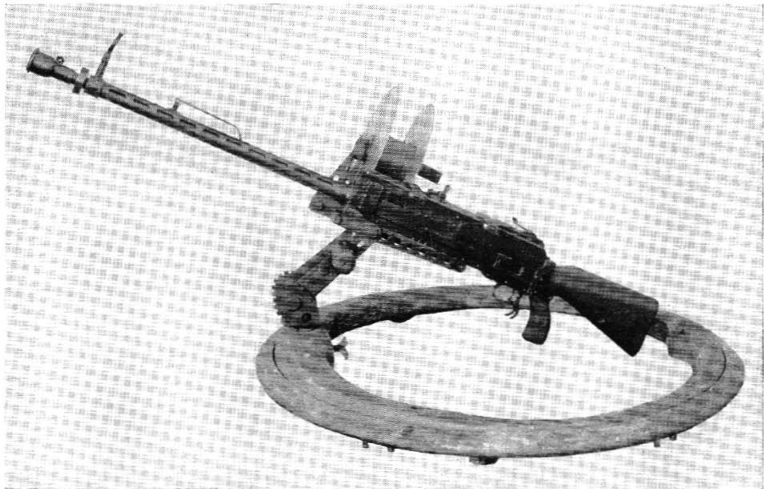
German Parabellum aircraft machine gun. This weapon, designed by Karl Heinemann, bears the following lettering on the left side, "S. M. Gew. Mod. Parabellum 1913. Berlin." It was used as a flexible machine gun in German World War I aircraft.
