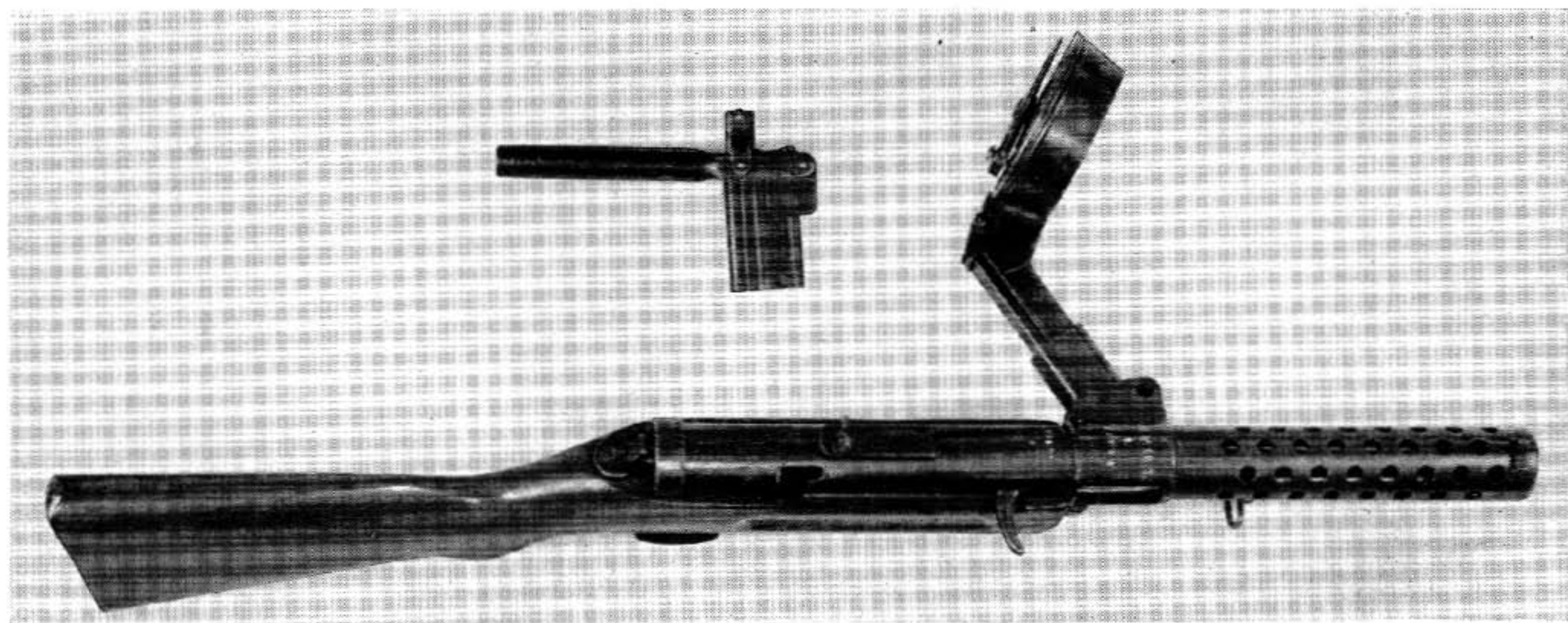
The German Bergmann Submachine gun of World War I, called the M.P. (Maschinen Pistole) 18. It has a straight blow-back action and shoots the 9 mm Luger pistol cartridge from a snail shaped magazine. The World War II submachine guns are no advance over this except in cheapness of manufacture due to their flimsy construction of tubing and stampings.
