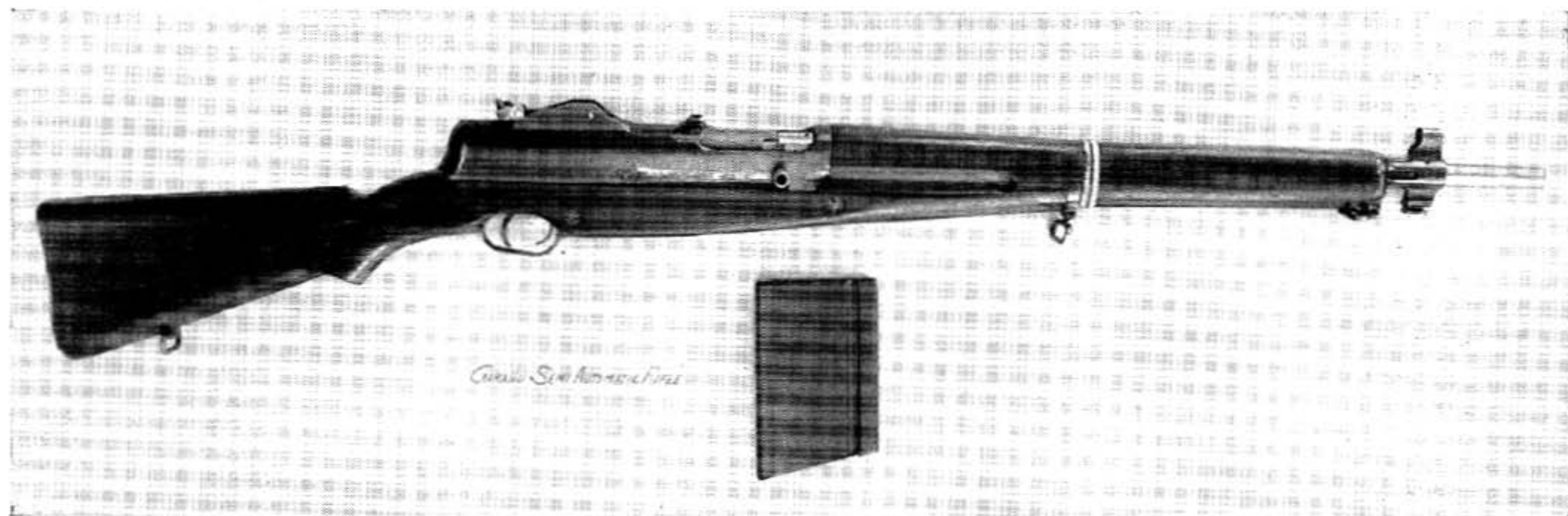
Garand's first semiautomatic rifle, a primer actuated model built at Springfield in 1920. It used the service .30 caliber cartridge.
