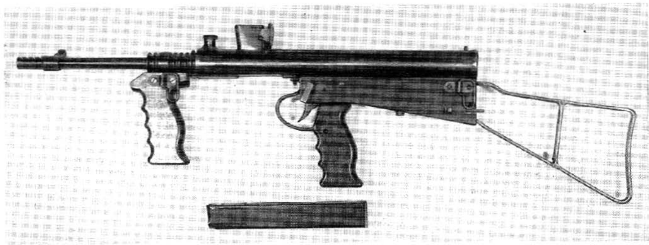
Australian Owen Submachine gun. Notable only for one thing: utter cheapness of construction.
