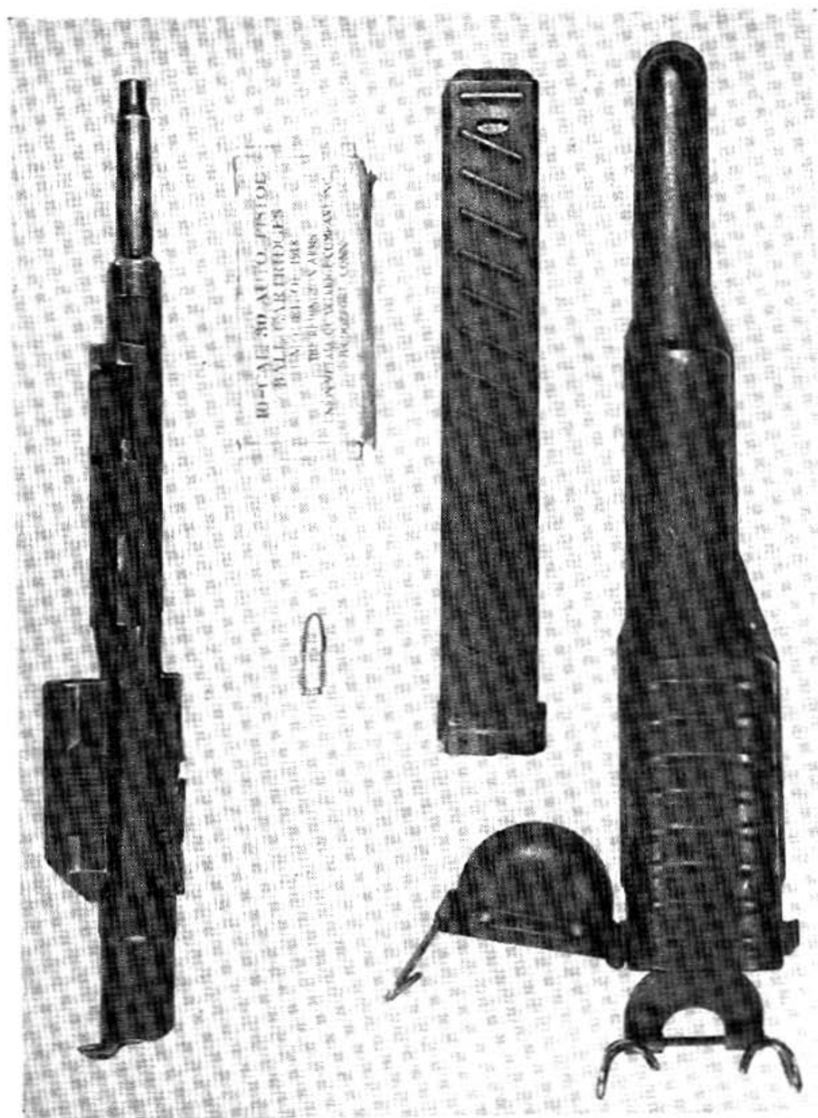
The Pedersen Device, shown with its ammunition, the 40 round magazine, and the metal scabbard used for carrying the device on the soldier's belt.
