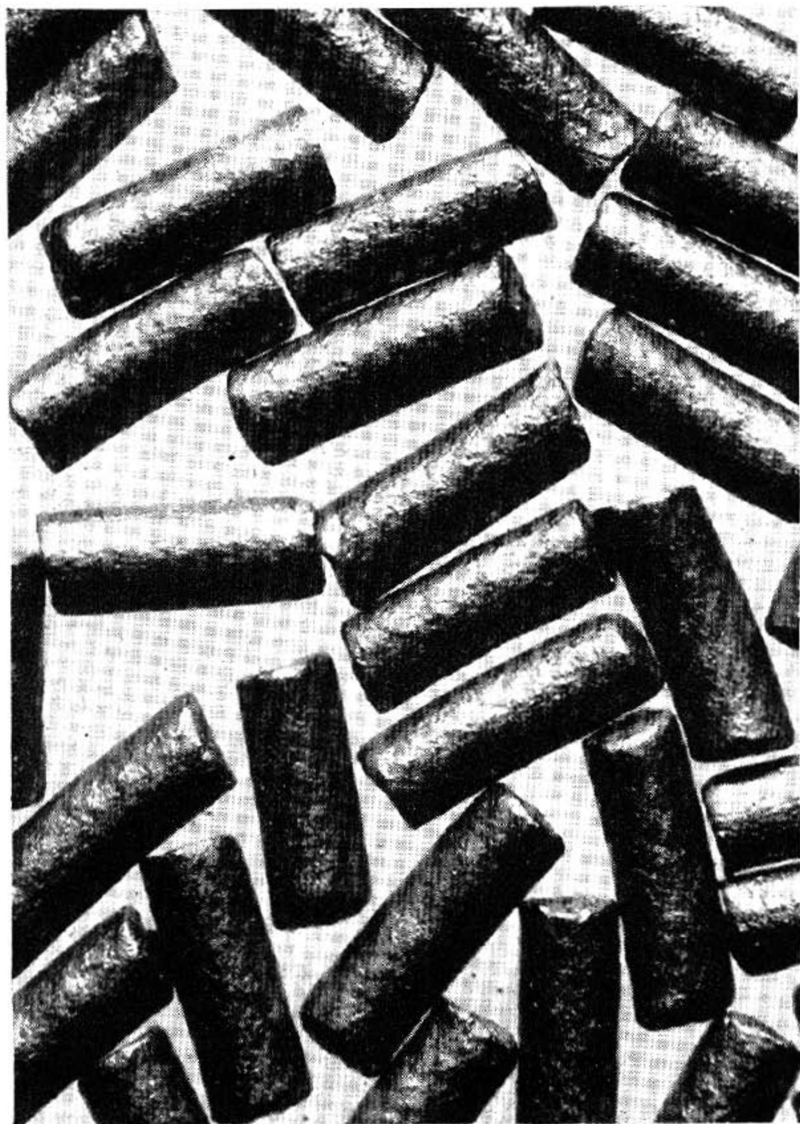
A modern smokeless rifle powder. DuPont's improved military rifle powder No. 3031. This powder is made in the form of little cylinders nearly a tenth of an inch long with a hole through the center of each. Actual length of the grain: seven and a half hundredths of an inch. Diameter: two and a half hundredths. This powder is used in loading service cartridges for the Springfield rifle.
