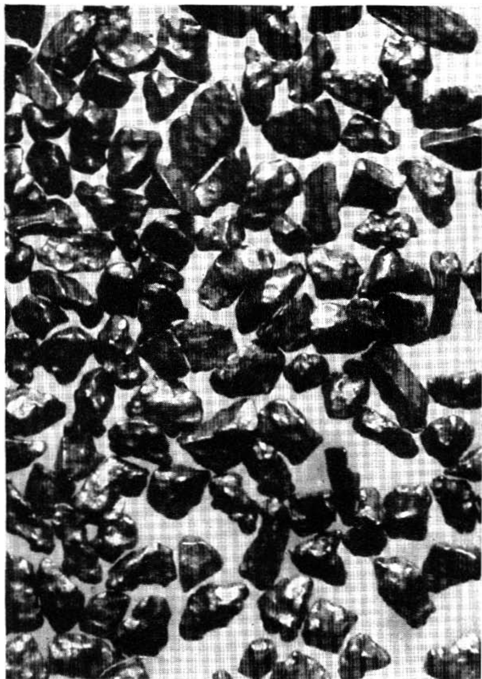
Black powder of fine granulation, such as is used in small caliber pistol cartridges and in cap and ball pistols. Grain size FFFG. Magnified 20 times.
