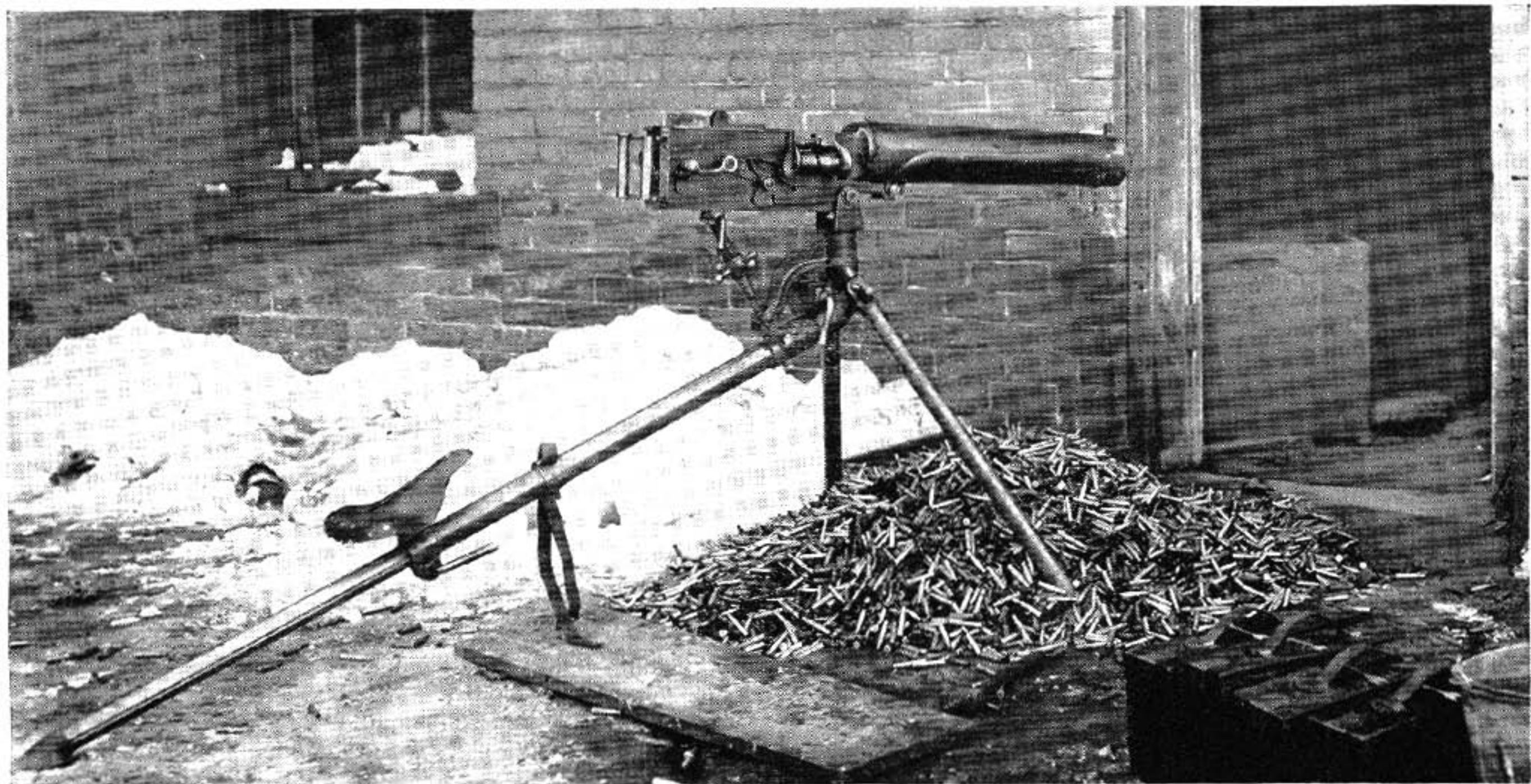
A machine gun of 50 years ago. A very early model of the Maxim at the end of a 20,000 round endurance test at Springfield Armory. Firing was into a sand pile in the room in front of the gun. The cartridges are the rimmed type of .30 caliber used in the then new Krag Model of 1892. It is interesting to note that there is very little difference between this early machine gun and some that were used in World War II.
