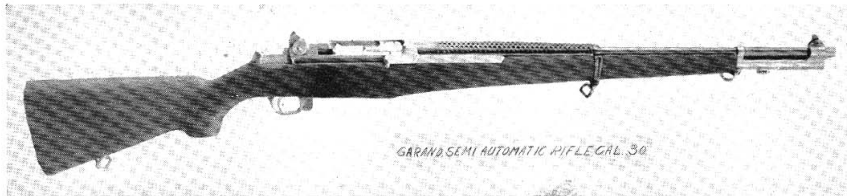
First model of the present .30 caliber M1 rifle. Garand first built two successive models of primer actuated .30 caliber guns, then a .276 gas actuated gun to take the Pedersen .276 cartridge. The gun shown above duplicates his .276 in .30 caliber. Photo taken September 10, 1930
