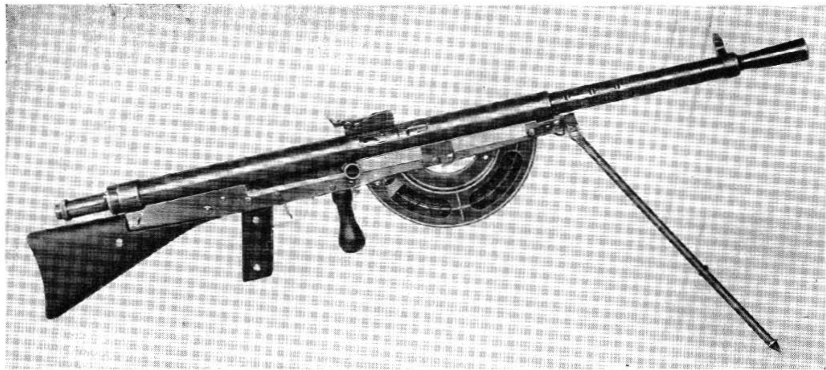
The French Chauchat machine rifle as used by the American Army in 1918. The gun shown was made for use with the 8 mm Lebel cartridge. The semi-circular magazine held 30 shots.
