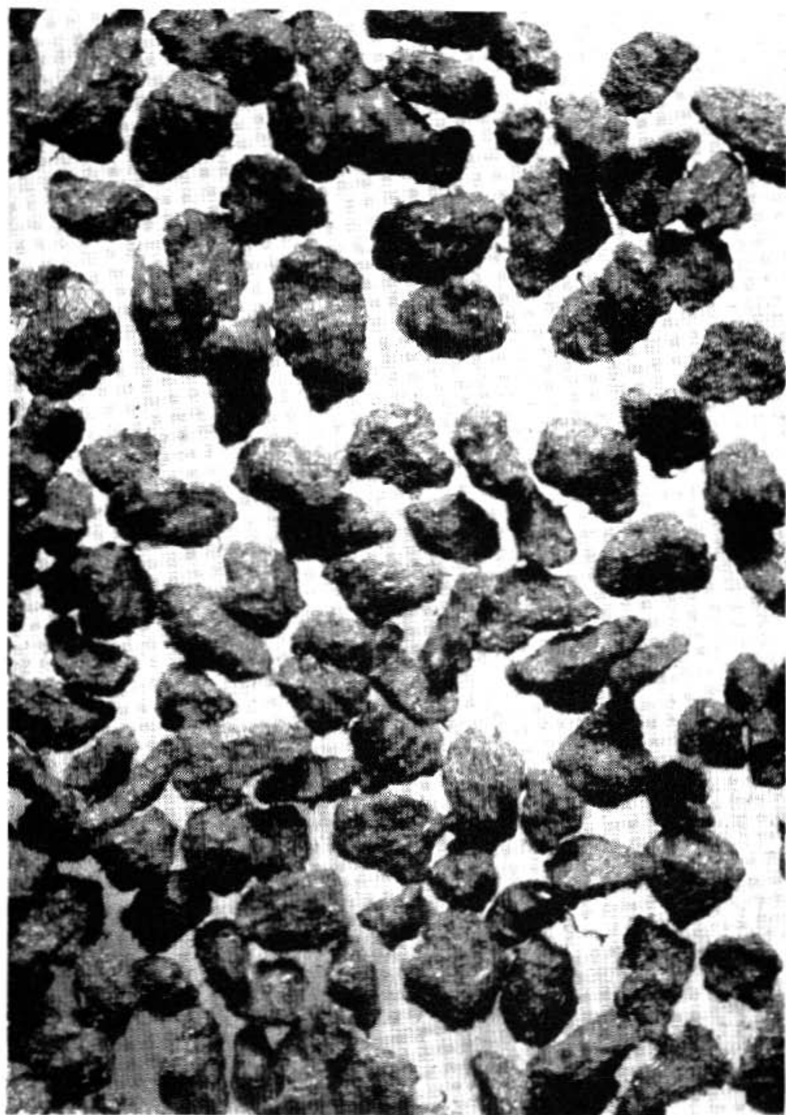
Lesmok powder, popular in .22 caliber rifle and pistol cartridges before the advent of the non-corrosive primer. It is a mixture of 85 percent black powder and 15 percent guncotton.
