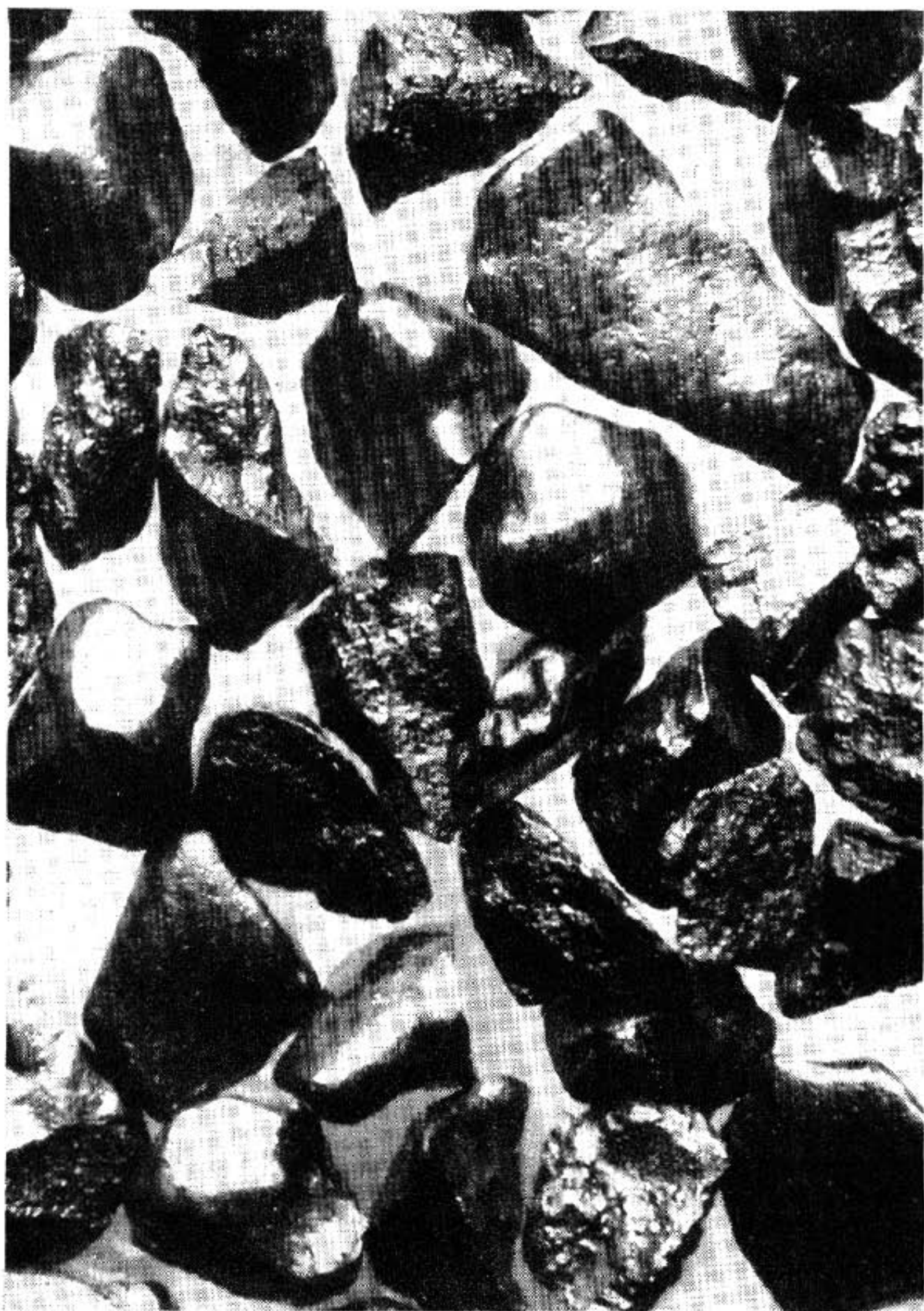
Old fashioned gunpowder. Black sporting powder size FFG. This photograph well illustrates the characteristic grain shape of black powder. The ingredients are first made into large sized grains which are polished, then broken if too large in size. The rounded and polished surfaces of the original grains as well as the fractured surfaces can be plainly seen. Magnified 20 times.
