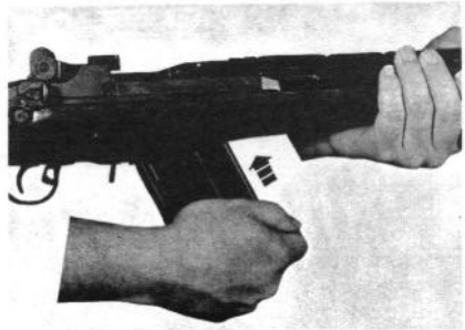
Figure 29. Loading the magazine into the rifle.
