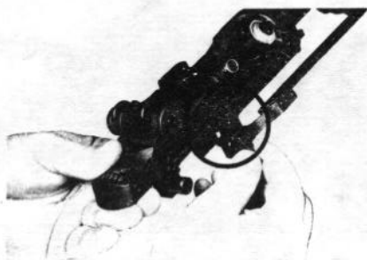
Figure 13. Removing operating rod.
