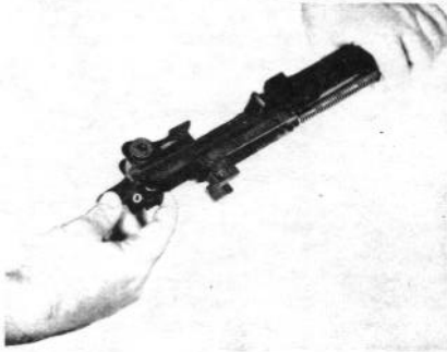
Figure 11. Removing the connector assembly.
