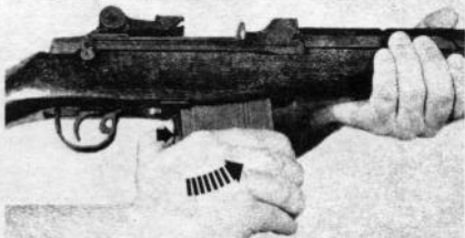
Figure 4. Removing the magazine.
