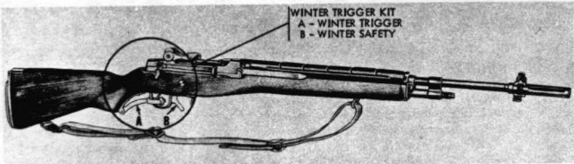
Figure 60. M14 rifle with winter trigger kit.
