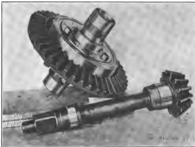
Fig. 30. The Equalizing Gear Complete, with Bevel Gear and Pinion
