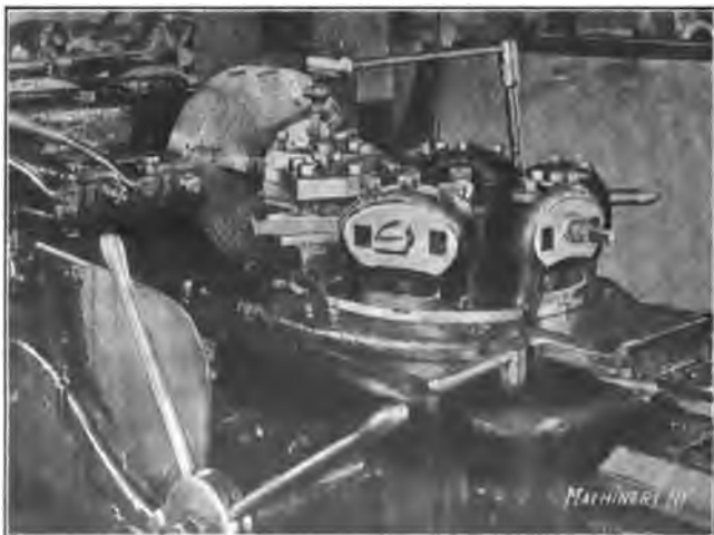
Fig. 36. Second Operation on the Flat Turret Lathe using Special Jaws
