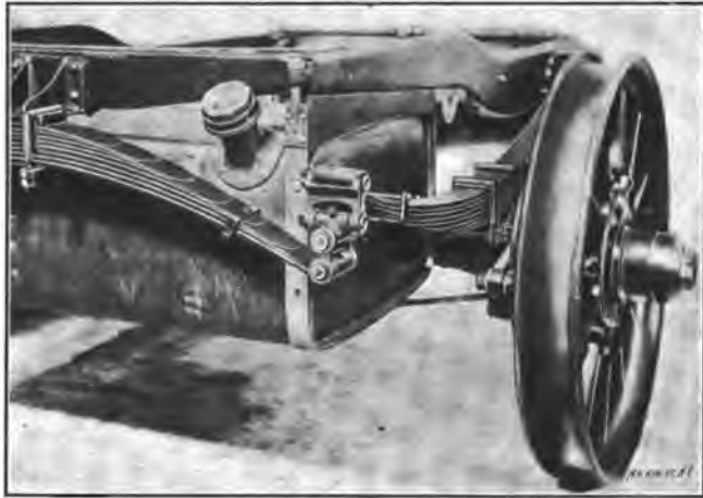
Fig. 28. Arrangement of Semi-elliptic Springs on the Lozier Motor Co.'s Four-cylinder Model
