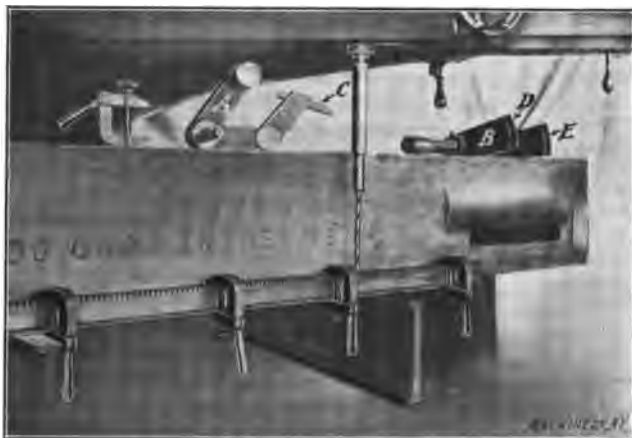
Fig. 5. Special Clamps for Holding Rack in Position when Drilling, and Fixtures used for Locating Tumbler Locking Plate
