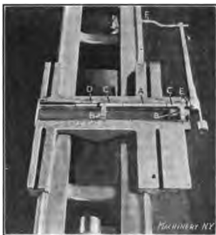
Fig. 6. Top View of Carriage, showing Method of Squaring the Carriage with the Bed. Springs B and D hold the Sweep in Position, enabling One Man to make the Test
