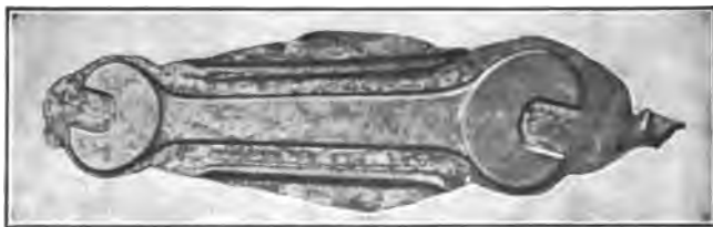
Fig. 29. A Forging showing the Effect of Flash and Back-flash
