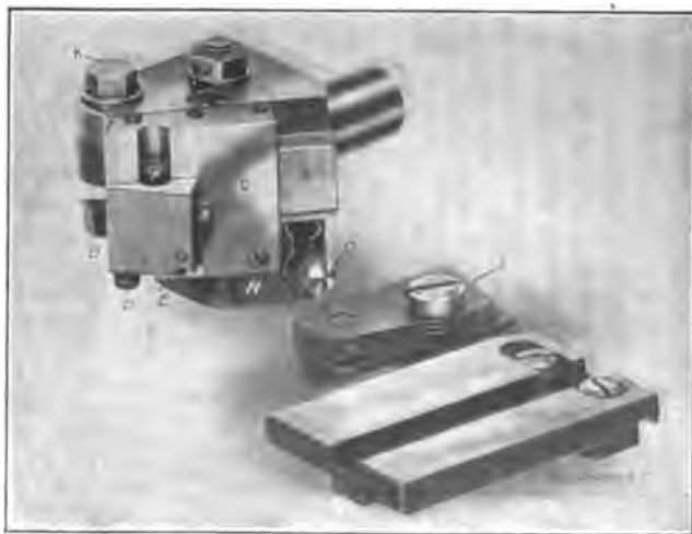
Fig. 25. Angular Cutting-off Tool held in Turret and operated by a Rising Block
