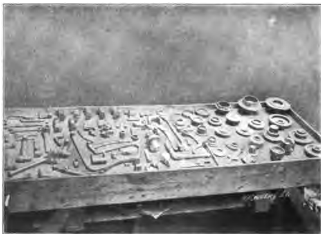
Fig. 49. Samples of Lead Castings or Proofs Taken from Drop Forging Dies for Testing the Accuracy of Outline
