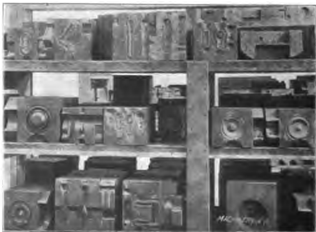
Fig. 57. A Few Examples of Drop Forging Dies in Storage
