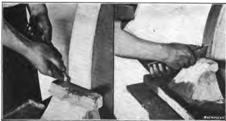
Figs. 38 and 39. Grinding the Top and Flank of a Turning Tool
