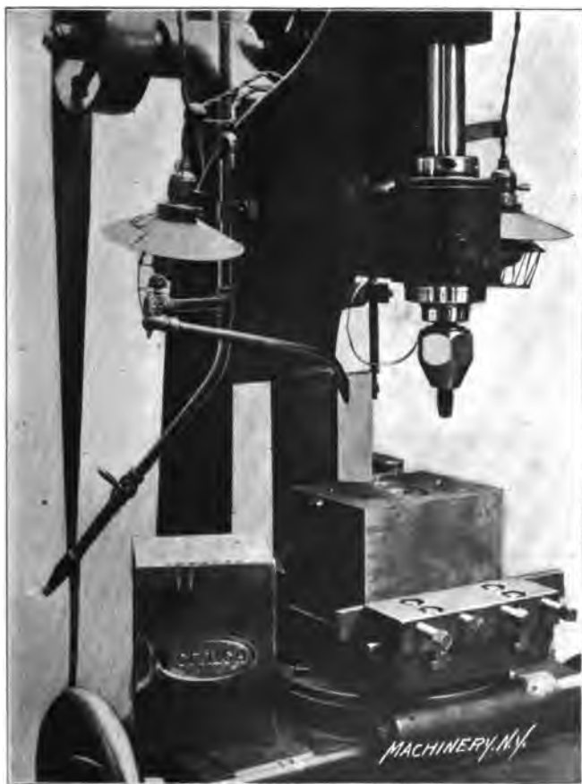
Fig. 41. Profiling Machine much Used in Die-sinking
