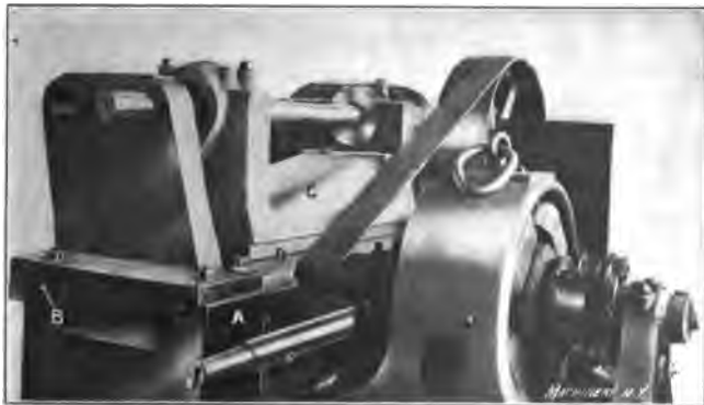
Fig. 131. Boring Jig with Portable Drive
