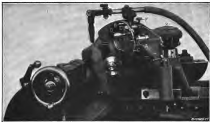
Fig. 5. End View of Landis Grinder, showing Automatic Cross-feed Mechanism
