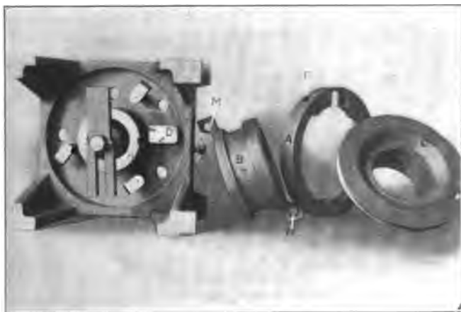
Fig. 78. Drill Jig for Parts of Friction Clutches shown at the Right
