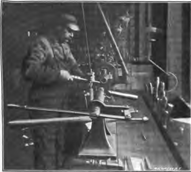
Fig. 33. View showing how the Tool is held when Spinning
