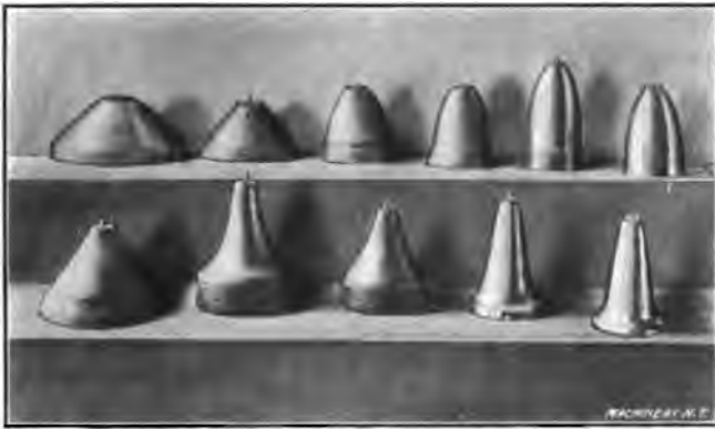
Fig. 22. Various Steps in Spinning the Two Brass Shells at the Right
