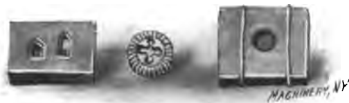
A B C Fig. 9. Blanking and Threading Dies in Protective Covers
