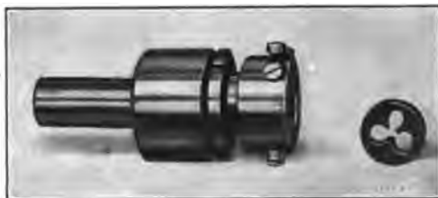
Fig. 16. Button Die Holder of the Draw-out Type
