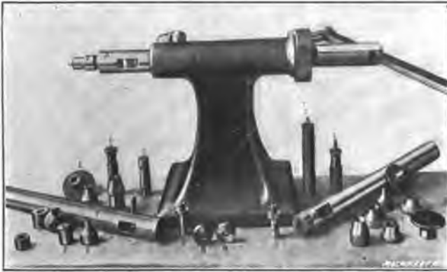
Fig. 35. Detailed View of a Spinning-lathe Tailstock
