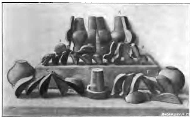
Fig. 29. Sectional Chucks made from Wood
