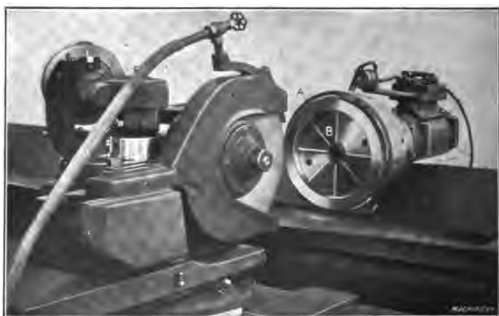
Fig. 19. Grinding Side of Steel Ring which is held by a Magnetic Chuck
