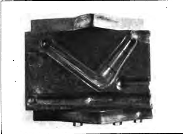
Fig. 54. Drop Forging Die and Bending Die for Steering Gear Part
