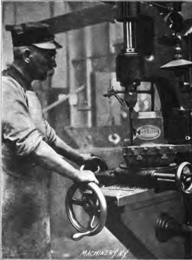
Fig. 42. Finishing the Die Shown in Fig. 40 on the Profiling Machine
