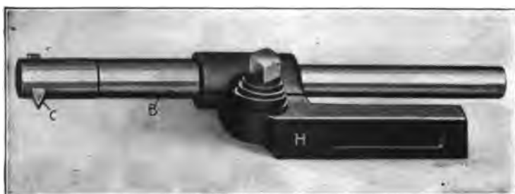
Fig. 45. Boring Tool with Inserted Cutter and Adjustable Bar
