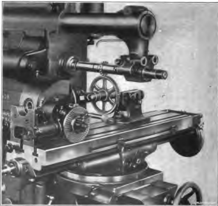
Fig. 6. Cutting the Teeth of a Spur Gear in a Universal Milling Machine
