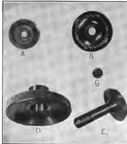
Fig. 32. Examples of Work Requiring Knurl-holder Application.
