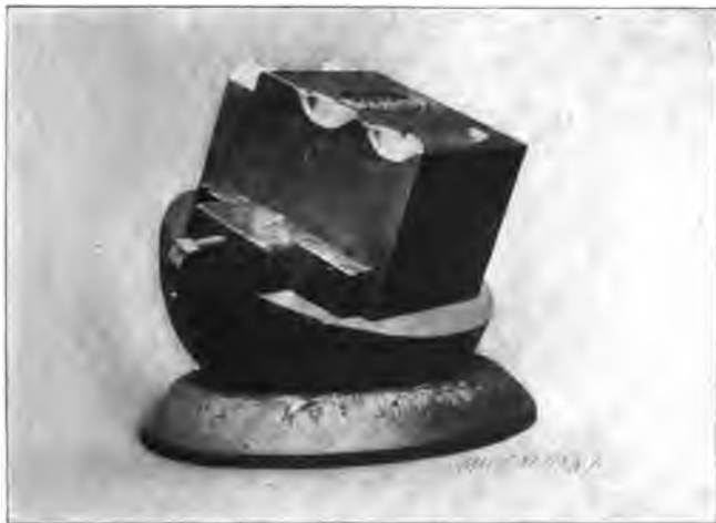
Fig. 43. Special "Ball Vise" Used in Sinking Drop Forging Dies
