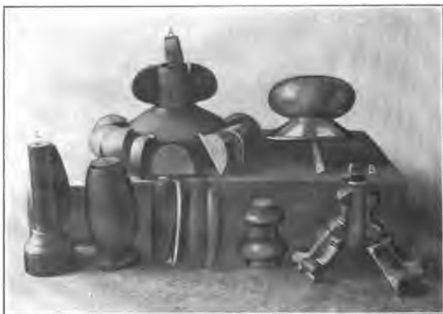
Fig. 30. Other Examples of Wooden Sectional Chucks
