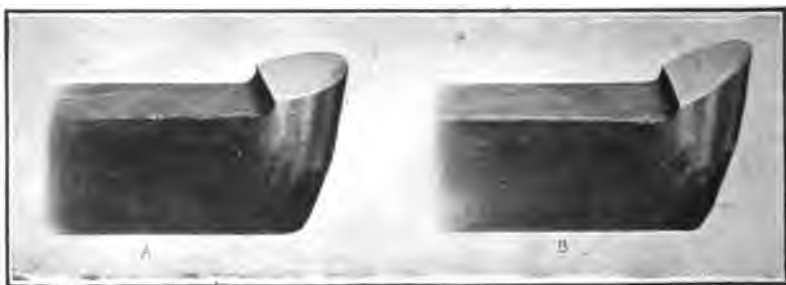
Fig. 37. (A) Blunt Tool for Turning Hard Steel. (B) Tool-point Ground to Give Keenness
