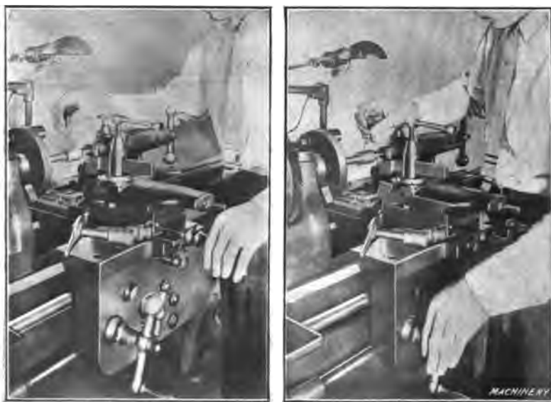
Fig. 11. Views showing how the Cross-slide and Carriage are Manipulated by Hand when Starting a Cut
