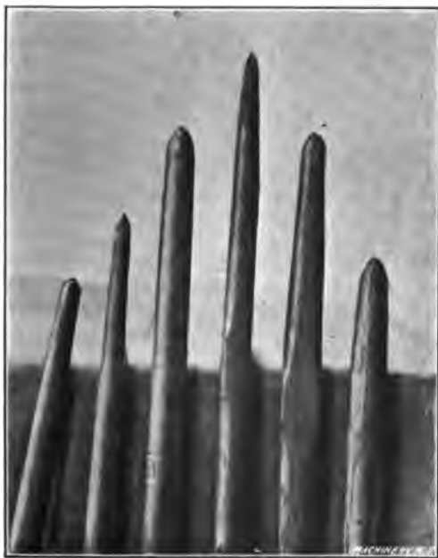
Fig. 44. Wooden Tools which are used on Large Thin Copper Blanks
