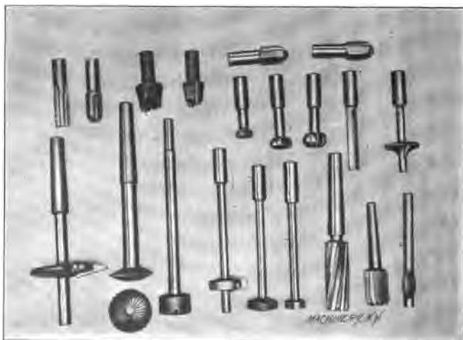
Fig. 46. Milling Tools Used in Die-sinking, with Examples of Fly-cutters
