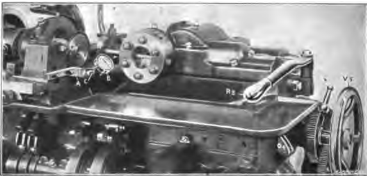
Fig. 33. Setting the Rising Block with the Aid of a Brown & Sharpe Dial Test Indicator
