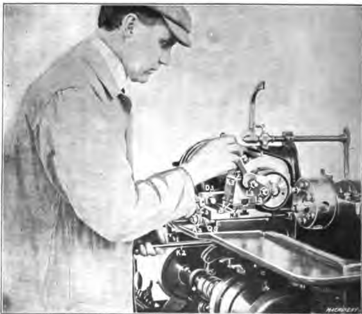
Fig. 21. Operator setting a Circular Form Tool
