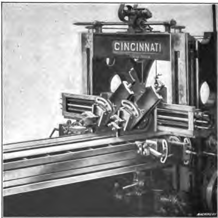
Fig. 12. Double-head Planer set for Planing Angular Surfaces
