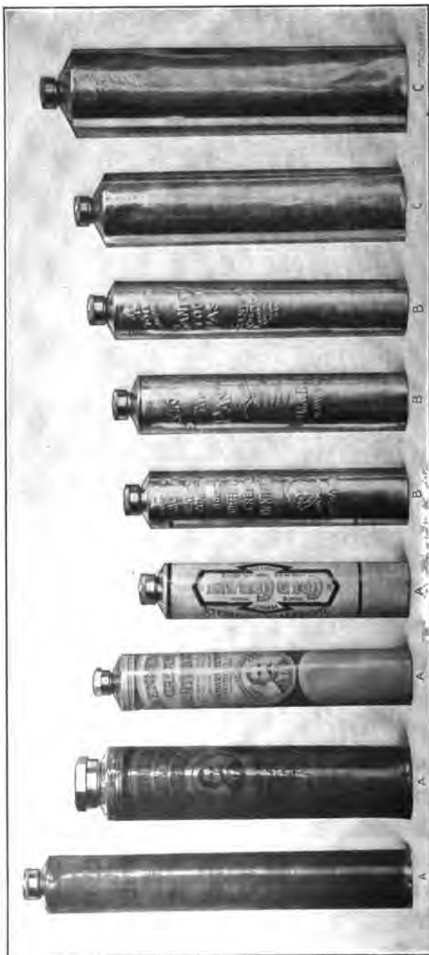
Fig. 89. Collapsible Tin Tubes made by Extrusion
