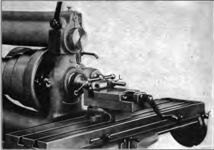
Fig. 25. Milling Slot with End Mill
