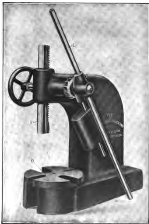
Fig. 26. Press for Forcing Mandrels into Work
