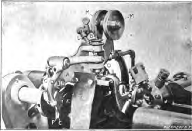
Fig. 10. Front View of the Index Drilling Attachment, placed on a No. 00 Brown & Sharpe Automatic Screw Machine
