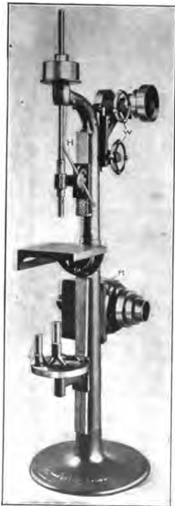
Fig. 28. Drill-press of the Sensitive Type
