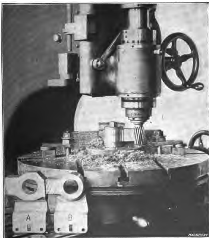
Fig. 23. Milling the Edge of a Steel Forging
