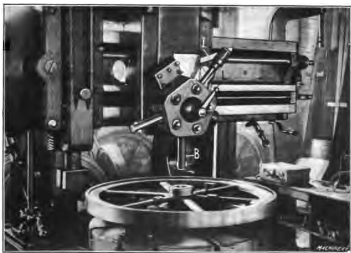
Fig. 10. Tool B set for Boring the Hub
