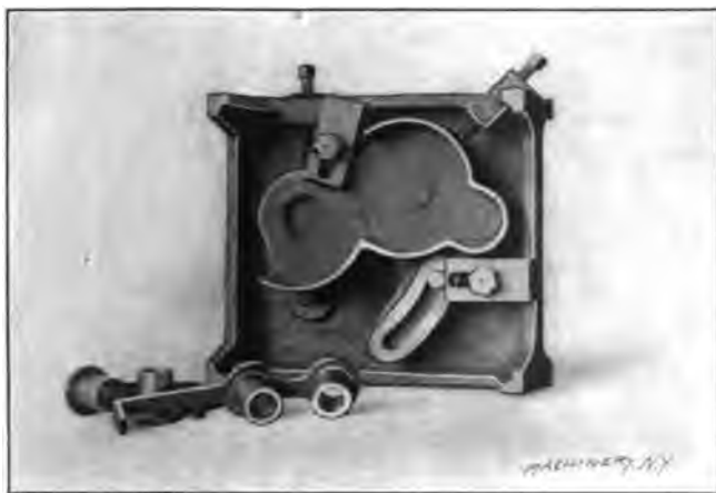
Fig. 1. Typical Open Drill Jig for Gear Guard
