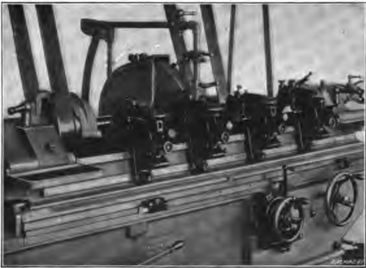
Fig. 12. Grinding Machine equipped with Four Universal Back-rests
