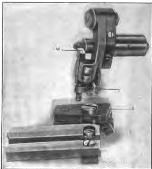
Fig. 18. Swing Tool for Delicate Turning
