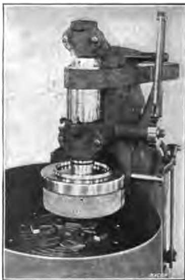
Fig. 29. Grinding Three Castings Simultaneously
