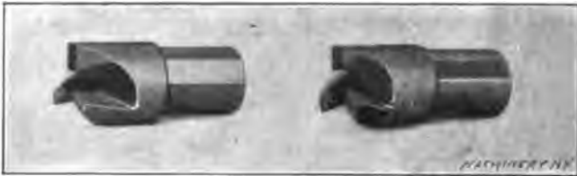
Fig. 21. Hollow Mills of the Solid Type
