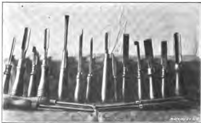
Fig. 45. Wood-turning Tools which are used in turning Spinning Chucks
