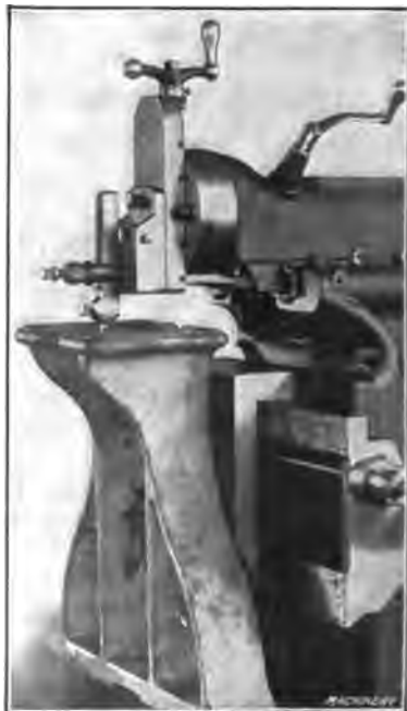
Fig. 46. Table removed and Casting Clamped to Cross-slide
