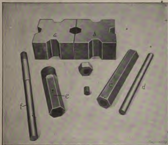
Fig. 42. Type of Dies and Tools used in making Hexagon Nuts in Center-feed Hot-pressed Nut Machine shown in Fig. 32
