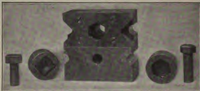
Fig. 12. Combination Square and Hexagon Double-deck Bolt Dies
