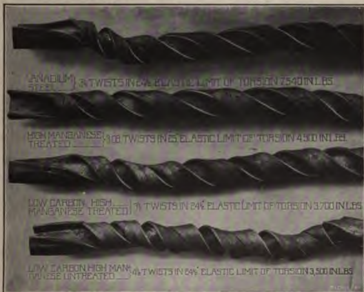
Fig. 3. Axle Steel Samples showing Difference in Physical Qualities. Length, 52 inches; Depth, 2 inches; Width, 1½ inch; Thickness of Flanges, 3/16 inch at Edge; 3/8 inch at Web; Thickness of Web, 3/16 inch
