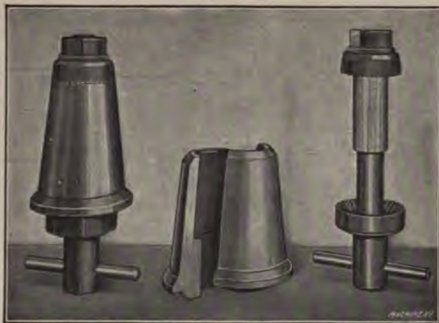
Fig. 7. Arbor for turning Tapered Bushings and Work for which it was designed
