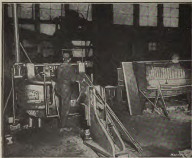
Fig. 15. 5-inch Ajax Forging Machine at Work in the Collinwood Shops of the L. S. & M. S. Railway, set up for making Coupler Pocket Filling Blocks for Freight Cars
