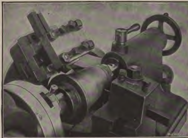
Fig. 8. Tools shown in Detail in Figs. 6 and 7, set up on Fay Automatic Lathe
