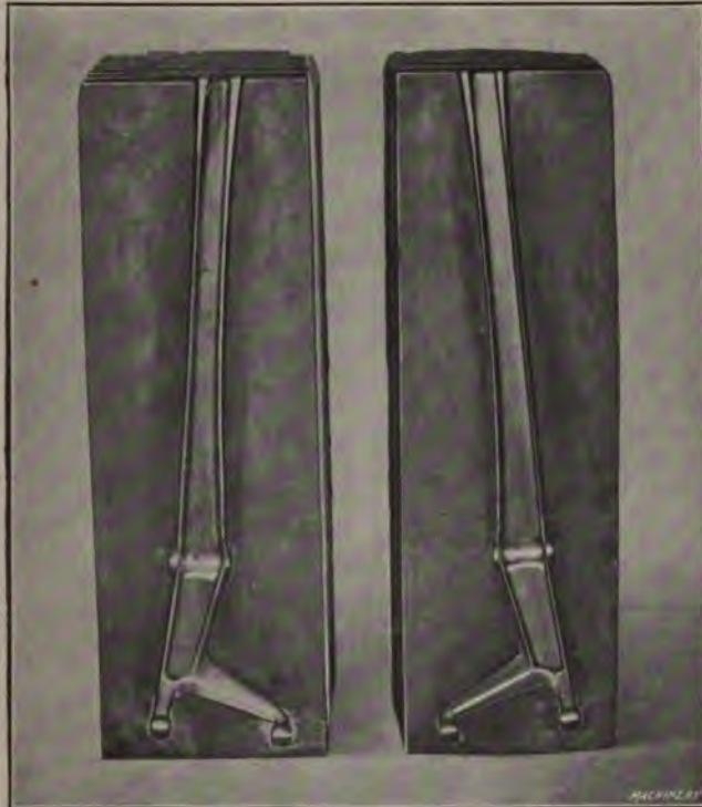
Fig. 20. Upper and Lower Dies used in Steam Hammer shown in Fig. 19 for finish-forming the Ford Front Axle
