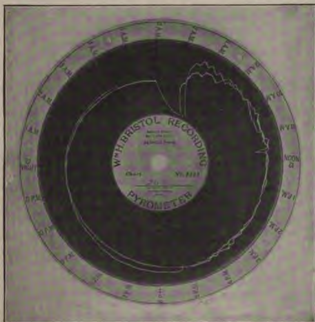
Fig. 3. Temperature Record obtained from an Annealing Furnace
