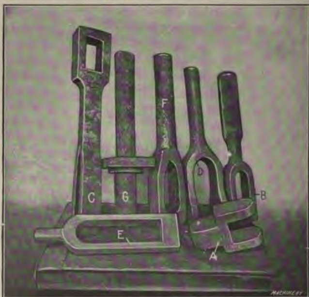
Fig. 25. Miscellaneous Examples of Lap-welding and Forming Operations accomplished on a 6-inch Ajax Universal Forging Machine
