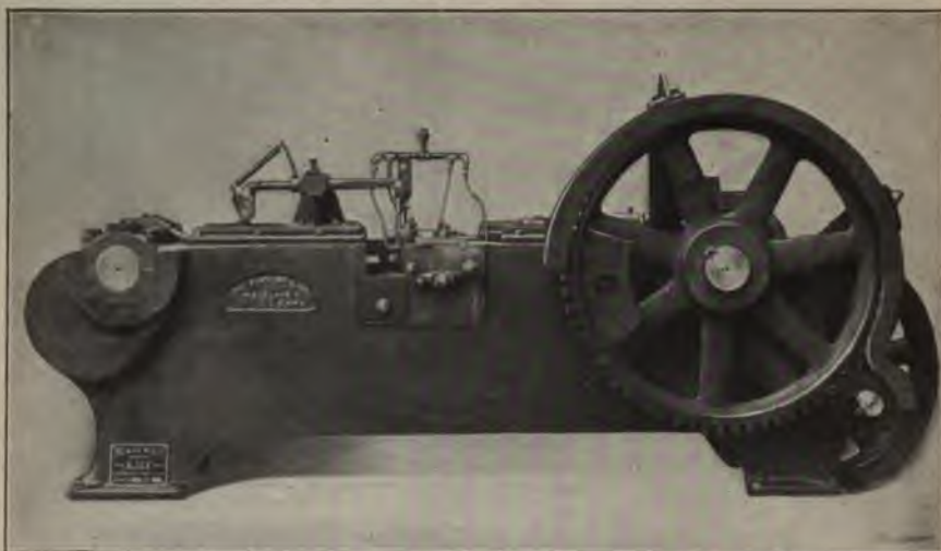
Fig. 34. Side View of "Ajax" Hot-pressed Center-feed Nut Machine showing Operating Side and Water Pipes for cooling Dies and Tools
