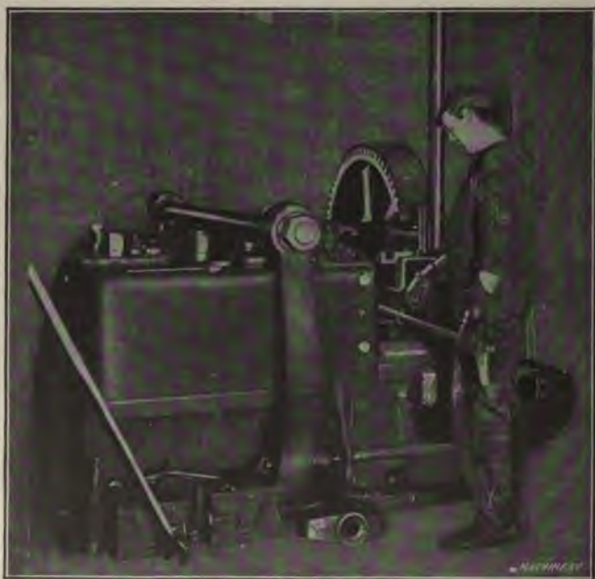
Fig. 17. "National" 3½-inch Forging Machine used in accomplishing the Preliminary Operations on the Ford Front Axle
