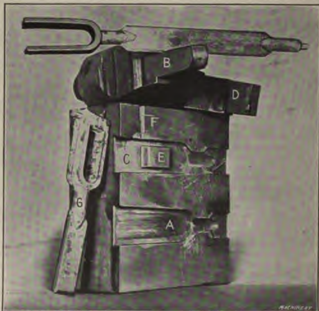
Fig. 30. Dies and Tools used in making Spring Hanger shown at B in Fig. 26—also illustrating Pin Welding Operation
