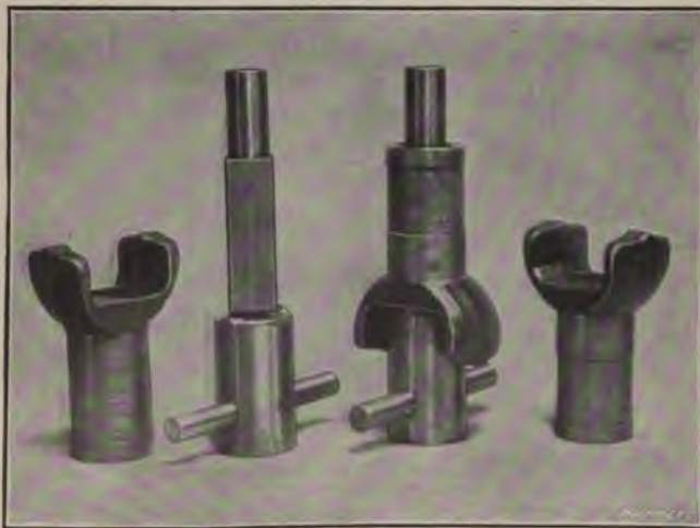
Fig. 12. Square Arbor for carrying Work with a Square Broached Hole
