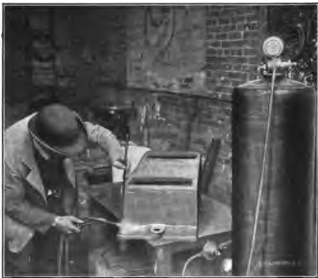
Fig. 5. Welding the Broken Flange of a Cast-iron Base. The Operator feeds the Joint with a Cast-iron Rod
