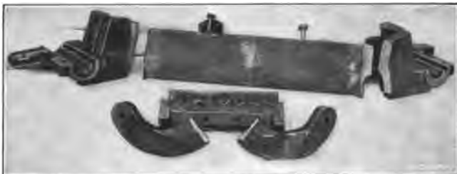
Fig. 5. Broken Casting from a Wood-working Machine
