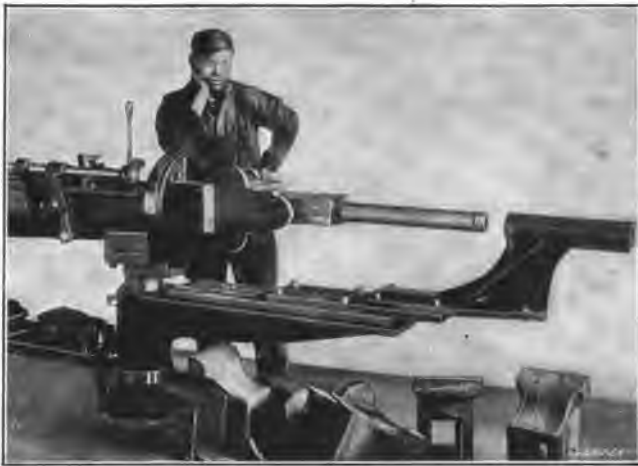
Fig. 15. Broaching Machine Finishing Rectangular Hole in Vise Body
