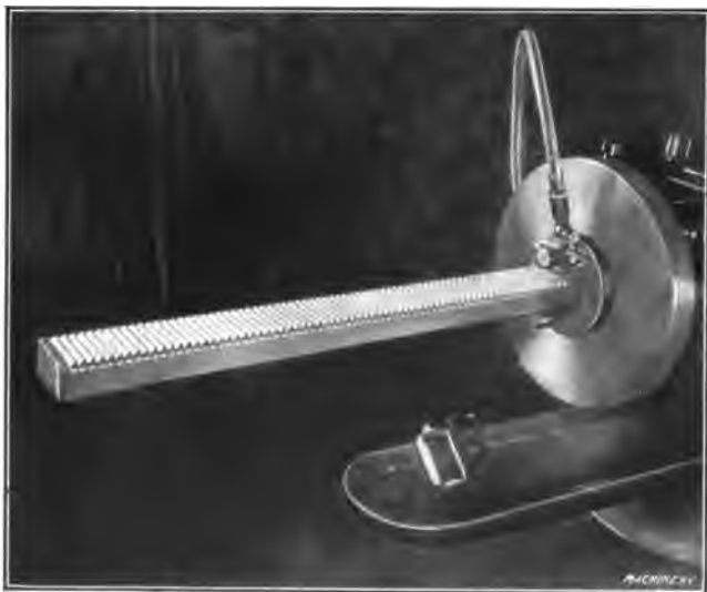
Fig. 13. Broach for Finishing Drop-forging shown in Fig. 14
