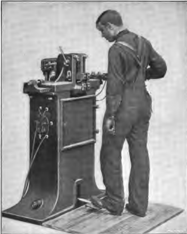
Fig. 3. Hand-operated Machine with Output of 250 Welds on Straight Stock with Welding Area Equivalent to \frac{3}{4} -inch Round Cross-section
