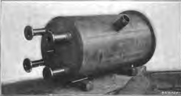
Fig. 1. Head, Flange and Branches welded in a 48-inch Tank with the Metallic Arc
