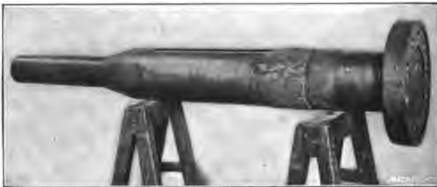
Fig. 2. A Built-up Fit on an Armature Shaft done with the Metallic Arc
