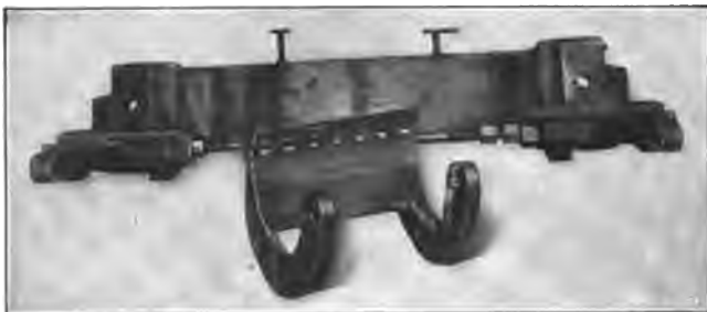
Fig. 6. Same Casting repaired with the Carbon Arc
