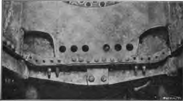
Fig. 3. Fractured Mud-ring of Locomotive Firebox prepared for making the Welds
