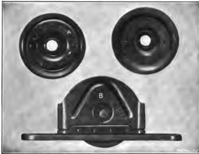
Fig. 5. Sash Pulley and Housing welded by the Point Method
