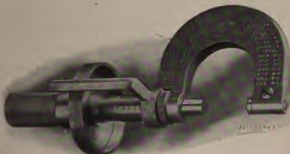
Fig. 24. Micrometer with Attachment for Reading Ten-thousandths of an Inch
