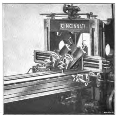
Fig. 12. Double-head Planer set for Planing Angular Surfaces
