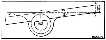
Fig. 39. Method of obtaining Helix Angle of Worm
