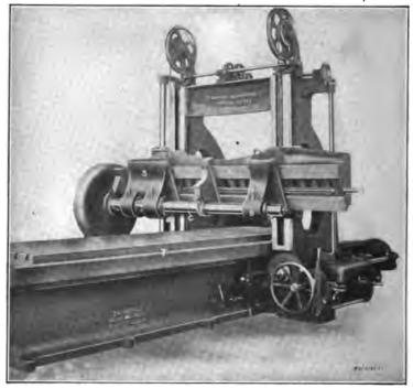
Fig. 80. Ingersoll Horizontal or Planer-type Milling Machine
