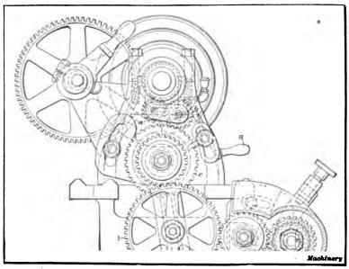
Fig. 26. Hnd View of Lathe Headstock
