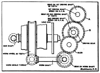
Fig. 2. Diagram of Gearing on the No. O Brown & Sharpe Automatic Screw Machine
