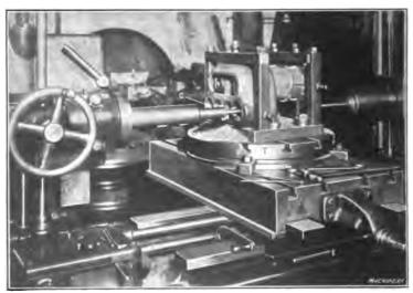
Fig. 81. Cylinder turned around for Machining Valve Seats
