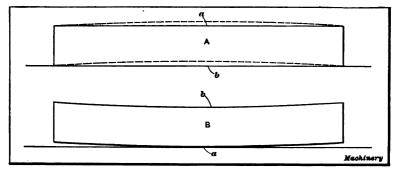
Fig. 88. Diagrams illustrating, on Exaggerated Scale, Distortion from Internal Stresses
