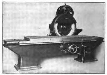
Fig. 25. Diamond Motor-driven Face Grinder
