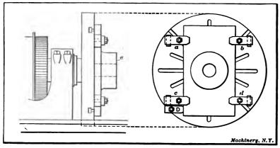
Fig. 88. Casting Clamped to Faceplate for Turning
