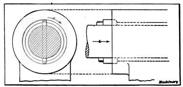
Fig. 24. Boring with a Flat Double-ended Cutter
