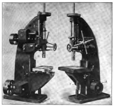
Fig. 82. Baker Bros. High-duty Type of Drilling Machine
