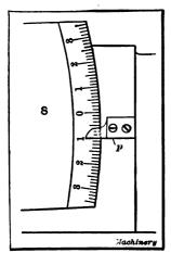
Fig. 11. Scale of Taper Attachment
