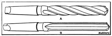
Fig. 26. A) Three-groove Drill. (B) Straight-fluted Drill
