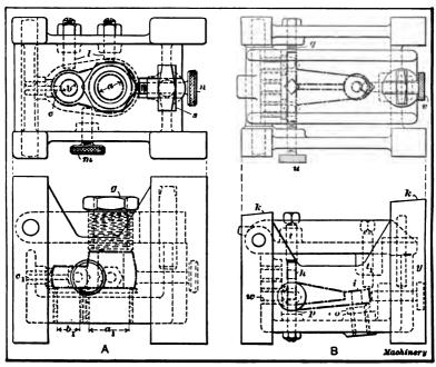
Fig. 15. Box Jigs for Drilling Parts shown by Heavy Dot-and-dash Lines
