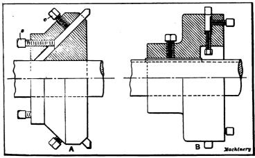
Fig. 27. Cutter-heads equipped with Adjustable Tools
