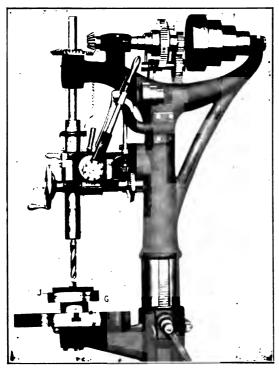
Fig. 10. Drill-press of the Wheel- and Lever-feed Type
