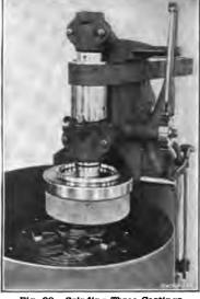
Fig. 28. Grinding Side of Saw Concave
