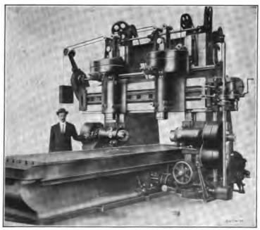
Fig. 84. Ingersoll Four-head Milling Machine
