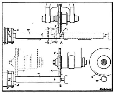
Fig. 1. (A) Diagram illustrating Method of Grinding by traversing Work past Face of Grinding Whoel. (B) Grinding by Traversing the Wheel
