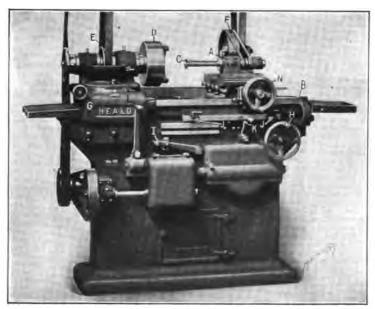
Fig. 22. Heald Internal Grinding Machine
