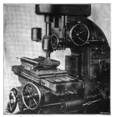
Fig. 20. Example of Milling on Vertical Milling Machine
