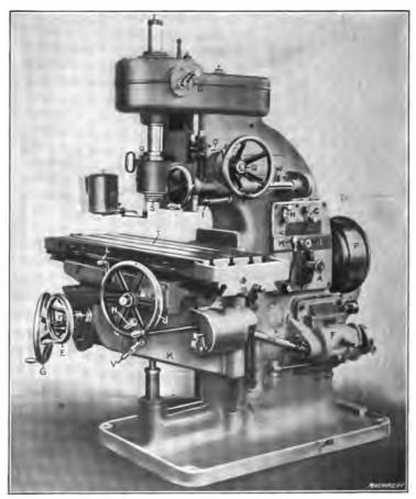
Fig. 19. Brown & Sharpe Vertical-spindle Milling Machine
