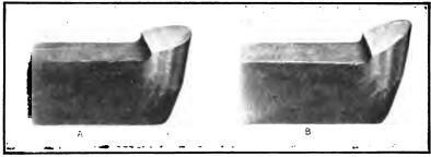
Fig. 87. (A) Blunt Tool for Turning Hard Steel. (B) Tool-point Ground to Give Keenness
