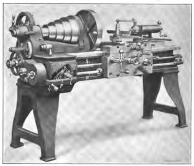
Fig. 40. Lethe Having Quick Change-gear Mechanism
