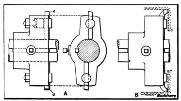
Fig. 25. Cutter-heads for Boring Large Holes
