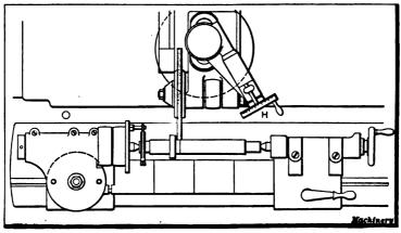
Fig. 18. Grinding Close to a Shoulder-Plan View
