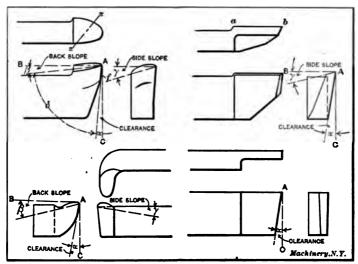
Fig. 88. Illustration showing the Meaning of Terms used in Tool Grinding as applied to Tools of Different Types
