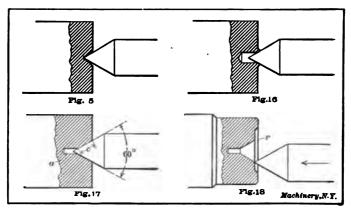
Figs. 15 to 18. Centers of Incorrect and Correct Form
