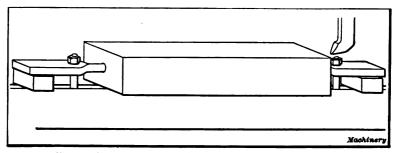
Fig. 10. Holding Block directly against Planer by Finger-clamps
