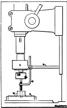
Fig. 28. Errington Automatic-reverse Tapping Chuck
