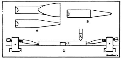
Fig. 26. Method of Holding Thin Flat Plates while Planing
