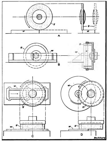
Fig. 28. Diagrams illustrating Four Methods of Surface Grinding
