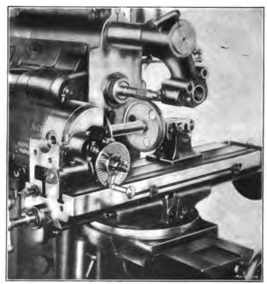
Fig. 88. Hobbing the Teeth of a Worm-wheel
