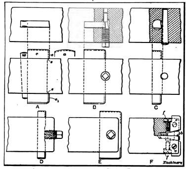
Fig. 28. Boring-cutters of Different Types
