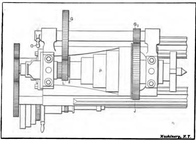
Fig. 2. Plan View of Headstock showing Back-gears
