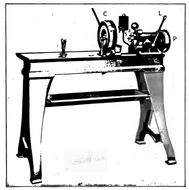
Fig. 19. Special Machine for Centering
