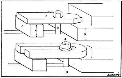
Fig. 17. Clamps for Attaching Work to Planer Platen
