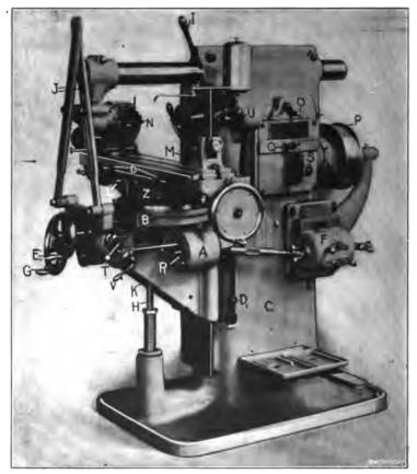
Fig. 28. Brown & Sharpe Universal Milling Machine
