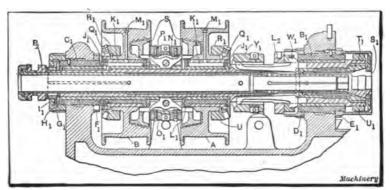
Fig. 5. Section through Spindle, Boxes. Pulleys, etc., of the No. 2
