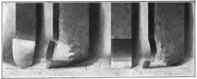
Fig. 40. Roughing and Finishing Tools
