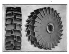
Fig. 18. Interlocking Side Milling Cutter
