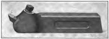
Fig. 40. Turning Tool with Inserted Cutter
