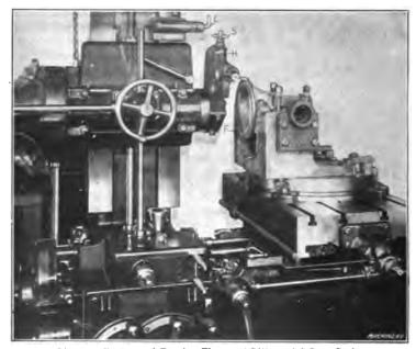
Fig. 38. Facing and Turning Flange of Differential Gear Casing
