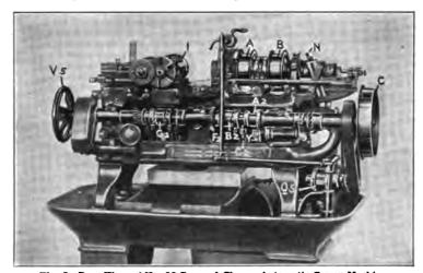
Fig. 2. Rear View of No. 00 Brown & Sharpe Automatic Screw Machine is slotted to hold hardened steel shoes  $P_1$  which bear on the hardened ends of the clutch levers.
