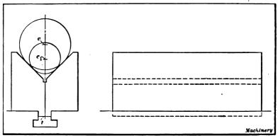
Fig. 27. V-block for Holding Cylindrical Parts
