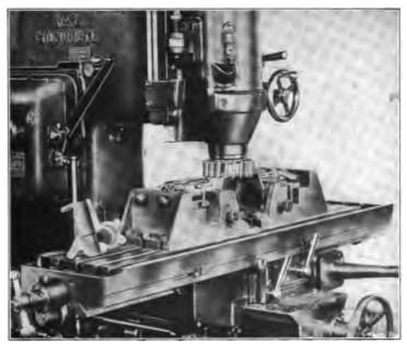
Fig. 27. Another Milling Operation Employing Two Fixtures
