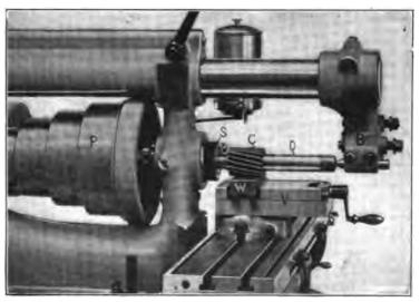
Fig. 8. Milling a Small Rectangular Block
