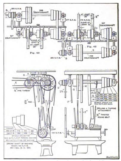
Figs. 42 and 48. Arrangement of Spindle Speeds for No. O Brown & Sharpe Automatic Screw Machines
