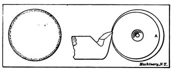
Fig. 21. Tool Steel should be centered Concentric, in order to remove the Decarbonized Outer Surface
