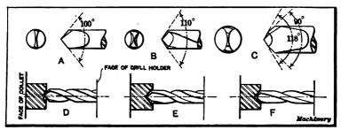
Fig. 25. Centering Tools-Incorrect and Correct Methods of Centering
