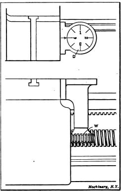
Fig. 59. Indicator used when Cutting Threads
