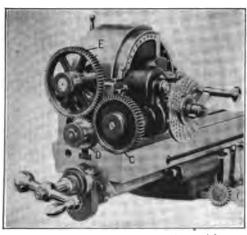
Fig. 2. Index Head geared for Differential Indexing
