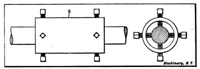
Fig. 51. Cat-head which is sometimes used as Bearing for Steadyrest
