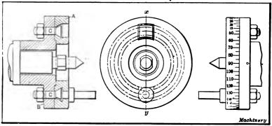
Fig. 29. Indexing Faceplate used for Multiple Thread Cutting
