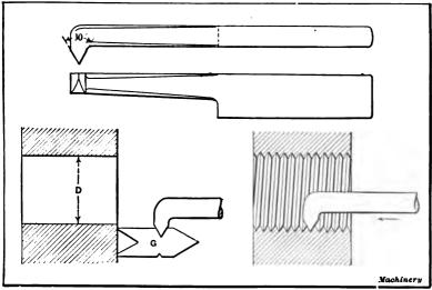
Fig. 81. Inside Thread Tool-Method of Setting and Using
