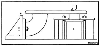
Fig. 25. Use of Angle-plate in Conjunction with Clamps for Holding Work
