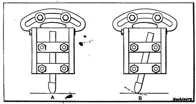
Fig. 18. Correct and Incorrect Positions for Planing Tool
