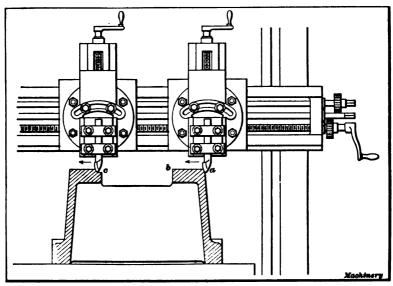
Fig. 15. Planing Two Surfaces Simultaneously with Two-head Planer
