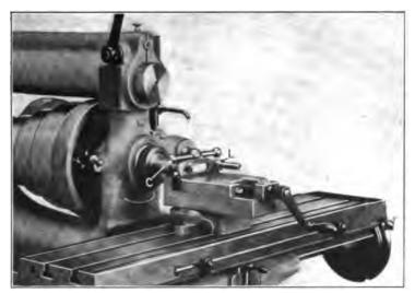
Fig. 25. Milling Slot with End Mill
