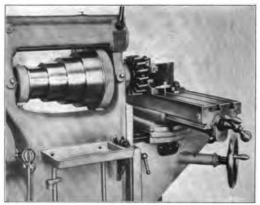
Fig. 27. Finishing Vertical Surface with Face Mill
