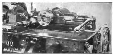
Fig. 88. Setting the Rising Block with the Aid of a Brown & Sharpe Dial Test Indicator
