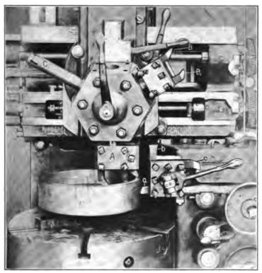
Fig. 18. Turning Gasoline Engine Flywheel on Vertical
