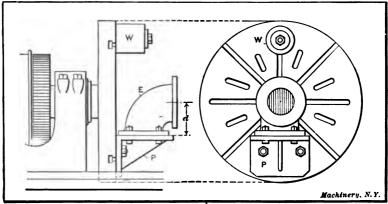
Fig. 89. Work Held on Angle-plate attached to Faceplate
