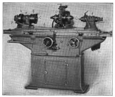
Fig. 2. Brown & Sharpe Universal Cylindrical Grinding Machine
