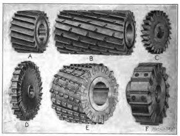
Fig. 8. Cylindrical, Side, and Face Milling Cutters
