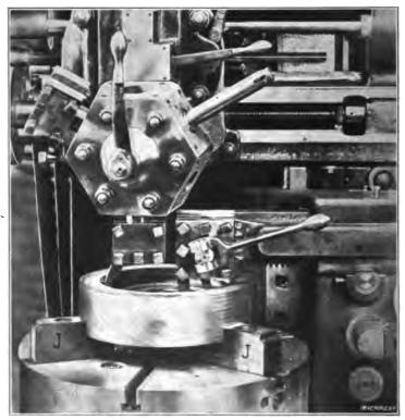
Fig. 19. Turning Gasoline Engine Flywheel-Second Position
