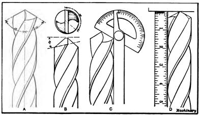
Fig. 83. Views showing Angles to be Considered when Grinding Drills, and Methods of Measuring Lip Angle and Clearance
