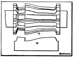
Fig. 16. Formed Cutter for Milling Part W
