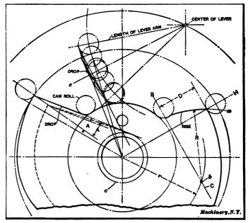
Fig. 4. Method of Laying out-Rise and Fall on-Came
