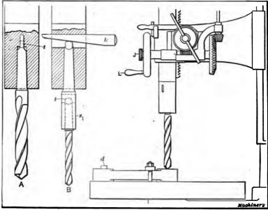
Fig. 4. Method of Holding and Driving Taper-shank Drills.
