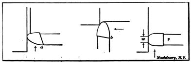
Fig. 29. Top of Tool should Slope away from Working Part of Cutting Edge
