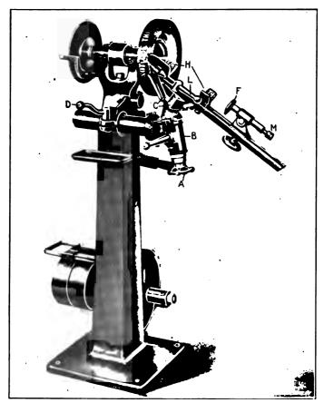
Fig. 86. Grinder for Sharpening Drills
