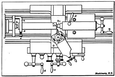
Fig. 5. Plan View showing Work Mounted Between Centers
