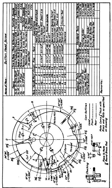
Fig. 40. Setting-up Chart for making a Button Head Screw on the No. 00 Brown & Sharpe Automatic Screw Machine
