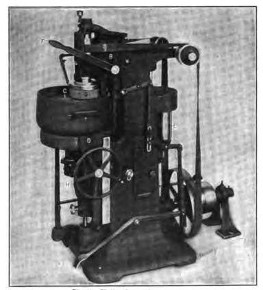
Fig. 27. Walker Rotary Surface Grinder
