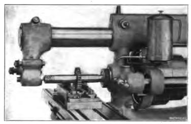
Fig. 14. Milling Groove with Interlocking Cutter
