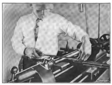
Fig. 12. Filing Work after Finishing Cut is taken
