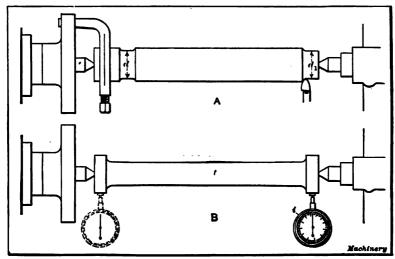
Fig. 48. Two Methods of Aligning Centers for Cylindrical Turning
