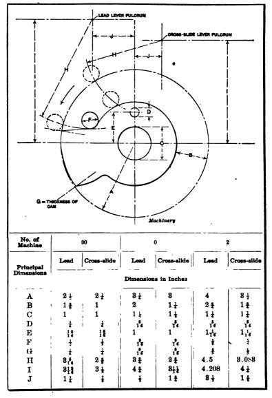
Generally the rise can be abrupt for about three-quarters of the way, and then gradually slow down as the tool approaches the work. A good method of laying out a curve of this form is shown in Fig. 4. The reason for making a curve of this form is that less time is necessary for one tool to clear another, which sometimes makes quite a considerable difference in the time required to produce one piece.
