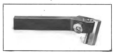
Fig. 46. Threading Tool
