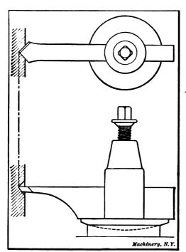
Fig. 35. Special Tool which Forms a Center for Starting the Drill
