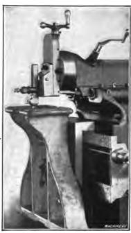
Fig. 46. Table removed and Casting Clamped to Cross-slide
