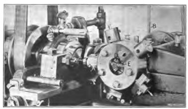
Fig. 87. Ratio Threading Attachment
