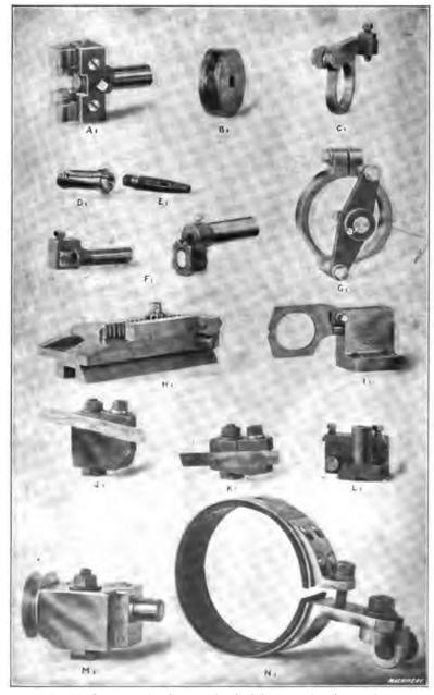
Fig. 89. Representative Group of Standard Tools and Attachments for the Brown & Sharpe Automatic Screw Machines
