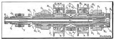
Fig. 4. Section through Spindle, Boxes, Pulleys, etc., of the No. 00 Brown & Sharpe Automatic Screw Machine
