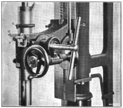
Fig. 1. Drill Spindle Feeding and Automatic Trip Mechanism
