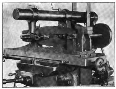
Fig. 18. Milling Slot of Crank-shaper Rocker-arm
