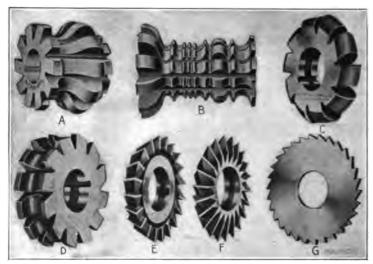
Fig. 10. Formed Cutters, Angular Cutters, and Slitting Saw
