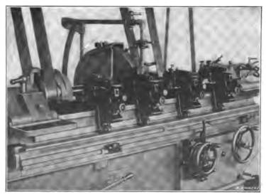
Fig. 12. Grinding Machine equipped with Four Universal Back-rests
