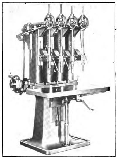
Fig. 29. Henry & Wright Multiple-spindle Drilling Machine
