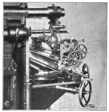
Fig. 12. Universal Machine arranged for Spiral Milling
