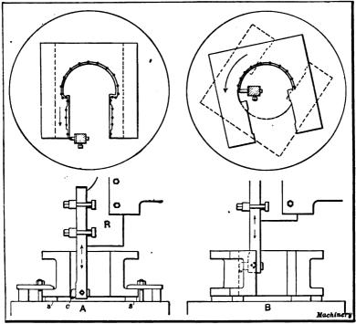
Fig. 50. Example of Straight and Circular Slotting
