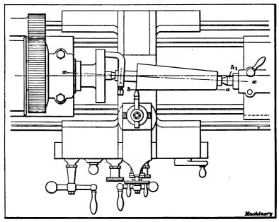
Fig. 1. Taper Turning by the Offset-center Method
