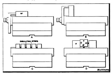
Fig. 81. End Views illustrating Different Methods of holding Work on Magnetic Chuck
