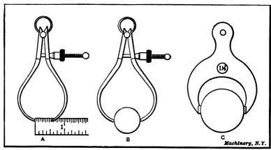
Fig. 10. Setting Calipers by Scale—Setting by Gage—Fixed Gage
