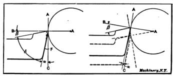
Figs. 85 and 86. Illustrations showing how Effective Angles of Slope and Clearance change as Tool is raised or lowered
