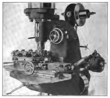
Fig. 28. Becker Vertical-spindle Machine for Continuous Circular Milling
