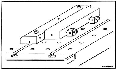
Fig. 22. Work held between Stop-pins and Strip Bolted to Platen
