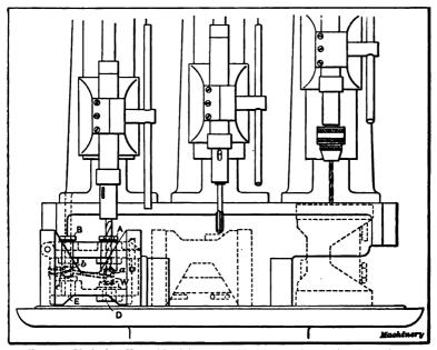
Fig. 80. Method of Using Multiple-spindle Machine for Successive Operations
