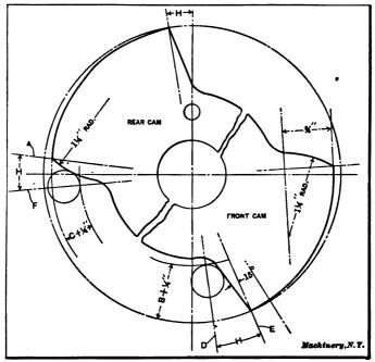
Fig. 6. Method of Determining Clearance on Cross-slide Cams
