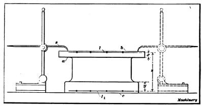
Fig. 86. Testing Alignment by using Surface Gage
