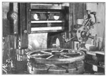
Fig. 9. Turning the Rim of a Flywheel
