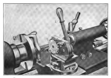
Fig. 82. Rivett-Dock Circular Threading Tool in Working Position
