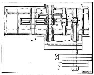
Fig. 2. Driving Mechanism of a Spur-geared Planer
