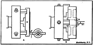
Fig. 28. Radial Facing-Boring Pulley Hold in Chuck
