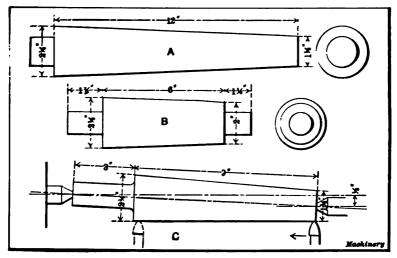
Fig. 2. Examples of Taper Work
