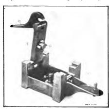
Fig. 18. Drill Jig of the Box Type
