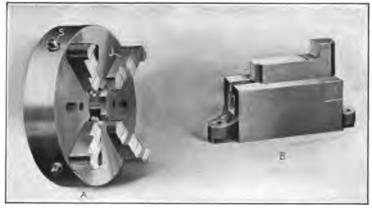
Fig. 27. Chuck and Faceplate Jaw
