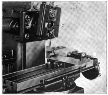
Fig. 84. Slotting Attachment applied to a Milling Machine
