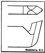
Fig. 49. Diamond-point Turning Tool
