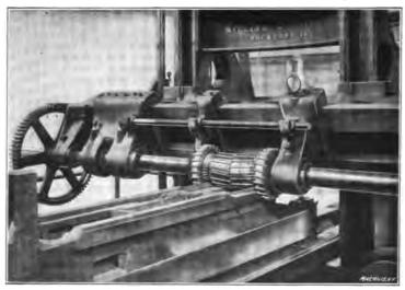
Fig. 81. Milling the Ways of a Turret Lathe Bed on a Horizontal Machine same general character, so that a great capacity or "range" is not needed. The Lincoln type is used very effectively in connection with the manufacture of firearms, sewing machines, electrical instruments and many other kinds of machinery.
