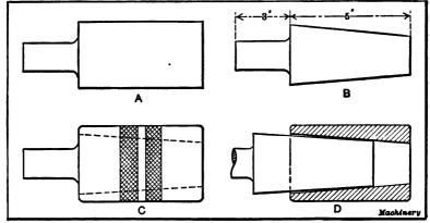
Fig. 4. Taper Plug and Gage
