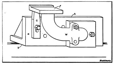
Fig. 24. Odd-shaped Casting attached to Angle-plate
