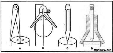
Fig. 18. Centering End with Punch preparatory to Drilling
