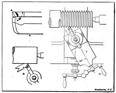
Fig. 61. Cutting Thread by using Compound Rost
