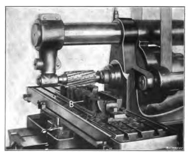
Fig. 7. Milling Cast-iron Bearing Caps
