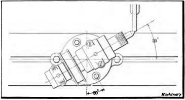
Fig. 20. Truing Conical Center of a Universal Grinder
