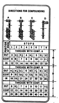
Fig. 48. Index Plate showing Positions of Control Levers for Cutting Threads of Different Pitch
