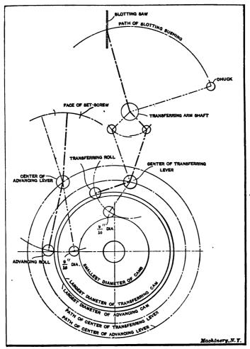
Fig. 14. Diagram used in laying out Transferring and Advancing Cams for the No. O Brown & Sharpe Automatic Screw Machine
