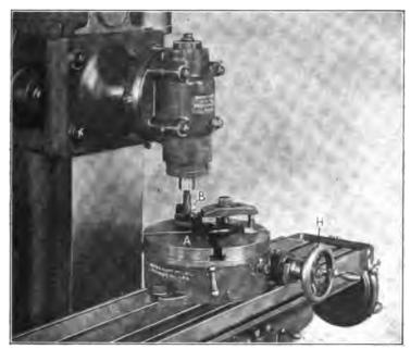
Fig. 86. Combined use of Vertical and Circular Milling Attachments
