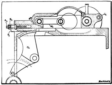
Fig. 14. Partial Section of No. 2 Machine showing Operation of Turret Slide
