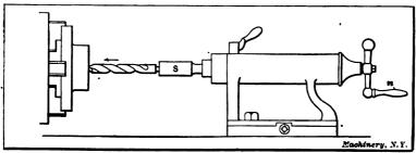
Fig. 34. Drilling in the Lethe
