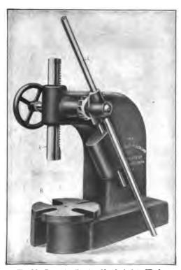
Fig. 26. Press for Forcing Mandrels into Work
