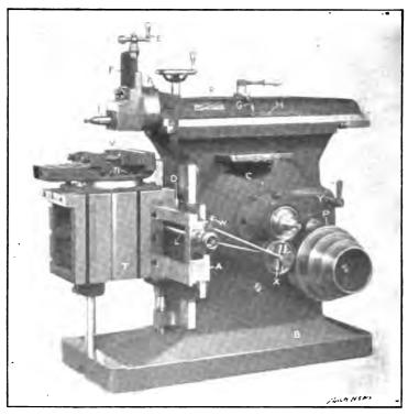
Fig. 42. Cincinnati Back-geared Crank Shaper
