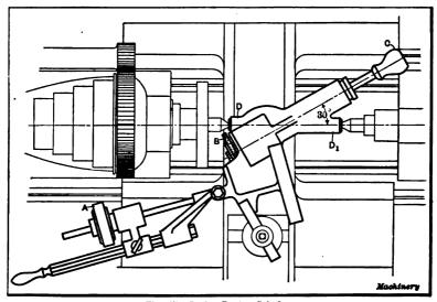
Fig. 47. Lathe Center Grinder
