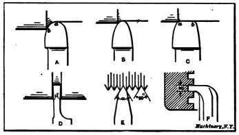
Fig. 84. Plan View of Lathe Turning and Threading Tools
