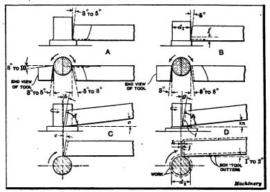
Fig. 24. Outting-angles for Box Tool Outters
