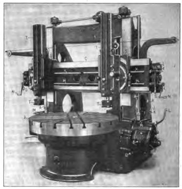
Fig. 1. Gisholt Vertical Boring and Turning Mill
