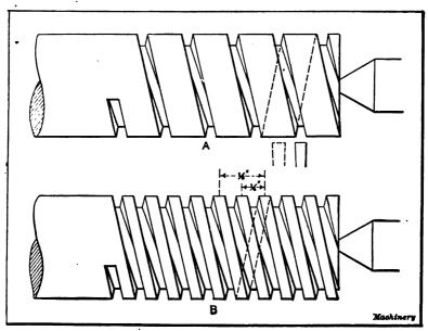
Fig. 28. Views illustrating how a Double Square Thread is Out
