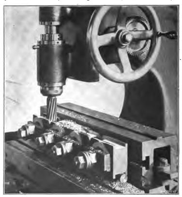
Fig. 22. Milling Connecting-rod Bearing Brasses on Becker Vertical Machine same position. The vertical milling machine used for this operation, is not the same as the one previously illustrated, although its construction is very similar and it is used for the same class of work.
