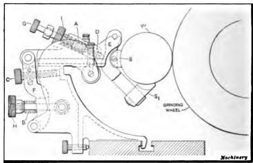
Fig. 11. Universal Back-rest for Supporting Work being Ground
