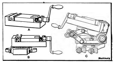
Fig. 5. Milling Machine Vises
