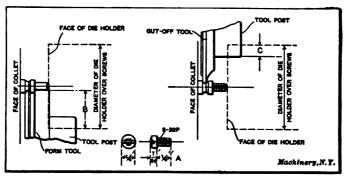
Fig. 5. Diagram illustrating Method of Finding Clearance for Die Holder
