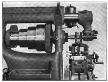
Fig. 82. Straddle Milling a Square Bolt-head
