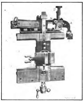
Fig. 9. A Lathe Taper Attachment
