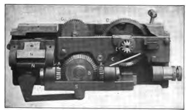
Fig. 4. Rear View of Lathe Apron
