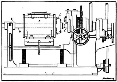
Fig. 29. Cylinder mounted on Korisontal Machine for Boring
