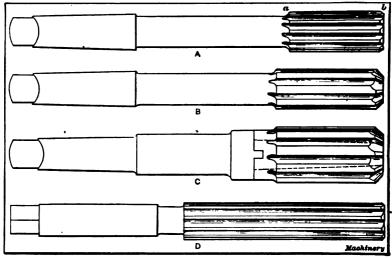
Fig. 8. Reamers of Different Styles
