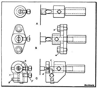
Fig. 26. Various Types of Centering Tool Holders
