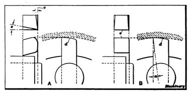
Fig. 28. Boring Tools for Roughing and Finishing Cuts
