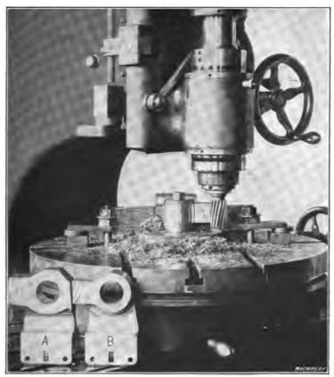
Fig. 28. Milling the Edge of a Steel Forging
