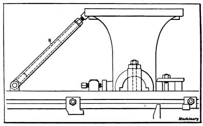
Fig. 21. High Work supported by Brace which takes Thrust of Cut
