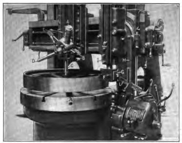
Fig. 12. Gisholt Mill equipped with Convex Turning Attachment
