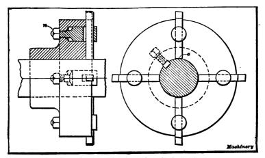
Fig. 26. Cutter-head with Four Boring Tools
