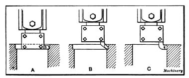
Fig. 6. Boring with Regular Turning Tools
