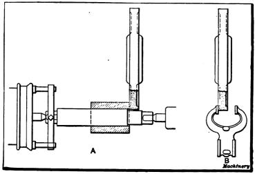
Fig. 17. Grinding with Side of a Recessed Wheel
