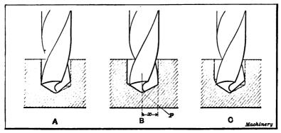
Fig. 84. Three Examples of Incorrect Drill Grinding
