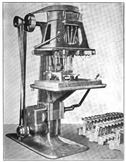
Fig. 81. Pratt & Whitney Adjustable Multiple-spindle Drilling Machine
