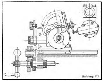
Fig. 15. Diagrammatical View showing Method of Milling Cams on the Milling Machine
