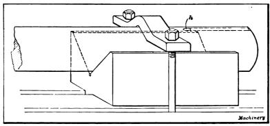
Fig. 28. End of Shaft Clamped in V-block
