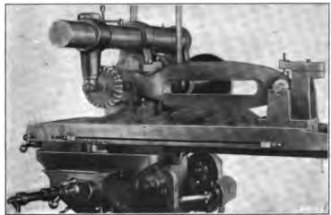
Fig. 19. Finishing End of Rocker-arm with Straddle Mill
