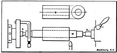
Fig. 24. Bushing mounted on Mandrel for Turning
