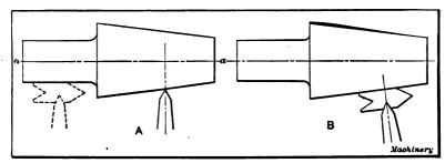
Fig. 80. Correct and Incorrect Positions of Tool for Taper Thread Cutting
