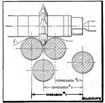
Fig. 7. Cutter for Milling the Teeth of Spur Gears
