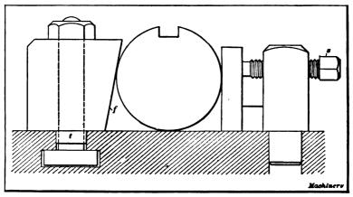
Fig. 80. Method of Holding Shaft for Splining or Keyseating
