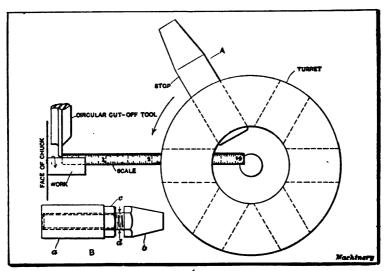
Fig. 22. Simple Method for setting a Stop
