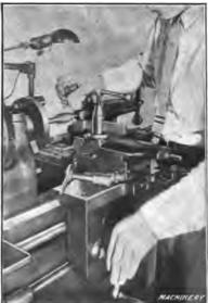
Fig. 11. Views showing how the Cross-slide and Carriage are Manipulated by Hand when Starting a Cut
