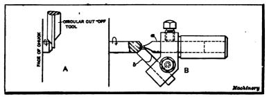
Fig. 28. Chamfering the End of the Work
