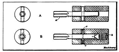
Fig. 28. Floating Reamer Holders
