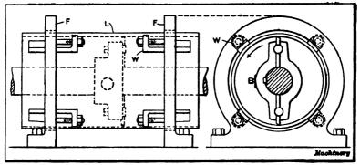
Fig. 85. Cylinder Lining Mounted in Fixture for Boring
