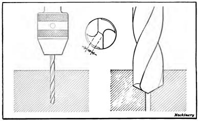
Fig 25. Pressure for Feeding Large Drill can be reduced by Dailling Small "Lead Hole"
