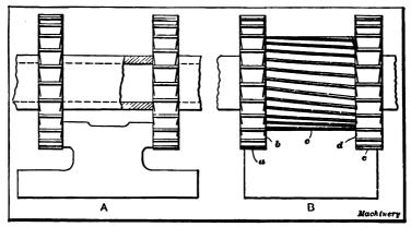
Fig. 17. (A) Straddle Milling. (B) Gang Milling
