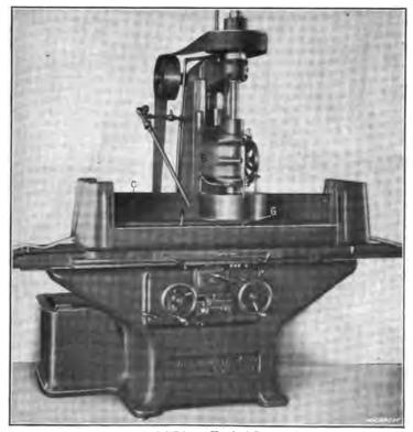
Fig. 26. Pratt & Whitney Vertical Surface Grinder
