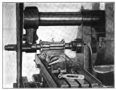
Fig. 15. Example of Form Milling
