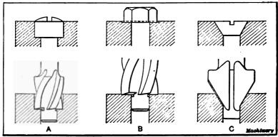
Fig. 18. Use of Counterbore and Countersink
