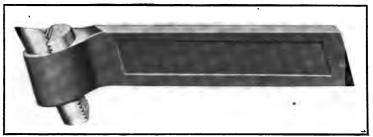
Fig. 48. Heavy Inserted-cutter Turning Tool
