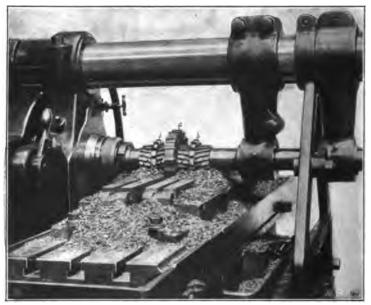
Fig. 22. Milling Two Parts Simultaneously
