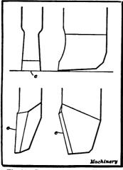
Fig 41. Square-nose Tool—Side-tool with Sloping Edge
