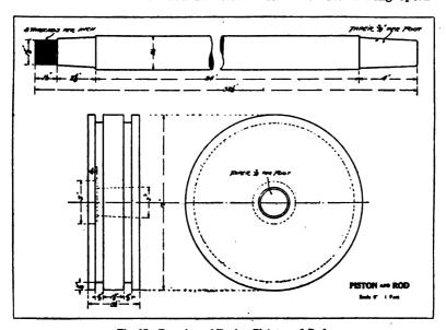
Fig. 15. Drawing of Engine Piston and Rod
