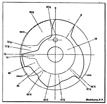
Fig. 8. Commendable Method of Laying out Cams
