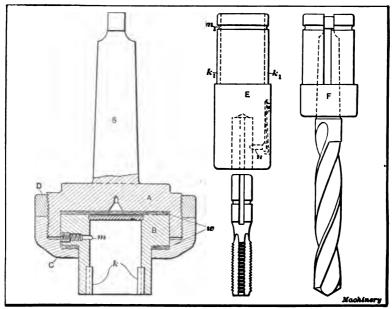
Fig. 21. Beaman & Smith Safety Drill- and Tap-holder
