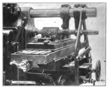
Fig. 20. Example of Gang Milling
