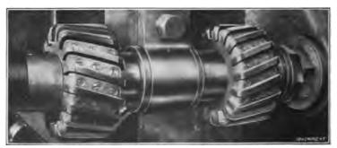
Fig. 83. Cutters used for Channeling Main-rods
