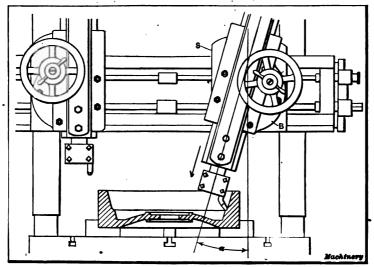
Fig. 18. Turning a Taper or Conical Surface
