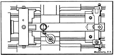
Fig. 53. Testing Work with Dial Indicator
