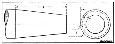
Fig. 12. Tool Point should be in same Horizontal Plane as Axis of Work for Taper Turning
