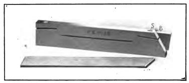
Fig. 44. Parting Tool with Inserted Blade
