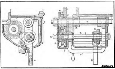
Fig. 42. Sectional Views of Quick Change-gear Mechanism
