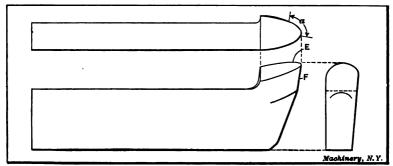
Fig. 9. Tool used for Cylindrical Turning
