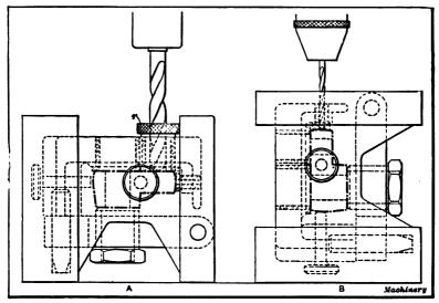
Fig. 16. Method of Using Jig
