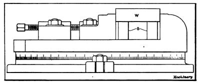
Fig. 28. Illustration showing use of Parallel Strips
