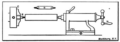
Fig. 14. Drilling Centers in the Lethe
