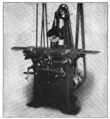
Fig. 24. Walker Surface Grinder of Reciprocating Type
