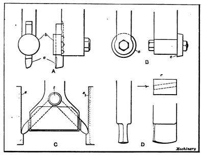
Fig. 89. (A) Planing Tool with Inserted Cutter. (B) Radius Tool (C) Tool having Two Cutters. (D) Finishing Tool
