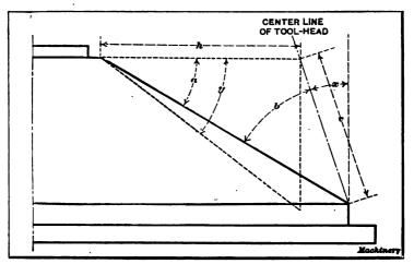
Fig. 15. Diagram showing Method of Obtaining Angular Position of Tool-head when Turning Conical Surfaces by using Vertical and Horisontal Feeding Movements
