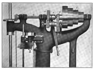
Fig. 8. Back-gearing and Feed Change-gears of Upright Drilling Machine
