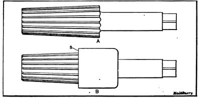
Fig. 18. Plain Reamer-Reamer with Stop Sleeve
