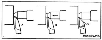
Fig. 22. Three Methods of Facing the End Square
