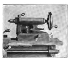
Fig. 8. Detail View of Lathe Tailstock
