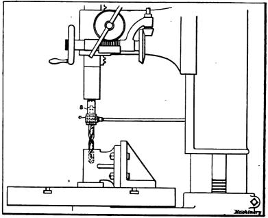
Fig. 24. Method of Applying Oil-tube Drill to Drill-press
