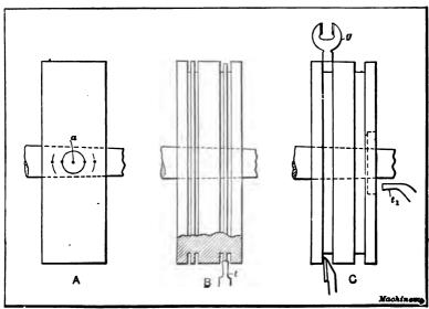
Fig. 20. Successive Steps in Turning Packing-ring Grooves
