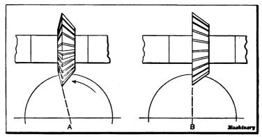
Fig. 14. Double- and Single-angle Cutters
