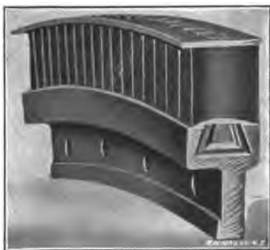
Fig. 46. Method of Attaching Blades of Curtis Turbine to Periphery of Wheel
