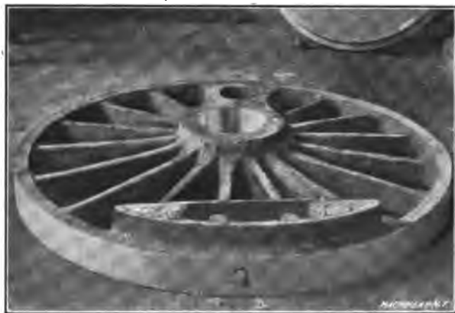
Fig. 20. The Counterweight Poured into Open Chambers
