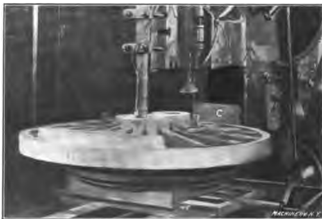
Fig. 22. Keyseating in the Slotting Machine with Special Squaring Plate for Setting the Work
