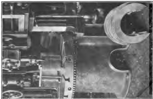
Fig. 40. Turning a Stack of Liners on the Boring Mill, after Facing
