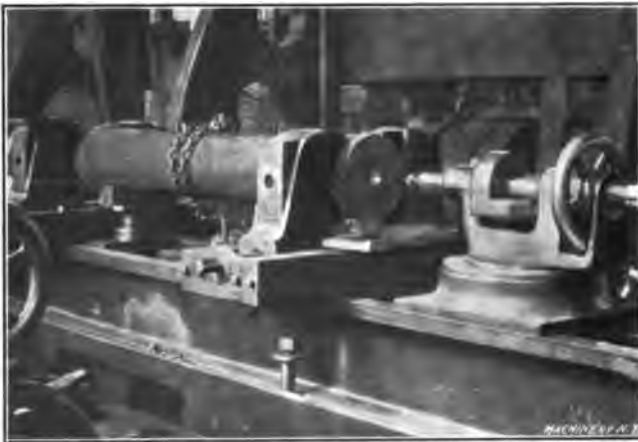
Fig. 8. Centering the Axle Preparatory to Turning
