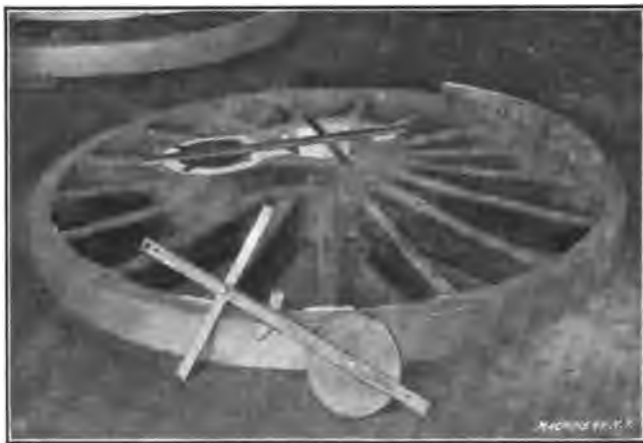
Fig. 21. Laying out the Keyseat for the Crankpin with Special Templet
