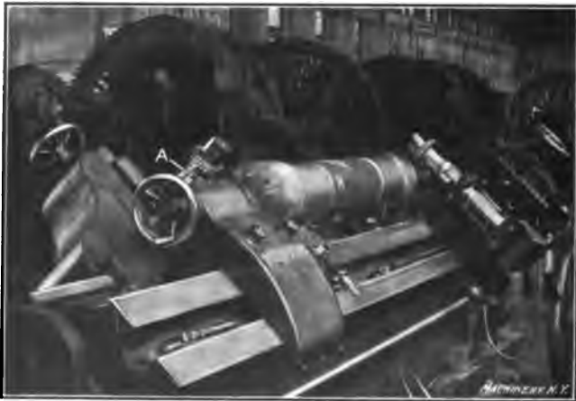
Fig. 11. Keyseating the Axles on a Special Quartering Milling Machine
