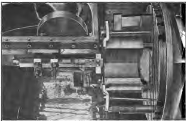
Fig. 42. Machining the Bore of a Stack of Liners on the Slotter
