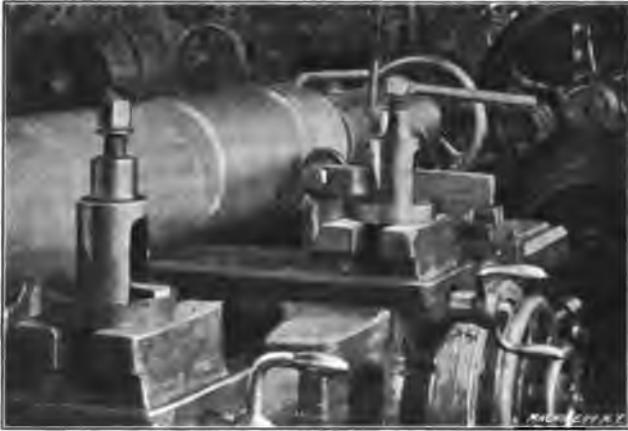
Fig. 10. Finishing the Axle Journals with the Rolling Tool
