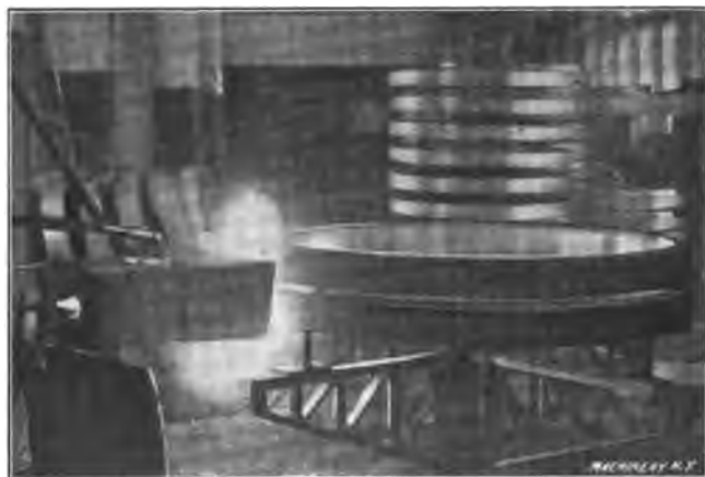
Fig. 26. Heating the Tires on a Turntable for Shrinking onto the Centers
