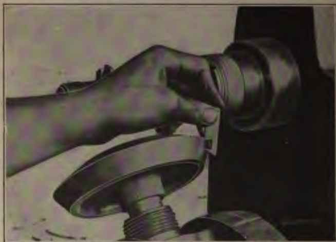
Fig. 10. Marking the Depth of Tooth with Depth Gage
