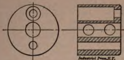
Fig. 50. Work to be Drilled in Jig, Fig. 51
