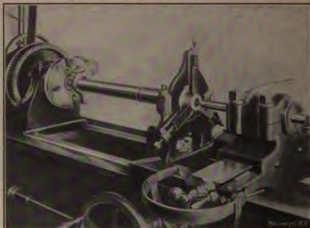
Fig. 80. Truing the Hole in the End of the Spindle with Boring Tool
