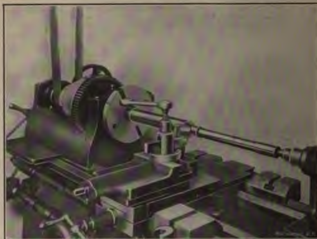
Fig. 81. Accurate Method of Testing Hole in Spindle
