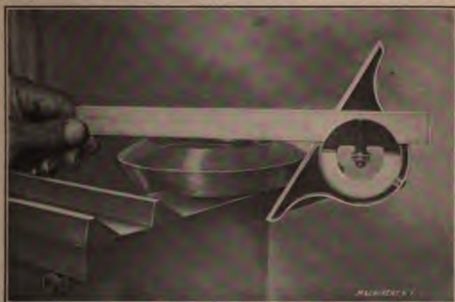
Fig. 6. Testing the Accuracy of the Angles
