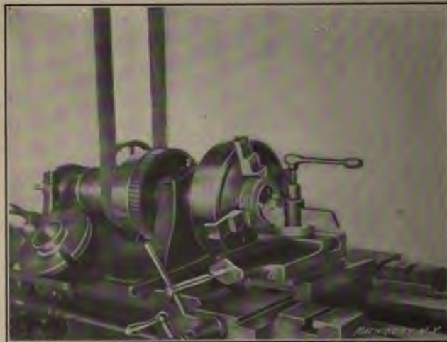
Fig. 40. Roughing the Bottom of the Recess
