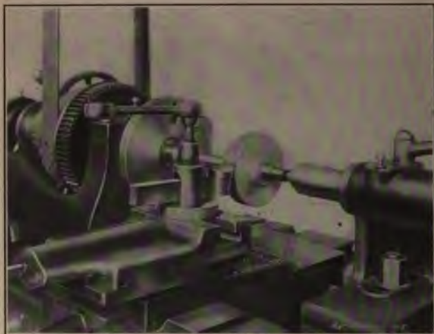
Fig. 47. Radius Tool for Tooth Surface
