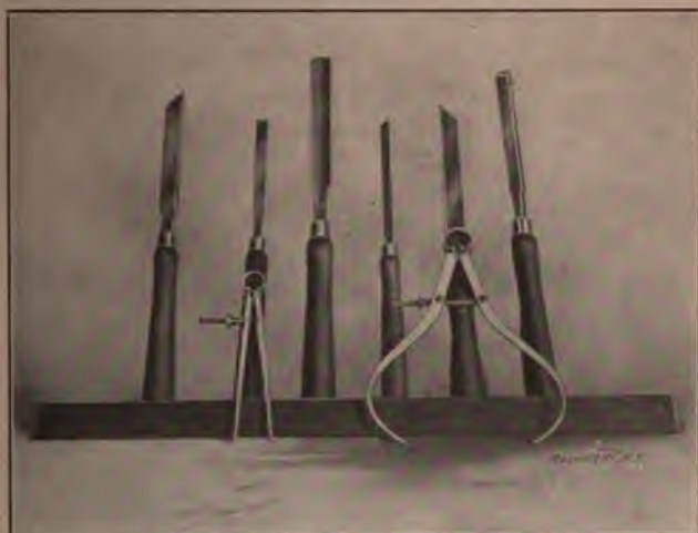
Fig. 29. Tools Used by Patternmaker
