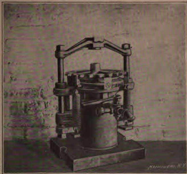
Fig. 64. Pneumatic Clamping Jig used for Drilling Sprocket Wheel
