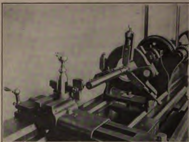
Fig. 65. Use of Test Bar and Indicator
