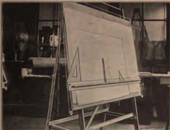
Fig. 36. Compact Drawing Board having Independent Vertical Adjustments for Board and Straight-edge
