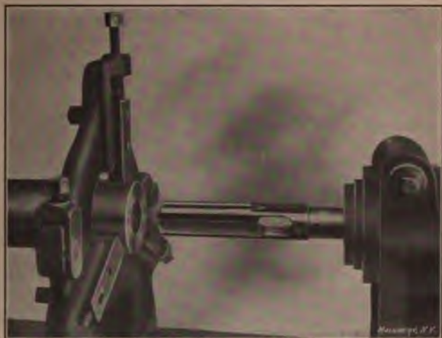
Fig. 78. Showing the Guide Drawn back to Expose the Drill
