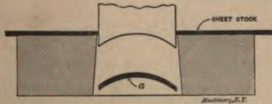
Fig. 54. Punching and Bending at One Operation
