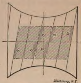
Fig. 29. Surfaces of Contact of the Hindley Worm
