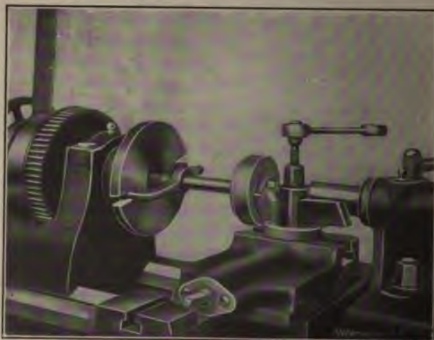
Fig. 44. Roughing the Outer Face
