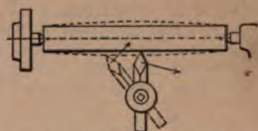
Fig. 6. Correct and Incorrect Setting of Tool
