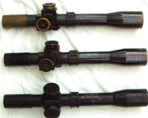
Three No.32 scopes: (top) a Mk1, (centre) a Mk2 and (bottom) a Mk3. It is easy to tell a Mk3 from the earlier scopes as its adjustment drums are in-line with each other while the drums on the earlier scopes are offset and require closer examination to tell them apart
