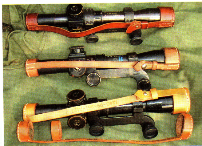
The leather lens caps with the metal stud were used throughout the life of the No.32 scope. The one on the bottom scope has a NATO number on it. The very bottom set of caps is modified by moving the retaining ring on a set of No.42 or No.53 scope lens caps – a common modification and one way of not losing the lens caps
