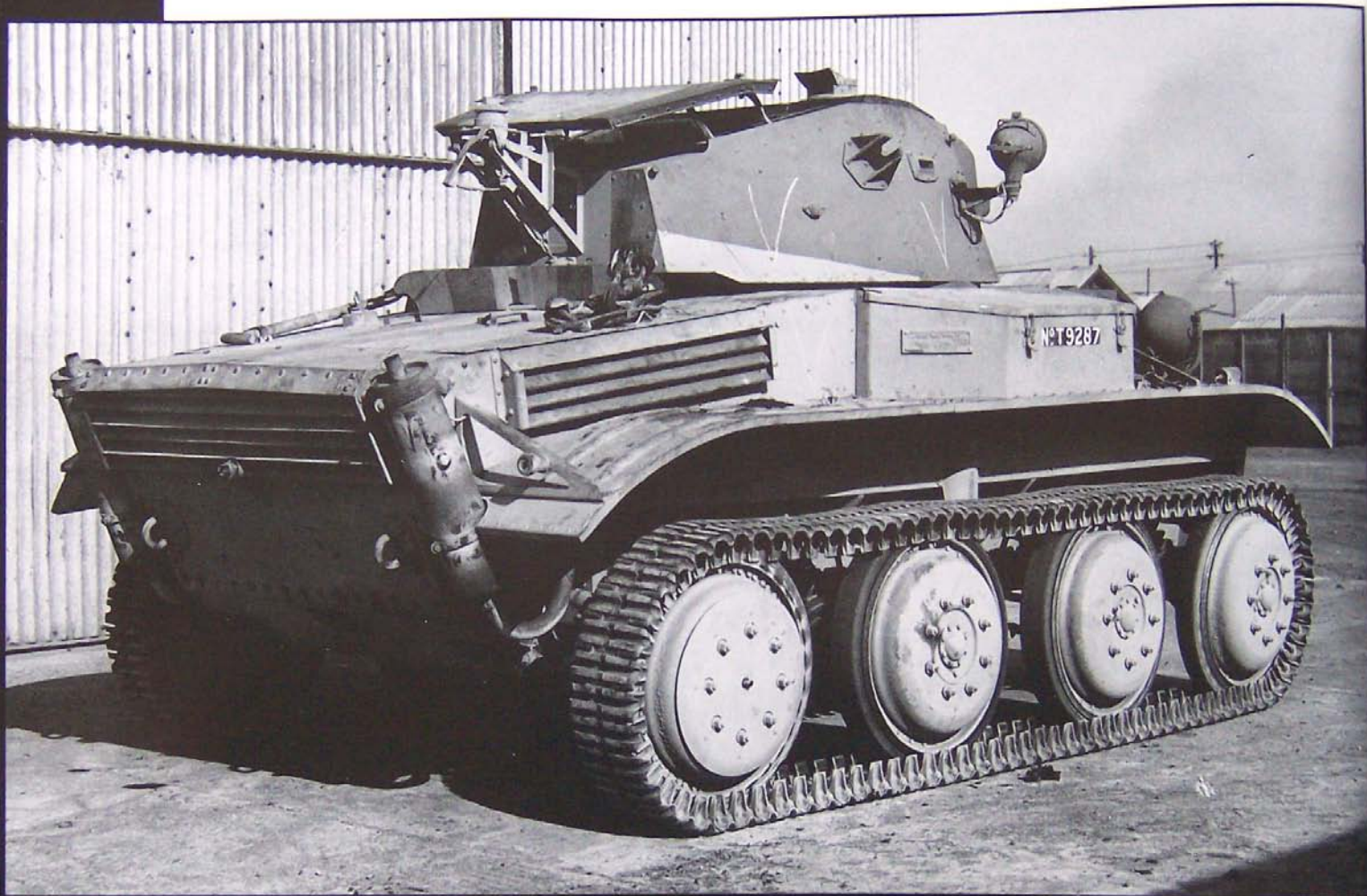
The same vehicle as the preceding photo. In this rear view the turret hatch is open and note that it raises up and then slides to the rear to rest on the back of the girder arrangement. Notice also the smoke launcher mount. The chalked "Vs" on the turret are a curious addition. Note the manufacturer's plaque on the right side stowage box. (IWM)
