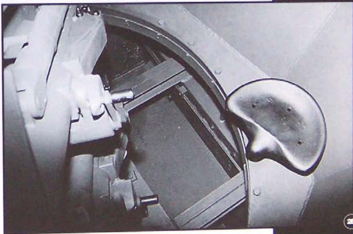
25) This interesting photo shows the coupling of gun/gunner's seat and turret. The arm carrying the seat fits into a simple arrangement. 26) This is the position of the left loader. Below the seat the intercom extension (Kst Pz. Nr. 21) was attached. Photo P Kwok. 27) The ready-to-fire ammo was stored in trays, eight magazines were stored here. 28) Another view of the left loader's seat.
