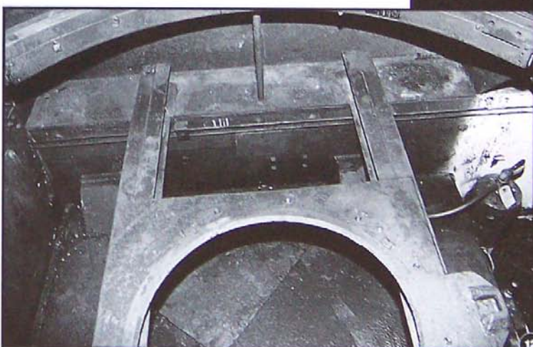
9) This tiny arrangement connects the gun with the turret, thus enabling side traverse. This detail will be shown on another photo. 10) A fine view onto the turret ring. The simple gun carriage is visible, too. 11) This close-up shows details of the turret ring. 12) The carriage arrangement was welded onto the hull sides.
