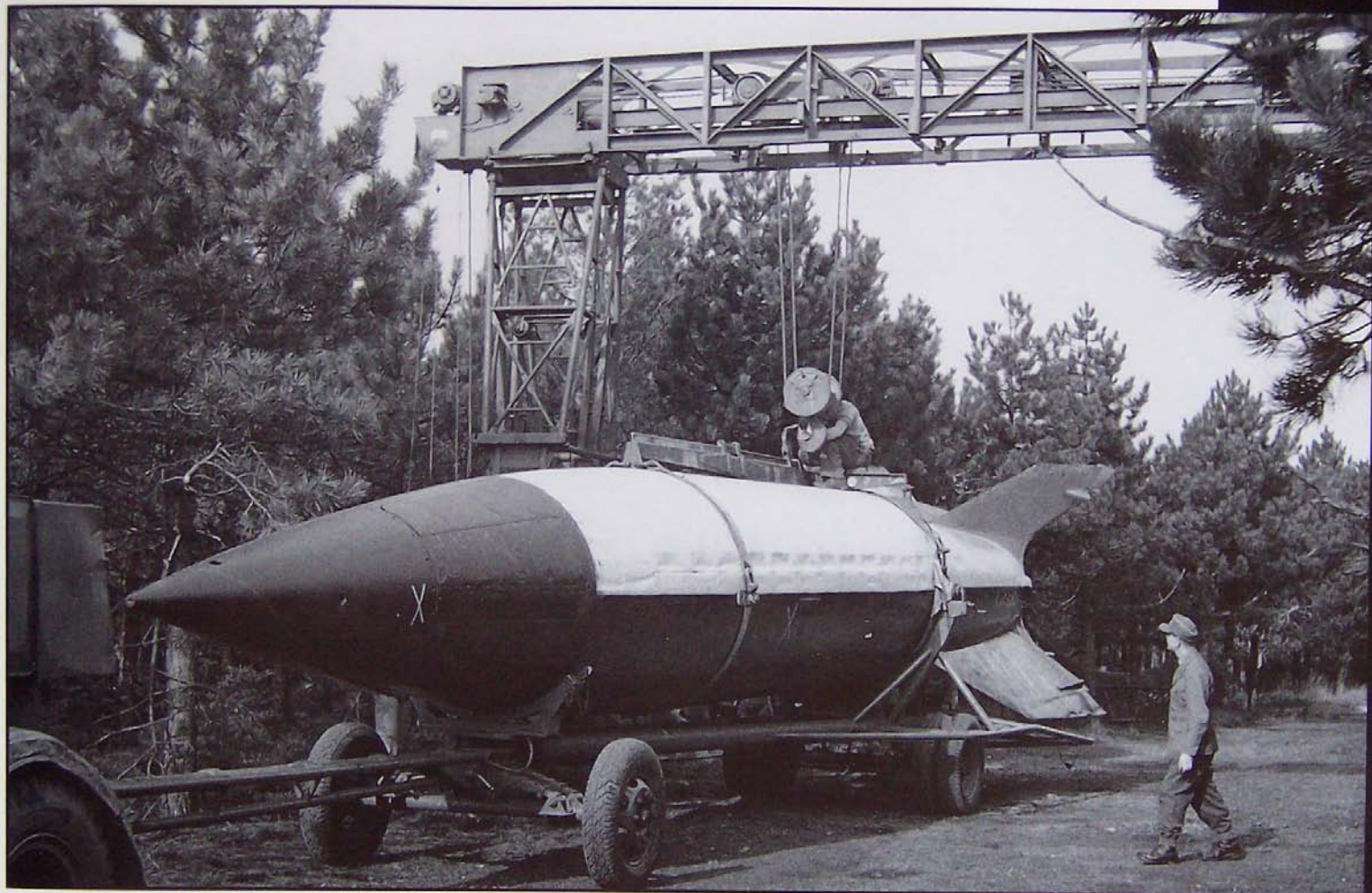
With the warhead attached, the V2 missile weighed about 6435 lbs (3015 kg), well within the working limits of this crane. When the warhead had been installed, the missile was ready to be transferred to the Meillerwagen launch trailer. The straps that had secured the missile to the Vidalwagen were fastened to a lift beam. This, in turn, was hooked to the gantry lift mechanism. When the crane was fully extended, as seen here, there was sufficient clearance to lift the V2 clear of the supports on the Vidalwagen and move it to the Meillerwagen. The size of the men here in relation to the rocket shows how large the V2 was. It was the largest tactical missile fired in combat, though some modern ICBMs are larger. (IWM)
