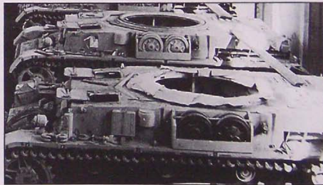
Above and below: The large assembly hall of Ostbau in Sagan. More than 10 Wirbelwind in various stages of production wait for completion. It is evident that different versions of the Pzkw IV were used. In the foreground of the lower photo, two late Ausf. H can be seen; the hulls farther in the back are possibly Ausf. G or early H. Note that early style drive sprockets were used. The empty brackets for the side skirts are visible, too. The hull with the number 4015 is already fitted with a turret. The typical Ostbau camouflage was also applied. The 2 cm Flakvierling 38 (Panzerabwehrung) waits for installation. Photos v. Seherr-Thoss.
