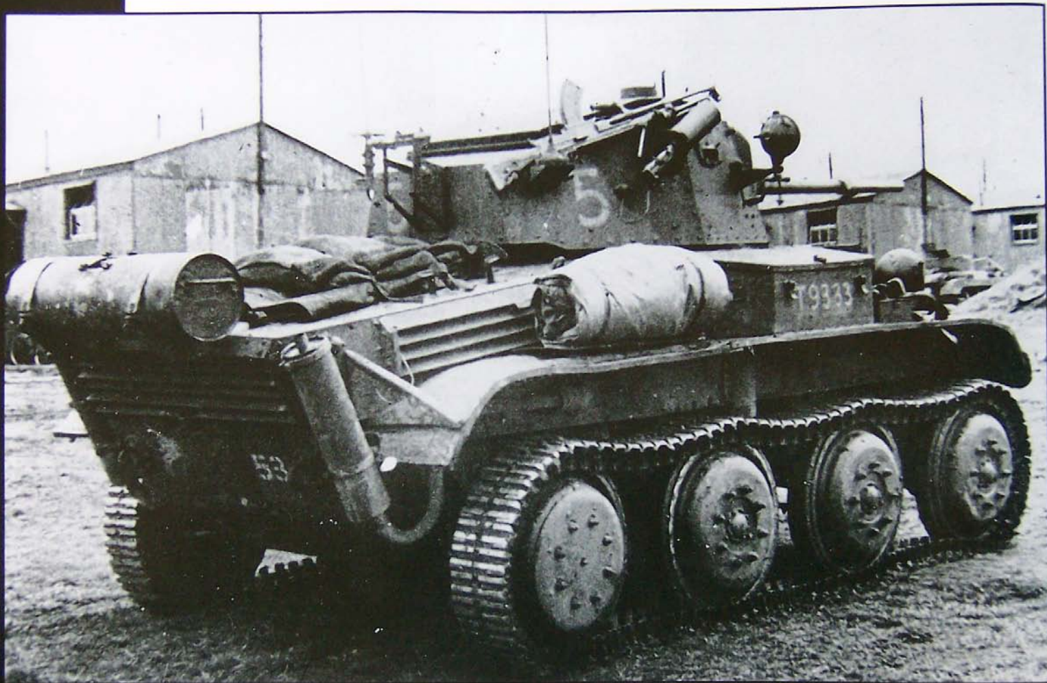
This photo and the preceding one could very well represent a portrait of a vehicle about to be loaded into its Hamilcar glider. The crew has already tied down its tarps, and the rear fuel tank and smoke launchers are fully rigged. The only airborne use of the Tetrach was in Normandy, when a squadron was deployed via Hamilcar. One of these tanks fell out of its glider on the way. Since the crew had to ride in the tank while in the air (there was no way to get in or out), they and their tank are still on the bottom of the Channel. (IWM)
