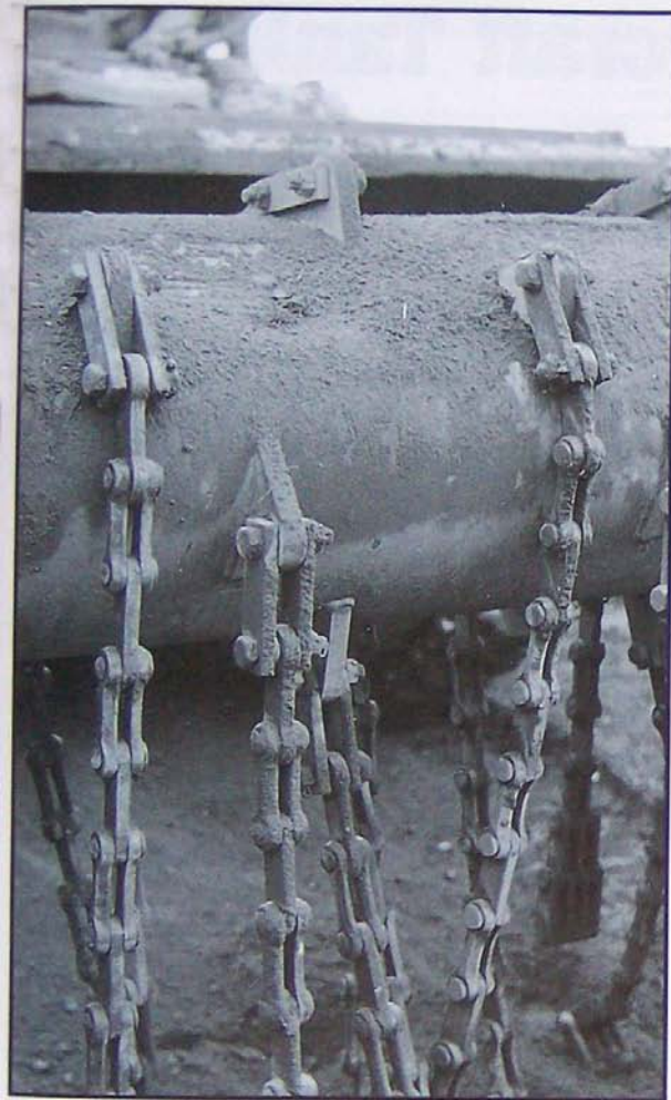
Left: An excellent close-up of the flail chains. The chains are secured with 2 flat pieces of steel. These, in turn, are secured to the rotor with bolts and locking nuts. This made it quite easy to replace broken or damaged chains. The chain links are composed of rounded end flat steel stock, alternating one, then two links. The links are permanently secured with steel rivets. Hanging just behind the rotor, one of the widened end links can be seen. These were composed of four links across to widen the contact area of the chain. Right: Two marks of the Crab were developed. The first, seen in all the previous photos, had
