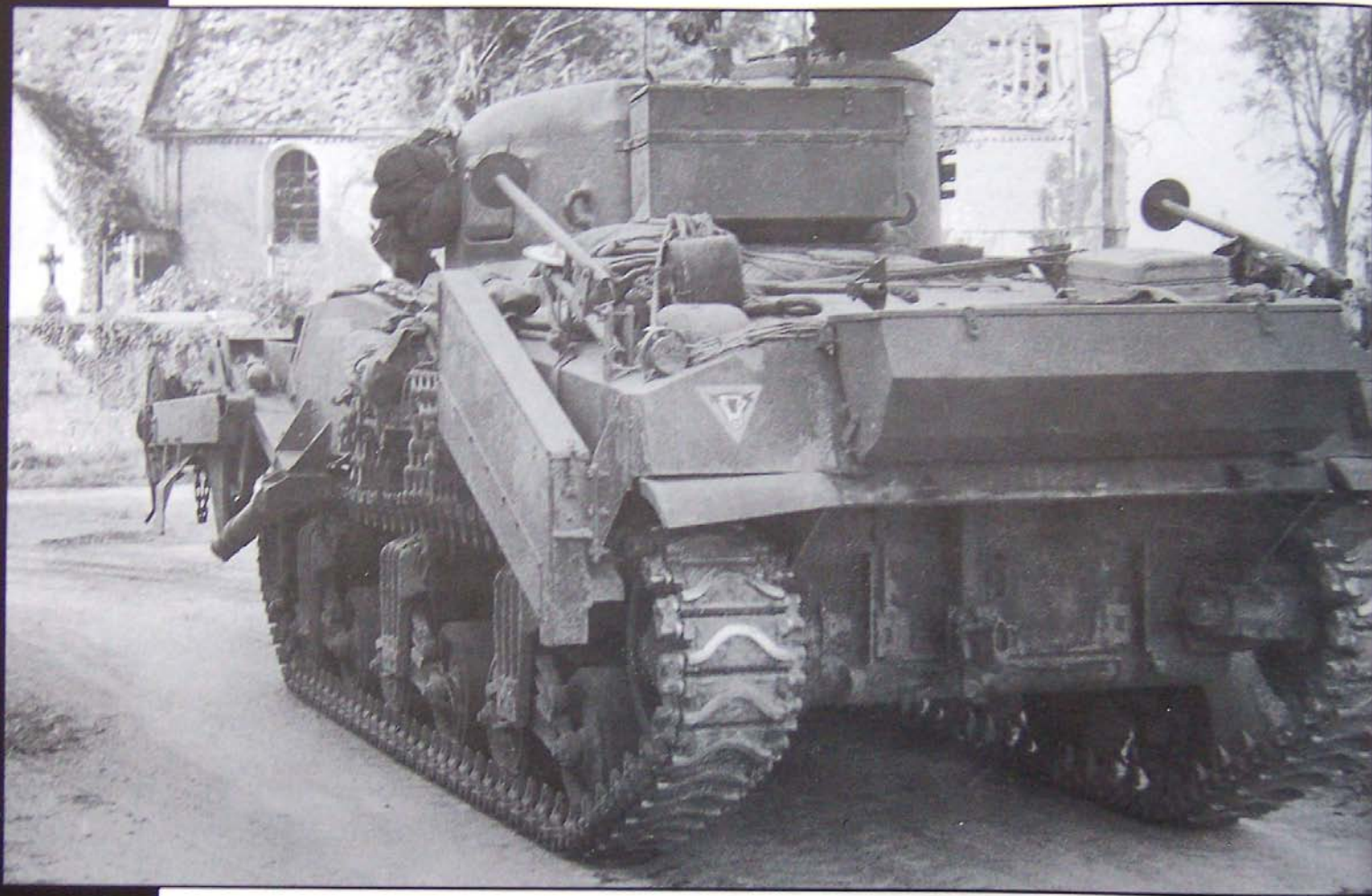
A Crab of the 79th Armoured Division, as shown by the distinctive division sign on the rear hull, is approaching the ruined church of Escoville, France. Dated July 19, 1944, this photo was taken not far from the famous "Pegasus Bridge," sight of the well-known British glider landings just prior to D-Day. This Crab has the typical British stowage bin on the hull and turret rear. Spare chains are more neatly
