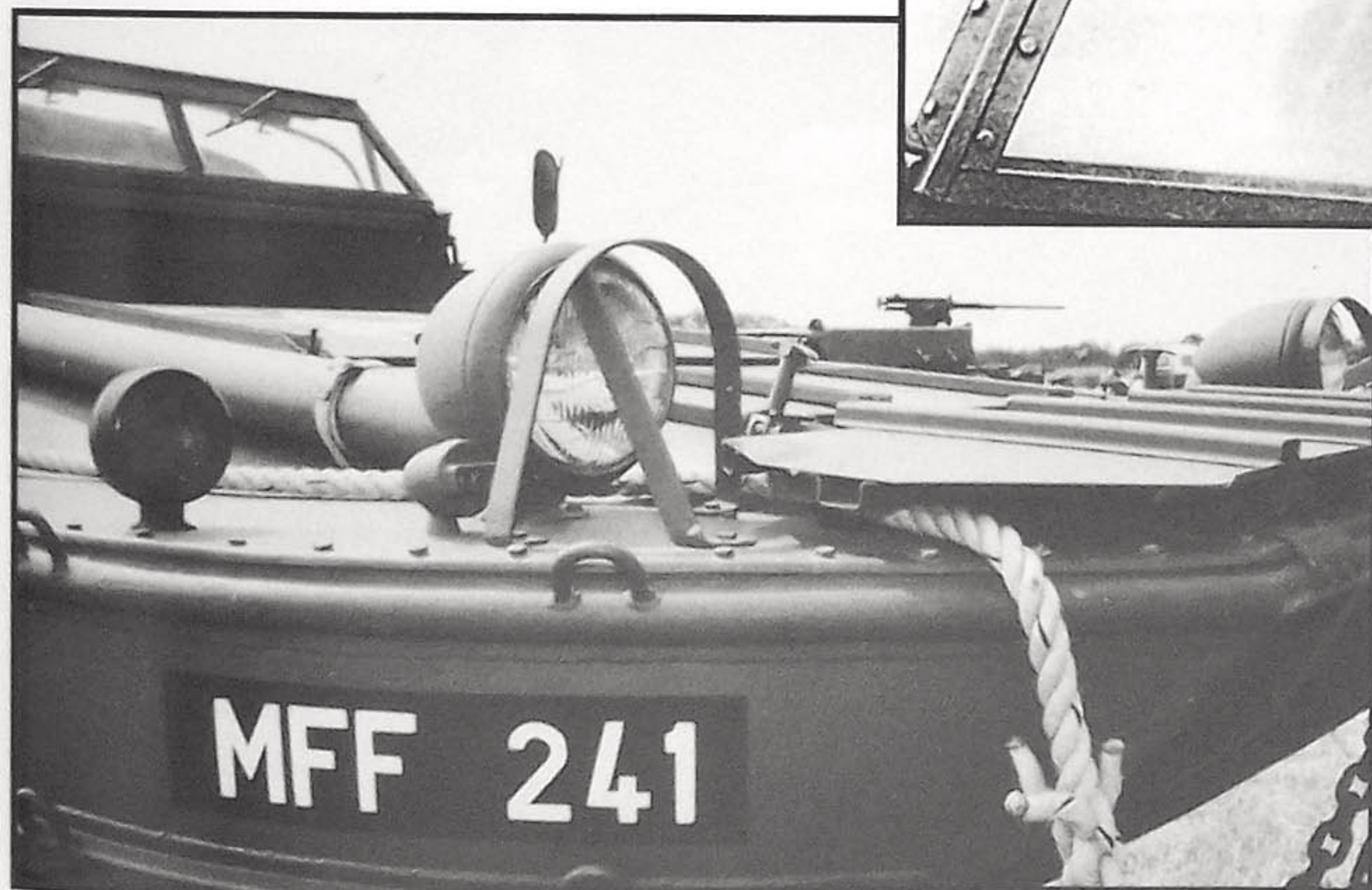
Top left and right: these two large side vents exhausted hot air from the engine compartment. Inset: this tech manual photo shows how the canvas top was attached to the side windshield panel. Above left and right: the front end lights and their frames. Several of the tie-down points can be seen in these photos. These were used to secure the various rope bumpers used in mooring the Duck. The large tube seen in the shot at right is a hand-pump for removing water from the cargo bed. The numberplate seen here is a civilian item.
