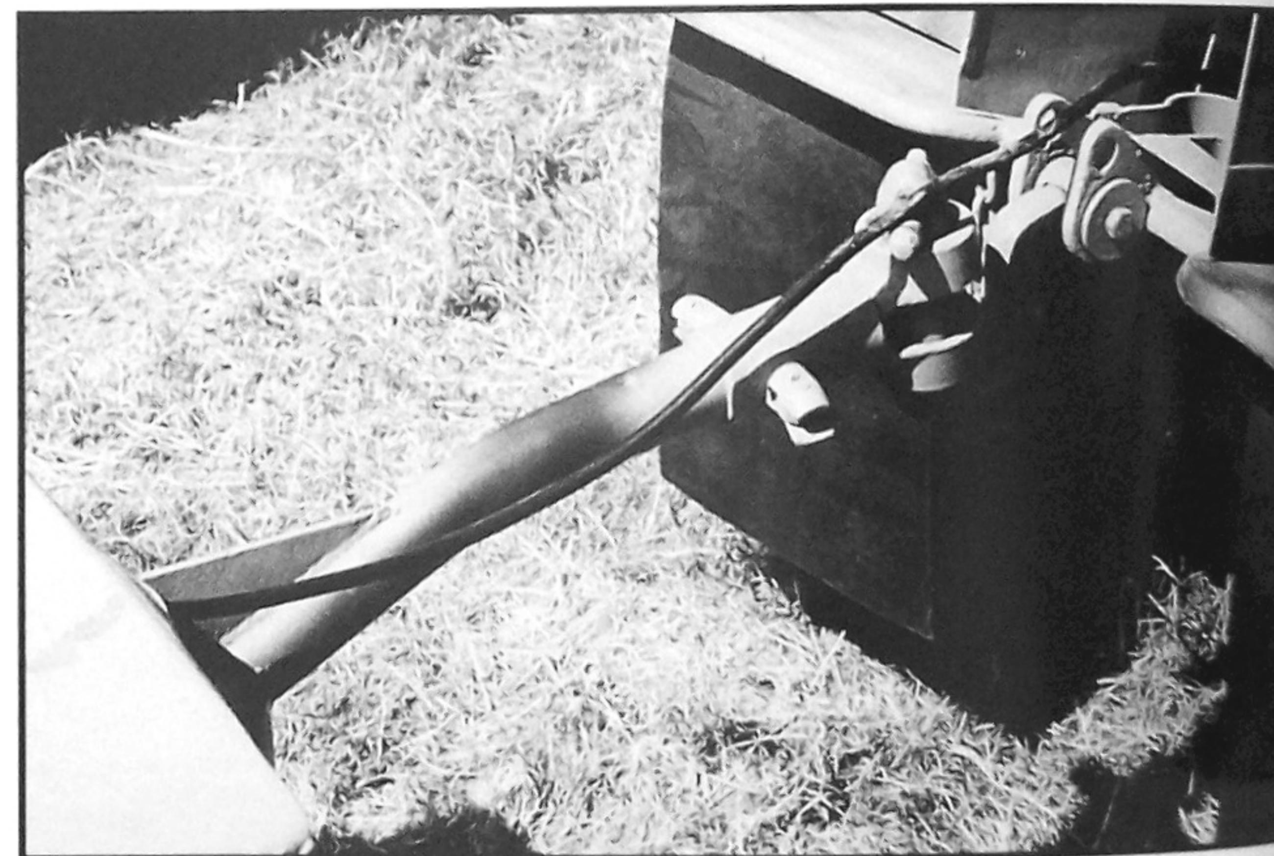
Above left: the rear rifle rack on the Beltring vehicle. This shot provides another view of the center housing. This vehicle has the correct rear marker light installed. Top right: the rear tow hook of the Münster vehicle is the heavier type developed for towing the 10.5cm LG 40 recoilless gun used by Fallschirmjäger units. Above right: this is the more common type of tow hook installed on Kettenkrads. The pintle itself is very similar to those seen on other German light vehicles, such as the Demag D7. The hinged base, however, was uniquely designed for the Kettenkard. This allowed it to cross obstacles of significant depth without "jack-knifing" the trailer. Here, the boom of the Sd.Ah 1 trailer is installed.
