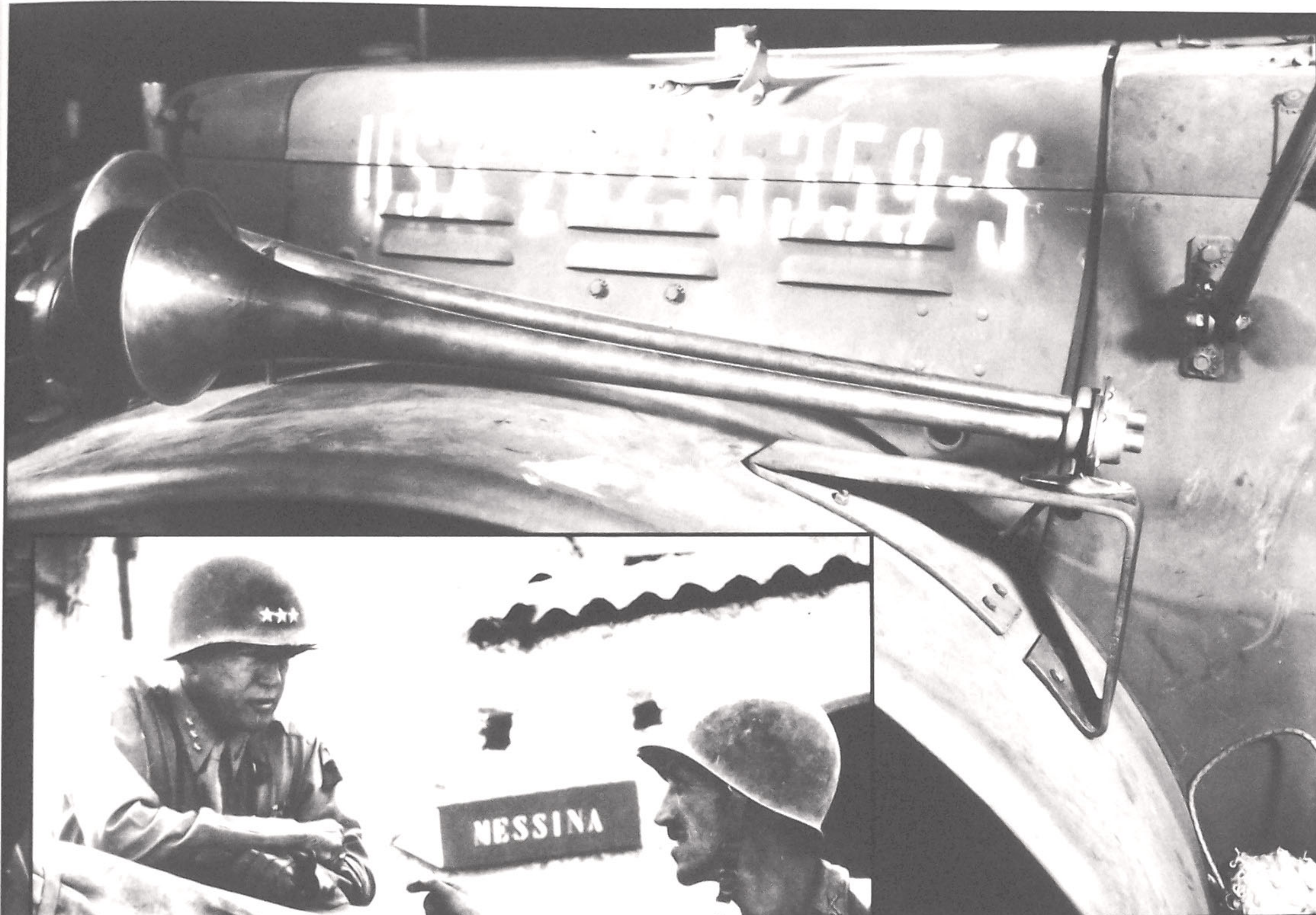
Above: regardless of the vehicle modified, Patton always insisted on installing large, loud air horns. The source of these particular parts is not known, but they are most likely custom made for this application. Commercial grade truck air horns were generally installed inside the engine compartment and these examples are nearly as long as the Dodge's front end! A special bracket has been fabricated to support them and the electrical leads are still to be installed (NA). Left: Patton also used a Dodge command car in Italy. This was a standard WC 56 car with very few modifications. Patton is seen here speaking with a GI just before his entrance to the port town Messina, Sicily on August 17, 1943 (NA).
