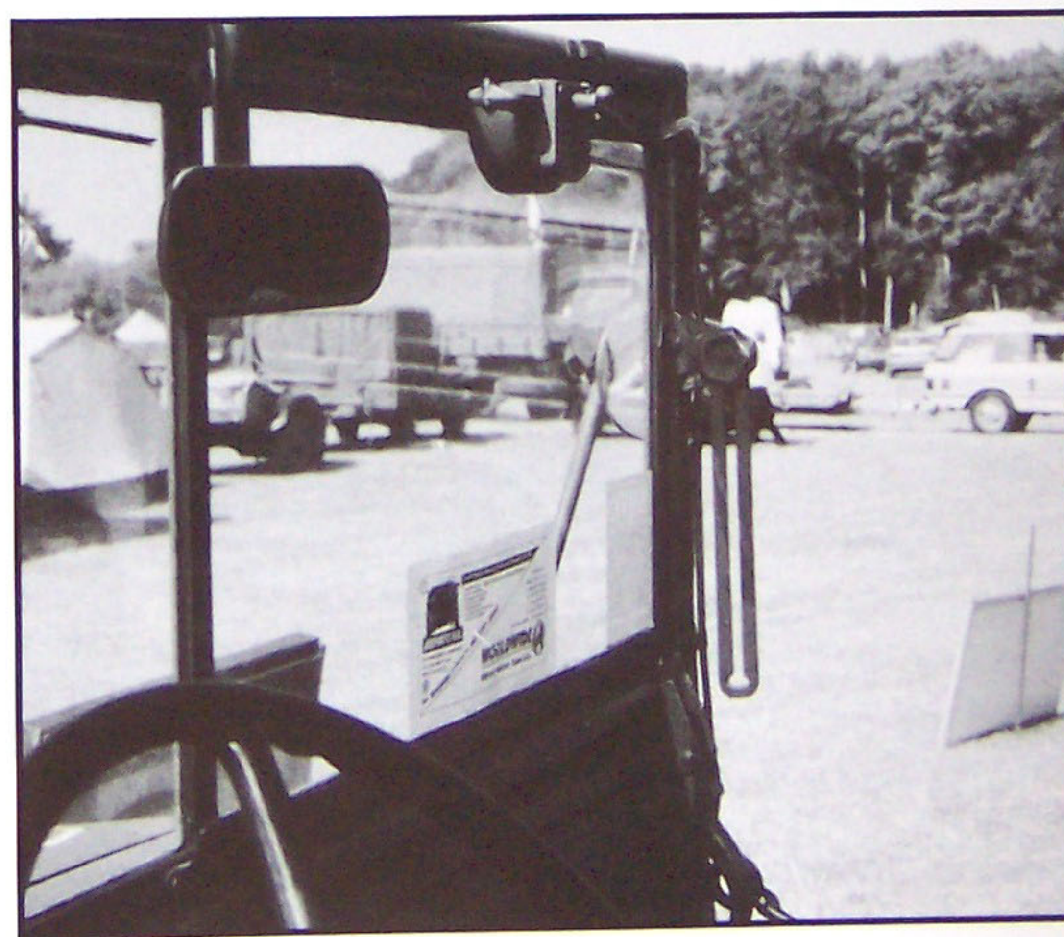
These three views of the windshield show the mechanism used to adjust the windshield glass. The star shaped knob was loosened and, as the windshield glass moved out, the knob axle moved along the sliding track. The two shots at right also show the windshield wiper motors and their wiring.
