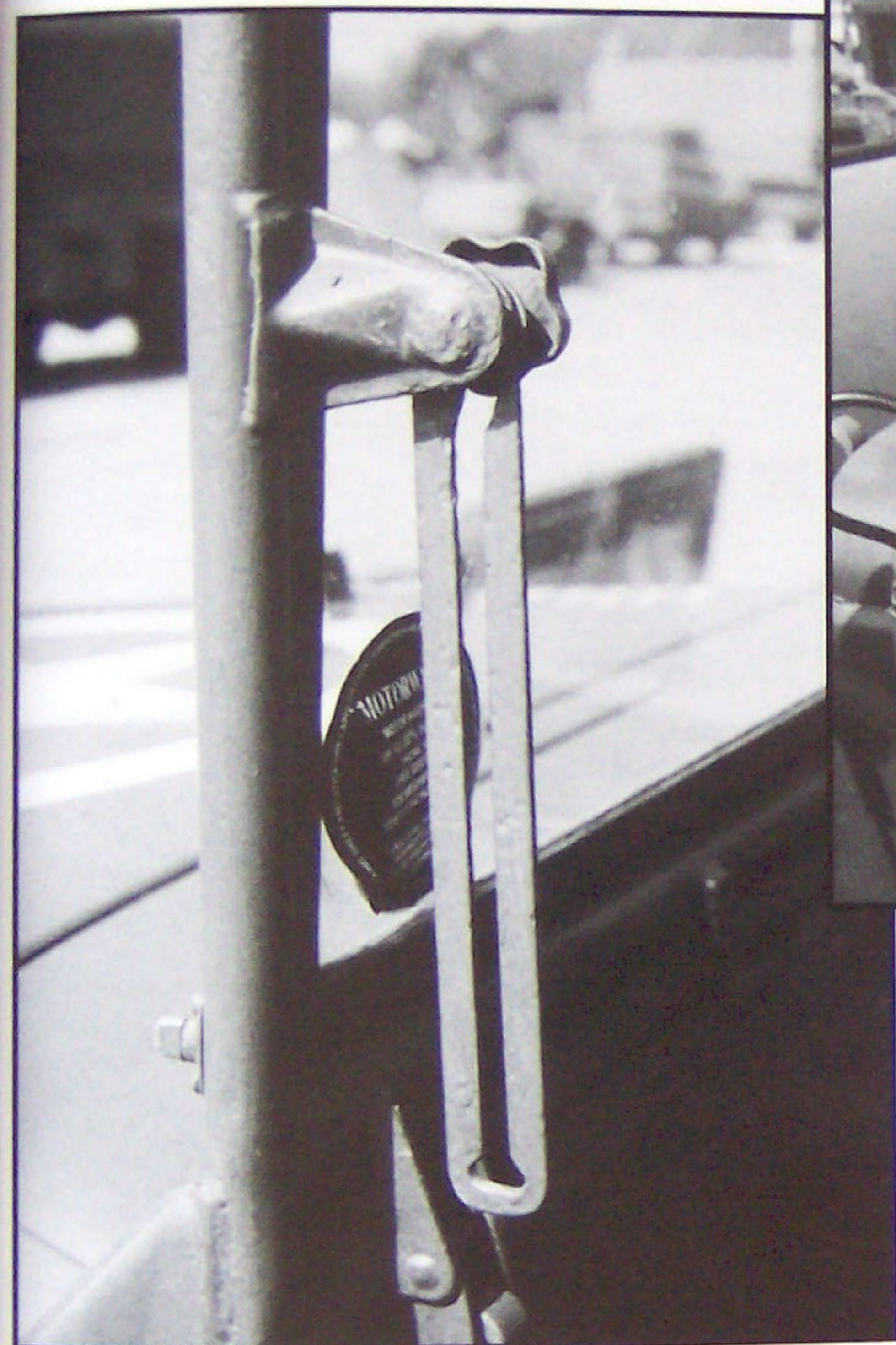
These three views of the windshield show the mechanism used to adjust the windshield glass. The star shaped knob was loosened and, as the windshield glass moved out, the knob axle moved along the sliding track. The two shots at right also show the windshield wiper motors and their wiring.
