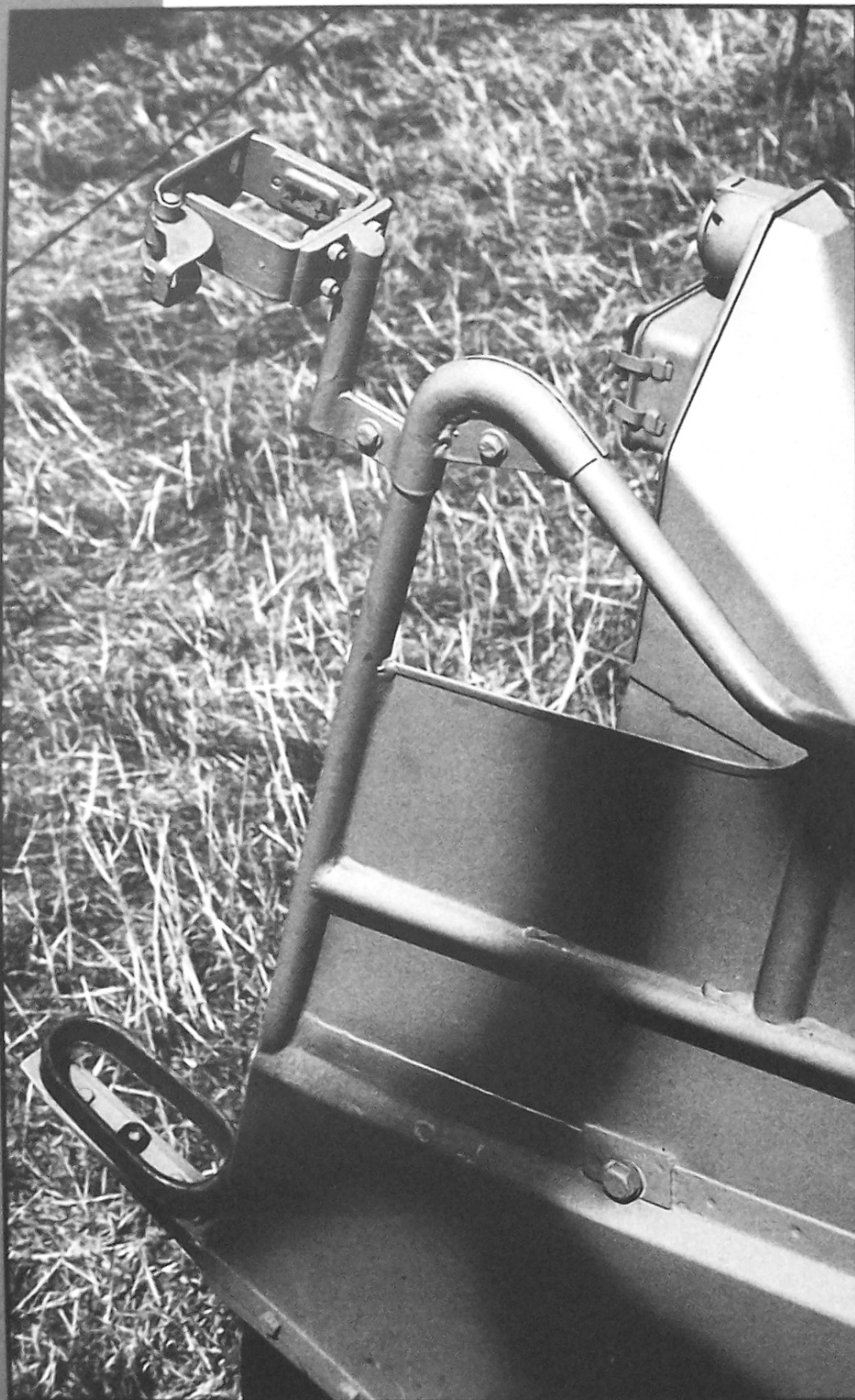
Above left: the rear rifle rack on the Beltring vehicle. This shot provides another view of the center housing. This vehicle has the correct rear marker light installed. Top right: the rear tow hook of the Münster vehicle is the heavier type developed for towing the 10.5cm LG 40 recoilless gun used by Fallschirmjäger units. Above right: this is the more common type of tow hook installed on Kettenkrads. The pintle itself is very similar to those seen on other German light vehicles, such as the Demag D7. The hinged base, however, was uniquely designed for the Kettenkard. This allowed it to cross obstacles of significant depth without "jack-knifing" the trailer. Here, the boom of the Sd.Ah 1 trailer is installed.
