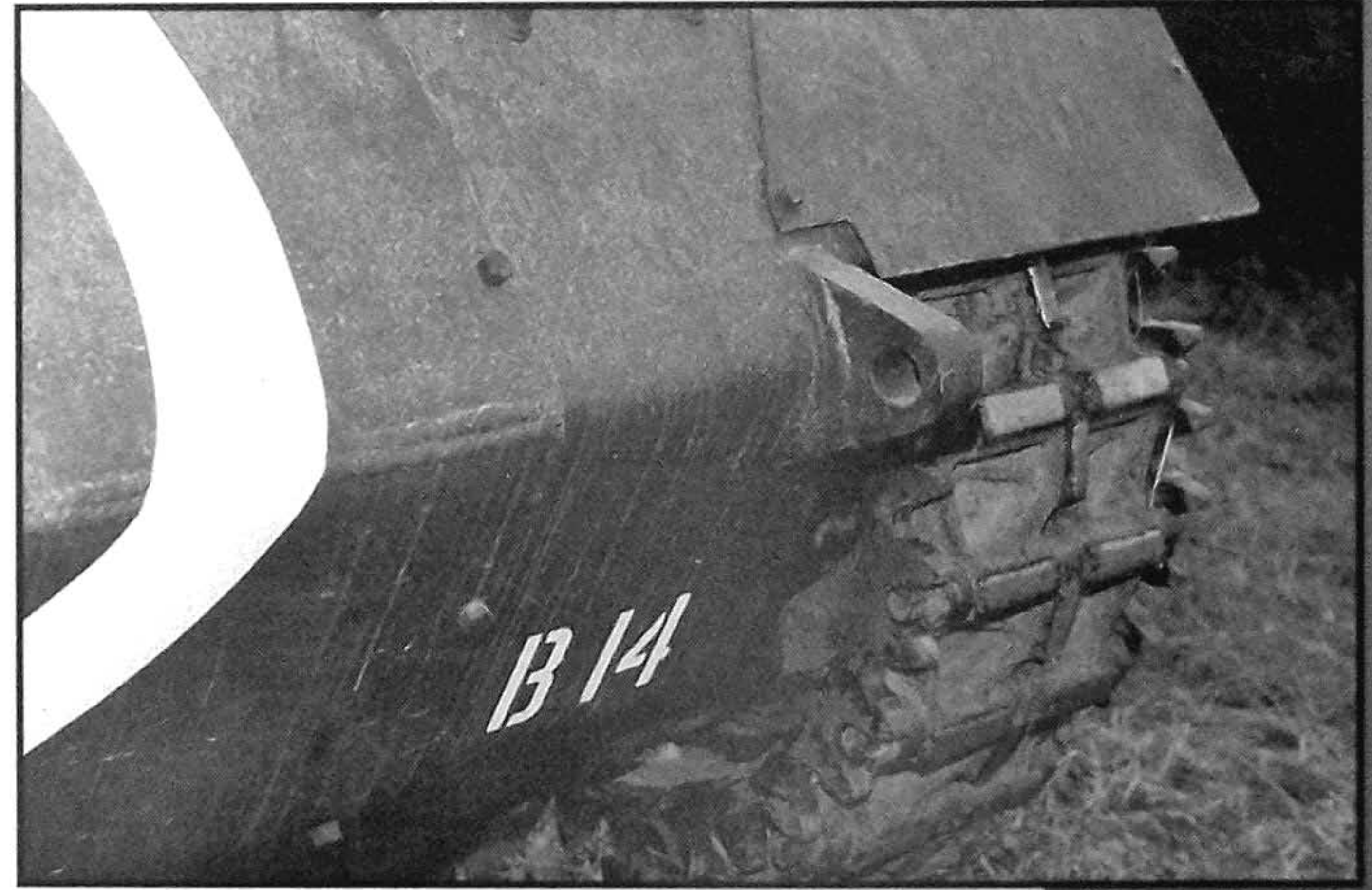
system. There are small blackout lamps fitted above the main driving lamps. Above right: Towing eyes were welded to the front of the glacis. Note the gearbox access plate is made from two sections welded together.
