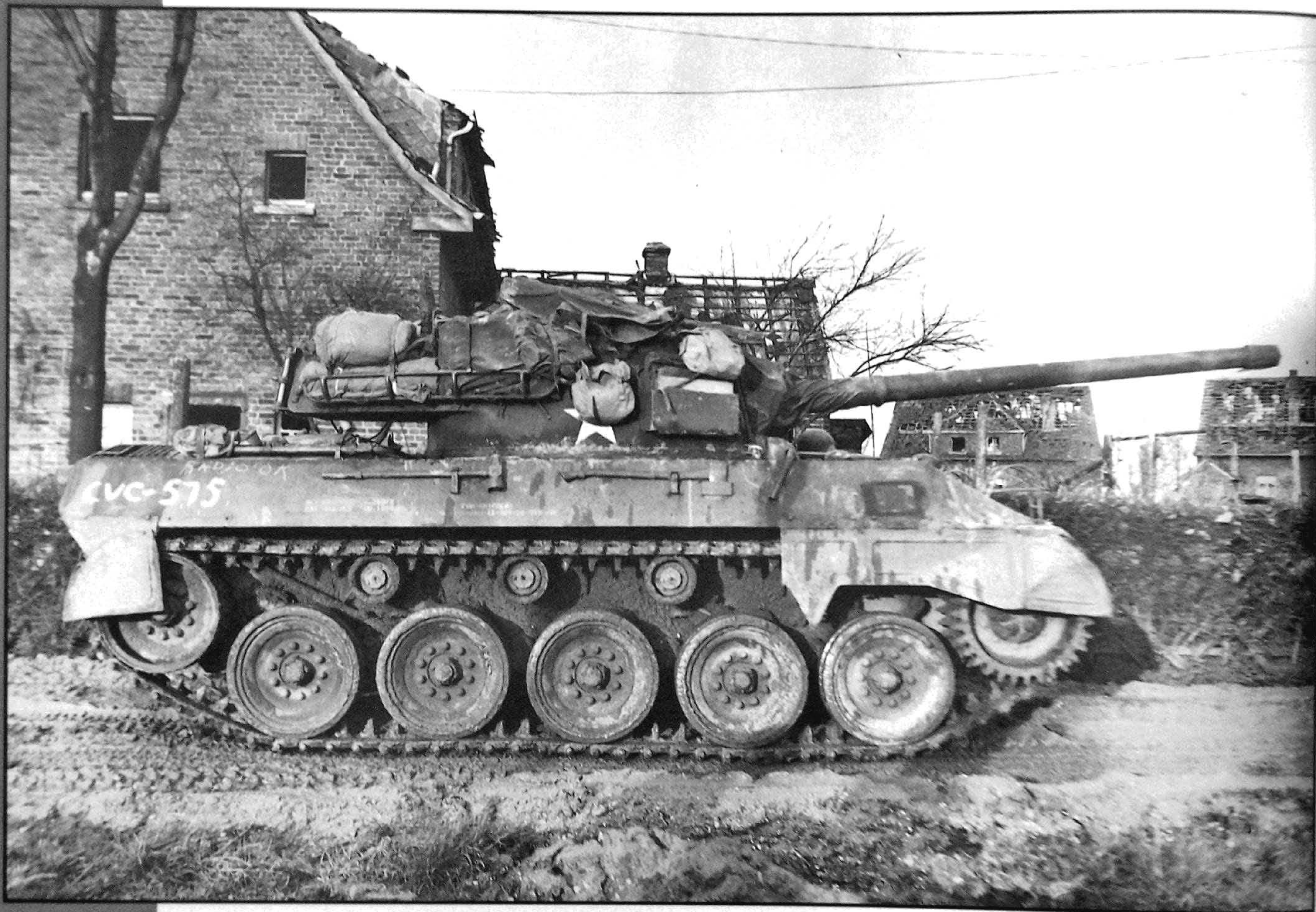
Above: An M18 is stopped in the town of Immendorf, Germany on December 11, 1944 during the initial penetrations into Germany. This side view provides a good impression of the side fender panels so often damaged or discarded by the crew. The shipping stencils can clearly be seen along the right side of the hull, as well as "radio OK" written in chalk. (NA).
