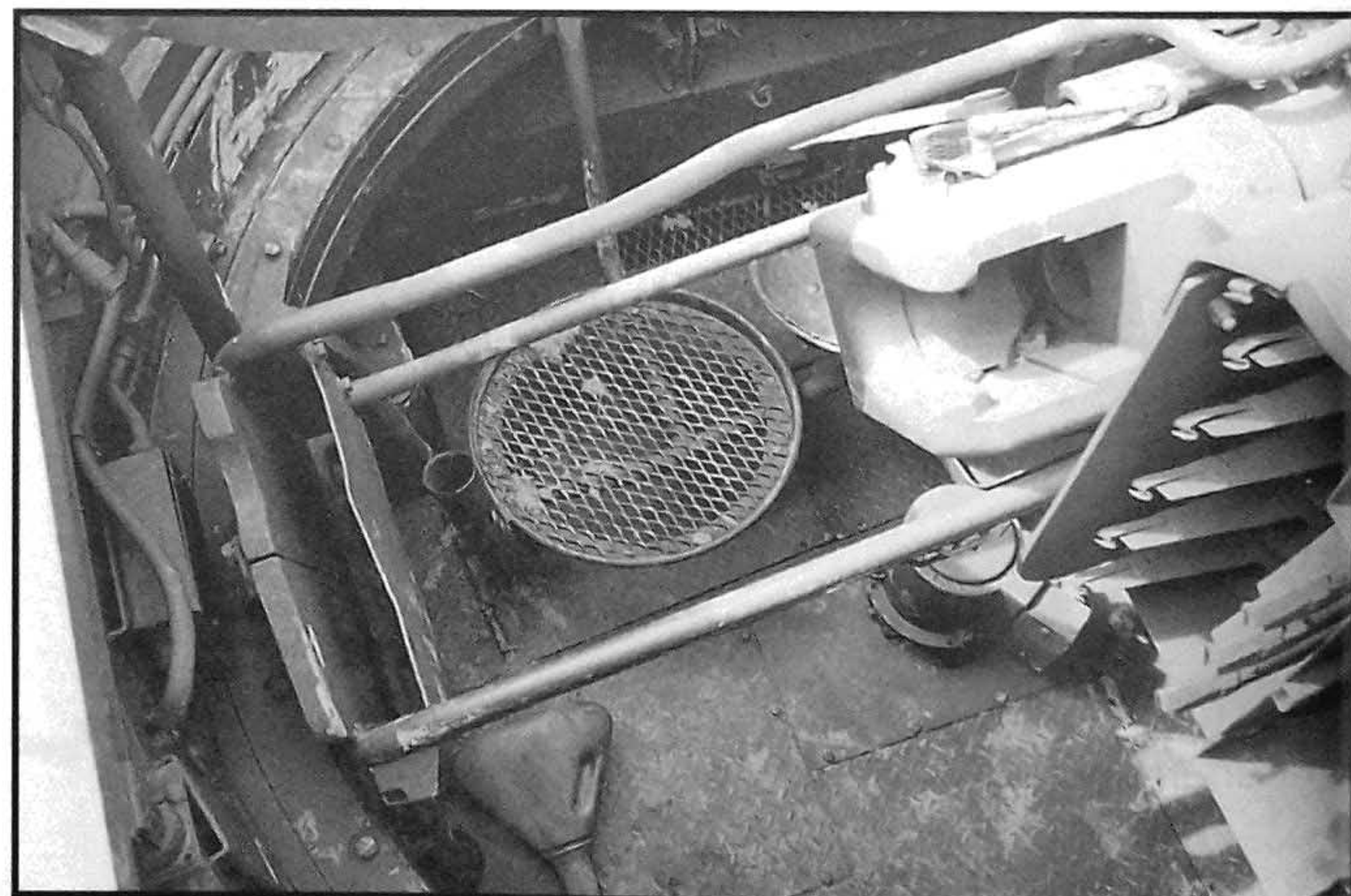
turret ready rack and 18 in each hull sponson. Above right: The M1A1 gun was fitted with a guard to prevent crew injury when the weapon recoiled. Note the commander's seat was formed from expanded metal mesh. This was because he needed to stand on it to operate the .50 cal machine gun.
