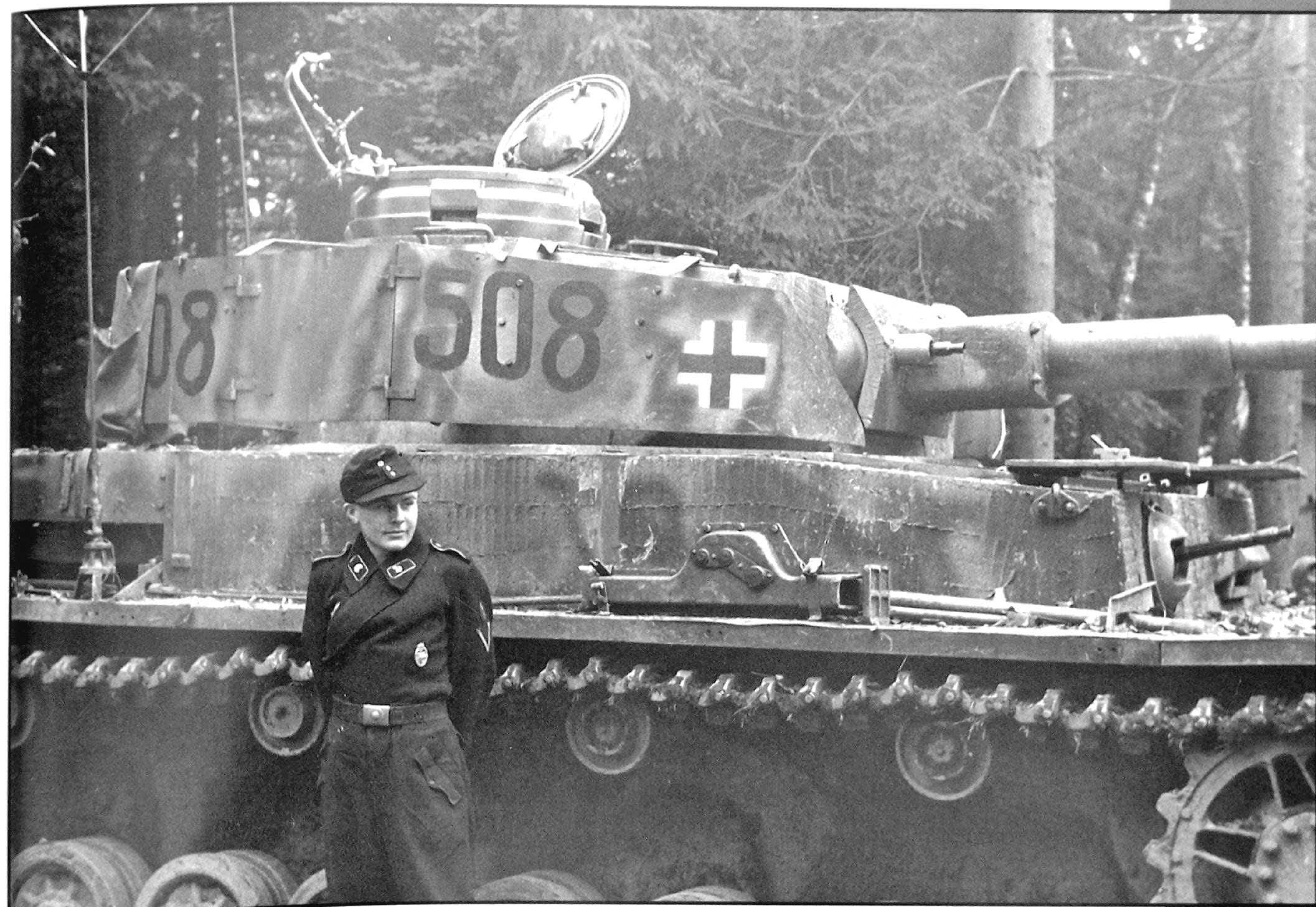
Combat photos of the the Panzerbefehlswagen IV are decidedly rare. This Panzer IV Ausf. J of the 111/ Panzer Brigade, 2111 Panzer Abteilung was photographed in September of 1944 in the Lorraine region of France. It is interesting in that it is being used in the role of a command tank, but was not manufactured as a Panzerbefehlswagen. Note the location of the standard radio antenna on the left rear fender,
