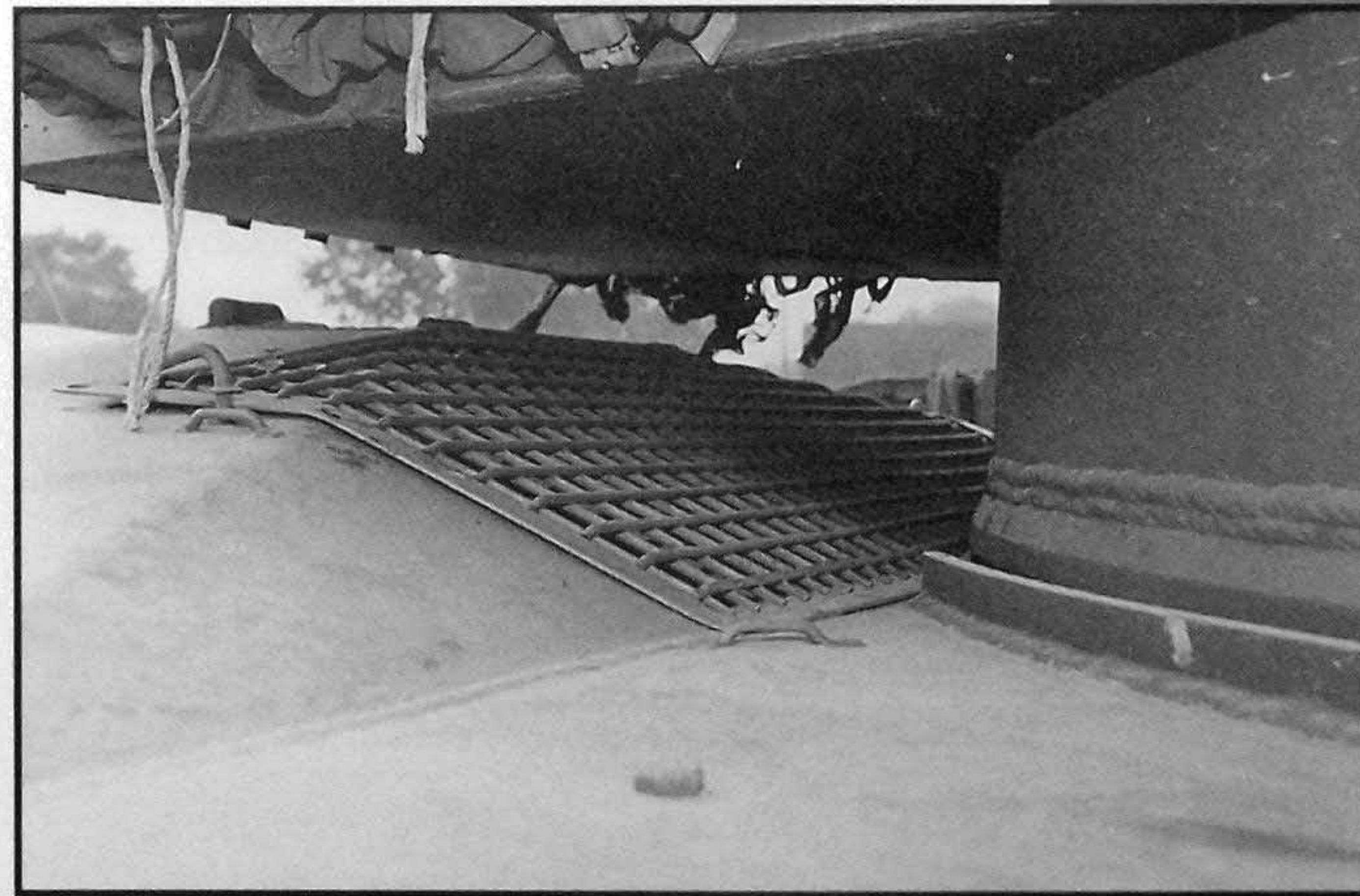
Tools were located in steel clips, secured by leather straps. Above right: A stout metal grille protected the engine air intake. Overhead protection was offered by the turret bustle.
