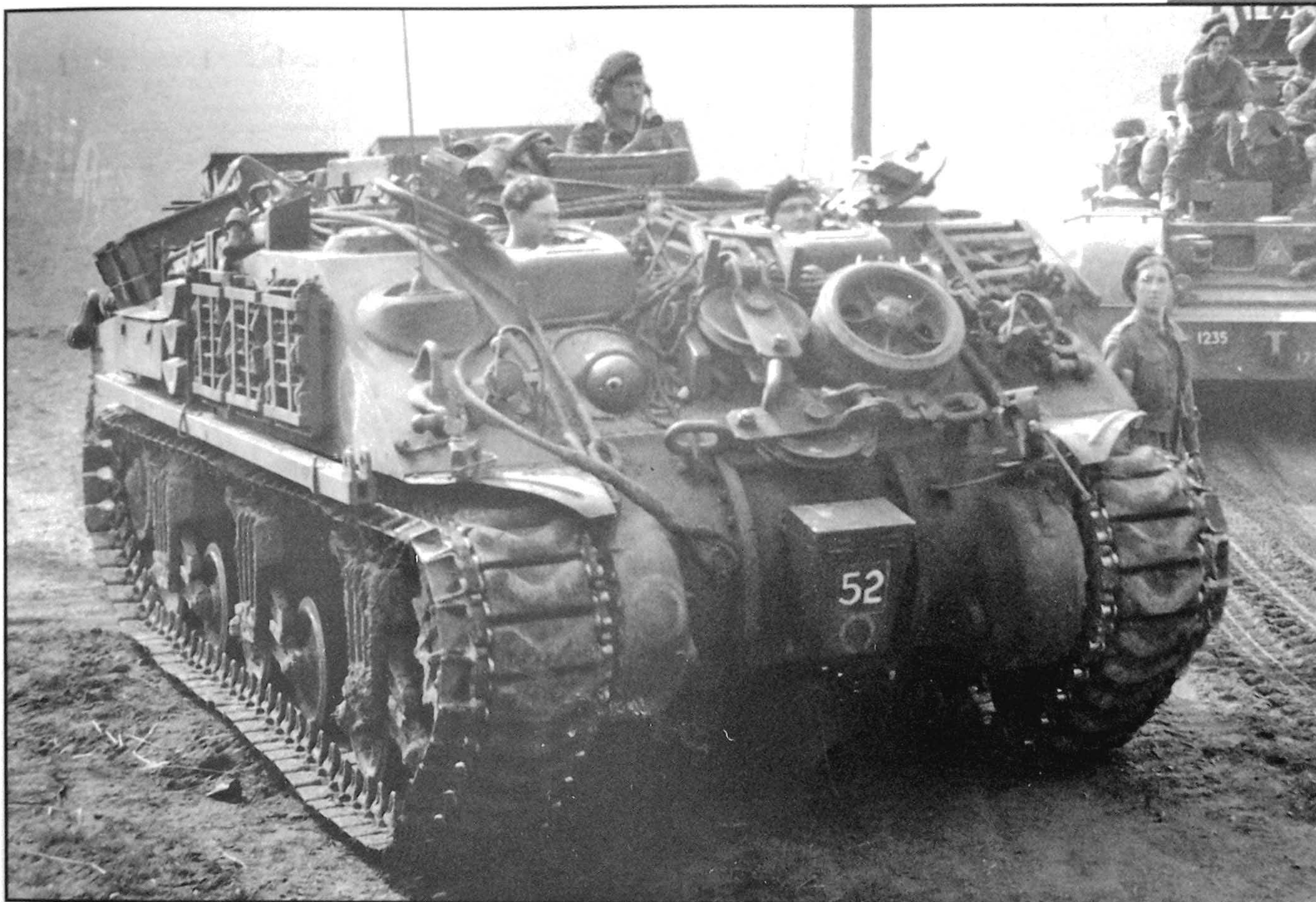
Sherman ARV Mk I festooned with equipment. Note duckbills or extended end connectors on tracks, two 15-ton snatch blocks, stored grousers on front three-piece housing and side sponson, spare road wheel and front vise. The stowage box on the front housed the chain block and cable used for recover-
