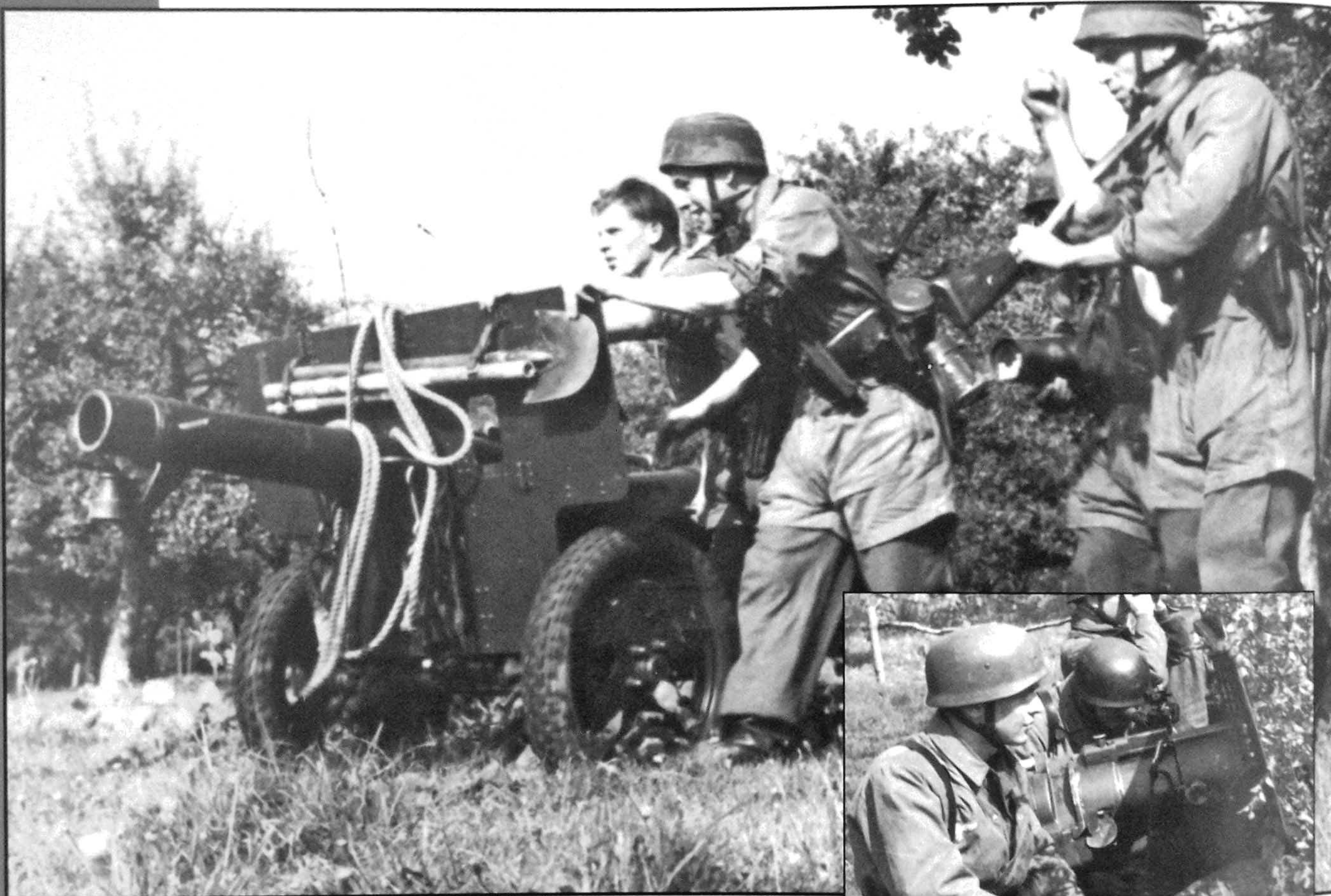
The extreme back blast of the weapon was always a problem in service. This not only presented a hazard to the crew, but also immediately revealed the position of the gun. This was made worse in darkness, when a bright flash accompanied the discharge. A fair amount of space was also necessary to ensure the gases did not completely engulf the crew. The problem of back blast was eventually reduced with changes in the ammunition. Above and inset: the 7.5 cm LG 40 in service with another Fallschirmjäger unit. The differences in the two guns were minor and involved the design of the small carriage. Note the different wheel pattern. (BA)
