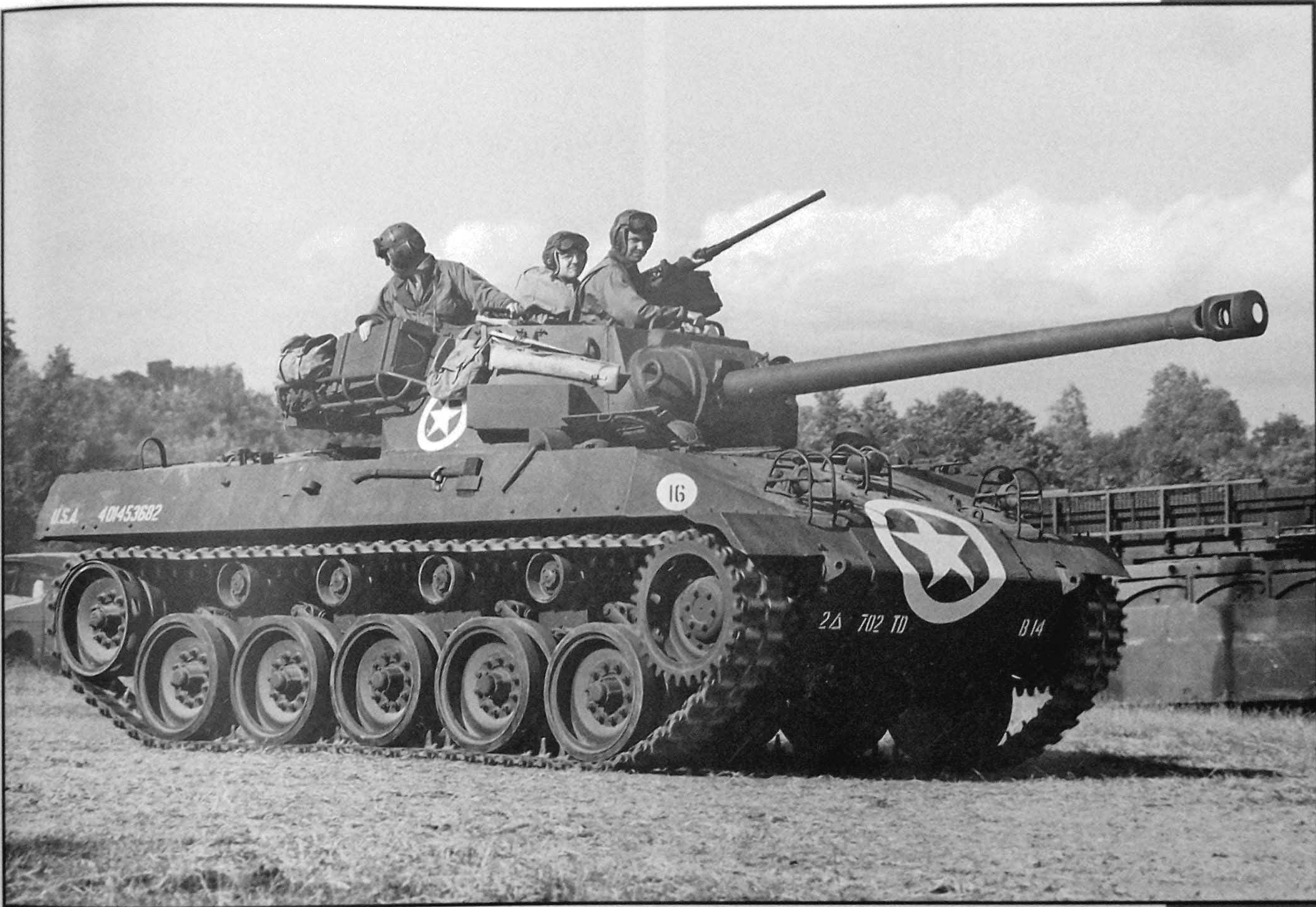
The torsion bar suspension was good and gave the M18 excellent mobility, which was a very good thing, as the armor was thin and the turret had an open top. The M18 was capable of extraordinary speed for an armored vehicle, up to 50 mph on a level paved surface.
