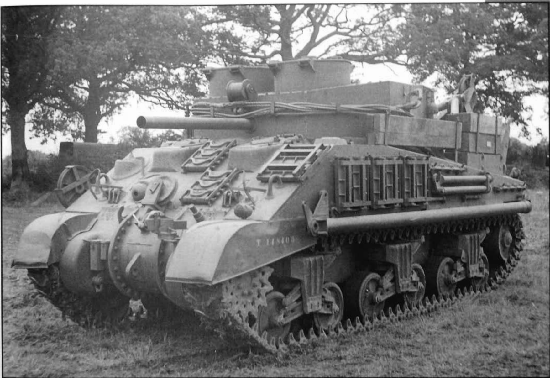
Three quarter front view showing circular hatches on superstructure, cable stowage, dummy gun, grouser and spare tracks. The hold fasts or earth anchors are stored on the side, along with the larger front jib. Gun planks and rear boom or A-frame can be seen at the back. Note the two added brackets
