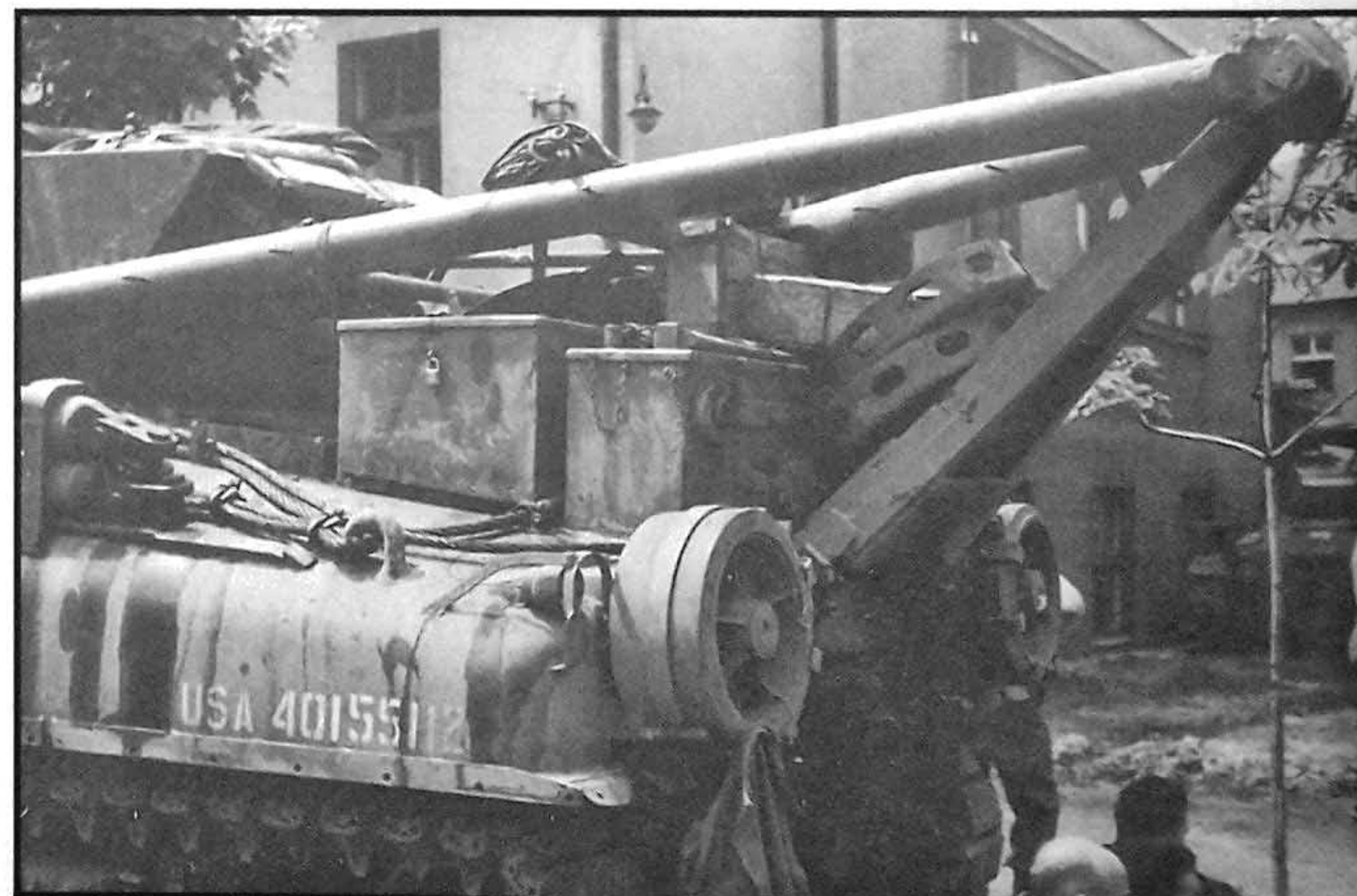
the round air filter is clearly visible. Note the curved fender flange behind the right rear idler. Above: Two further views of FRAULEIN. The large bipod-style assembly mounted on the left side of the hull is a towing brace. In these photos the boom is folded to the rear. FRAULEIN's boom is secured to the twin brackets on the rear of the hull. In this configuration, the M32 could function as a wrecker.
