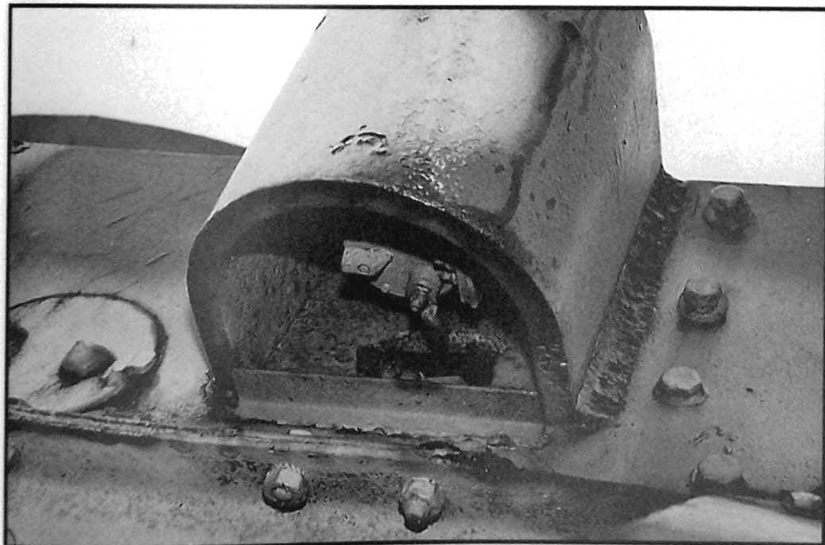
Top left: Although heavily corroded, the mechanisms of the commander's vision ports can be seen clearly. The handle at the bottom opens and closes the external armored covers. The vision ports were fitted with thick armored glass. Above each port is a rubber-padded headrest. To the right can be seen the fixed base unit for an artillery style scissors periscope. Top right: The armored cover for the external
