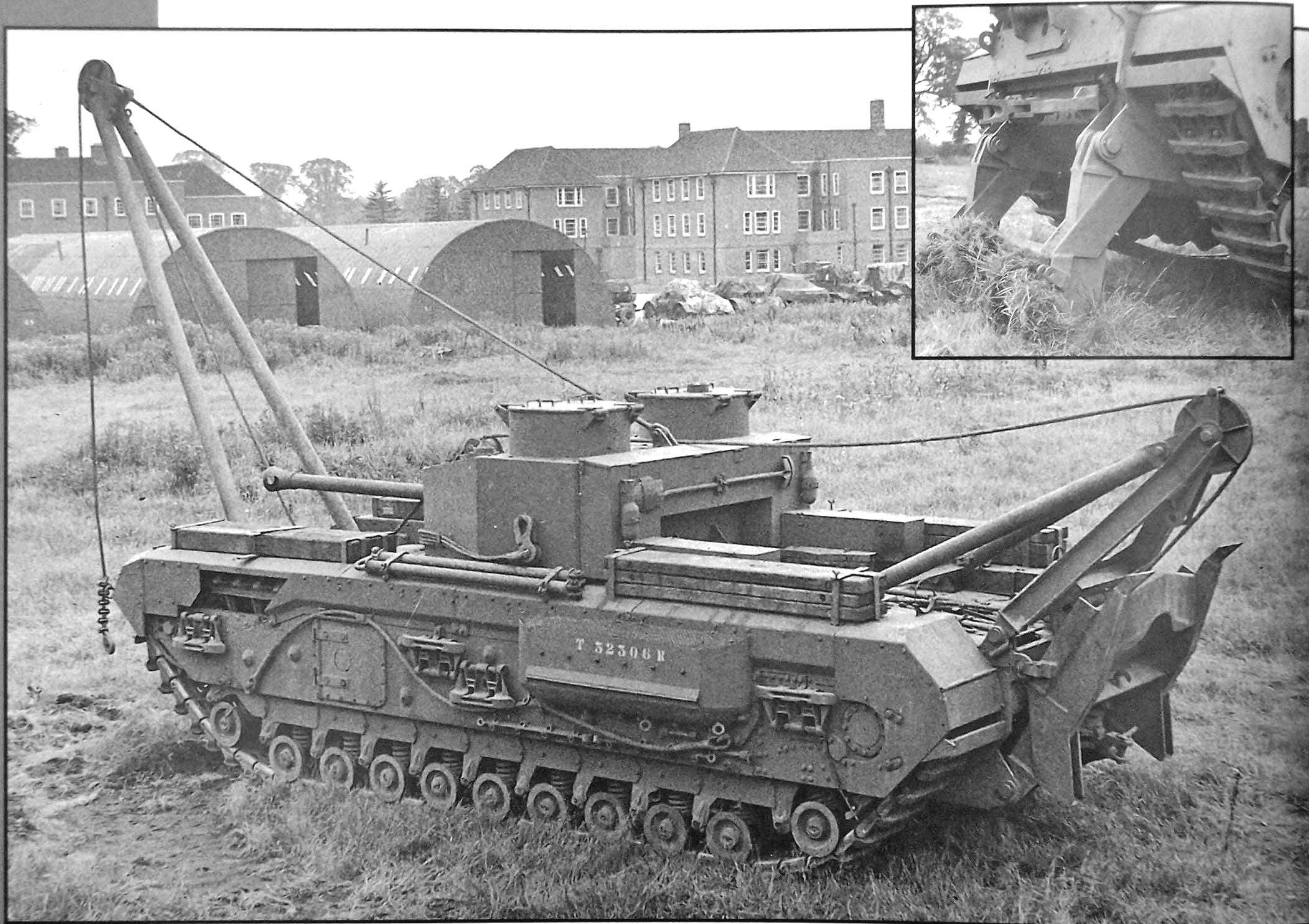
A Churchill ARV Mk II with its boom erected and ready to lift. All the recovery equipment was essentially the same as that used on the Sherman ARV MK II. This Churchill sports the early rounded air intakes and circular superstructure cupola. The fenders over the tracks and drive sprocket are very different from the other marks of Churchills. They are flat and without the support ribs. The front fender and mud
