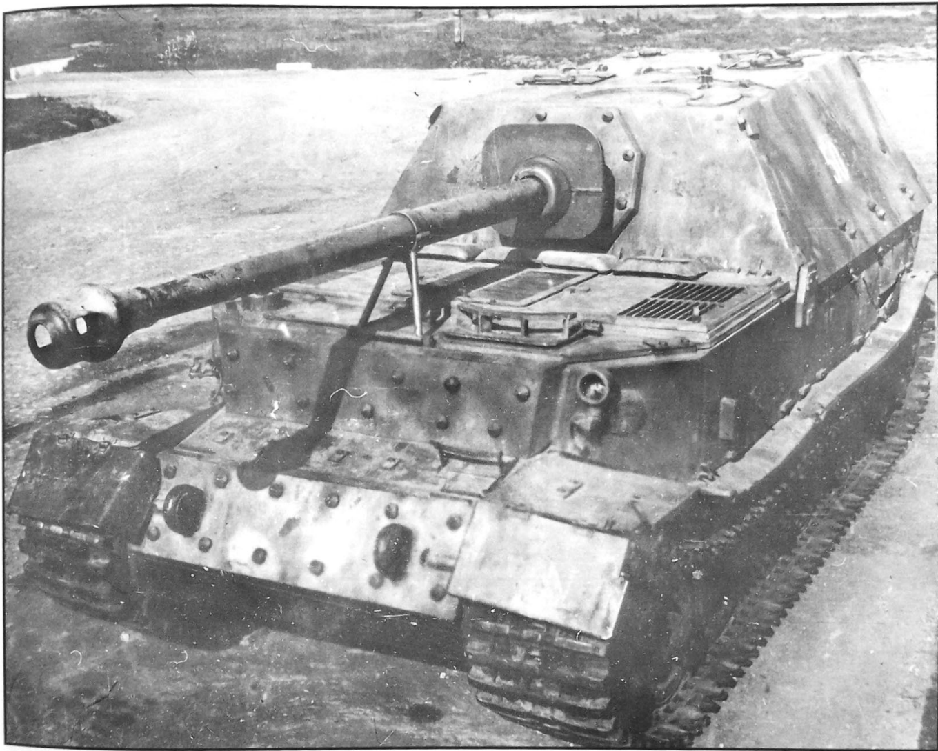
As far as possible, Ferdinand 501 was repaired after the obligatory examinations. The missing rear escape however, although still existing, was not installed. (Photo S. Netrebko)
