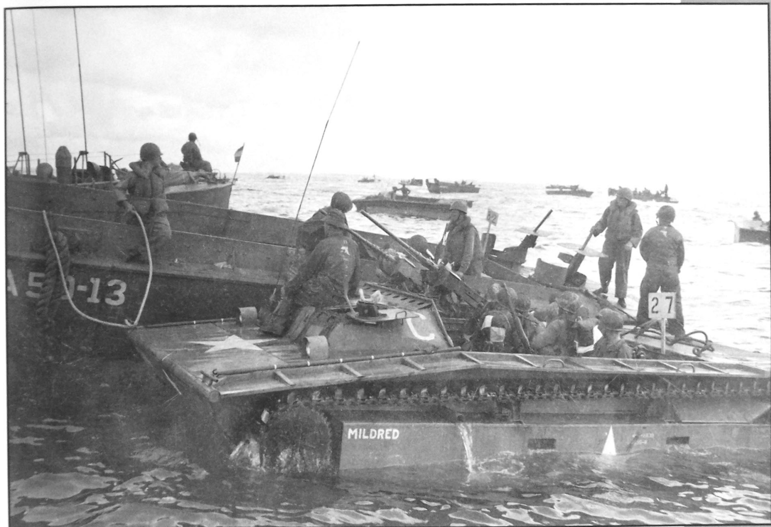
Men of the 7th Infantry Division move from an LCPV to an LVT-2 for the final ride into the beach during the Kwajalein landings, on February 1 1944. The wooden hulls of the LCPVs were vulnerable to damage by the coral reefs surrounding Kwajalein Island. This LVT-2 bears the name "Mildred" painted on the
