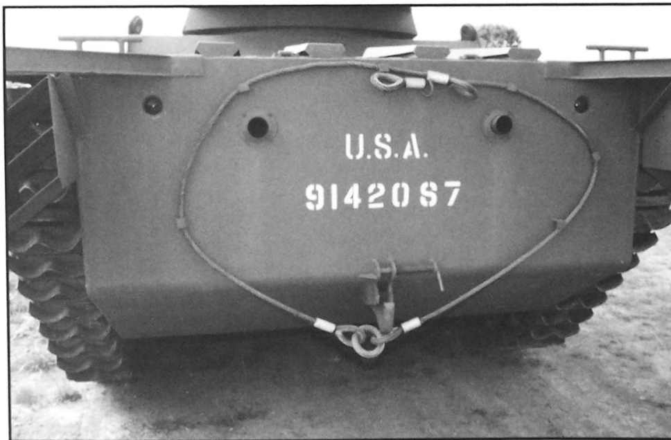
The rear hull (or stern) details visible here are the tail lights, engine exhaust ports, tow cable and it's mounting brackets and towing hitch. On the top deck you can see the armored covers for the engine vent and the early to mid production chock cleats.
