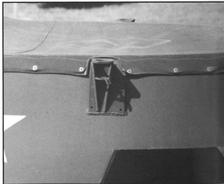
This vehicle appears to have a later production style turret. Even with the canvas cover attached, you can see that this turret does not have the ring mounted .50 caliber M.G. position in the turret top rear. It does have the mounts on the turret sides for the .30 caliber MGs. Also note the small circular weld detail on the turret cheek for the main gun mount.
