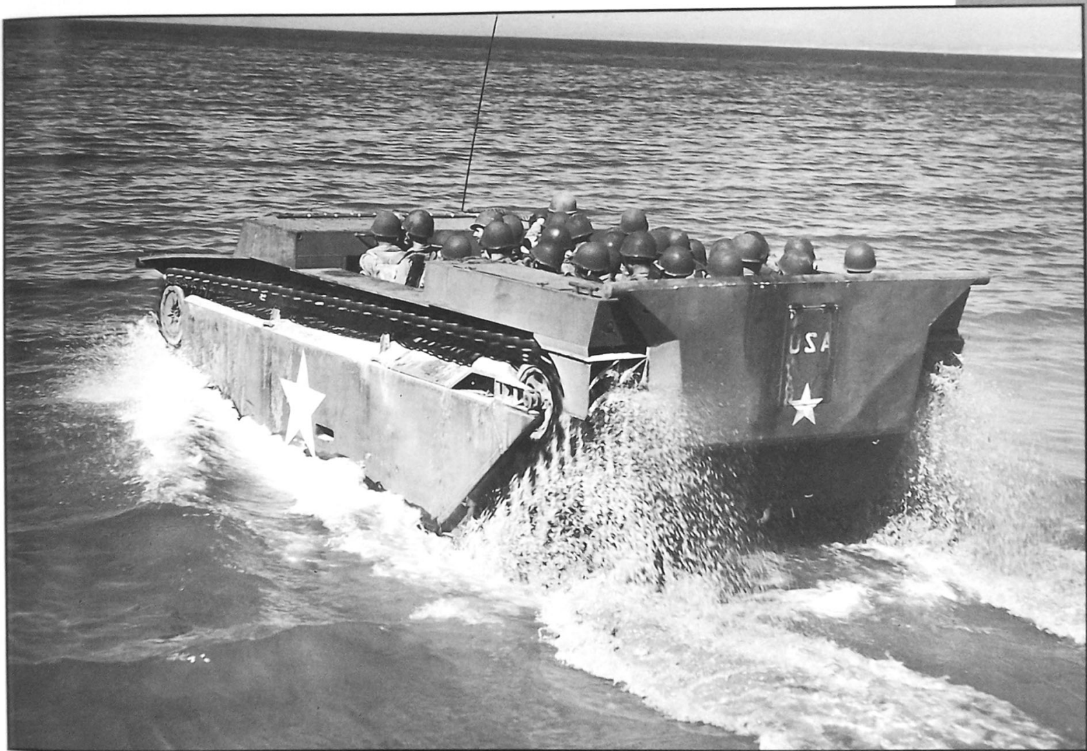
This photo shows an LVT4 also in the late war green color. No LVT4's were probably ever painted in the blue color as they were a later war version of the LVT and still being produced when the decision to paint LVT's in the green finish was made. A curious detail on this particular vehicle is that a piece of the
