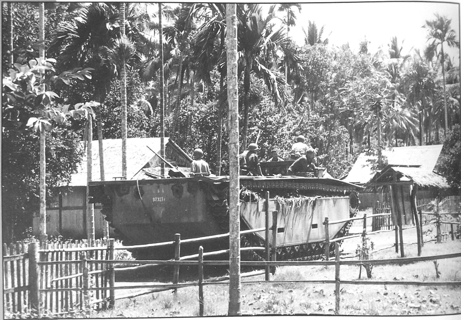
An Army LVT2 in support of the 124th Regimental Headquarters is seen moving through a native village on Morotai Island on September 17th 1944. An interesting feature on some WWII LVT2's and A2's is shown in this photo, the crew appears to be using a replacement radio mounted in the right front of the cargo compartment. You can see the antenna protruding above the vehicle in this position. Early LVT's
