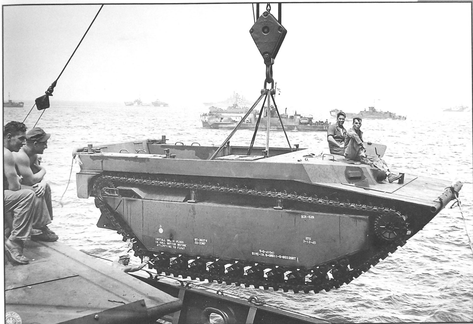
A great photo of an early production LVT4 that has been returned to a maintenance facility and rebuilt with some of the late production modifications, like the added vision ports in the cab front and sides and added armor plate in the cab sides. Note the three vision ports located on the front of the cab, the post-type
