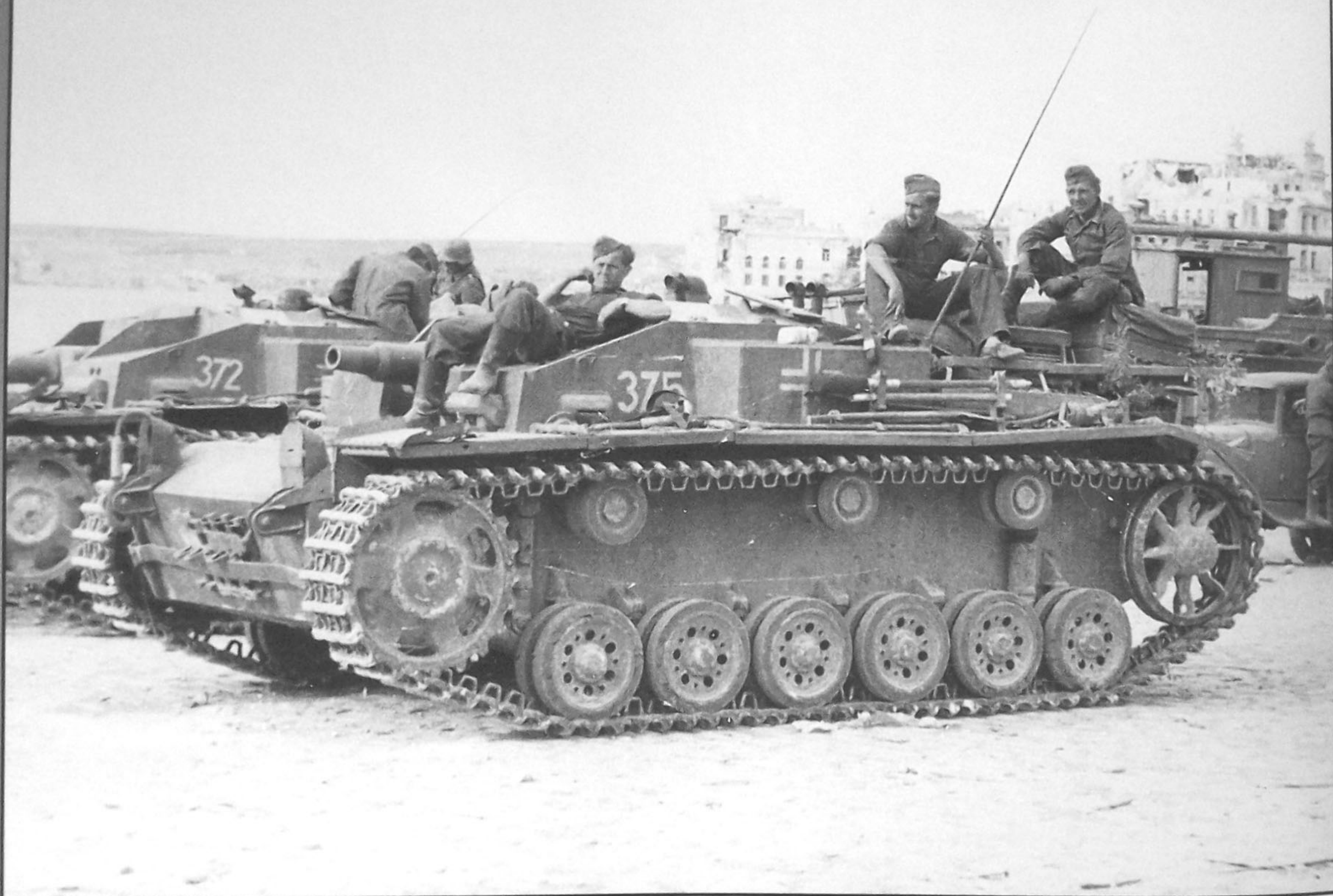
This StuG E and its crew await their orders at a port in southern Greece. The Ausf. E can be recognized by the large square boxes on either side of the upper superstructure. These were provided to accommodate the installation of new radio sets. (BA)
