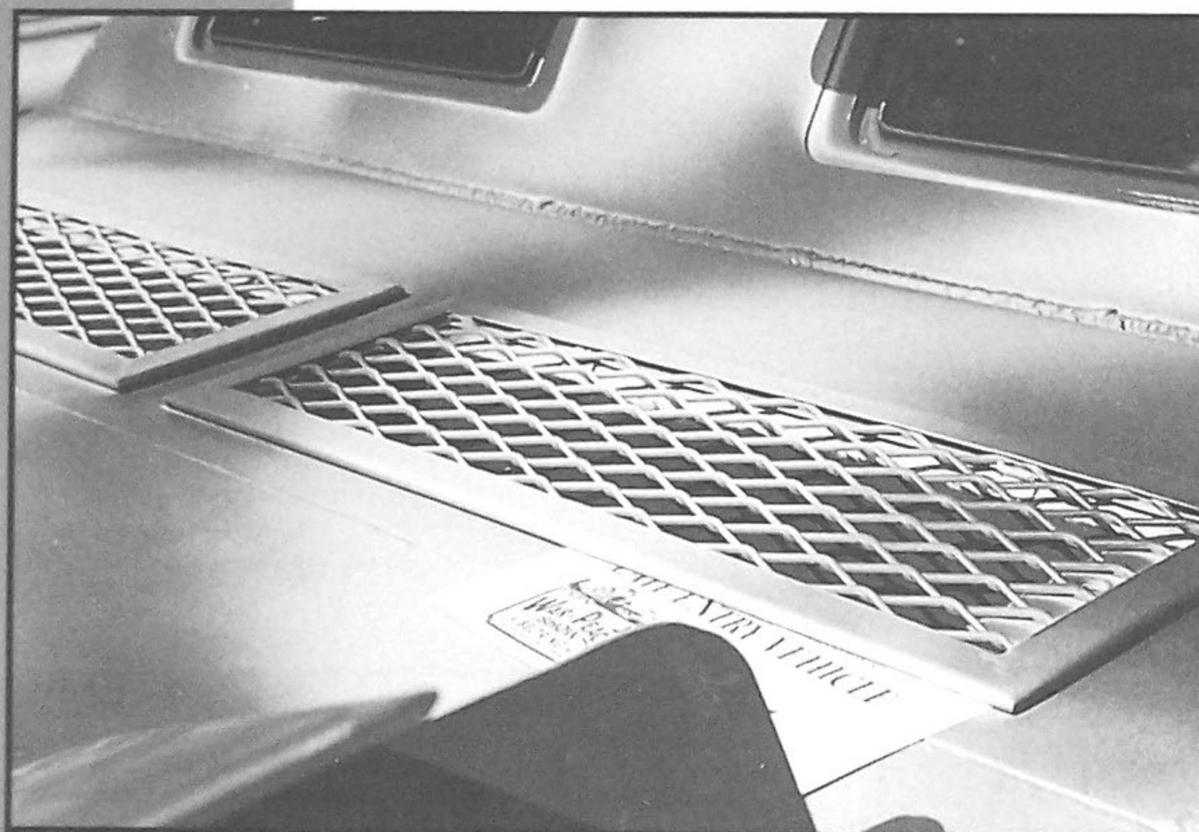
Top left: The engine access hatch on the right side of the engine compartment. This shot provides a closer look at the Solex carburetor and the intake manifold. The top of the right side stowage box and the rear of the pick can also be seen. Above left: These two grated openings provide ventilation for the engine and are located just in front of the driver's visor. Above right: A close-up of the latching mechanism on the side engine access hatch.
