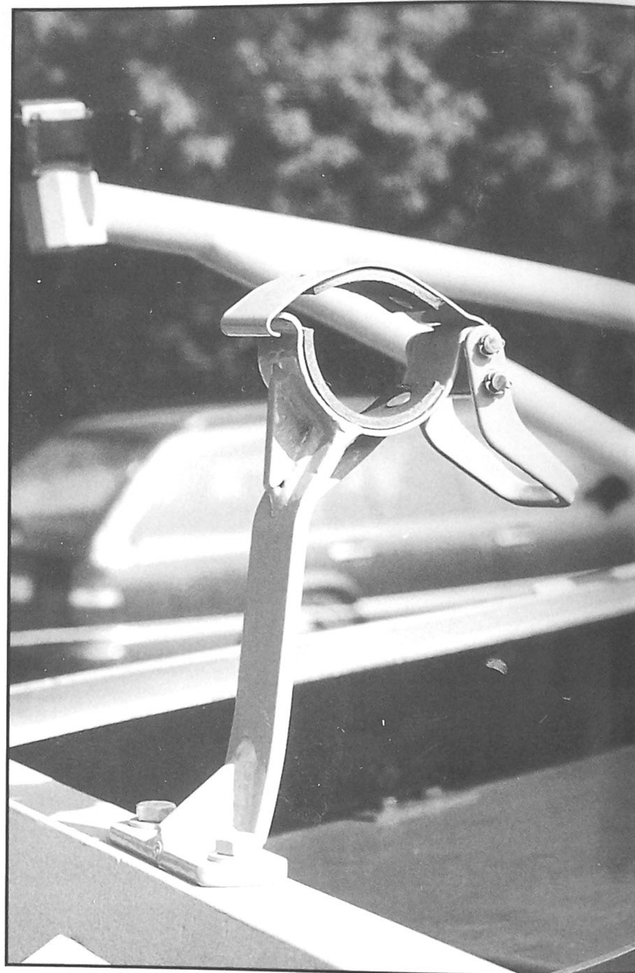
Top left: Another of the tarp tie-downs located around the top of the hull. Above left: This is the rear mounted MG rail. The two MG mounts denote a 250/1 (s MG), which carried the second, support half of the "Halbgruppe." Above right: This very interesting late detail is the travel lock for the rear mounted MG. It is installed on the top of the right rear superstructure.
