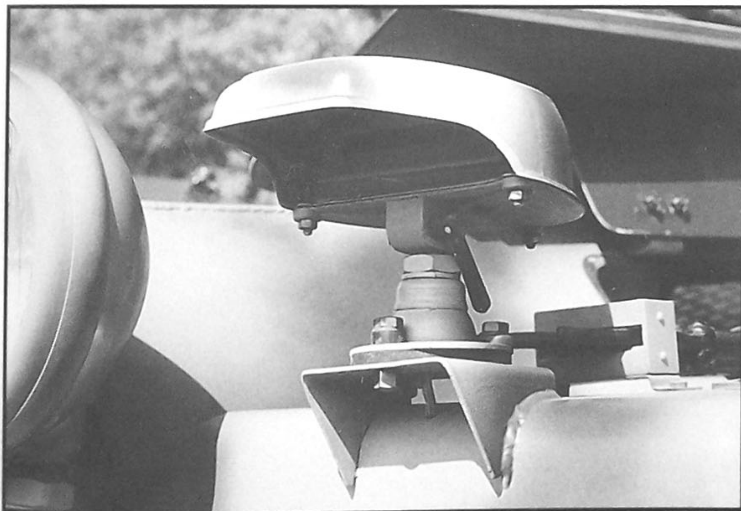
Top left: An overall view of the left fender showing the layout of the Notek light, distance marker and wire cutters. Above left: A close-up of the Notek light and its mount. Note the weld bead where the mount meets the fender. Above right: Another close-up of the distance marker, this time on the left side fender. This photo provides a good perspective of the mount of the rearview mirror mounted on the marker rod.
