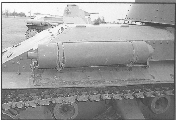
the jack. Above right: the large muffler on the right rear of the hull. Visible in this photo is one of a series of small rods welded along the fender line. It is thought these rods are to attach external stowage.
