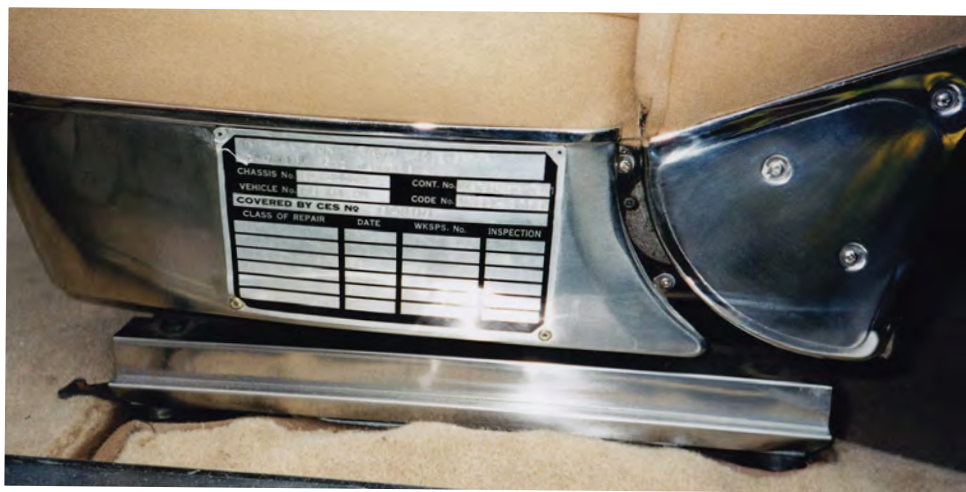
The military identification plate was fitted to the base of the passenger's side front seat. (Reinhard Stadthaus)
