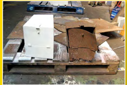
Little of the tin work was usable but it at least provided patterns so replacements could be made.
