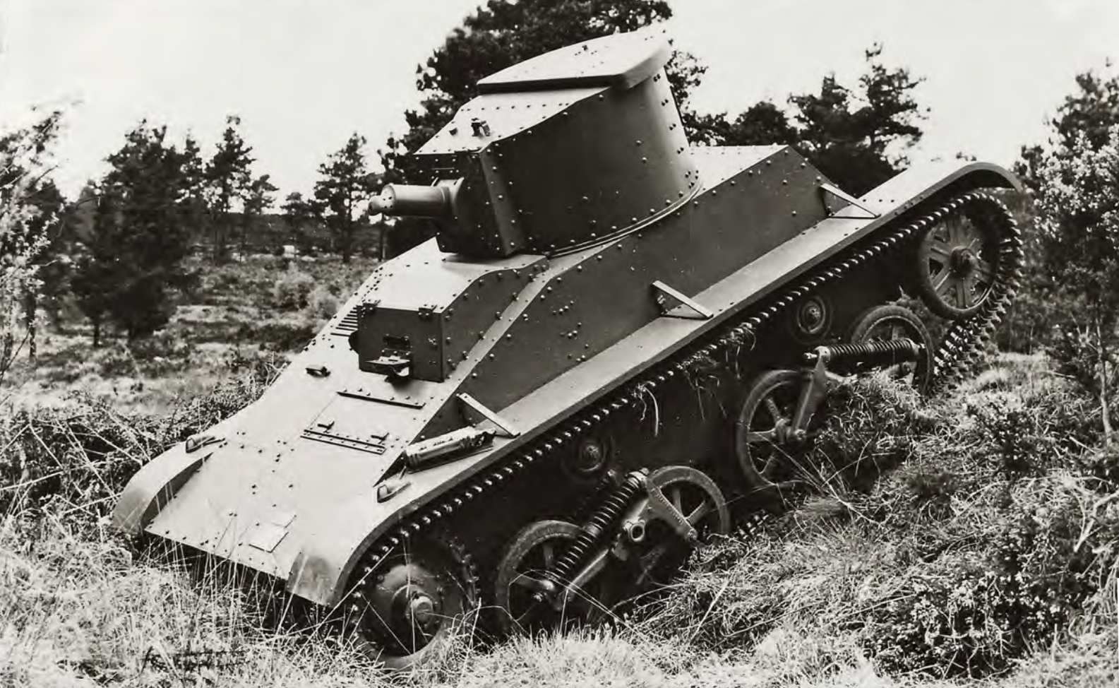
M1934 during cross-country trials. This one has coil spring suspension but like all these light tanks has front sprocket drive.
