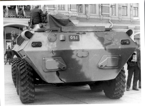
Rear view of the early BTR-90 prototype, showing the early hydro-jet propulsion system doors.
