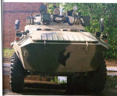
Above: An early BTR-90 prototype at the Omsk arms show in 1999 (Andrey Aksenov) Left: The BTR-90s turret, borrowed from the BMP-2, is apparent in this view.
