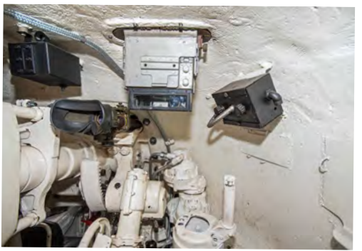
Above: The gunner's position showing his sight and periscope.
