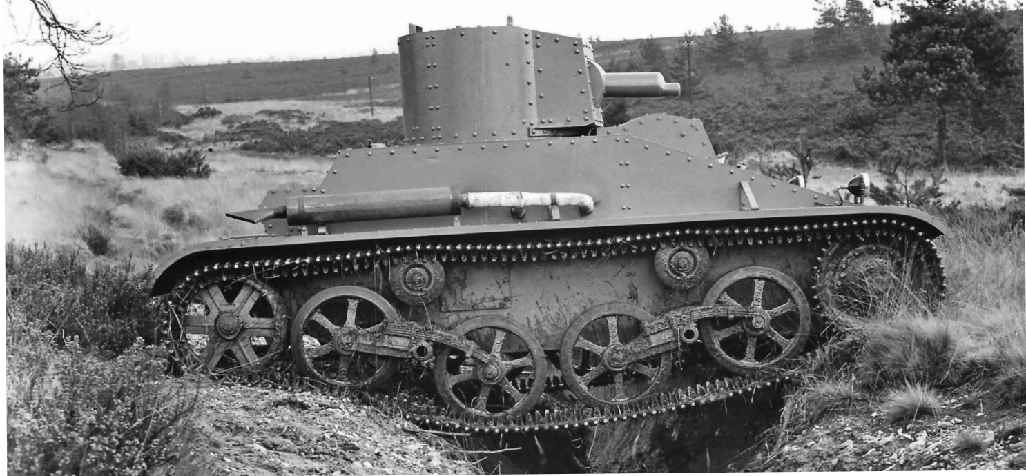
Above: M1933, with the original leaf spring suspension, giving a trench crossing demonstration.
