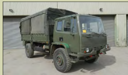
The DAF 4x4 Truck , Cargo capacity of 5000kg, Fitted Cummins 5.9 ltr Turbo Diesel, permanent 4x4, Hi Lo Ratio with Diff Lock, PAS, Air brakes, Nato style rear hitch, Engine power 145hp, Maximum road speed 89 km/h, Range 500 km, Year from 1994. Guide price from £4,500 (40 Available)
