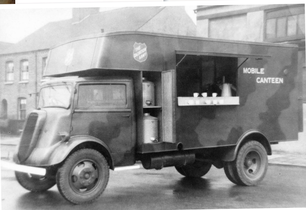
Above and right: Many 3-ton civilian wartime chassis were converted to canteens such as this Ford 7V operated by the Salvation Army. Note the placing of the hot water storage tanks behind the cab.
