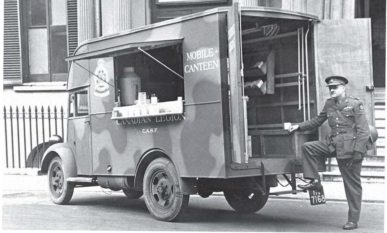
Above: The smaller Fordson E88W also provided a useful chassis to mount canteen bodies. This one, complete with camouflage paintwork, has been donated by the Canadian Legion.
