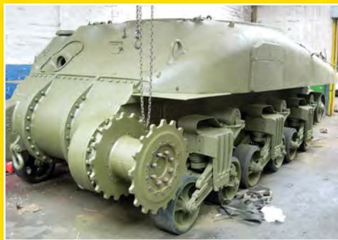
A rolling chassis with the three-piece transmission housing in place.
