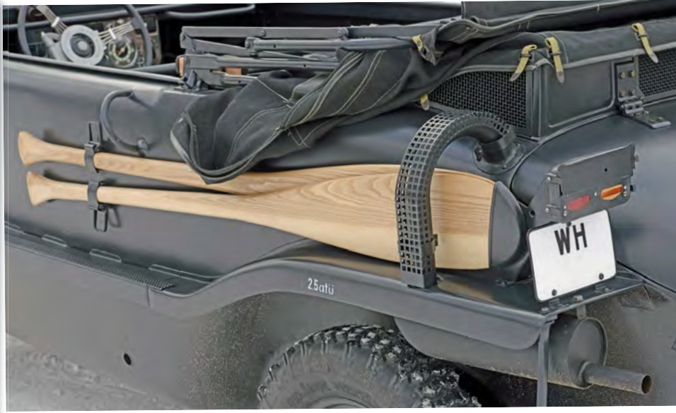
The fact that the exhaust system was located beneath the rear wheelarch proved to be one the Type 128's weak points. Note the twin oars.
