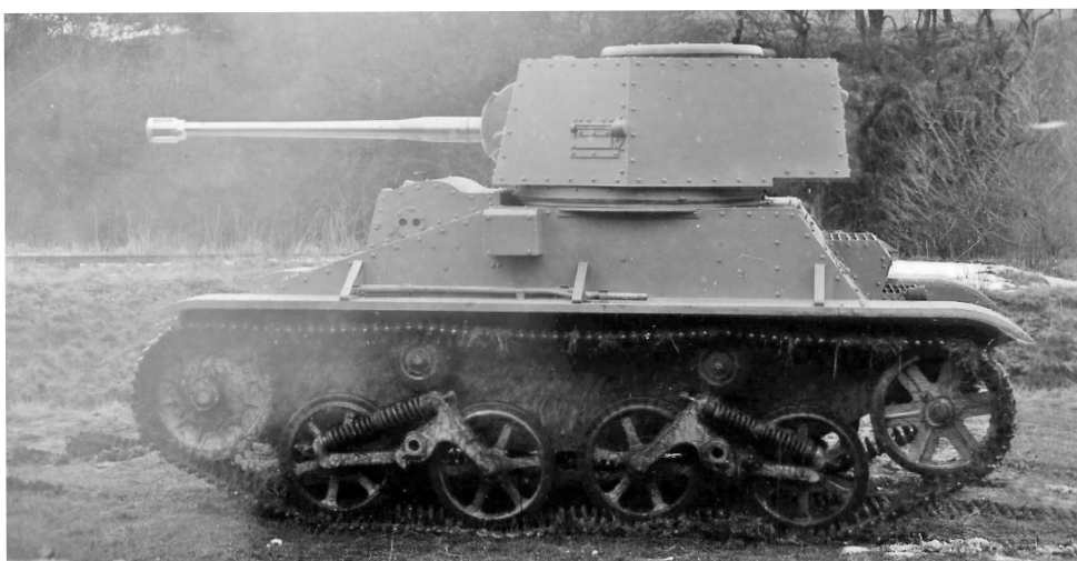
The Vickers-Armstrongs Light Tank fitted with its 40mm gun, as used by Latvia and now on display in Kubinka.
