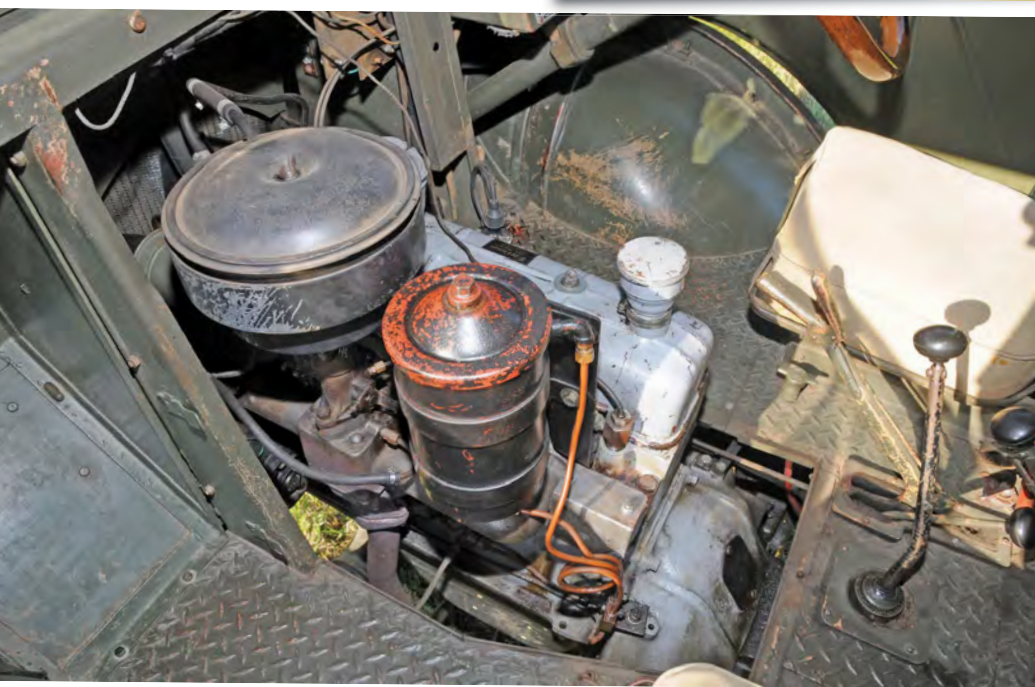
Six-cylinder 85bhp 3.5-litre GM engine runs as sweet as a nut following its rebuild by Pat Curran.
