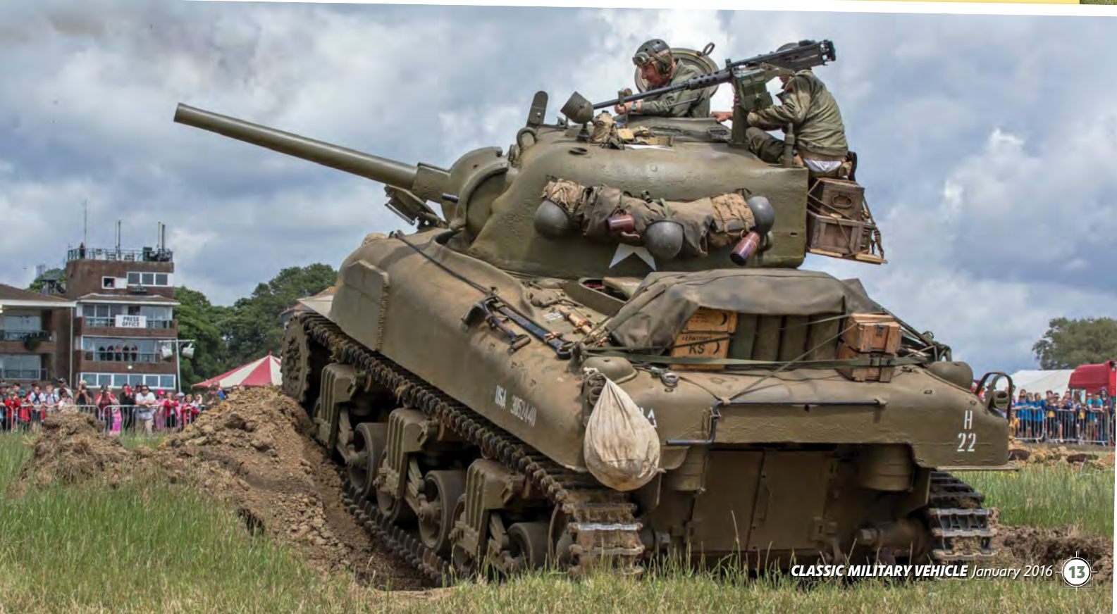
Below: It is said that the British Army requested that turret pistol ports remain a feature of Lend Lease Shermans although the US Ordnance Department had directed in the spring of 1943 that they be deleted from Shermans destined for US forces. Grizzly turrets, however, were cast by General Steel in Pennsylvania and did not have turret ports.
