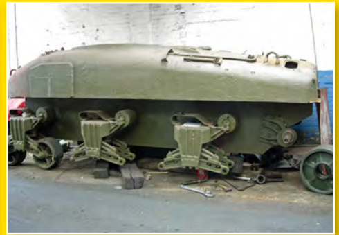
First the wheel stations were overhauled and refitted so giving Jez a rolling chassis.
