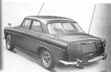
These are the military handbook identification drawings of the 'Car, Saloon, Grade 2, 4x2, Rover 3½-litre'. The roof aerial is a standard Rover fitment; the rear aerial is for the R/T. The flagstaff mount on the bonnet differs from those on known cars, and there is an additional spotlight below the front bumper. (Dave Cole)
