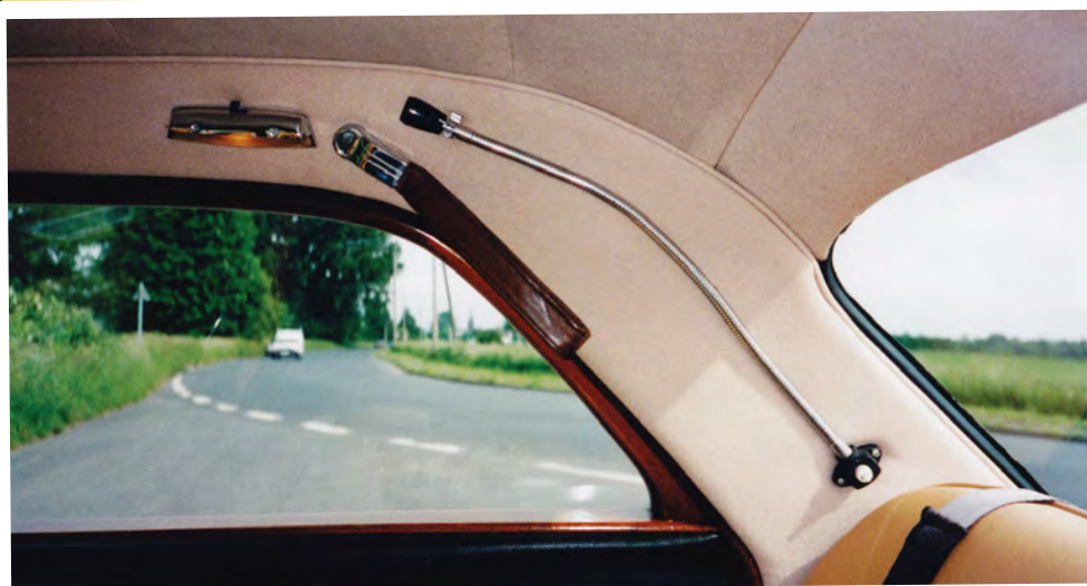
Additional reading lights like this one seem to have been fitted to all the military Rovers. The dowager strap was a standard production feature, although in this case the original cloth-faced type has been replaced with a leather one. (Reinhard Stadthaus)
