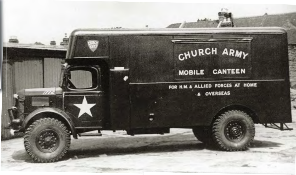
Above: A further image of the Austin K4 3-ton depicting the position of the rear opening doors. This one has been fitted with a large roof rack, although what it was used for is unknown. This type of canteen served both at home and abroad. Right: An Austin K4 3-ton canteen seen here at the coachbuilder's premises, believed to be J C Clark of Greenside, London. The drop down is closed but just visible under the front of the body is the spare wheel and the door for providing access to the water heater behind the cab.
