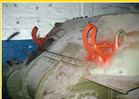
Jez and his team fabricated such items as new light guards.
