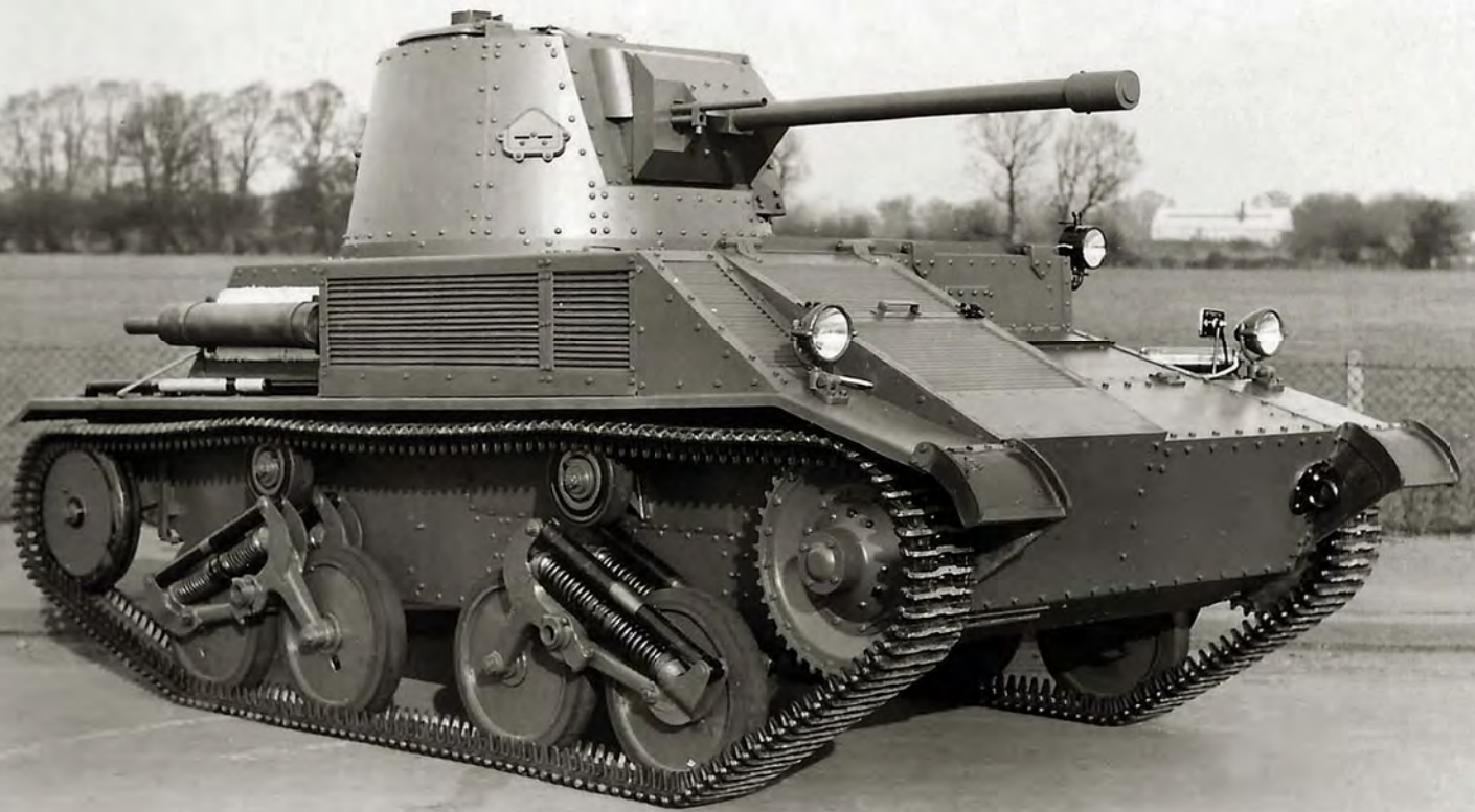
A very late production, the Vickers-Armstrongs Command Tank with a 40mm gun in an enlarged turret. In fact this tank is larger in most respects than the ordinary commercial light tanks but it never sold.
