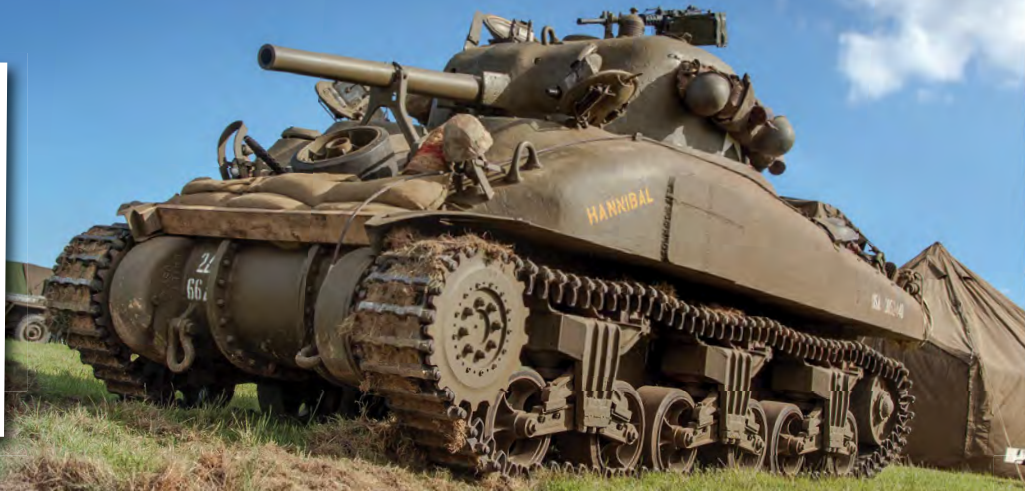
Above right: Because the US Ordnance Department had decreed that US-produced Shermans would be manufactured with a one-piece differential housing by September 1943, it has to be concluded that the Grizzly was the last M4-family gun tank to be produced with the three-piece housing.
