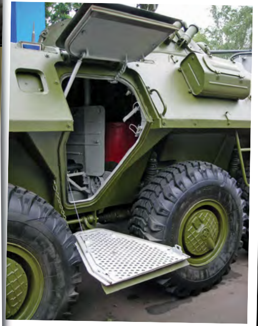
The BTR-90s exit doors are between the second and third axles as with all Russian wheeled APCs since the BTR-70, with the doors opening vertically to form a footplate and overhead cover respectively.
