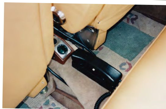
Above and left: The system fitted to 08 FM 40 is different, with the head unit mounted on the front parcel shelf but the R/T handset between the seats. Those are not cables beside the handset, but the tubular stalks of the front seat belt lower mountings, and the domestic carpet in the footwells is not original! (Reinhard Stadthaus)
