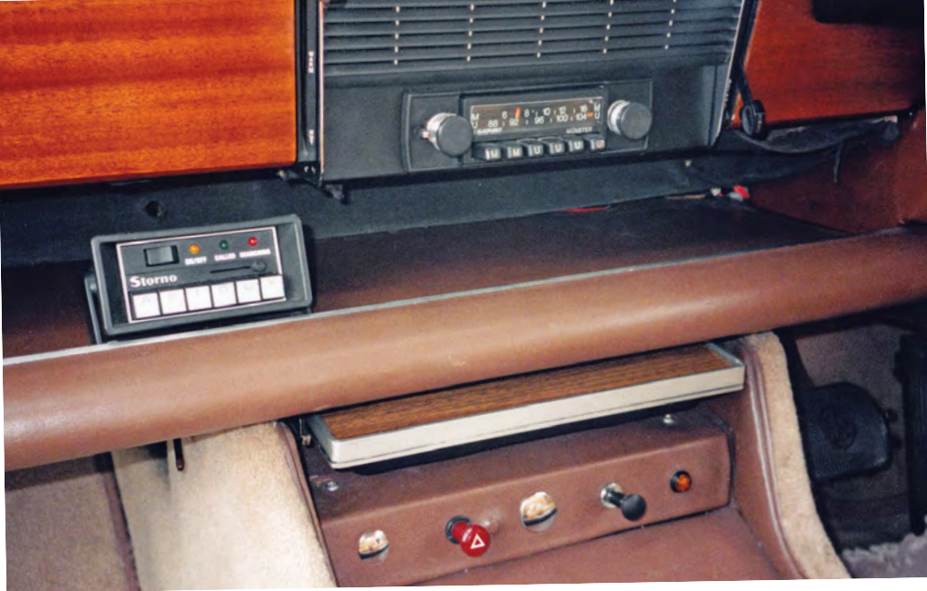
Above and left: The system fitted to 08 FM 40 is different, with the head unit mounted on the front parcel shelf but the R/T handset between the seats. Those are not cables beside the handset, but the tubular stalks of the front seat belt lower mountings, and the domestic carpet in the footwells is not original! (Reinhard Stadthaus)
