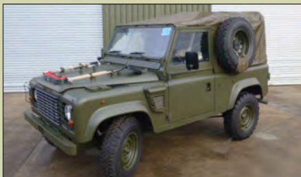
Land Rover Wolf 90 300Tdi Hard Top RHD , Fitted 300Tdi engine, 5 speed R380 gearbox, Hi/Low transfer box with centre diff lock, full FFR installation kit, 24-volt electrics, PAS, front and rear disc brakes etc, Mileage from 45110km, Guide price from £10,995 (6 Available)
