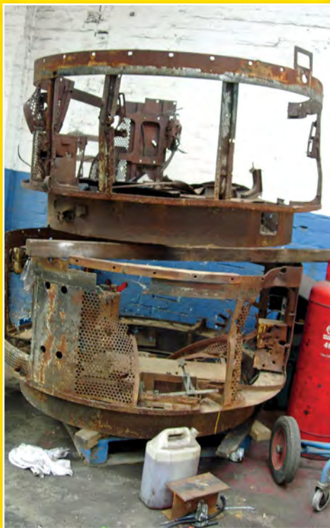
Above: Neither of the two battered, original, turret baskets were usable...
