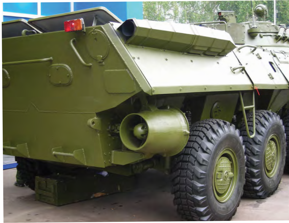
The latest BTR-90 has a myriad of engineering modifications, including new tyres and hydrojet propeller pods mounted externally to the armoured hull.
