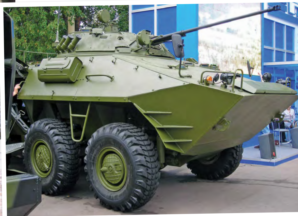
Above: An early BTR-90 prototype at the Omsk arms show in 1999 (Andrey Aksenov) Left: The BTR-90s turret, borrowed from the BMP-2, is apparent in this view.
