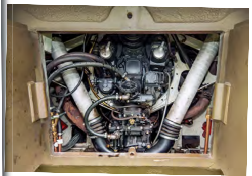
Hannibal's Continental R975 nine-cylinder radial was rebuilt by Carl Brown's C & C Military.
