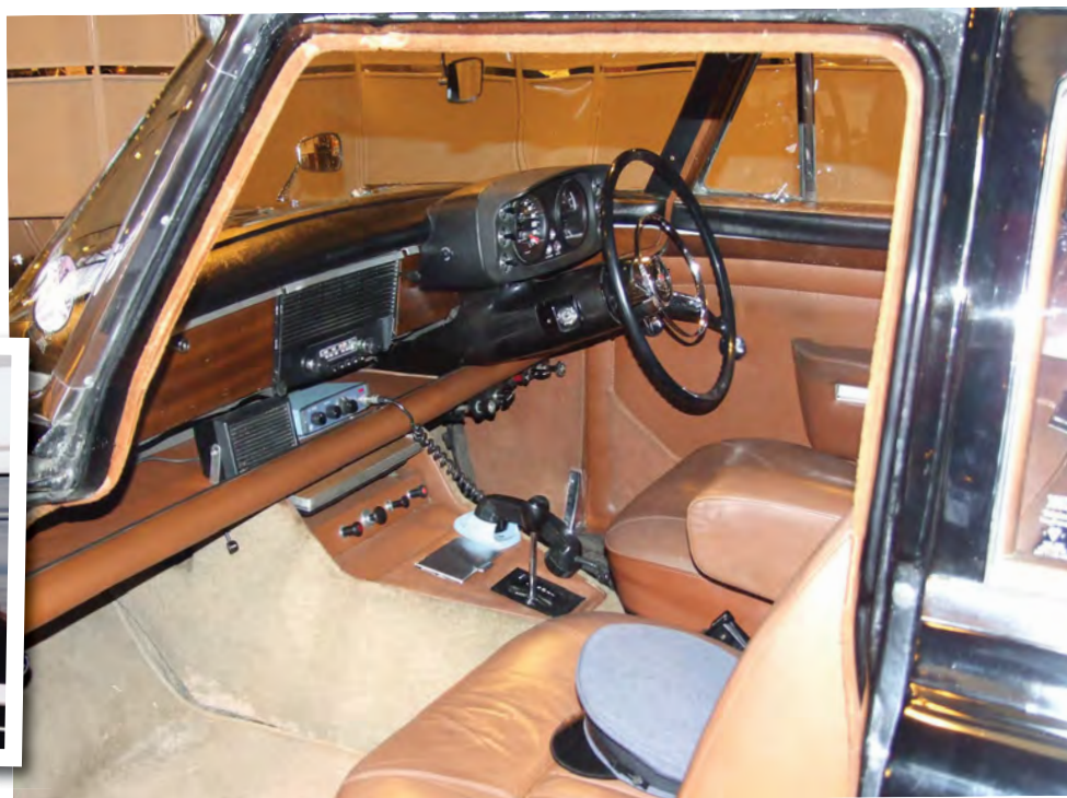
The front interior of 59 AM 19 shows the R/T system with its tuner and speaker mounted on the parcel shelf and the handset on the console next to the driver. (Dave Cole)
