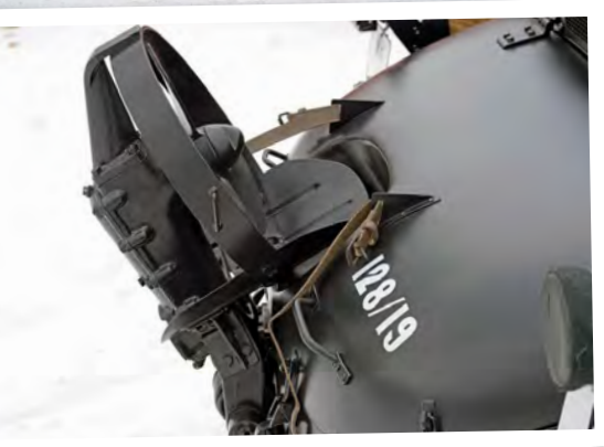
Above: Schwimmwagen employed a three-blade propeller which could be lowered down when it entered the water. Right: Type 128 cabin was relatively well equipped.
