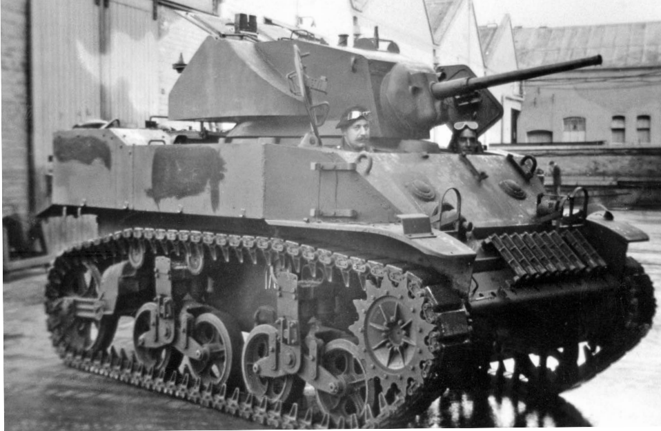
This M5A1 has been newly delivered into British hands and awaits stowage. However, it does provide an excellent view of the fared shield attached to the right side of the turret, behind which was kept the anti-aircraft machine gun.
