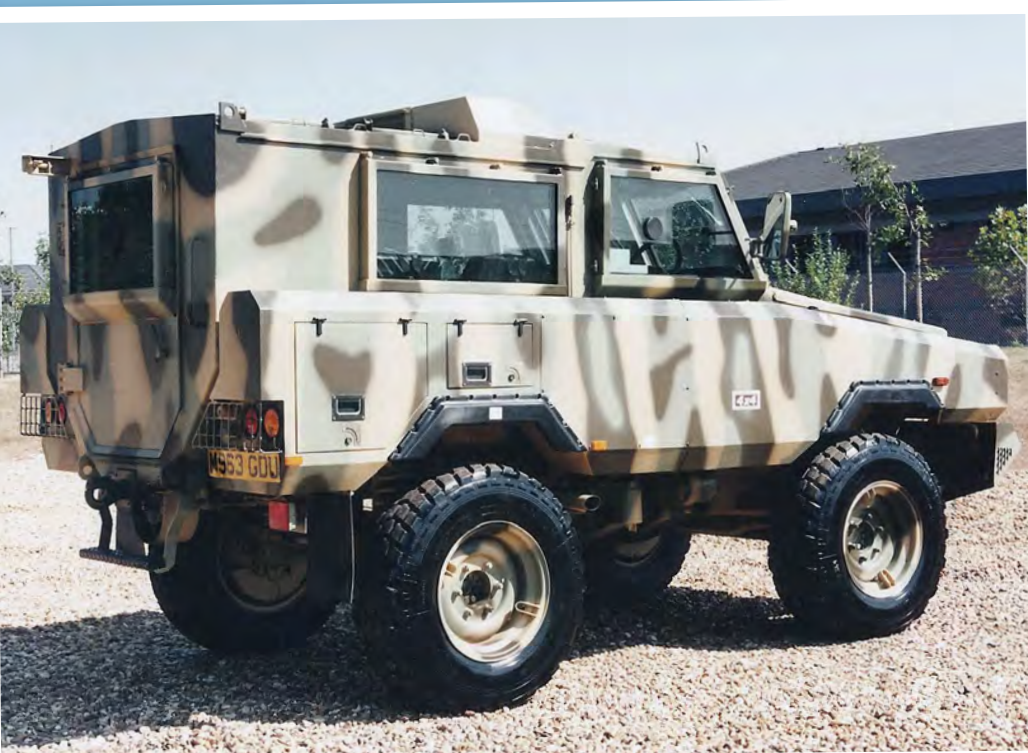
The Alvis 8 showing the rear door access for crew, and storage lockers for tools and other ancillary equipment.
