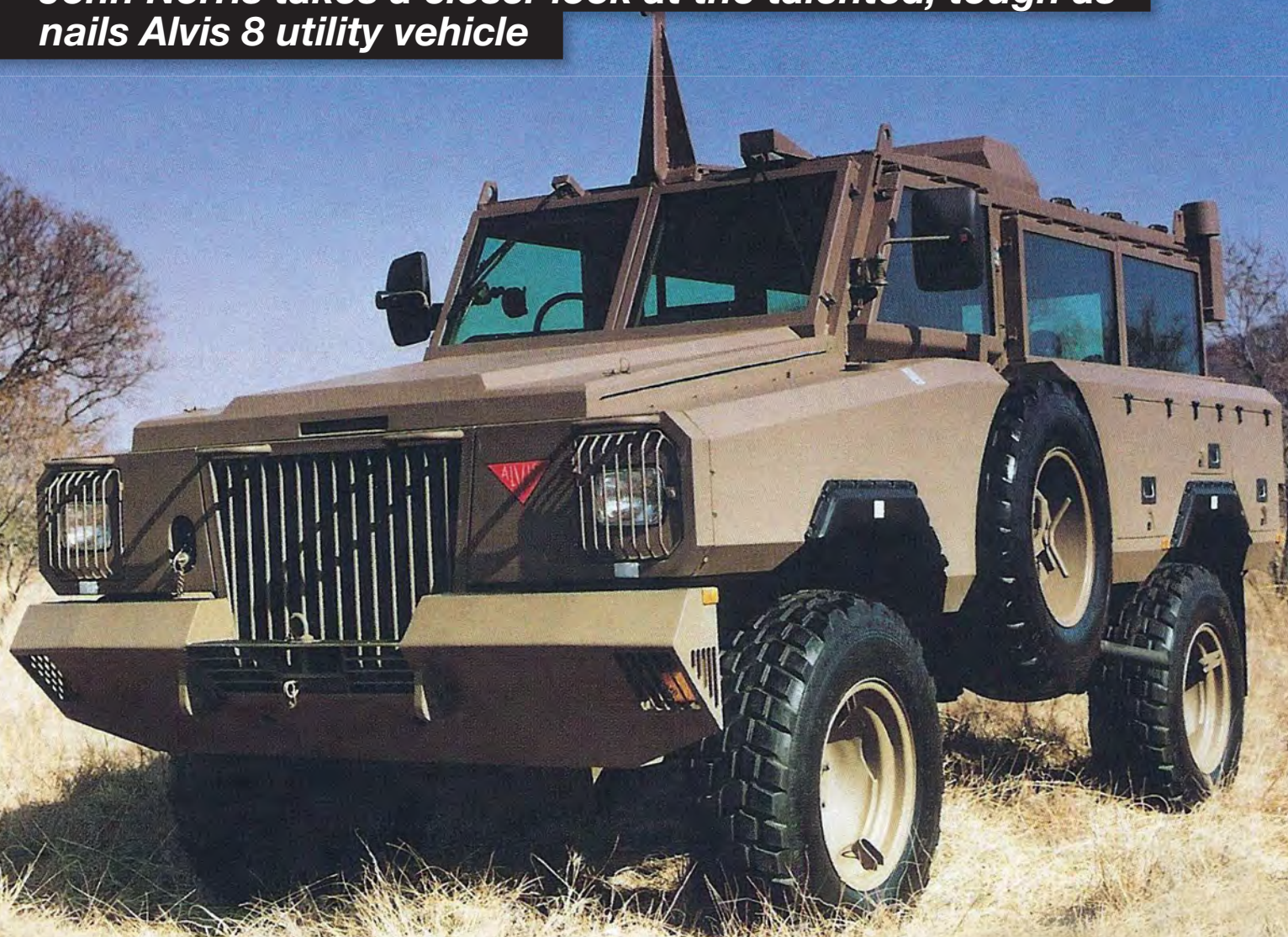
The Alvis 8 in its basic role as an APC for nine men and two-man crew. It had impressive protection against blasts.
