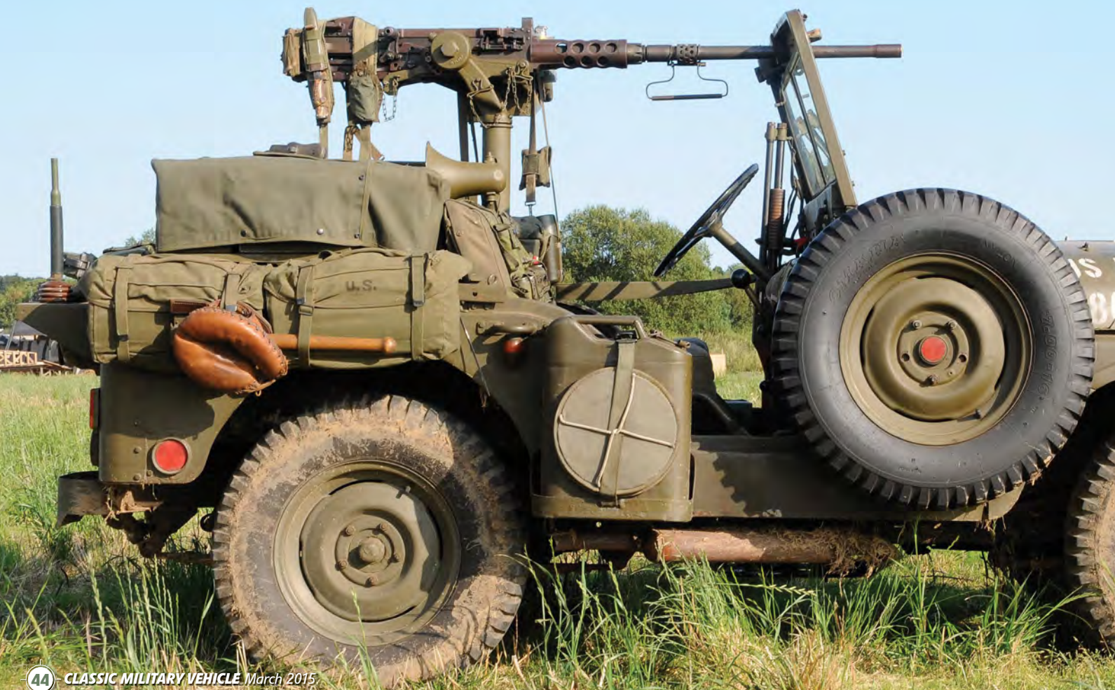
Below: The side mounted spare wheel on the C type models leaves the back free for the gun breech and spare ammo tubes. The windscreen is split in half for the barrels to slot through. James's .50 calibre variant has a smaller cut out to the screen.
