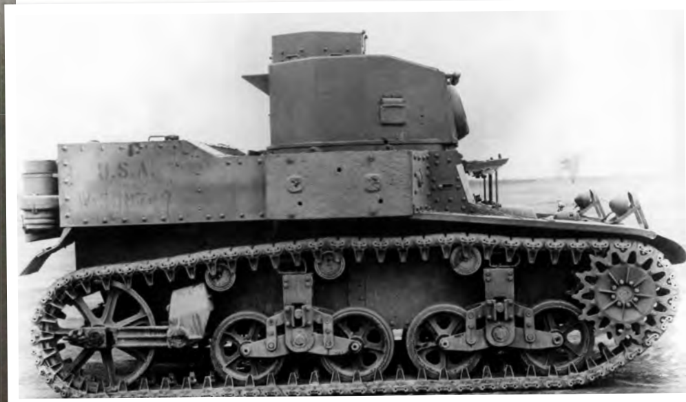
The converted tank with the enlarged engine compartment to accommodate the two Cadillac engines. Designated M3E2 it was later rebuilt, almost to M5 standard.
