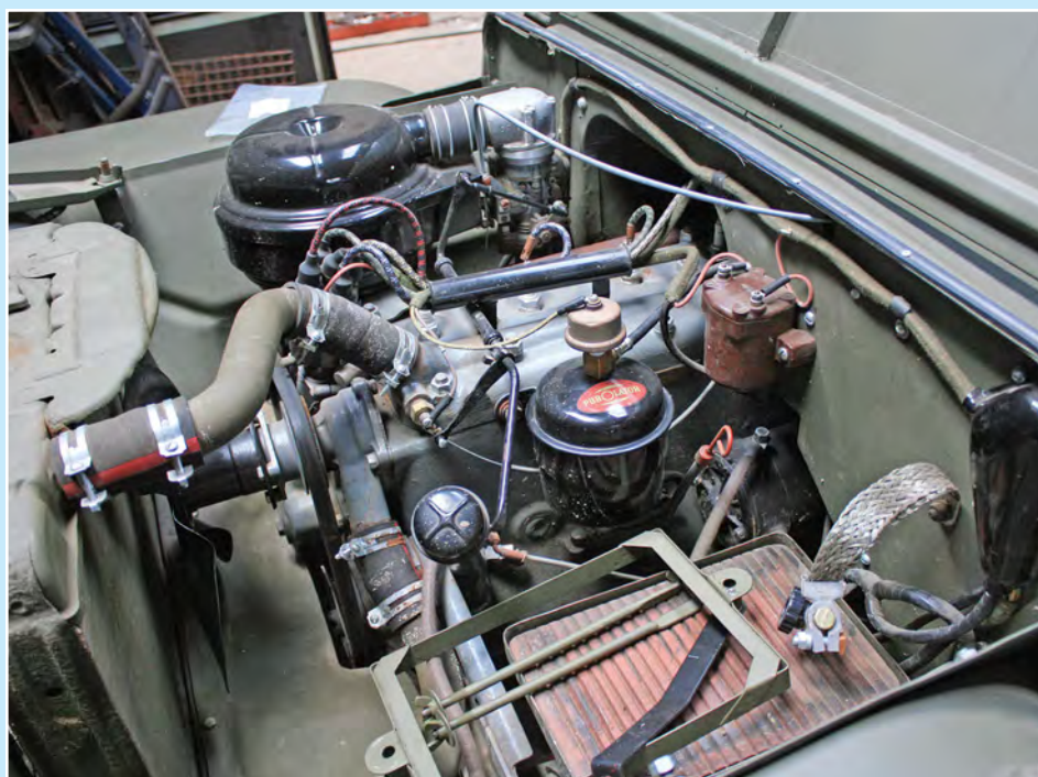
Ford GP was fitted with Fordson N tractor engine which is very different to the later GPW unit.
