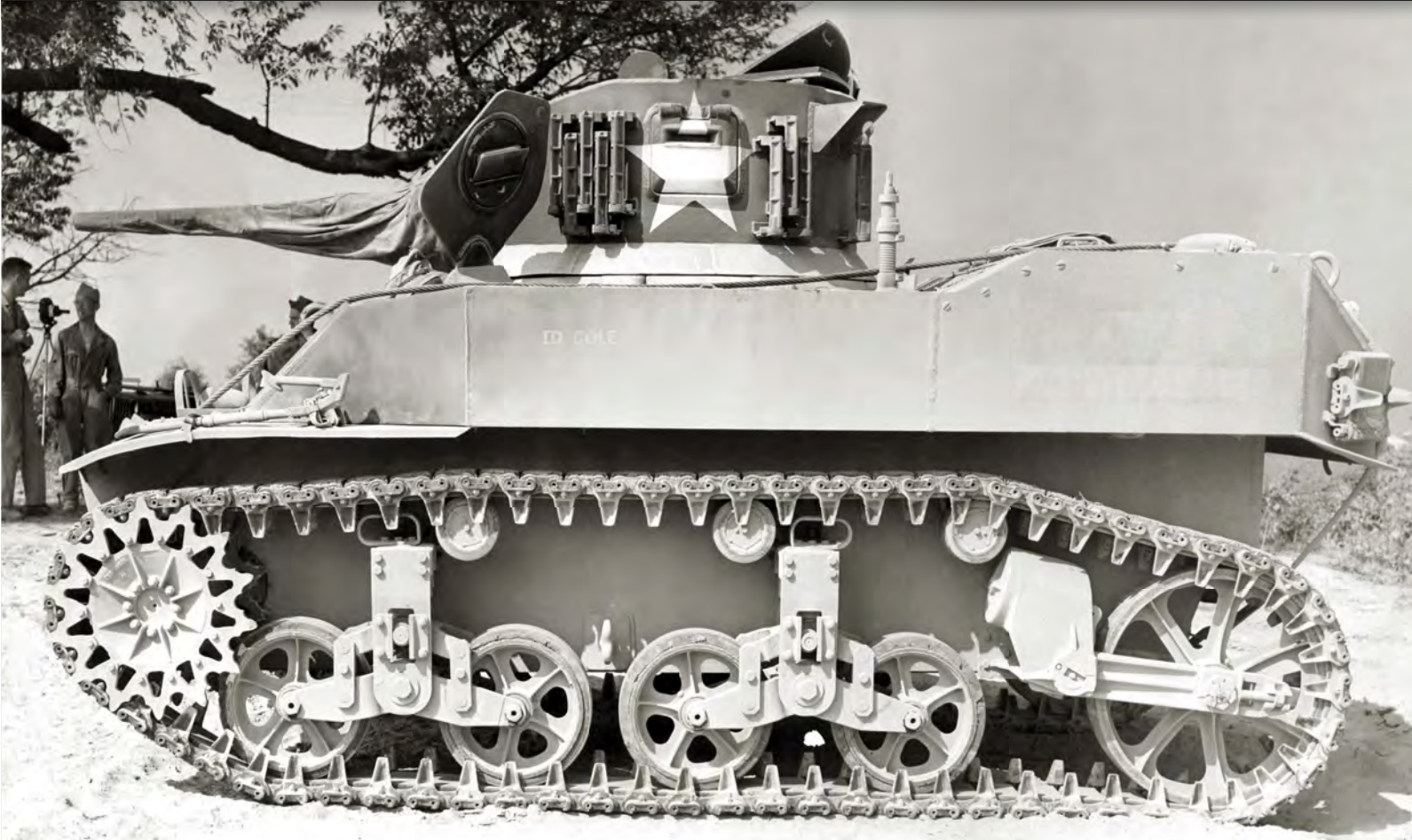
An M5 in mint condition, in what appears to be a desert setting. The driver's hatch is wide open but a canvas shroud covers the gun and mantlet.
