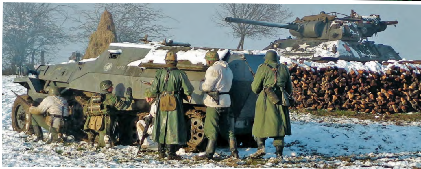
Above: Hugo Jottard's OT-810 (Czech post-war copy of the Sd.Kfz 251 Ausf D).
