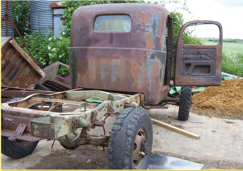
Above and right: This is how the WC1 arrived. All the woodwork had been removed due to infestation.
