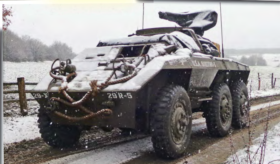
Above: Like the Ford M8, due to limited forward visibility, the M20 is difficult – and dangerous – to drive without an assistant.
