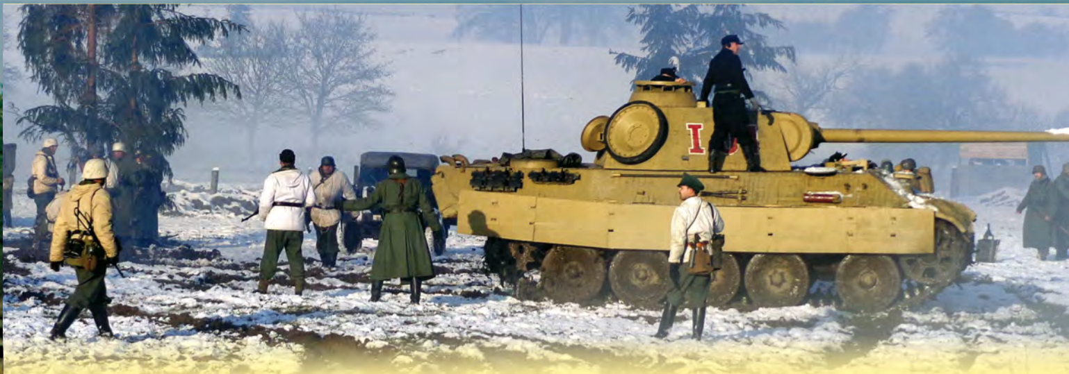
The Pz.Kpfw. V Panther, in fact a super copy built on a T-55 recovery tank by a Polish team, was a major attraction of the re-enactment.
