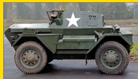
Above: An ex-WW2 British Army Daimler Dingo armoured car. These were introduced in 1940 and continued in service until 1968.
