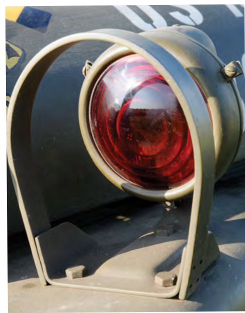
Extra lighting was added to the Dutch models to make them road legal.
