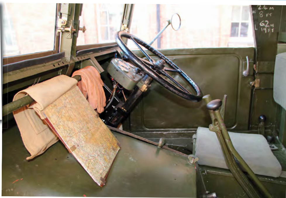
Above and right: Inside the cab it is certainly cosy with the six-cylinder petrol engine situated between driver and passenger – the open-sided nature of the cabs was very much a welcome relief in summer but not so much in winter.
