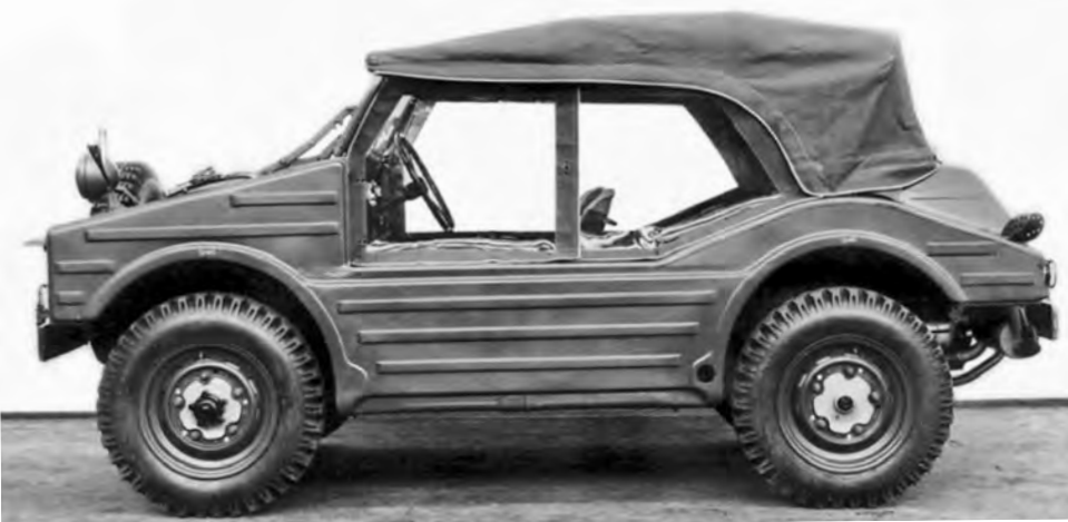
The Karmann redesign went further than is immediately obvious. Note in particular how the tail has been changed and the canvas hood repositioned relative to it.
