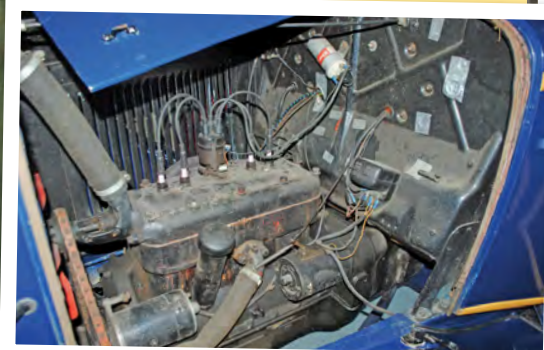
Above: The Ford 3.3-litre engine is awaiting a new head gasket. Right middle: As you would expect, the driver's seat and the controls are very simple. Far right: The cab of Jones's van with original headlights.
