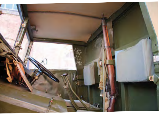
Above and right: Inside the cab it is certainly cosy with the six-cylinder petrol engine situated between driver and passenger – the open-sided nature of the cabs was very much a welcome relief in summer but not so much in winter.
