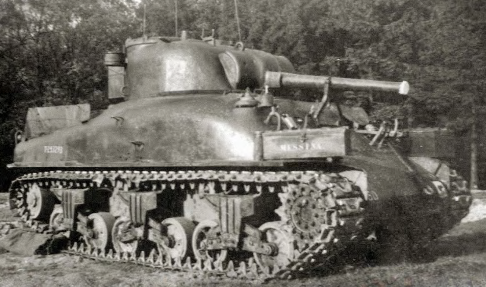
The M4A1 Sherman II Command tank which was the mount of Brigadier Mike Carver in North West Europe. The number of extra aerals is the real clue although outwardly it looks like any other Sherman, with perhaps a bit more stowage.
