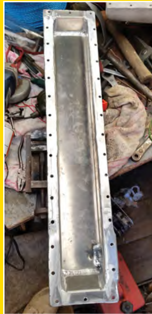
Above and above right and below: One of the biggest jobs of the whole restoration was the radiator, with the bottom tank having 13 holes in it and requiring some serious work to bring it back to life.
