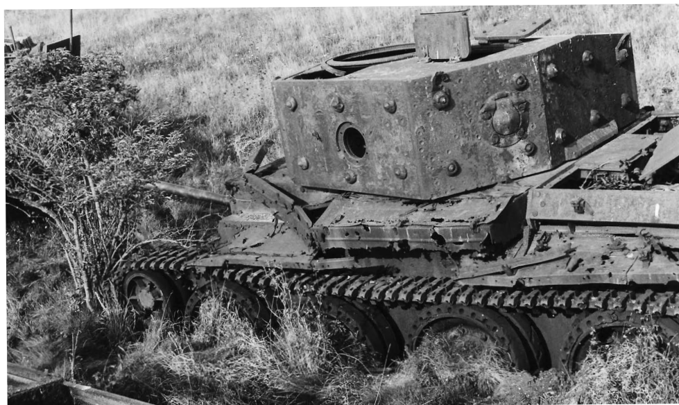
The A24 Cavalier Amoured Observation Post tank as found on Salisbury Plain before recovery to the Tank Museum. It bore the Panda's head marking of 9th Armoured Division but requires a lot of work before it can go back on show again.
