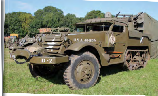
Above: Half-tracks fulfilled a number of roles throughout WW2, this example being a White M16 anti-aircraft variant – carrying four .50 calibre machine guns and owned by Stuart Wright. Note the hinged top sections of the hull sides allowing greater movement with the gun.
