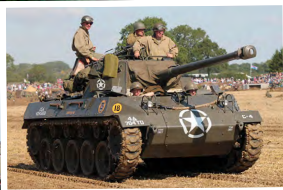
Above: This Hellcat shows its turn of speed as it heads into the arena. The M18 had a top speed of 55mph (88km/h), making it the fastest piece of armour used during WW2.
