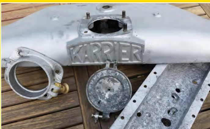
Above and above right and below: One of the biggest jobs of the whole restoration was the radiator, with the bottom tank having 13 holes in it and requiring some serious work to bring it back to life.
