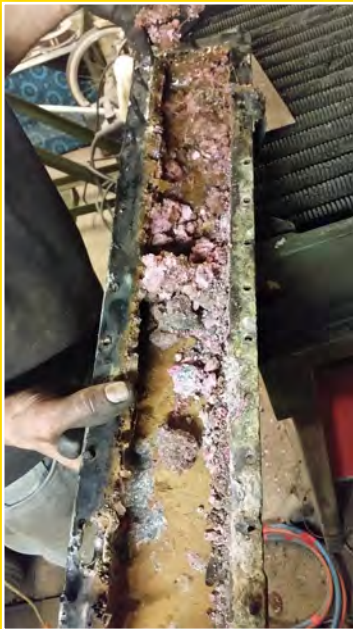
Above and above right and below: One of the biggest jobs of the whole restoration was the radiator, with the bottom tank having 13 holes in it and requiring some serious work to bring it back to life.
