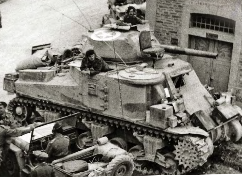
Left: A Grant Command tank in South African service in Italy. It has been adapted to look a bit like a Sherman although the seat in front of the turret is a bit of a giveaway. Notice too that the hull-mounted 75mm gun has been removed and the area in front of it cluttered up with stores.
