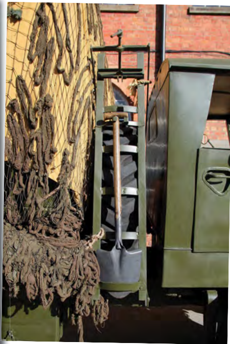
The spare wheel is stowed behind the driver’s side of the cab.
