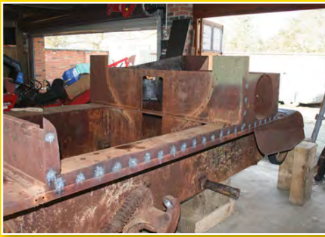
Most of the right-hand armour plate had been removed and holes cut in the sides of the forward compartment.
