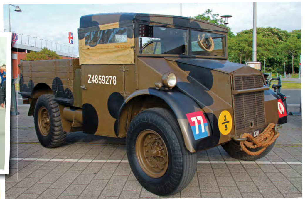
Above: The theme of rare British WW2 vehicles continued with this 1940 Guy Ant which is owned by Jim Ayles-Smith from Essex. 500 were built between 1939 and 1942 with 50 being adapted for use in Norway as a radio truck. Subtle changes included a solid roof, doors, dynamo unit and heating system for the engine. This vehicle actually never got to Norway though and was used in the push through Europe in 1944.
