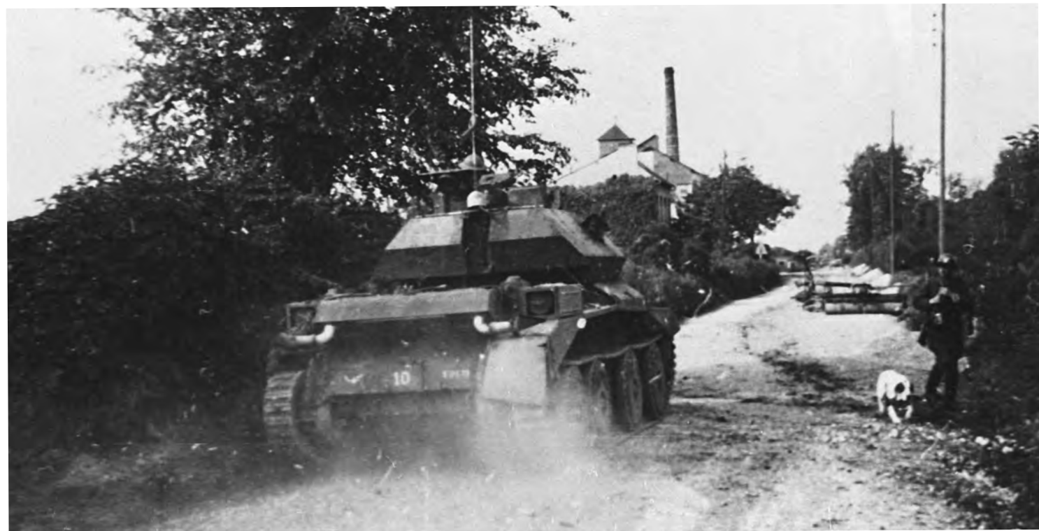
Another A13 Mk II, this time belonging to 5th Royal Tank Regiment, hurries along a road in France. Notice the agricultural equipment used as a partial road block and the soldier with the dog on the right. The wireless aerial on the turret could be folded flat to reduce the tank's silhouette. [Tank Museum 1324 D3 1]
