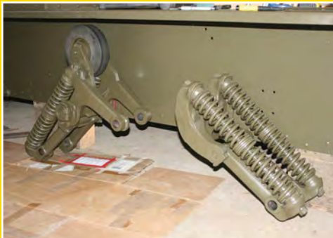
Suspension components refitted after overhaul and painting.
