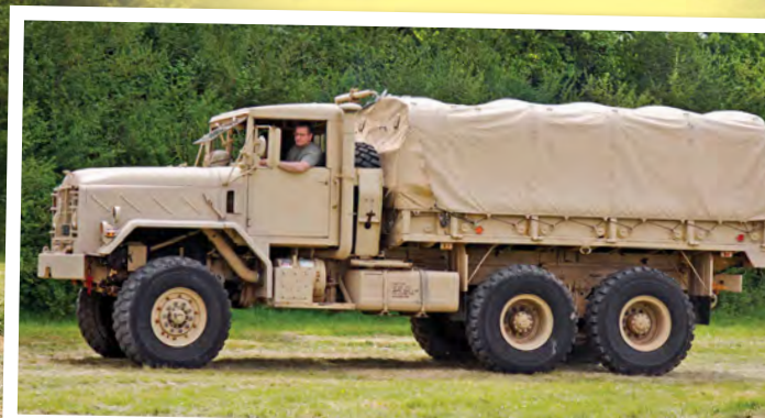
Below: Powered by a 14L Cummins diesel engine, this AMG General M923A1 general service truck served in Iraq 1 and recently saw service in Afghanistan with the US Army, attached to the 118th MP Brigade towing artillery. The owner is Andy Wright, and it has been in his possession for a year.
