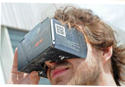
Google's cardboard virtual reality viewer allows a smart phone or android device to be slotted in the end.
