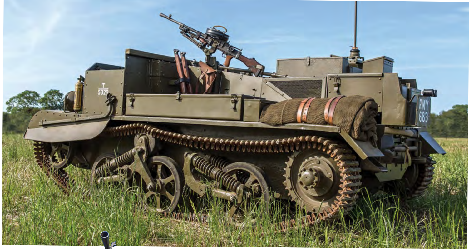
The rear of the Scout Carrier is virtually a mirror image of the Bren, with the storage locker on the left and the crew compartment on the right. A Bren is pintle mounted for use by the radio operator.
