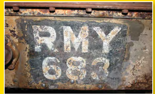
Carefully removing layers of paint revealed the original registration number.
