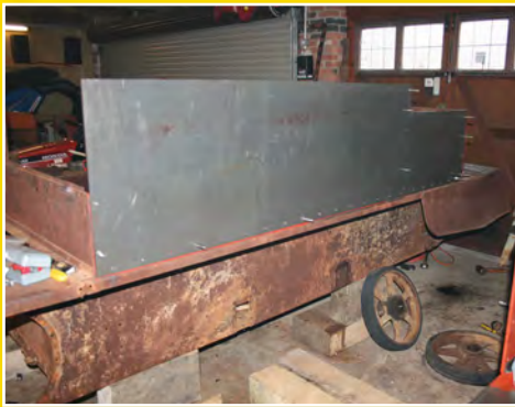
Sheet steel replacing the right-hand side armour temporarily fixed in place.
