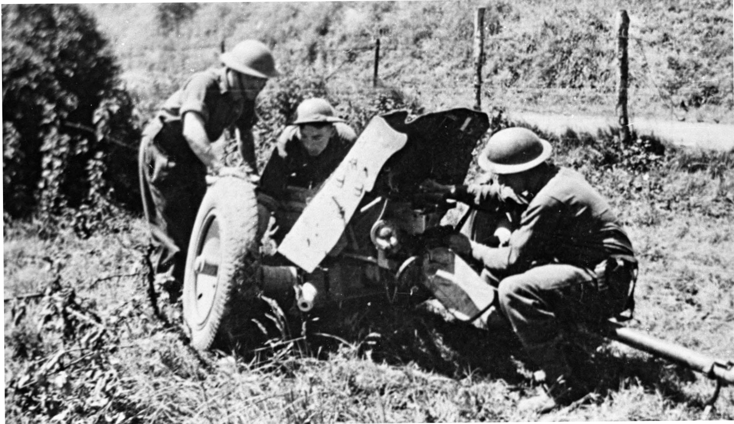
British soldiers examining a knocked out 3.7cm Pak 36 anti-tank gun near Honicourt. This gun had the ability to penetrate 30mm of armour at 500 yards so it could just about deal with a British cruiser tank. [Tank Museum 1323 D2 1]
