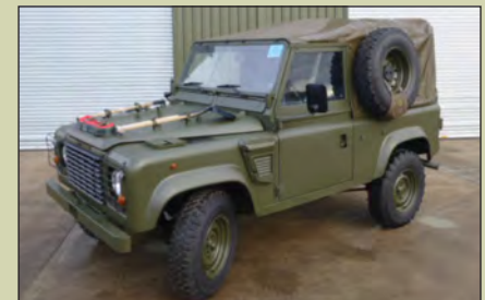
Land Rover Wolf 90 300Tdi Hard Top RHD , Fitted 300Tdi engine, 5 speed R380 gearbox, Hi/Low transfer box with centre diff lock, full FFR installation kit, 24-volt electrics, PAS, front and rear disc brakes etc, Mileage from 45110km, Guide price from £6,950 (6 Available)
