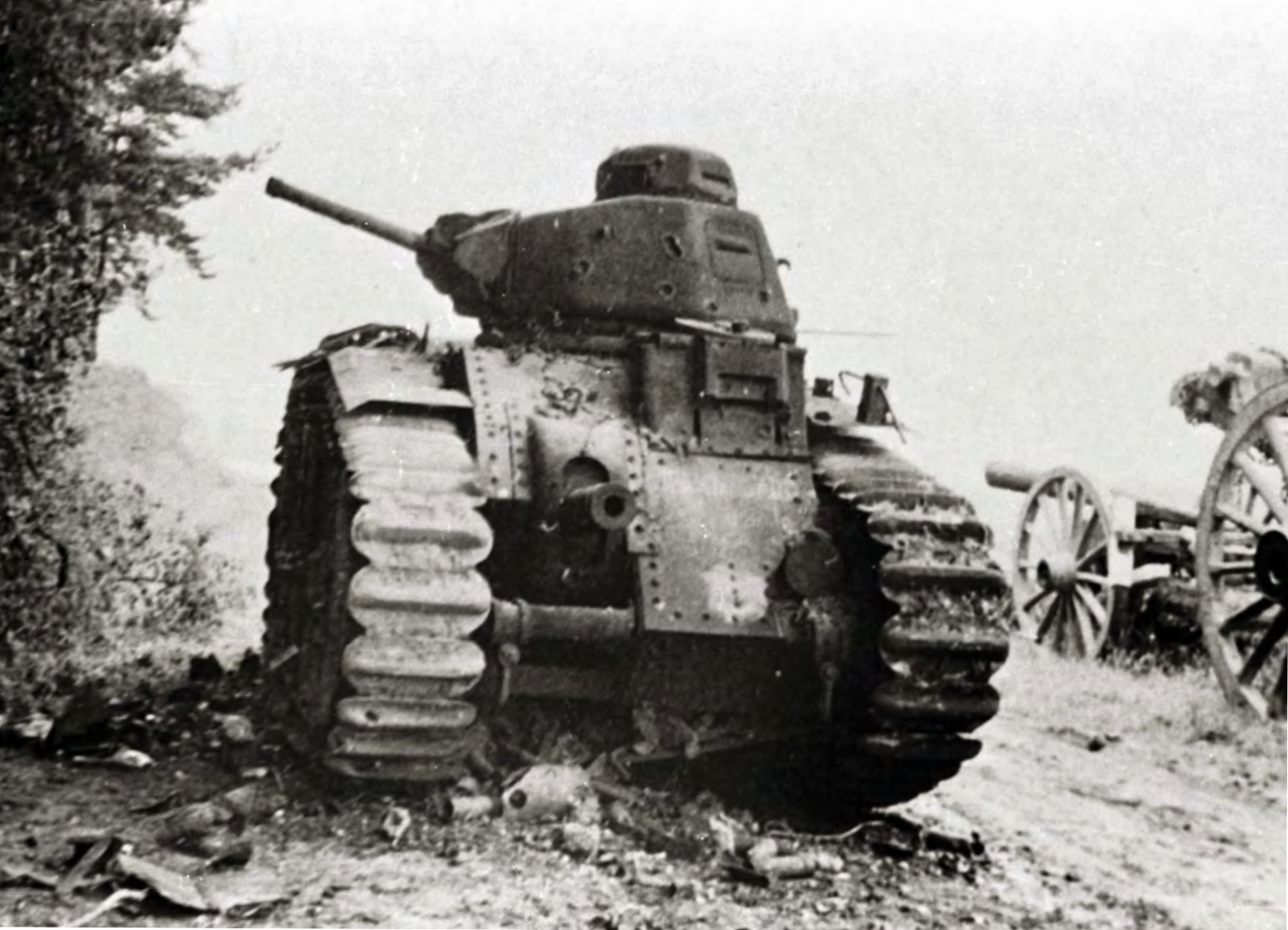
The Char B1 bis was a powerful French tank but it came to grief just the same. Its 60mm frontal armour was twice as thick as a British cruiser and it weighed 31 tons. An excellent tank by 1940 standards it was let down by having a one-man turret, which here has been struck a number of times. [Tank Museum 1323 E2 1]
