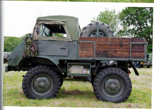
Above and left: The Unimog model number U411-10 proved useful to the Swiss Army for work in mountainous regions to tow heavy trailers and act as an alpine gun tractor. They can pull loads up to around 2 tonnes. Current owner Daniel Craig has had it for around four years.
