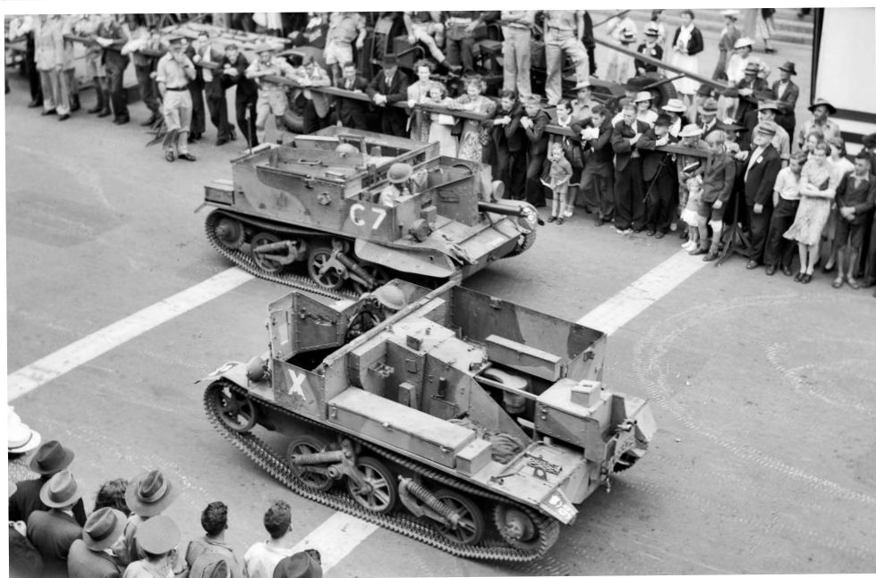
Here the Scout Carrier passes a Universal while providing an excellent view of its internal layout. (Australian War Memorial)
