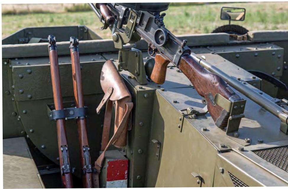
Unlike the Bren Carrier, the Scout was intended as a fighting vehicle and so was equipped with a pintle-mounted Bren in addition to a Boys anti-tank rifle.
