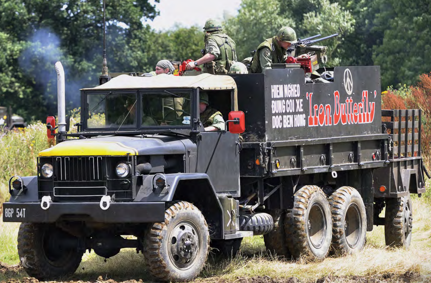
Iron Butterfly, belonging to Colin Topliss, was Rolling Thunder's first replica gun truck – it's a second generation model with double skin armour built on a M35 A2 6x6 cargo (2.5 ton) truck.
