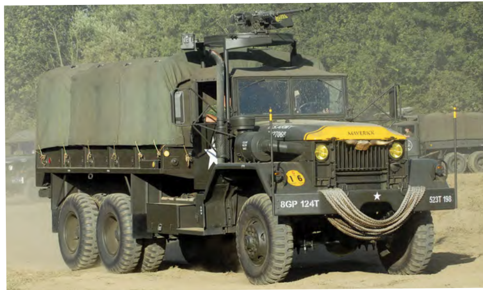
Above left: This M54 A2 6x6 cargo truck (5-ton) named Maverick is fitted with a gun ring and .50 calibre heavy machine gun. It was used mainly for the movement of cargo but also as prime mover for the 155mm Howitzer. It's owned by Stuart Beeney. Above right: Peter Frost, our resident peace protester, can cover any period of the anti-war movement from the early days with suit and tie to full on hippie. Pete brings colour to the display, and serves as a reminder of a very much forgotten aspect of the Vietnam conflict.
