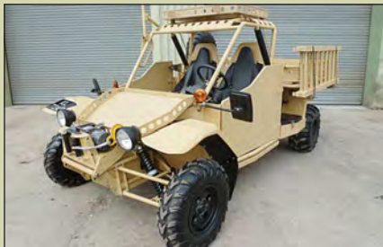
EPS Springer ATV LHD , 1.1 ton payload, 2 seater left hand drive configuration, 4x2, fitted Lombardini 1.4 litre diesel engine and 2 speed forward and 2 reverse CVT, 1.4 litre Lombardini diesel engine, etc, Year 2009, Mileage from 100 kms, Excellent Condition, Guide price from £7,500 (5 Available)
