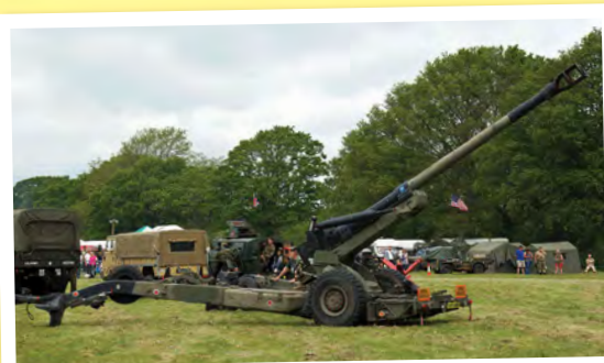
Above and right: The 155mm SP gun was used by NATO forces during the seventies; the gun section is driven by a dedicated Mk1 VW Golf engine so it doesn't need to be towed by tractor to its place of deployment. Below: This variant of the 1939 Morris Commercial CS8 truck, belonging to Bob Edgeley, was used by the Signals as a wireless truck. This unit saw service with the 2nd Army and continued into post-war service again with the Signals units. The vehicle is still original and at present has no specific unit markings applied.
