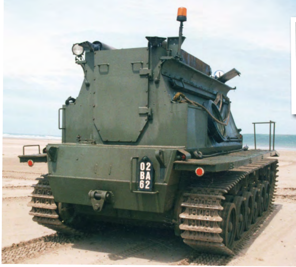
Above: The prevention of water ingress was key to the success of the BARV and a curved coaming was fitted around the top of the superstructure to prevent water washing over on to the roof. Left: The large door in the rear of the superstructure is normally sealed, but can be unbolted to facilitate an engine or gearbox change. Routine maintenance can normally be undertaken from inside the vehicle.
