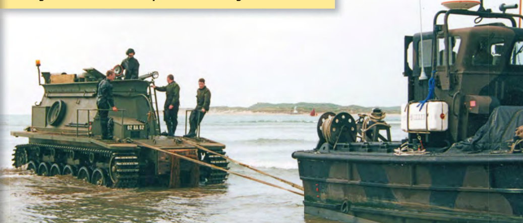
Below: BARV 02 BA 62 takes up the strain as it prepares to pull a landing craft off the beach as part of the training exercise.
