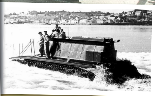
Above: The prototype Centurion BARV underwent trials at Instow, but the construction method was quite different to production vehicles, being riveted plate over a girder frame rather than welded armoured plate. Left: The Centurion BARV took over the role first performed during WW2 by the Sherman BARV and the similarities in the design are clear to see.
