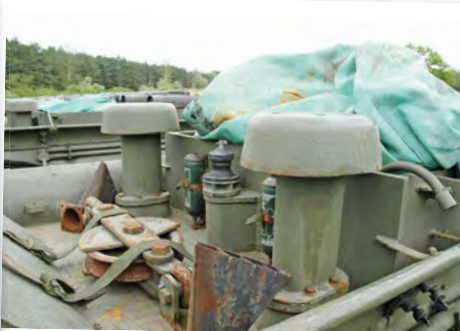
Above left: Looking down into the interior we see the air filter units in grey and the door through into the engine compartment. Above right: To the rear of the commander's cupola are the two raised air intakes with an aerial mount between them. The fishtail exhaust outlets aren't normally there, having been removed from the exhaust silencers at the rear.
