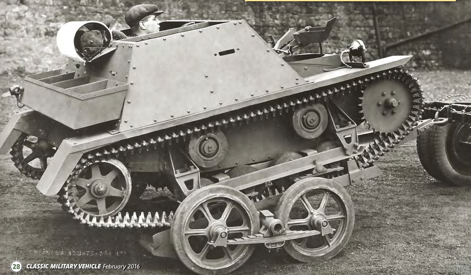
Below: At the other end of the scale the Vickers-Carden-Lloyd transporter carrying a Carden-Lloyd Mark VIA which could be towed by more or less anything, but note again it has no brakes.
