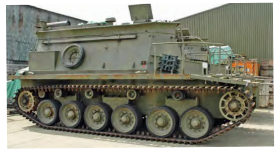
Above: The prevention of water ingress was key to the success of the BARV and a curved coaming was fitted around the top of the superstructure to prevent water washing over on to the roof. Left: The large door in the rear of the superstructure is normally sealed, but can be unbolted to facilitate an engine or gearbox change. Routine maintenance can normally be undertaken from inside the vehicle.
