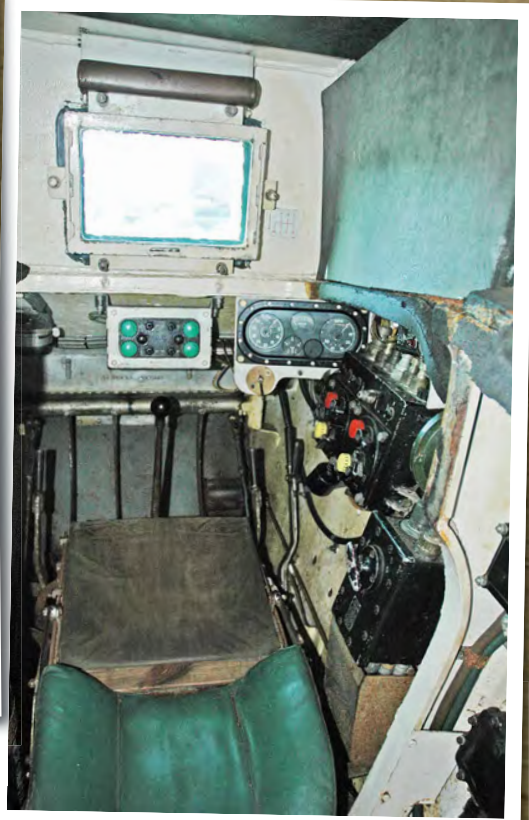
Above: The interior is surprisingly roomy with the turret basket removed and the increase in height with the new superstructure. Right: Driver controls are pretty much as per the standard Centurion gun tank, but vision is limited to the one small glass panel and directions from the vehicle commander via the intercom system.
