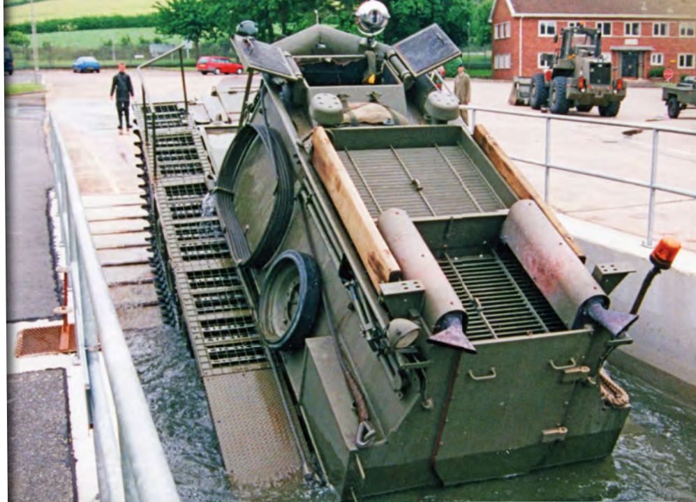
Above: Another view of the Centurion BARV in the dip tank, which coincidentally shows the normal depth at which it can operate in the sea. The open mesh walkways allow the free movement of water and reduce unwanted buoyancy when entering the water. Above right: Salt water can play havoc with the BARV so the vehicles are washed off in a dip tank (shown here) to remove the potentially corrosive salt water. This view offers a good look at the layout of the roof area on the BARV, including the open commander's cupola at the front.
