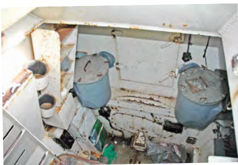
Above left: Looking down into the interior we see the air filter units in grey and the door through into the engine compartment. Above right: To the rear of the commander's cupola are the two raised air intakes with an aerial mount between them. The fishtail exhaust outlets aren't normally there, having been removed from the exhaust silencers at the rear.
