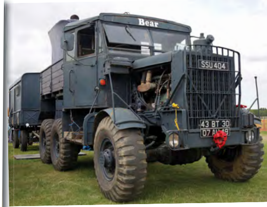
This Scammell Explorer, built in 1955, originally saw service with the RAF before being transferred to the Army where it served with the TA in Glasgow, before its final decommissioning in 1970. It is powered by a Meadows 10.6-litre petrol engine and is owned by Neil Turner who has had it since 2008.
