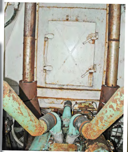
Above: Viewed from the engine compartment we see the massive Meteor petrol engine and the twin exhaust stacks running up to the rooftop. Left: A spare armoured glass vision block is carried inside the vehicle.
