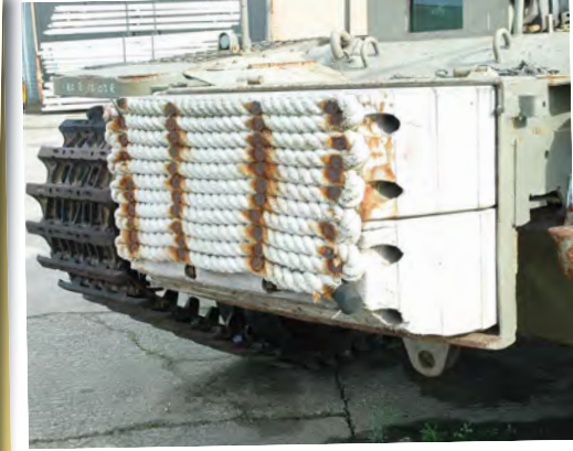
Above left: A drop down access ladder is provided at the rear of the track guard. Middle: Everything has to be exceptionally well sealed against the ingress of water, including the fuel filler at the rear of the vehicle shown here. Above right: A large wooden pushing block was mounted at the front of the vehicle, which was sometimes covered in rope (as shown here) or latterly in plastic blocks.
