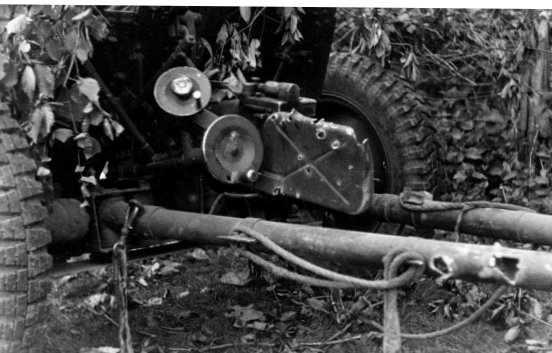
The gun shield only offered protection to fire from the front. Note the gunner's handwheels. The upper wheel, with the firing button in its centre, controls the barrel's elevation; the lower wheel controls the traverse. The shrapnel-perforated guard protects the gunner from the barrel's recoil.
