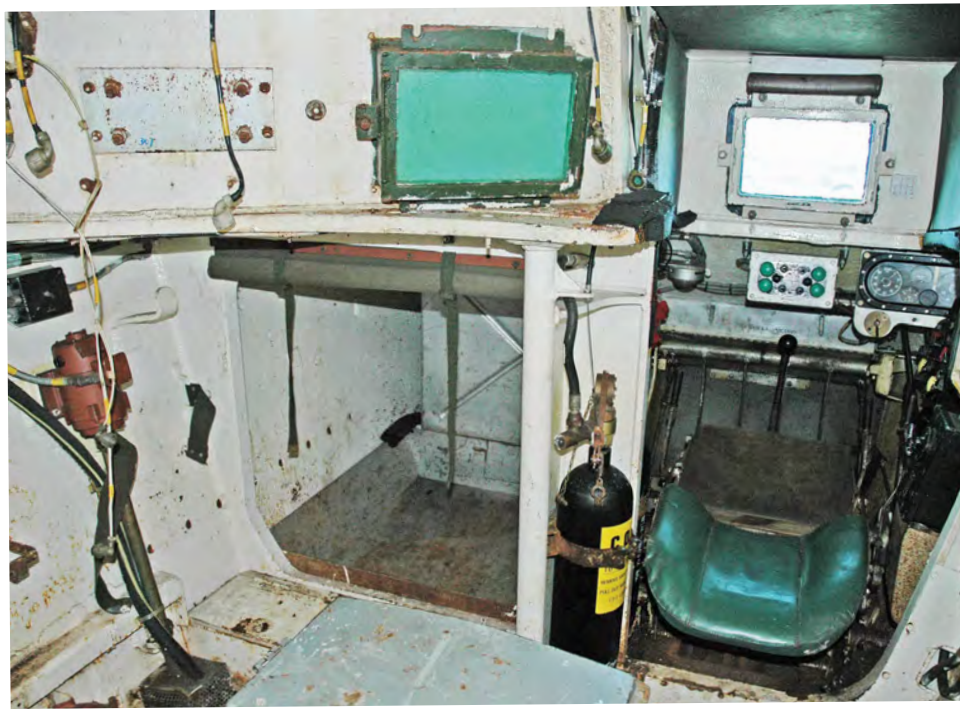
Above: The interior is surprisingly roomy with the turret basket removed and the increase in height with the new superstructure. Right: Driver controls are pretty much as per the standard Centurion gun tank, but vision is limited to the one small glass panel and directions from the vehicle commander via the intercom system.
