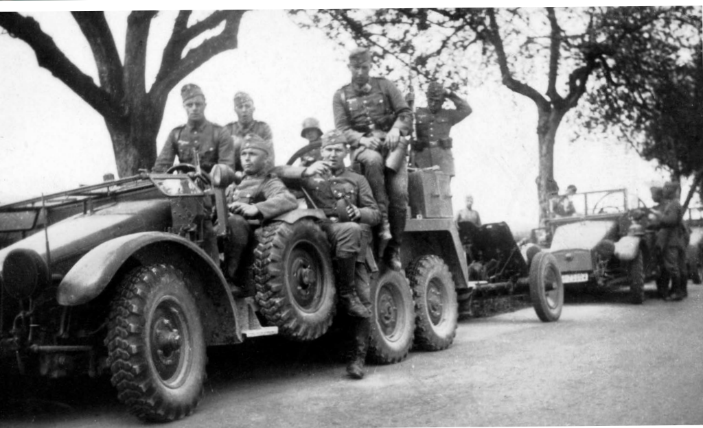
An anti-tank platoon rests by the roadside, almost certainly on pre-war manoeuvres. (The steel helmet worn by the soldier in the rear of the lead vehicle is the model issued during the Great War, which would be replaced by the lighter Model 1935 helmet prior to the outbreak of war in 1939.) The gun tractors are the Krupp L 2 H 43, known informally as the Krupp-Protze. The flat-four air-cooled engine allows the bonnet to taper sharply downwards to the front, giving the driver good visibility of the terrain ahead.
