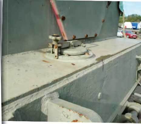
Above left: A drop down access ladder is provided at the rear of the track guard. Middle: Everything has to be exceptionally well sealed against the ingress of water, including the fuel filler at the rear of the vehicle shown here. Above right: A large wooden pushing block was mounted at the front of the vehicle, which was sometimes covered in rope (as shown here) or latterly in plastic blocks.
