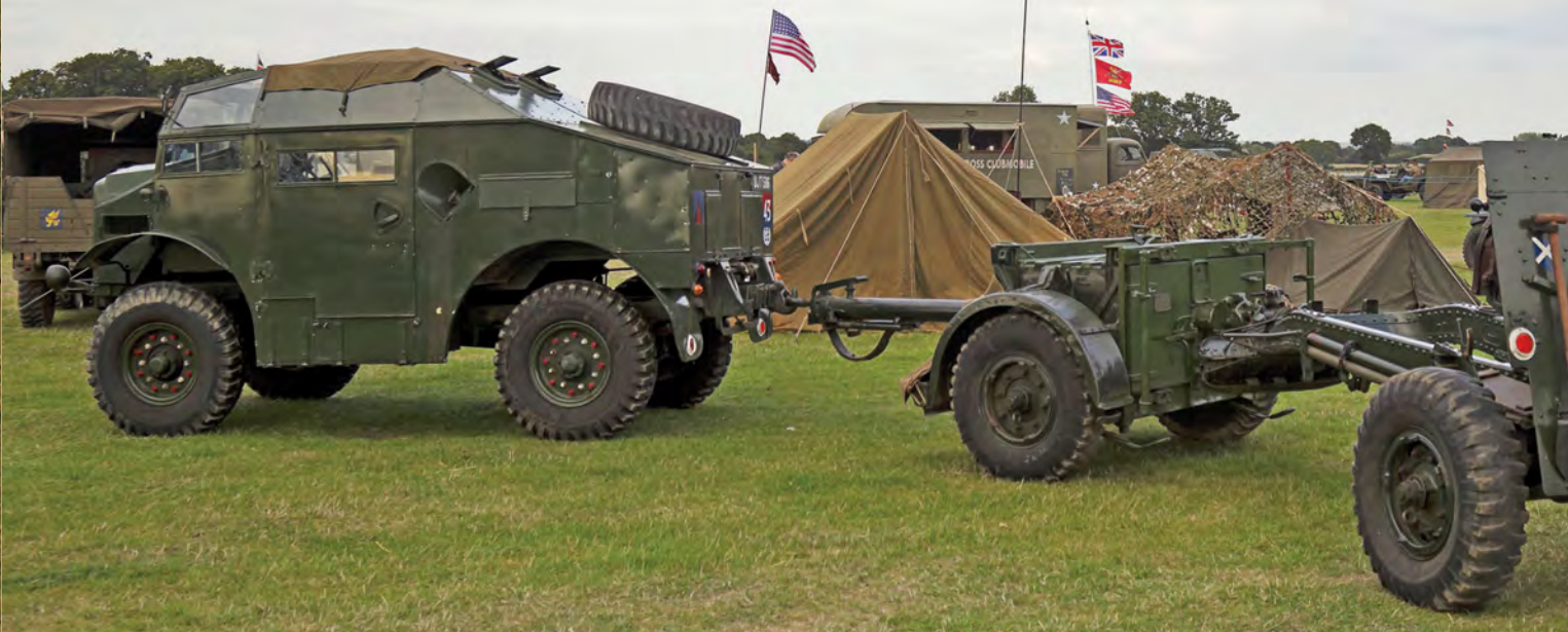
Above and below: The C8 MKII field artillery tractor is based on the Morris Commercial and has been extensively restored since leaving service with the British Army. The 25 pound field gun is an Ordnance QF Mk2 on a Mk1 carriage. The gun is in RA colours and is of the 1938-1960 pattern. Current owner is Andy Thomas who's had it since 2014 and it forms part of the FRS collection.
