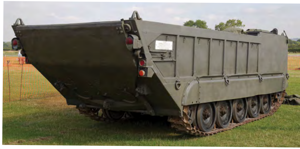
This M762 mobile missile launcher served with the British Army and was operational as a launcher for the Lance missile delivery system. Built in the US during the 1970s they were deployed in Germany and in the UK and were built on the iconic M133 chassis. Currently owned by a film prop company it is under restoration assessment by Mick Wilson.
