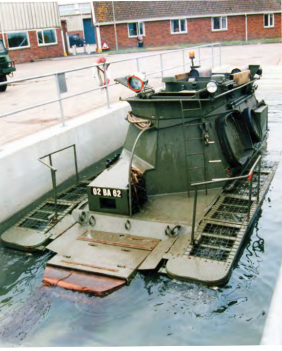
Above: Another view of the Centurion BARV in the dip tank, which coincidentally shows the normal depth at which it can operate in the sea. The open mesh walkways allow the free movement of water and reduce unwanted buoyancy when entering the water. Above right: Salt water can play havoc with the BARV so the vehicles are washed off in a dip tank (shown here) to remove the potentially corrosive salt water. This view offers a good look at the layout of the roof area on the BARV, including the open commander's cupola at the front.
