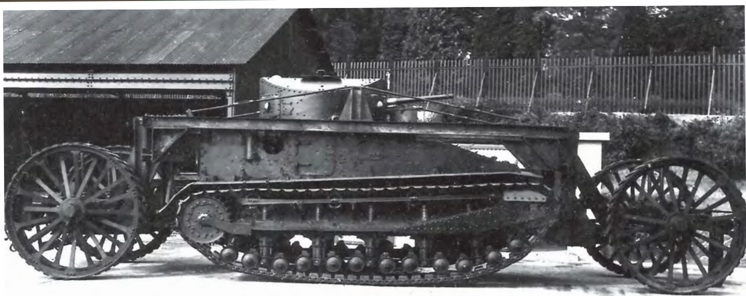
The Southern Command transporter carrying a Medium Mark I tank with minimal ground clearance. What could have towed it?
