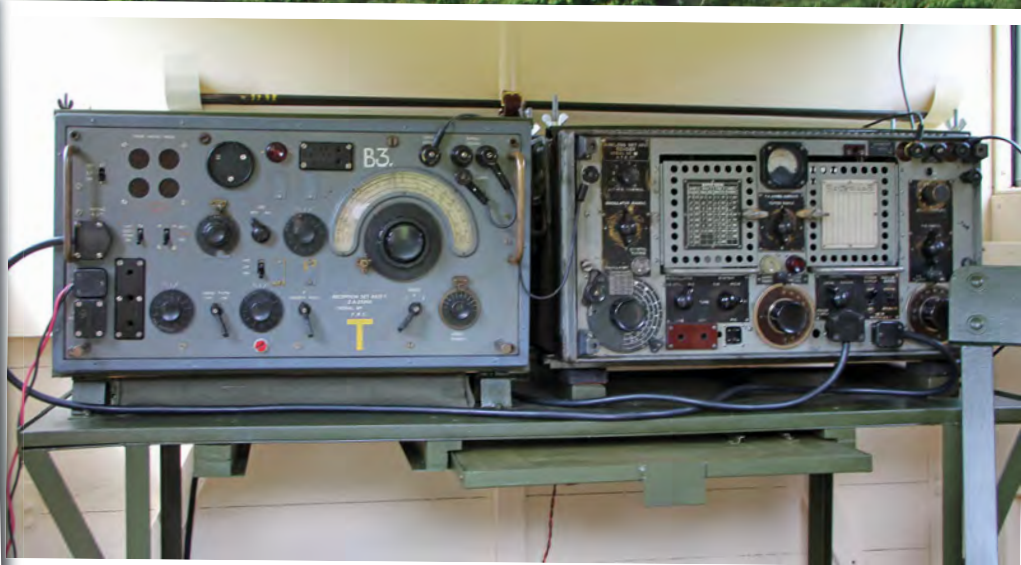
Above: Bob was unable to track down a wireless set Number 2, opting for the slightly later Number 12 set instead. Fortunately many of the original fittings, including the fixings for a ship's type speaking tube used for speaking to the driver, had survived. Left: Used as a Communications HQ the wireless truck would have been deployed behind the front line.
