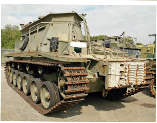
Above: Photographed at Witham, here we see the wooden nosing block used to push landing craft and vehicles off the beach. Right: Photographed in 2007, this was one of the vehicles that turned up at Witham Specialist Vehicles for disposal.
