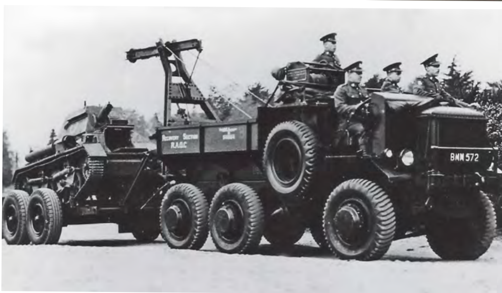
An AEC/FWD tractor of the RAOC pulling a four-wheel light recovery trailer with a Light Tank Mark IIB loaded up. This is a pre-war photo but this combination was used early in WW2 carrying Light Mark VIB tanks.
