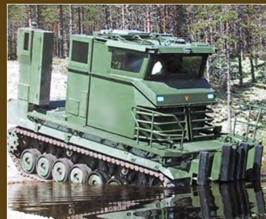
The successor to the Centurion BARV is the Leopard-based Hippo Beach Recovery Vehicle developed by Hägglunds Moelv.
