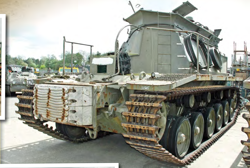
Above: Photographed at Witham, here we see the wooden nosing block used to push landing craft and vehicles off the beach. Right: Photographed in 2007, this was one of the vehicles that turned up at Witham Specialist Vehicles for disposal.
