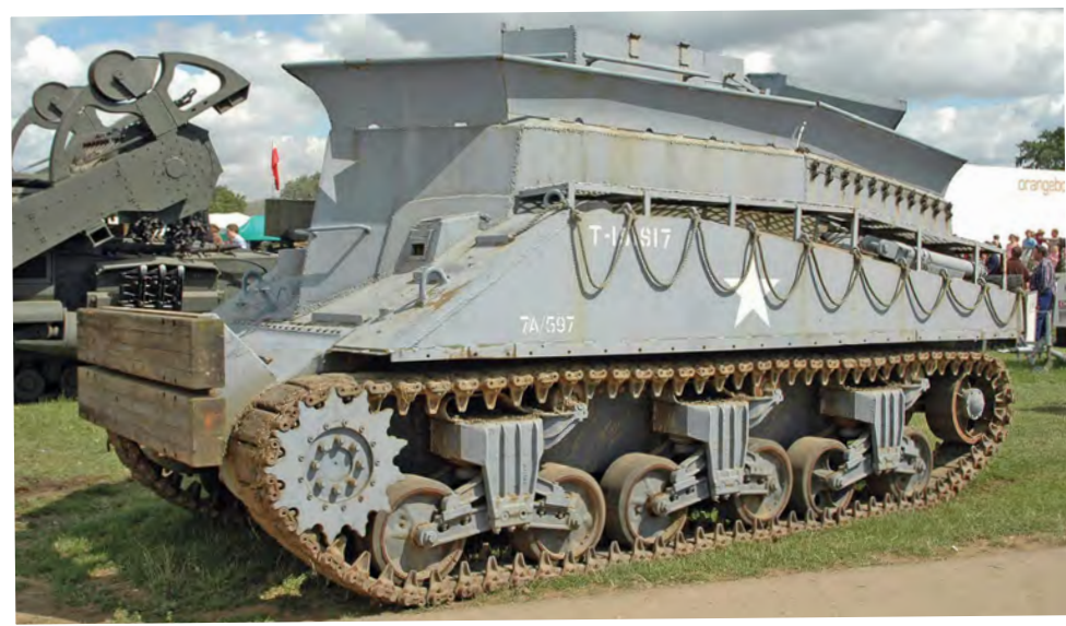
Above: Photographed at Witham, here we see the wooden nosing block used to push landing craft and vehicles off the beach. Right: Photographed in 2007, this was one of the vehicles that turned up at Witham Specialist Vehicles for disposal.
