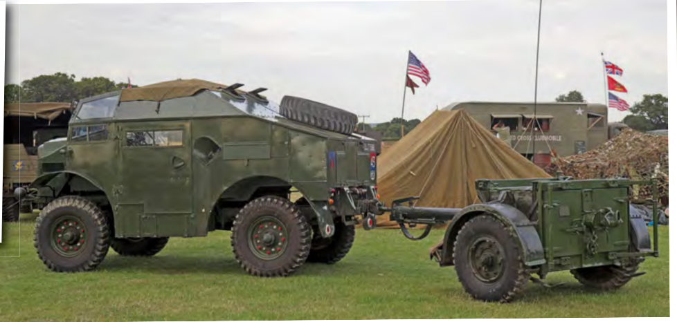
Above and below: The C8 MKII field artillery tractor is based on the Morris Commercial and has been extensively restored since leaving service with the British Army. The 25 pound field gun is an Ordnance QF Mk2 on a Mk1 carriage. The gun is in RA colours and is of the 1938-1960 pattern. Current owner is Andy Thomas who's had it since 2014 and it forms part of the FRS collection.
