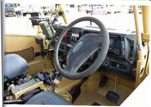
Much of the dashboard area will be familiar to anyone who drives a Defender but a great many more controls and switches have been added to the R-WMIK+.
