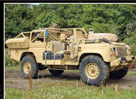
Like the WMIK, the 110 DPV underwent a number of upgrades and changes with this late version of the DPV looking not too dissimilar to the WMIK with the full length roll cage come gun mount.
