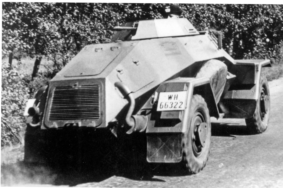
This is a Light Armoured Reconnaissance Car (Machinegun) (leichter Panzerspähwagen (MG) (Sd Kfz 221)) photographed from the rear. The exposed radiator grille shows this to be an early version; later versions had an armoured cover, open at the bottom, over the grille. The car is painted two-thirds dark grey/one-third dark brown. Fixed armament is a turret-mounted MG 34. A sub-machine gun also formed part of the car's equipment. The two crewmen were each armed with a pistol.
