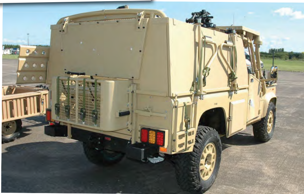
Rear three-quarter view of a brand new R-WMIK+ Land Rover fresh from stores that turned up at a Help For Heroes fundraising event near Worcester in 2011. The central armour panel raises up for better crew access.
