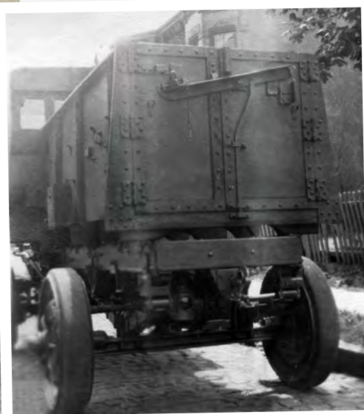
This shows how the differential is located above the rather spindly back axle. Running above the axle you can make out the half shafts which run to ring gears located within the rear wheels.
