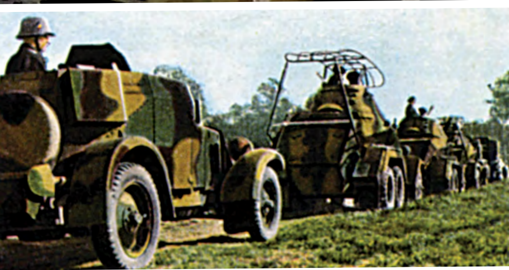
A Kfz 13 Machinegun Car (Maschinengewehrkraftwagen) brings up the rear of this armoured column. Based initially on the Adler Standard 6, it is a later version with the wheels of the Adler 12N 3G. In front of the Kfz 13 is a six-wheeled radio-equipped Sd Kfz 232 with its typical frame aerial. All of the vehicles are painted in the three-colour yellow/brown/green camouflage of the Reichsheer; this scheme remained in use until 1937 when two-thirds dark grey/one-third dark brown was adopted.
