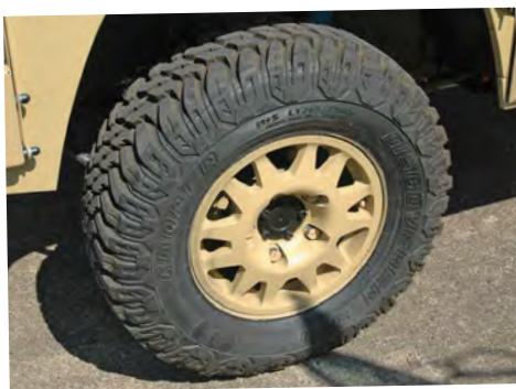
Later variants of the WMIK have seen the fitting of aluminium alloy wheels, initially as a 12-spoke design and latterly as a 15-spoke design, though these are the earlier variant.
