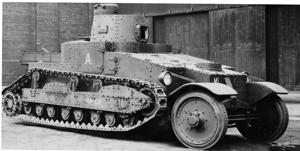
The wheel-cum-track armoured car D3E1 seen here posed on its wheels. Although it still survives the interior is a hollow shell.
