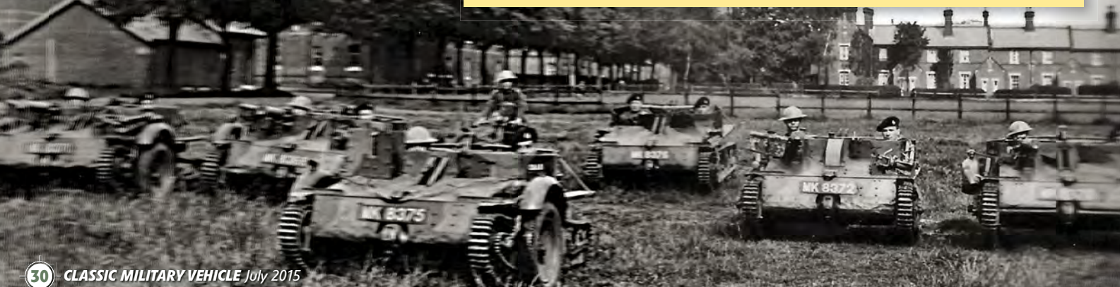
Below: The wheel-cum-track Carden-Loyd carriers, some with their wheels still in place but others without them. They were probably more trouble than they were worth.
