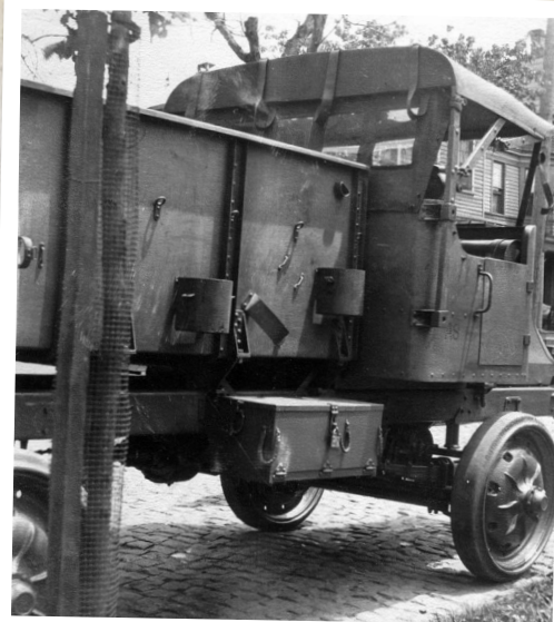
Above: Fitted with a steel ammunition body this Militor is to be used for carrying ammunition for heavy artillery. Drilled into the side of the cab can be seen the letters AS (Air Service) confirming that the cab had been taken from a Heavy Aviation truck which was primarily used by the Air Service.
