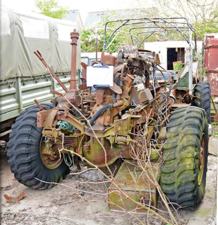
Above: Instantly recognisable as being AEC Matador related, this rolling chassis is actually from a Dorchester Armoured Command Vehicle making it a very rare beast indeed.
