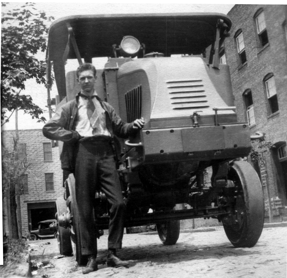
The bonnet of the Militor was copied from the Renault style. The fan located behind the radiator would draw air in through the numerous vents in the bonnet and blow it out into the cab which was good in cold weather and would have been not so pleasant when hot.
