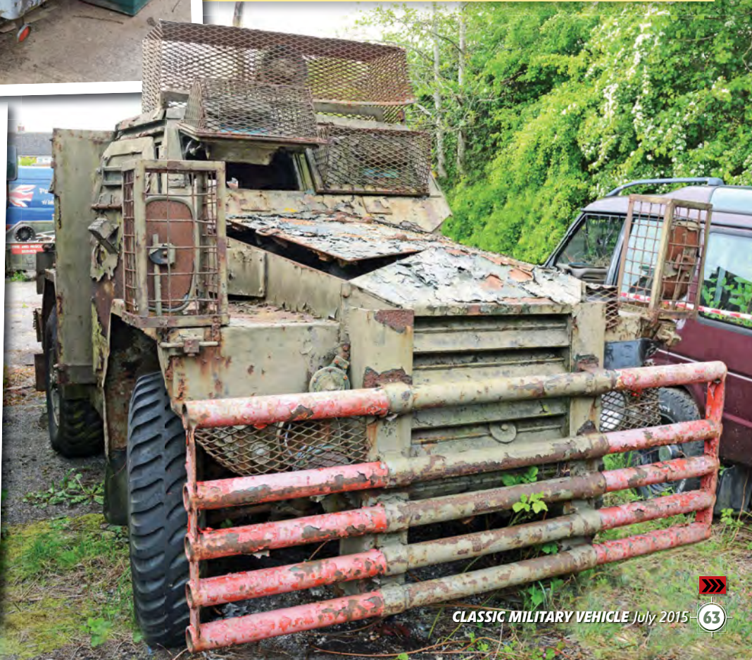
Below: Once common and often hated by enthusiasts, the Humber Pig is undoubtedly an imposing vehicle and one that I've always loved. In fact I've owned two of them! This example is a rare Flying Pig, although the side screens have been removed and the mesh guards are a late service addition.
