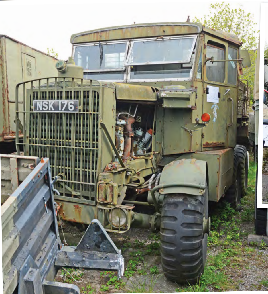
Above: Scammell Explorer with original Meadows petrol engine, which is very rare now with most having been swapped for less thirsty diesel units. Below: Despite Land Rovers being his bread and butter, Neil Mitchell had a particular penchant for wreckers and this Foden is one of the more recent additions to the collection.
