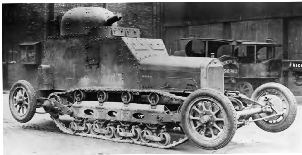
The mysterious Vickers-Wolseley wheel-cum-track armoured car also photographed at the Vickers factory and seen here standing on tracks.
