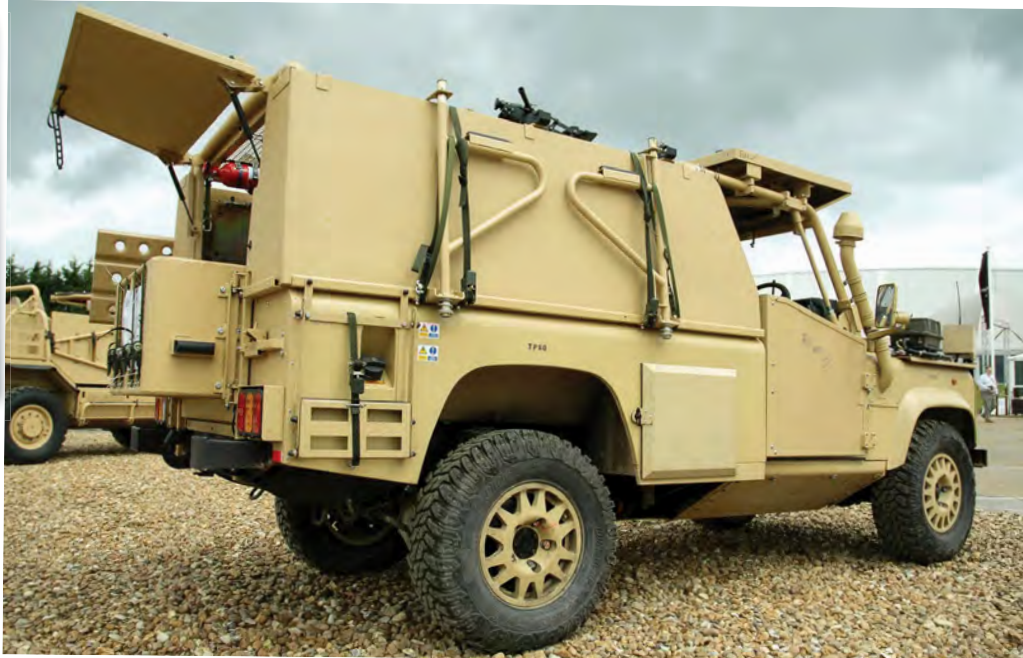
Rear three-quarter view of a production R-WMIK+ that was displayed at the Protected Mobility defence show in 2011. Note the raised rear armour panel.
