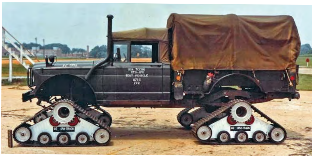
Above: In 1974 the Aberdeen Proving Ground tested an M715 fitted with a UNA-Track Kit consisting of four independent track assemblies which replaced the wheels on a one-for-one basis. It was hoped that it might prove useful in Alaska but it was found that power steering and other steering system modifications would be required and the idea was shelved.
