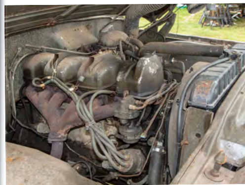
Above: It has been reported that the six-cylinder 3772cc Tornado powerplant was somewhat underpowered and unreliable, perhaps because of a lack of experience when it came to maintaining overhead camshaft engines. Left: Note the enormous hood-mounted Donaldson dry air cleaner. Below: The M715 retained much of the civilian Gladiator's cab panels but note how the front wheel arches have been radiused and lipped to accommodate military tyres. The cab roof and door tops were also removed and replaced by canvas.
