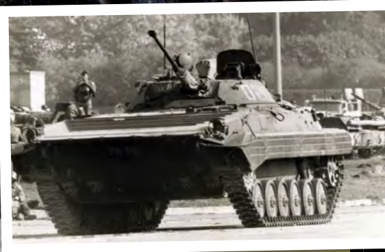
Above: The BMP-2 MICV was introduced during the war in Afghanistan. These later production vehicles feature upgraded turret armour and new polyurethane filled track guards, providing increased stability in water.
