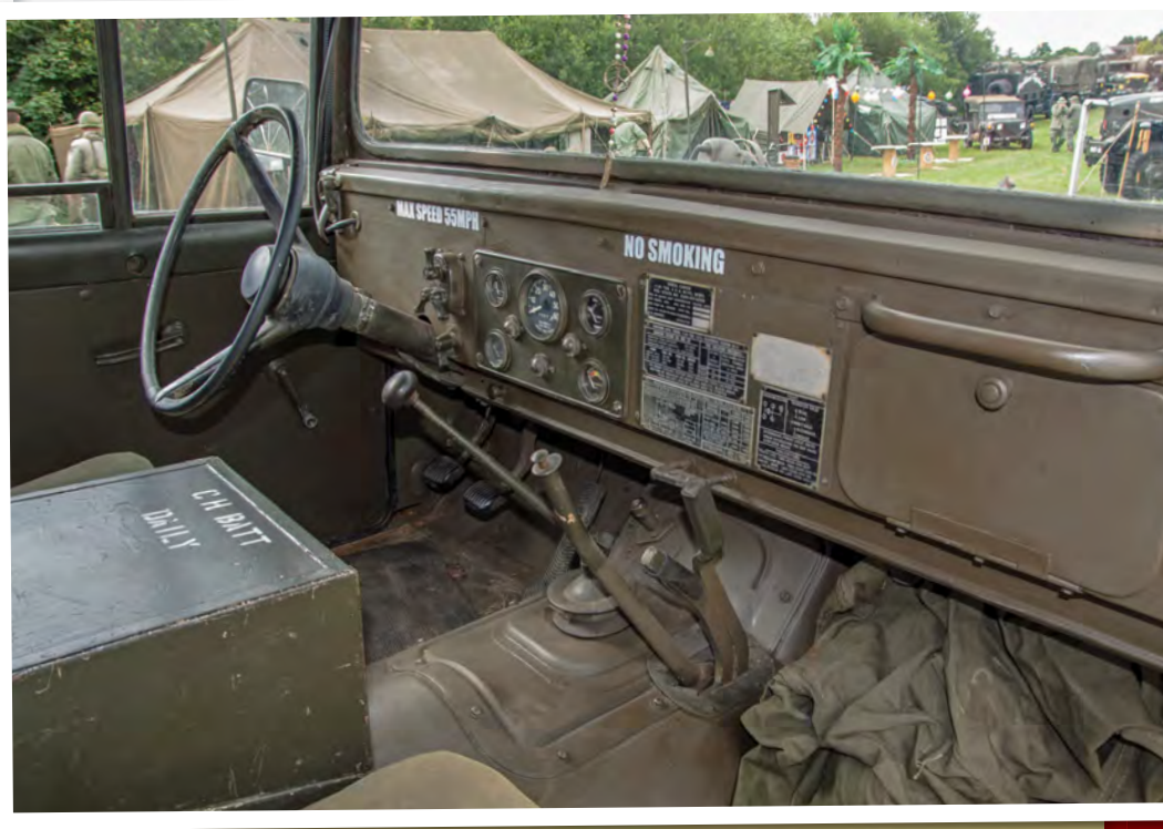
The M715's utilitarian cab interior. A large battery box sits between the two seats.
