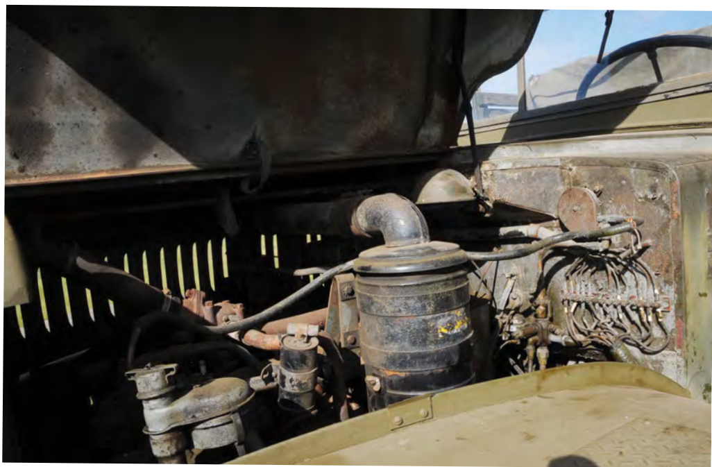
The 8676cc Hercules RXC delivers 106bhp and is virtually unburstable.
