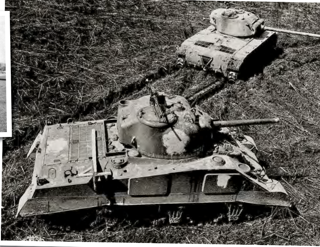
Right: The M4A3, powered by a Ford petrol engine, was probably the best of the series. It saw most wartime service with the US Army.
