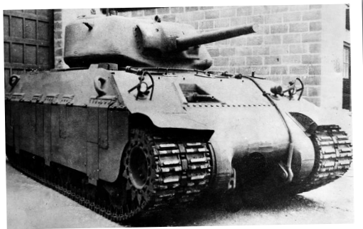
T14 was a Heavy Assault Tank, based on the Sherman which arrived in Britain for evaluation but was never adopted. The only survivor is still at Bovington.
