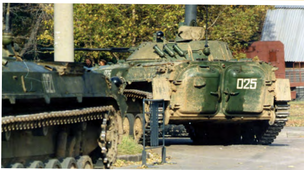
Above: The BMP-2 MICV was introduced during the war in Afghanistan. These later production vehicles feature upgraded turret armour and new polyurethane filled track guards, providing increased stability in water.
