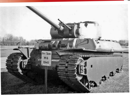
Above: The Heavy Tank M6, seen here in the mile of tanks at Fort Knox, was reckoned to be on a par with the Tiger but was regarded as a bit dated and never went overseas during the war.
