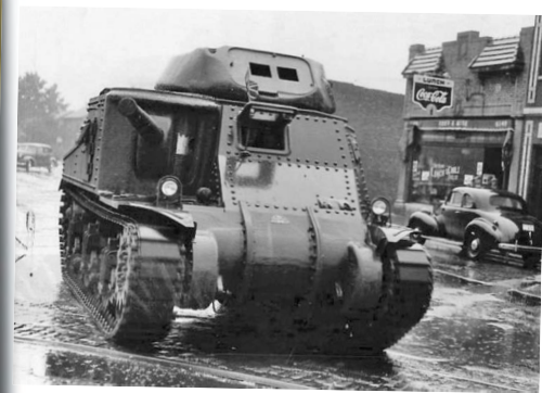
Above: The version of the M3 for British service was known as the Grant. Seen here on a test drive in the rain, before any turret guns were fitted.
