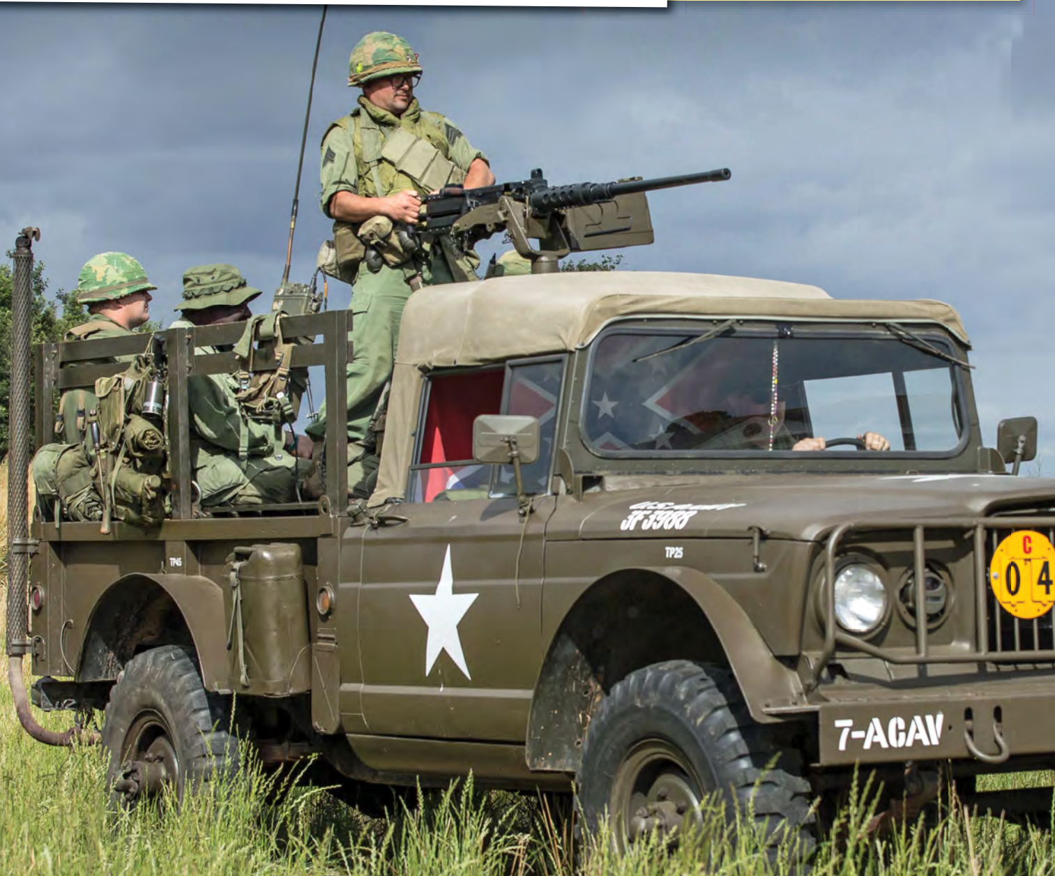
Above: It has been reported that the six-cylinder 3772cc Tornado powerplant was somewhat underpowered and unreliable, perhaps because of a lack of experience when it came to maintaining overhead camshaft engines. Left: Note the enormous hood-mounted Donaldson dry air cleaner. Below: The M715 retained much of the civilian Gladiator's cab panels but note how the front wheel arches have been radiused and lipped to accommodate military tyres. The cab roof and door tops were also removed and replaced by canvas.
