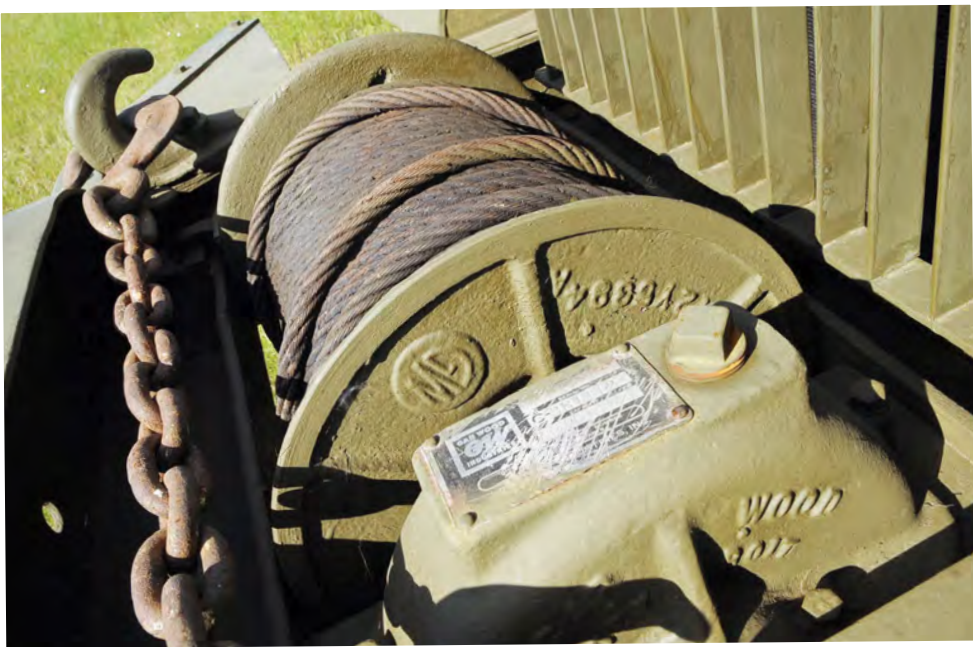
15,000lb (6818kg) capacity Gar Wood winch is mounted behind the front bumper.
