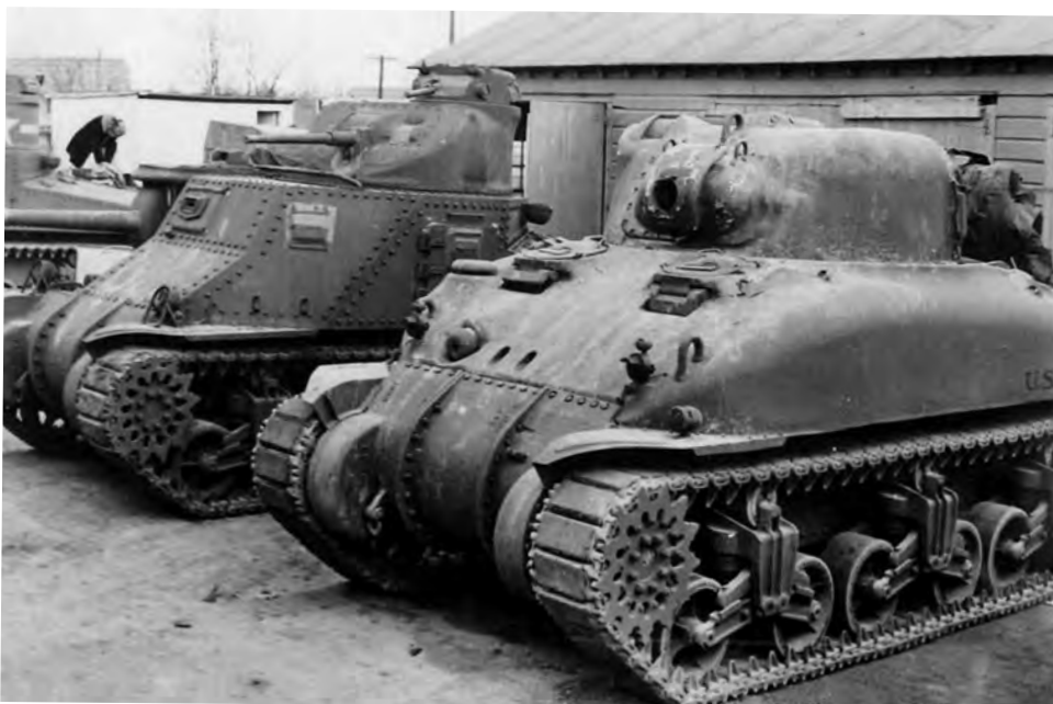
An early M4A1 alongside an M3 Lee. Notice the early pattern suspension.
