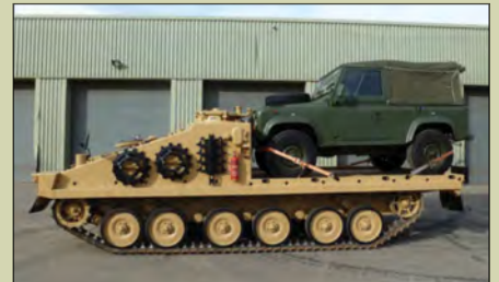
Alvis CVRT Shielder , Tracked Armoured load carrier with flat bed platform. The flat bed can be adopted for a wide range of roles such as logistic carrier, bridge layer repair / recovery and towing. Built to a high specification the vehicle hull is composed of aluminium armour to protect the crew, etc. Mileage from 500, Excellent condition, Guide price from 12,500 (4 Available) .
