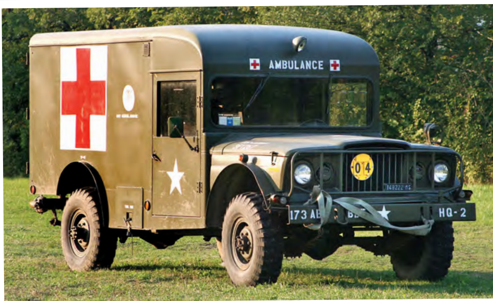
Above: The M725 ambulance featured a panel body containing four stretcher racks. (Photo courtesy Roberto Ferrari)
