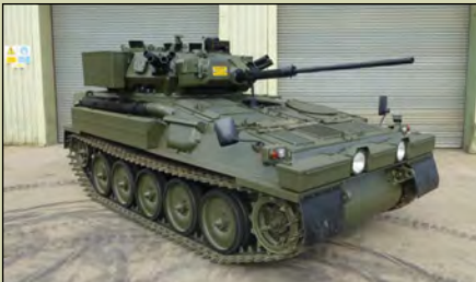
CVRT Scimitar Armoured Reconnaissance Vehicle , Fitted Cummins BTA 5.9lt Turbo diesel, Automatic Gearbox with Neutral turn capability, Maximum road speed 72 km/h, Range 750 km, etc, 820 miles, Excellent condition, Guide price £39,995 (1 Available)
