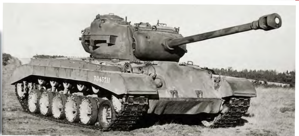
The M26, otherwise known as the Pershing, saw service with the US Army in Germany, and later in Korea. A few, like this one, were supplied to Britain but were never used. It was armed with a 90mm gun.
