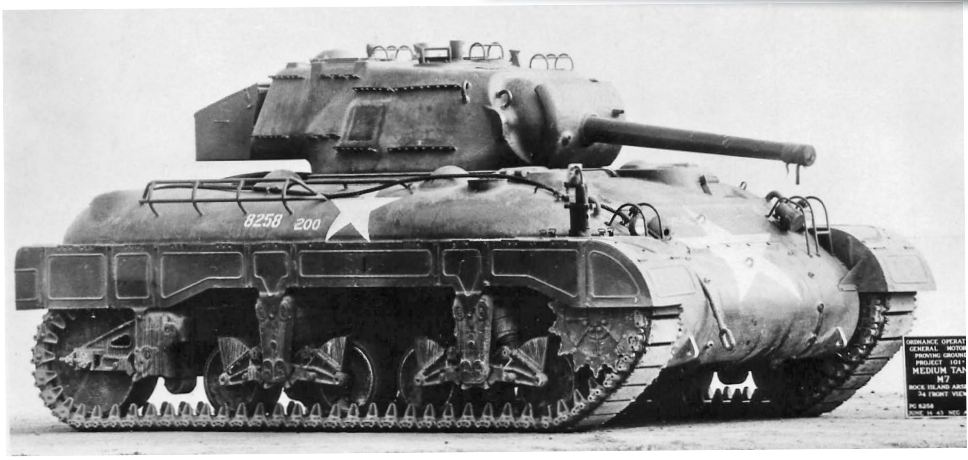
Below: The M7 as a Medium Tank, a rival to the Sherman. It was designed as a Light Tank and could have been a good one but it was an inadequate Medium.
