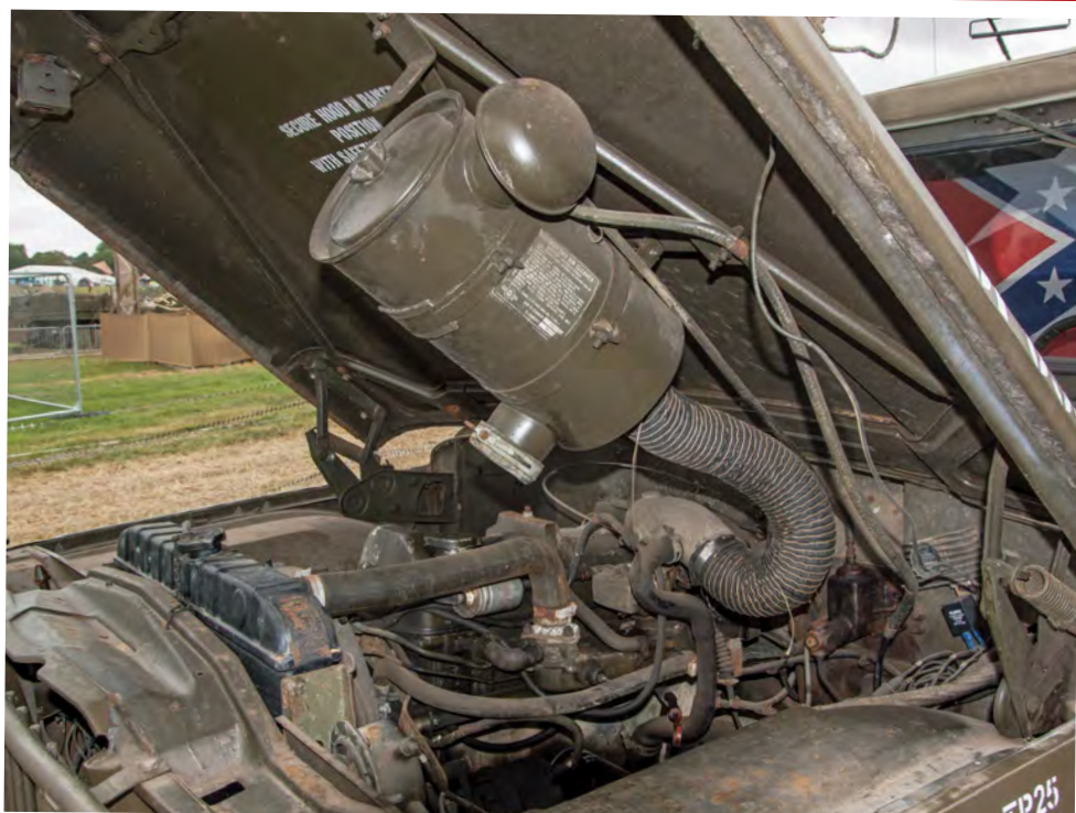
Above: It has been reported that the six-cylinder 3772cc Tornado powerplant was somewhat underpowered and unreliable, perhaps because of a lack of experience when it came to maintaining overhead camshaft engines. Left: Note the enormous hood-mounted Donaldson dry air cleaner. Below: The M715 retained much of the civilian Gladiator's cab panels but note how the front wheel arches have been radiused and lipped to accommodate military tyres. The cab roof and door tops were also removed and replaced by canvas.
