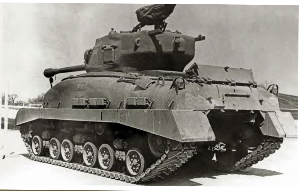
The combination of a long 76mm gun in the new turret with horizontal volute suspension, seen here on an M4A1, was the most up-to-date version of the Sherman to see service. That was towards the end of WW2.
