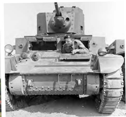
Left: An M2A4, the first American tank to be sent to Britain and only ever used for evaluation. Above: The M5A1 was the next in line, identified by the radio bustle on the back of the turret. The Stuart VI in British service as shown here.
