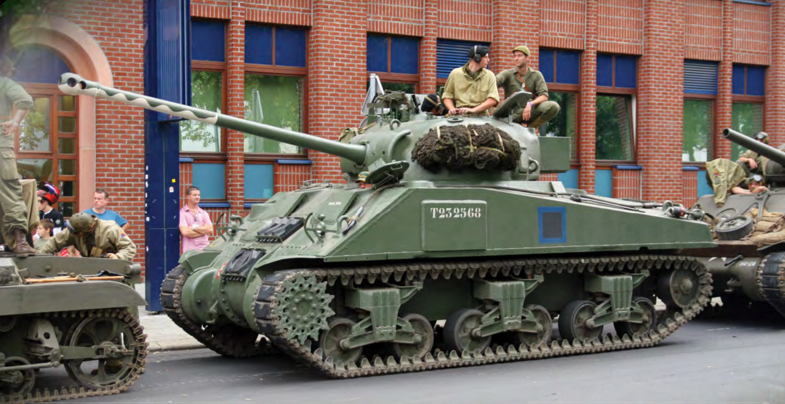
Relatively few Fireflies still exist in running condition. This example belongs to the Belgian Tank Museum and illustrates the disruptive pattern sometimes painted on the 17-pounder's barrel to disguise its length lest the extremely potent tank be singled out for attention by the enemy. (John Blackman)
