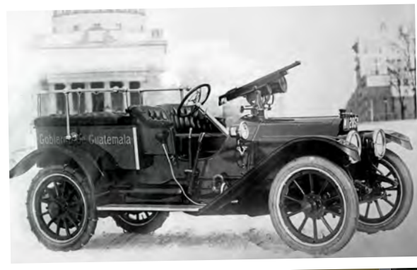
Above: Manufactured for the Guatemala police is this Type 55 Cadillac. Fitted to the scuttle of the car is an M1895 Colt-Browning machine gun and a searchlight. (Photo: US Library of Congress). Left: The two stars in the window signify that this Cadillac limousine is the property of a general. The passenger is fully enclosed against the weather but the driver has not been forgotten as he does have half side screens made from canvas.
