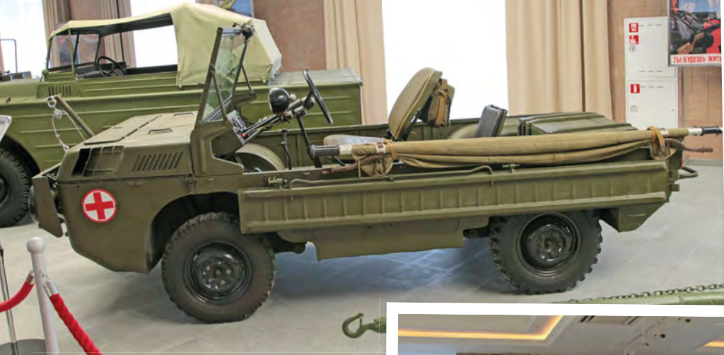
Above: The LuAZ-967M (TPK) amphibious battlefield evacuation vehicle. Above right: The museum has examples of the original Ford GPA amphibian and the Soviet MAV later developed from the American original, as seen here.
