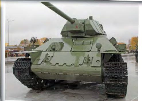
Above: A T-34 M-1941 with additional 'ekrani' armour plating on the hull and turret. Left: The museum has several T-34s in its collection, including this welded turret T-34 M-1941 complete with battle scars.
