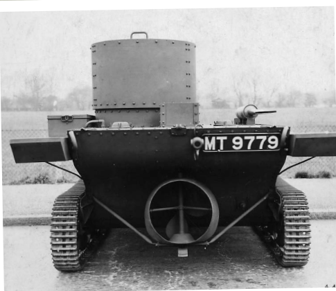
Above: This is a rear view of A4E11, one of the two Light Amphibians tested by the British Army. Note the cowled propeller used for steering which is normally referred to as a Cort nozzle. Left: Almost certainly A4E11 viewed from the side. These little tanks weighed less than 3 tons so they went fast on land and floated but they were hardly bullet proof.
