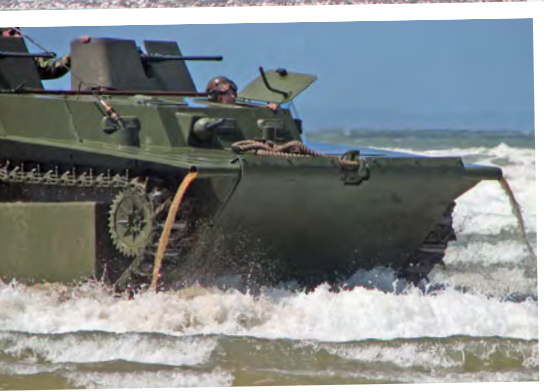
Above: With pumps running to drain the water the Buffalo drives out of the sea. Right: Buffalo at speed running in shallow water.
