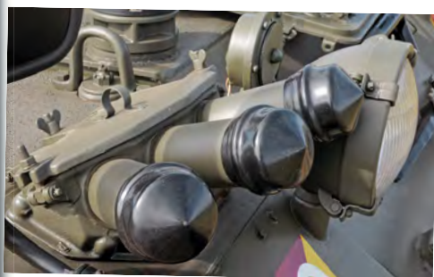
There are six smoke grenade launchers, three mounted each side over the front wheels.
