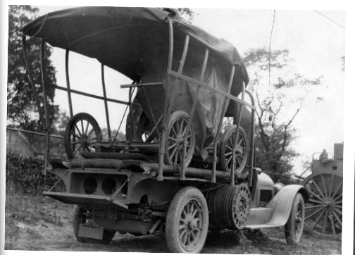
With the side screens folded up you can see how the searchlight fitted into the back of the Cadillac. The glass mirror would easily have been susceptible to damage and great effort has been taken to secure the searchlight into place. (Photo: US National Archives).
