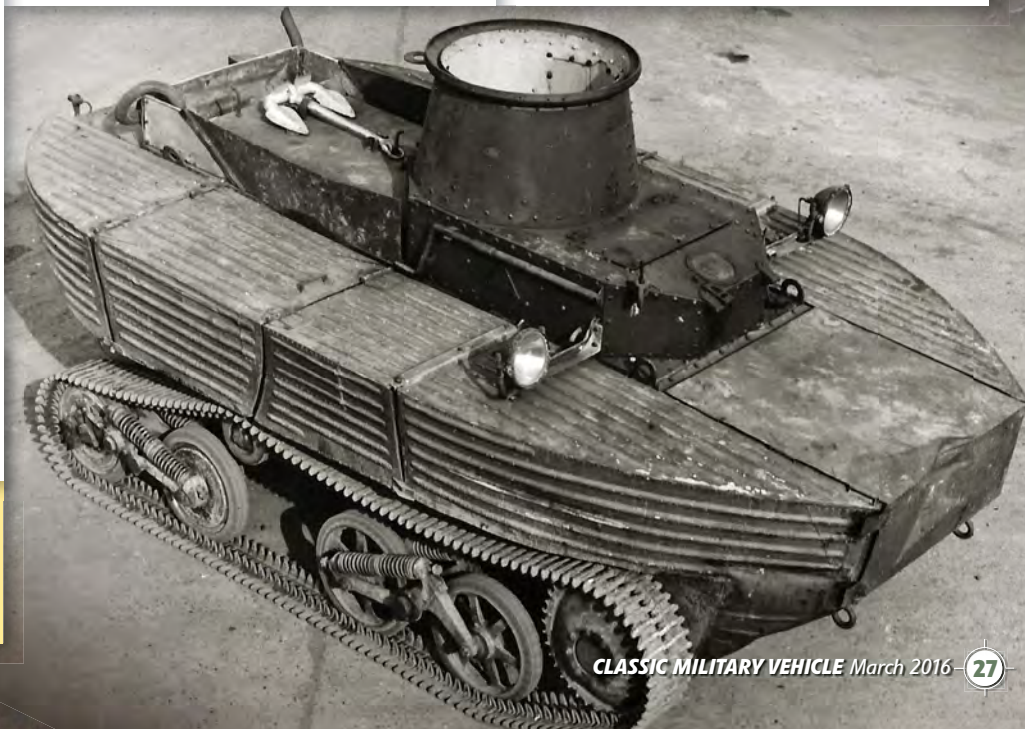
Right: L1E3 photographed later and as it is now, with spoked wheels on the front bogie and just the one return roller each side. The anchor on the aft deck is a nice nautical touch, but would you really need it?
