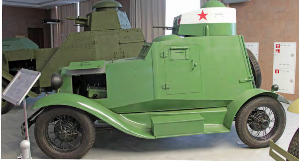
The FAI armoured car was based on the GAZ-A chassis. The colour scheme is from military manoeuvres conducted in the mid-1930s.
