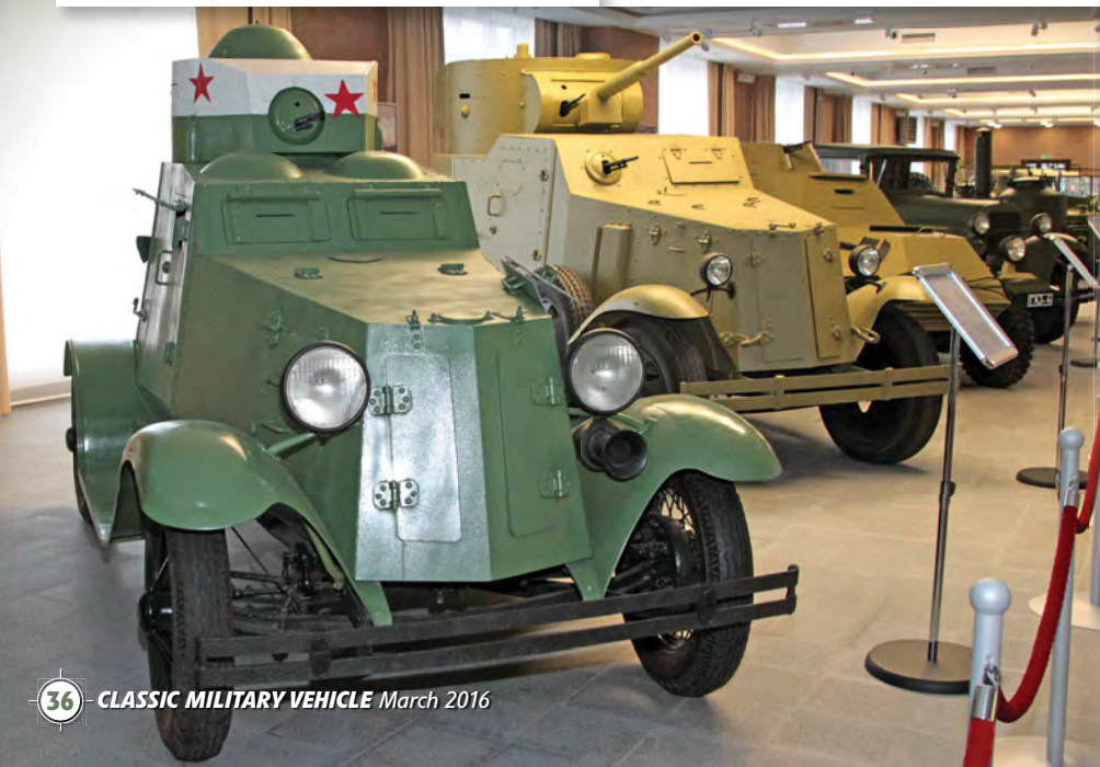
Above: A BA-27 armoured car, or a very good reproduction. The BA-27 was the Soviet Union's first series production armoured car, based on the AMO F-15 truck. Left: One of the curiosities of seeing Soviet light and medium armoured cars parked up together is that the latter are not as large compared to the former as expected from looking at wartime photographs.
