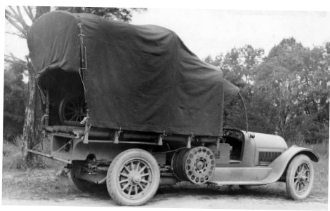
Above: The searchlight was powered by the engine of the Cadillac and the long power cable located on the drum by the rear wheel shows how far away from the Cadillac the searchlight could be located in case it came under fire. (Photo: US National Archives).
