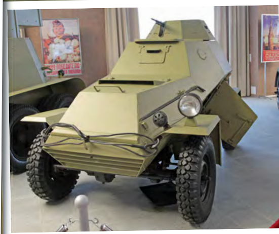
Above: The BA-64B armoured car was built at the Gorky Avtomobil Zavod. Early BA-64s were based on the GAZ-64 chassis, later BA-64B vehicles on the GAZ-67 chassis.
