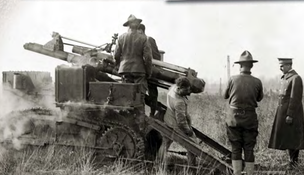
Below: The stabilisers on the back of the tractor have been deployed to prevent the tractor flipping over when fired. It does appear that the man standing to the rear has had a very near miss with the recoil. (Photo: US National Archives).
