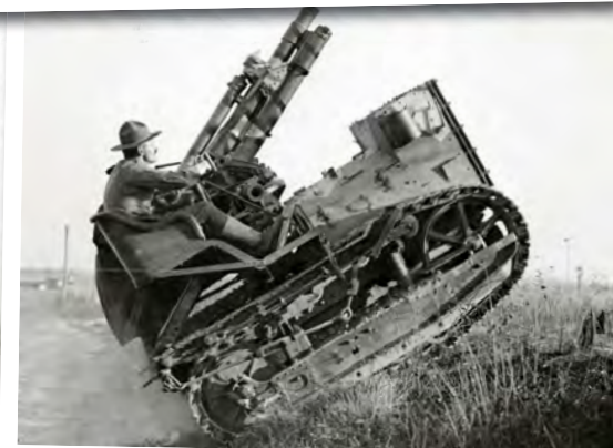
Above: During testing one of the 2.5 ton tractors was made to climb such a steep slope that it tumbled over backwards. I don't know if this photo is of that incident just before it happened, but the tractor certainly does not look very stable. (Photo: US National Archives).
