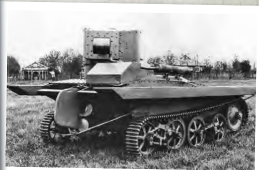
One of the first Vickers-Armstrongs amphibious light tanks photographed near Chertsey; note the large rudder.
