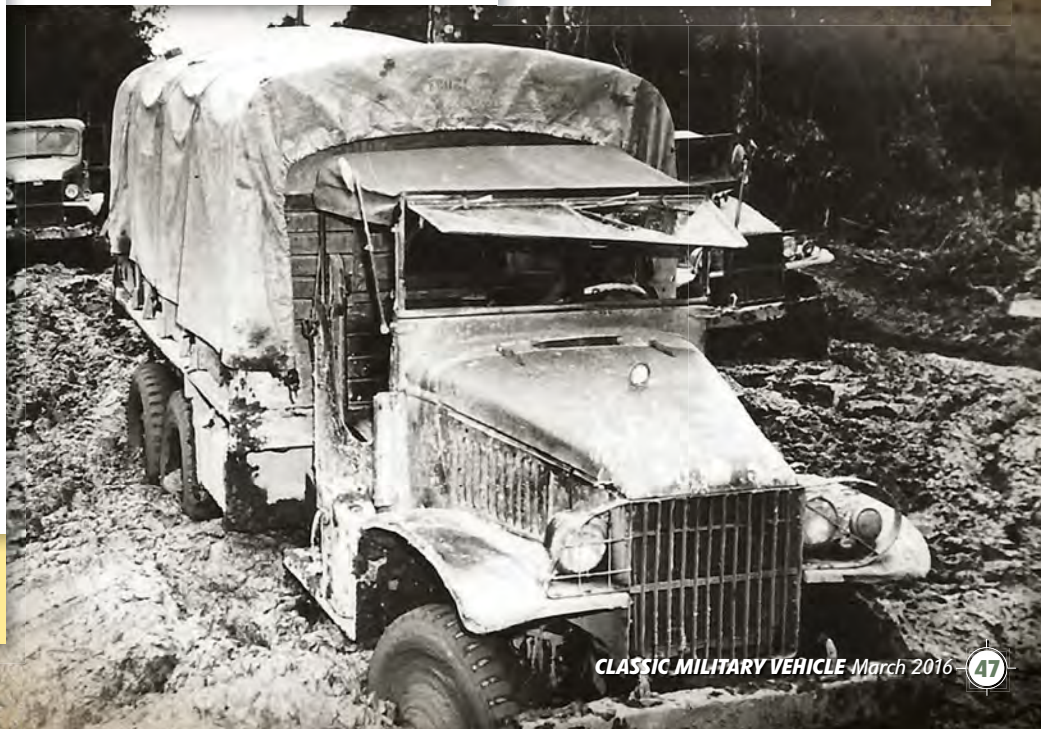
Right: GMC CCKW 353 bogged down on the Ledo Road turned into a quagmire (1880th Aviation Engineer Battalion).
