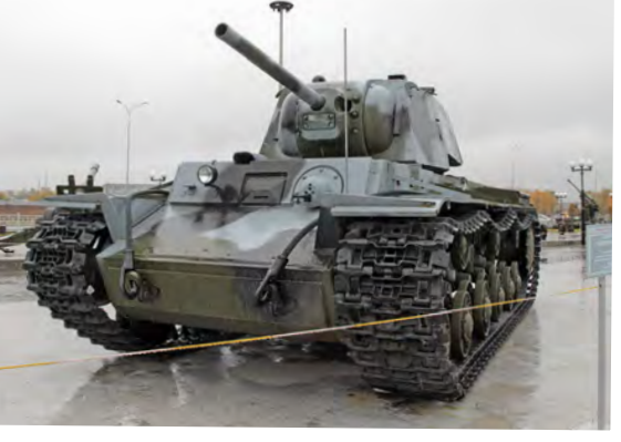
Above: An early welded turret KV-1 heavy tank. The tracks have suffered considerable small calibre shell damage. Right: A 2S7 203mm self-propelled gun flanked by MiG-25 and MiG-21 aircraft.
