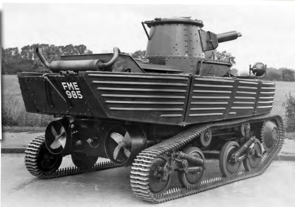
L1E3 when new, posed to show its two ducted propellers. The outer hull was really two pontoons, filled with kapok.
