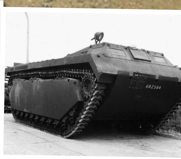
A partially armoured LVT III in British service, normally operated by the Royal Army Service Corps. This one mounts a spotlamp on top of the cab.
