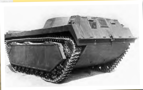
Above: The armoured version of the LVT-3 showing the frontal machine gun position, blanked off on this vehicle. The LVT-3C also had folding panels to cover the cargo space, although the extra weight reduced its effective carrying capacity.
