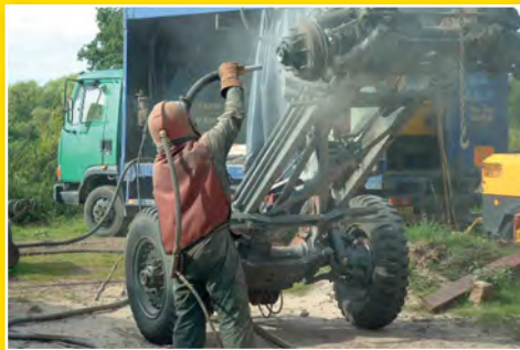
Described as the best £110 he has ever spent, shotblasting the chassis and cab meant that any bits of rust and dirt built up over the previous 50 years were blasted away.
