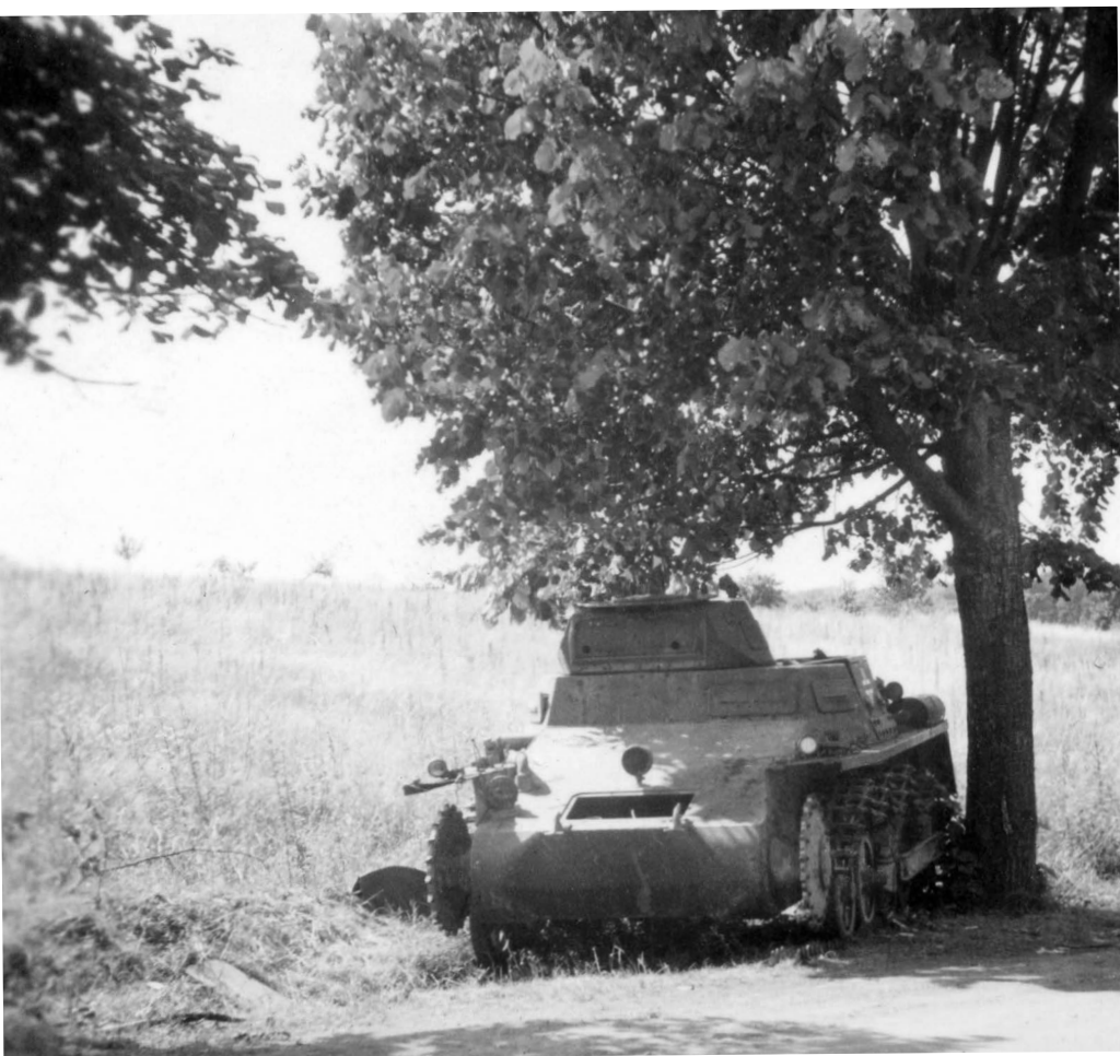
This PzKpfw I Ausf A has been knocked out on active service, but it is not known where. The white Balkan cross on the hull side with its centre painted out indicates either the campaign in the West in 1940 or, less likely, that in the East in 1941. The photograph clearly shows the hatch in the nose of the hull used by mechanics to service the steering brakes.
