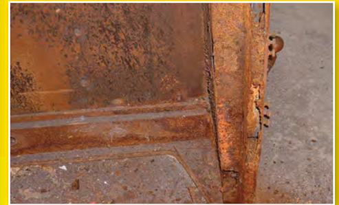
The vehicle was plagued by rust having spent its life outside when working in the recovery industry.
