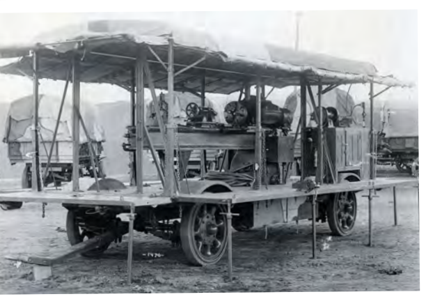
Above: The lathe is a vital tool in any workshop and this enormous one (probably manufactured by Lodge and Shipley) was the largest one that the HMORS were provided with.
