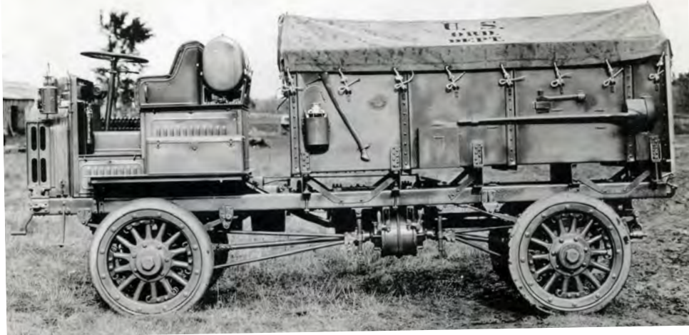
Above: With a top speed of 60mph (96km/h) the light repair truck was a relatively fast machine and was used to make emergency repairs to guns in situ. Below: The steel ammunition body was used for carrying a variety of different cargos in its narrow body. The steel sides were supposed to provide an element of protection for the cargo but this benefit was negated by the canvas top.
