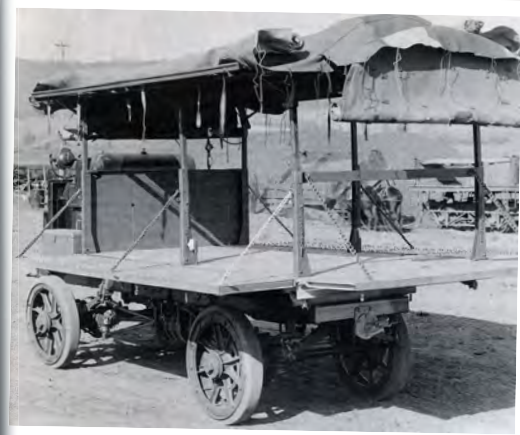
Above: Looking rather spartan is the FWD baggage truck. This would be used for carrying large bulky items of equipment used by the workshop such as tents.
