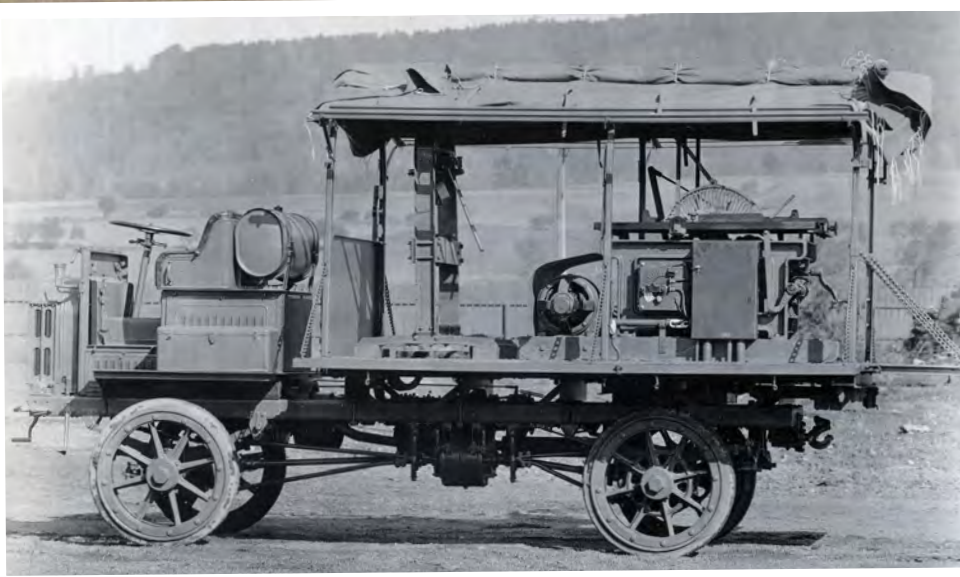
Equipped with a 24in circular saw this FWD was used for cutting through wood and would make short work of wooden beams up to 8in diameter. Also on the back of the trucks is a very heavy press.
