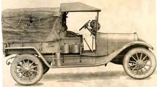
Above: With a top speed of 60mph (96km/h) the light repair truck was a relatively fast machine and was used to make emergency repairs to guns in situ. Below: The steel ammunition body was used for carrying a variety of different cargos in its narrow body. The steel sides were supposed to provide an element of protection for the cargo but this benefit was negated by the canvas top.
