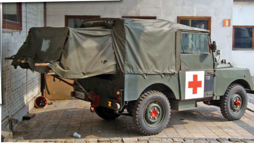
Above, left and below: Minerva in ambulance version, capable of transporting two juxtaposed stretchers.
