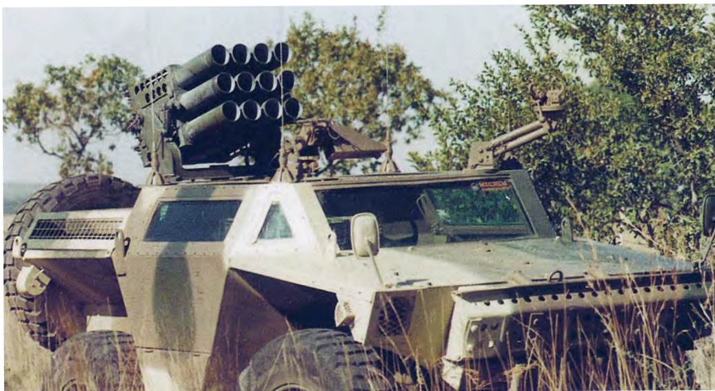
The Acorn could carry surprisingly large calibre support weapons such as this multi-barrel rocket artillery system.
