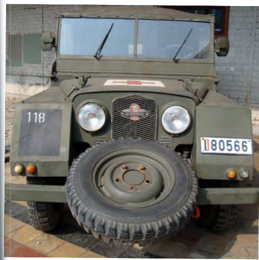
Above, left and below: Minerva in ambulance version, capable of transporting two juxtaposed stretchers.
