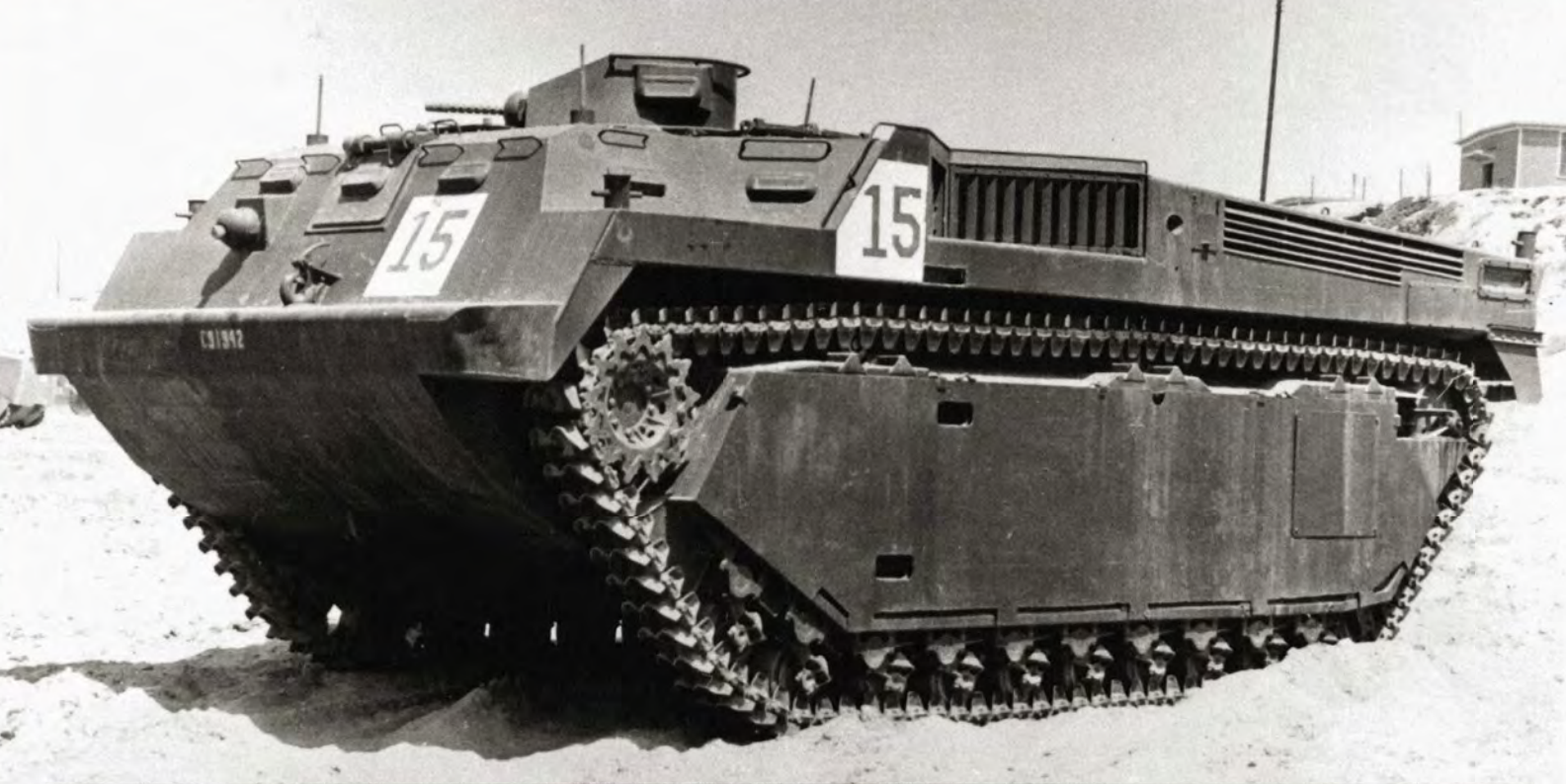
Above: A fully armed LVT-3C in service with US forces. Behind the engine air intakes are the ventilation louvres for the covered passenger compartment, but notice in particular the armoured crew cab at the front and the superimposed machine gun turret.
