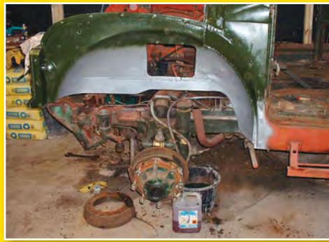
Above left: Shotblasting revealed where repairs were needed. Above right: Taking the gators off the hubs was certainly the hardest job which Tony faced.
