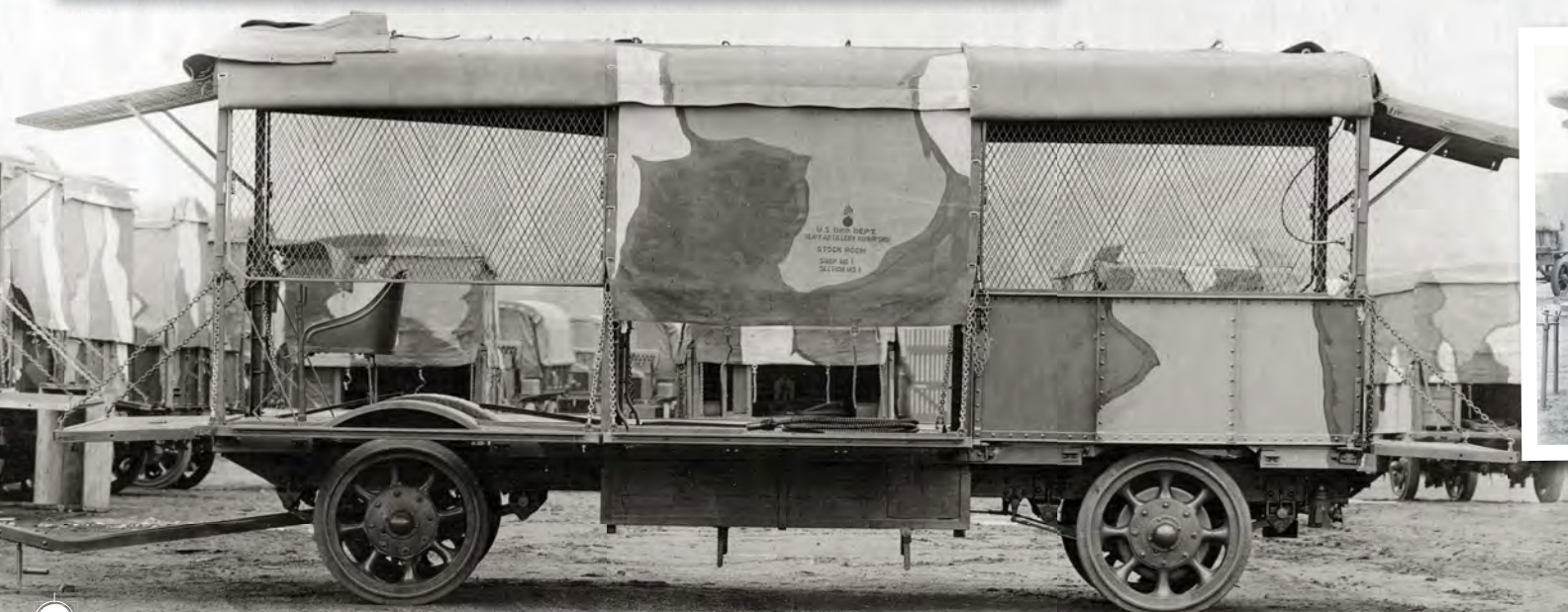
Below: This stock room trailer was designed for carrying the larger spare parts. This image shows that each trailer had a driver who was equipped with just a chair and a handbrake.
