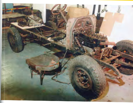
The chassis and original engine exposed before refurbishment. It's a Lancia Tipo 64, four-cylinder side-valve petrol unit with a capacity of 4940cc. It produced 70bhp at 2200rpm.
