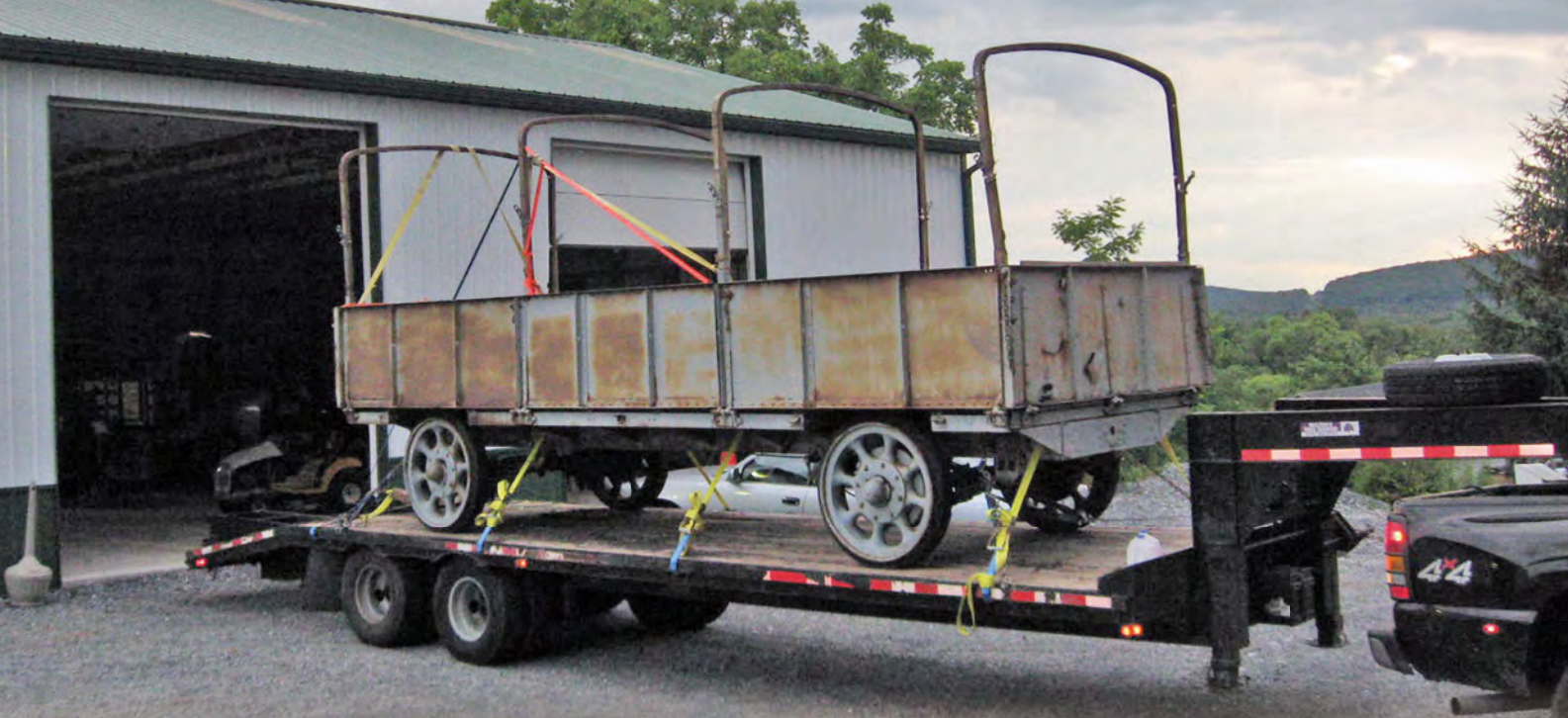
Dave Lockard's HMORS trailer. The hood bows were cleverly designed so they would telescope down during transportation. Ideal for low garage doors.
