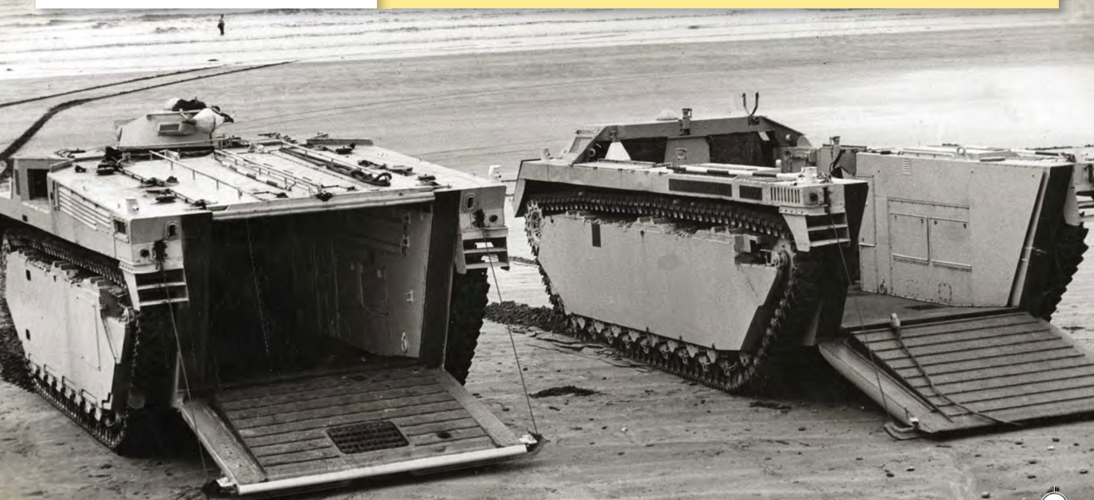
Below: A regular LVT-3 and a covered LVT-3C parked alongside one another on a beach. This suggests that the British must have had at least one LVT-3C.
