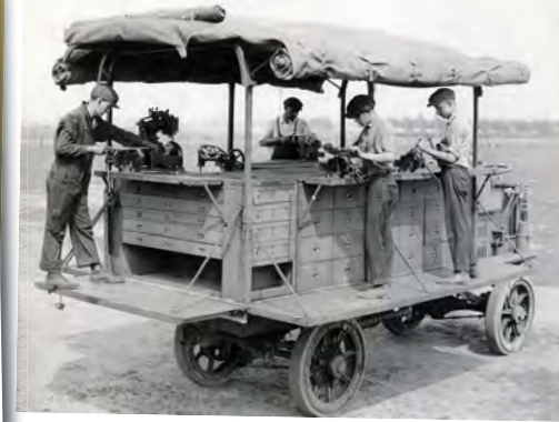
Above: The purpose of the equipment repair truck was to repair small arms and any other small items.
