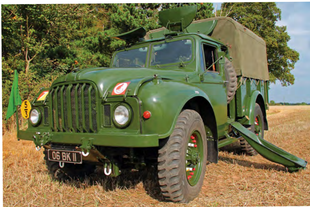
Above: The spare wheel carrier as well as all the hatches had to be rebuilt and refitted to the vehicle. It was tasks like this which led to the restoration taking so long with Tony wanting to make it correct in every way.
