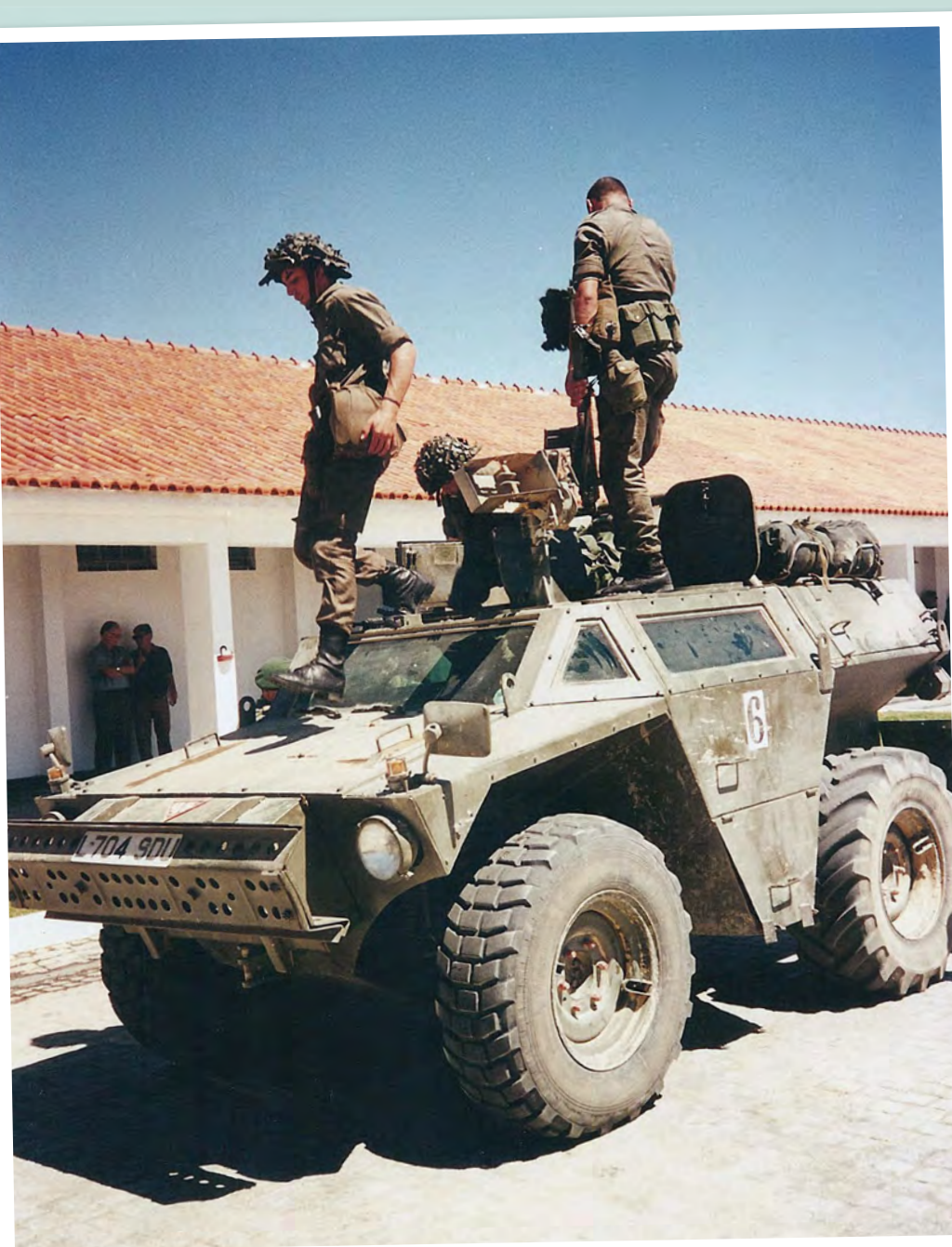
Above: Access was through hatches in the roof and personal kit could be carried outside.
