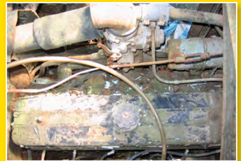
The copula on the vehicle had been left off, leaving the engine open to the elements.
