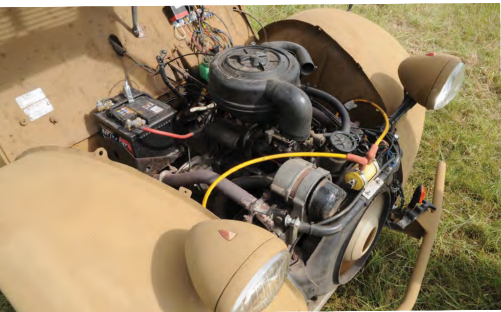
The original prototype would have had a rather feeble 425cc engine fitted, but Mike's fitted a more practical 602cc unit.
