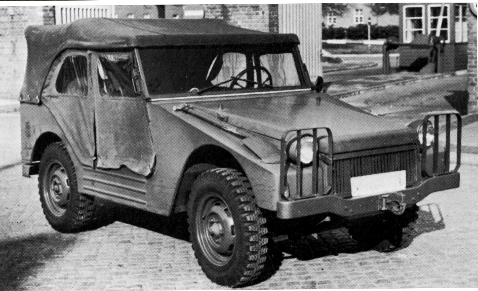
The Type 31 was improved to become the Type 34. Some obvious differences visible in this picture are the headlamp guards, the front bumper with its NATO hitch, and the three strengthening swages along the body sill. The side screens are also different from the simple canvas 'door' seen on the Type 31 prototype, and the shovel mounted on the wing gives an authentic military air to the vehicle.
