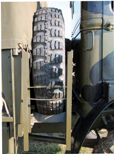
The spare wheel on the Bedford is carried behind the cab on the driver's side.
