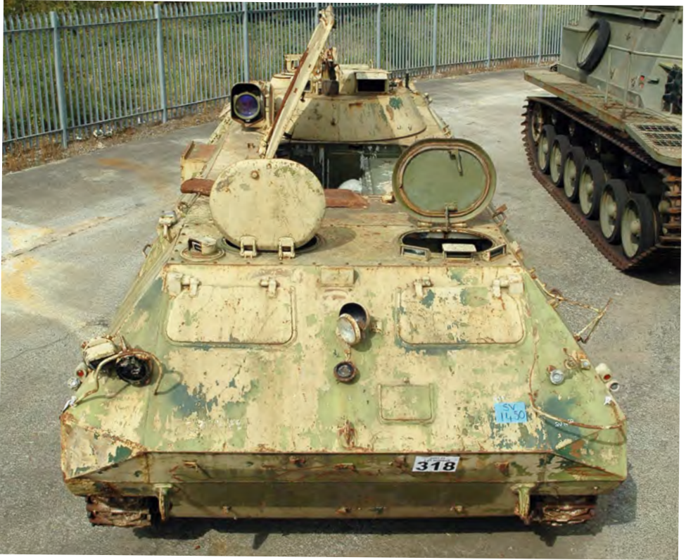
Above and below: The curious looking ACRV M1974 was offered for sale at an MoD tender sale held at Witham back in September 2007. The paintwork is, as you can see, original to the vehicle. The ACRV stands for Armoured Command and Reconnaissance Vehicle. It was based on the same basic chassis and running gear as the 2S1 122mm self-propelled howitzer.
