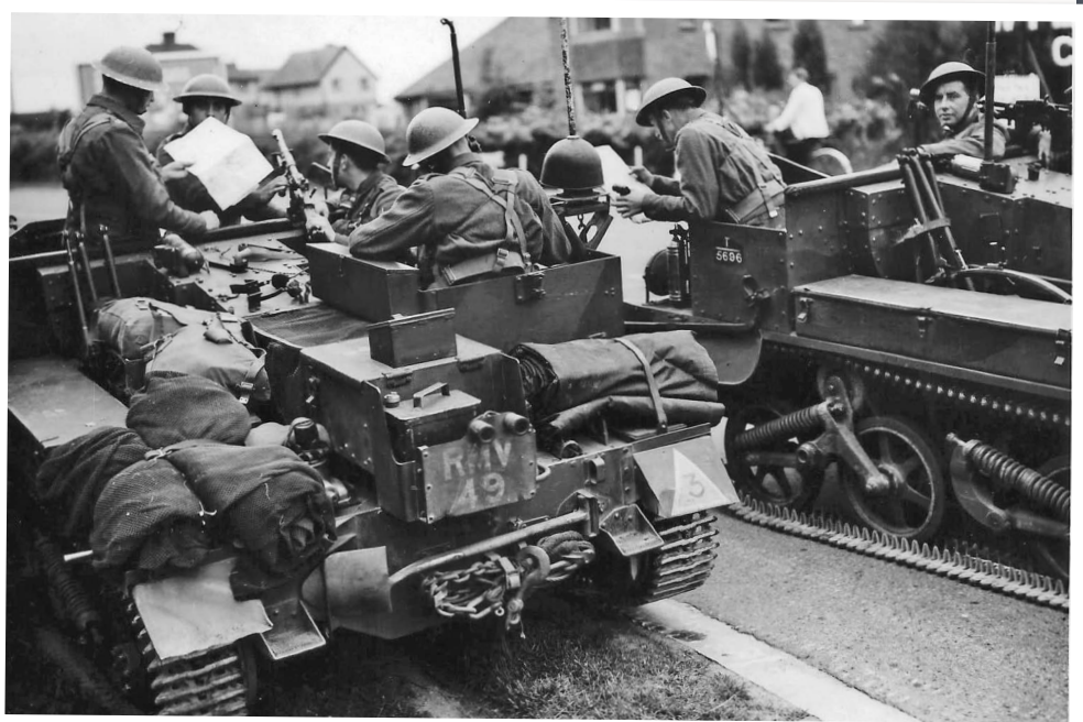
Scout Carriers of the Royal Gloucestershire Hussars of the Yeomanry Armoured Detachment serving in Britain after the Fall of France. They are essentially a mirror image of the Bren Gun Carriers at the back, with the stowage locker on the left and a compartment for a third man on the right.
