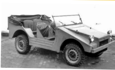
Above: This is another factory photograph, showing the overall layout of the Type 31 model. Note the two swages on the sill panel; Type 34 models had three. Right: The Type 31's two-stroke, twin-cylinder engine was borrowed from Goliath cars of the period. This is the GP700 model, introduced in 1950.
