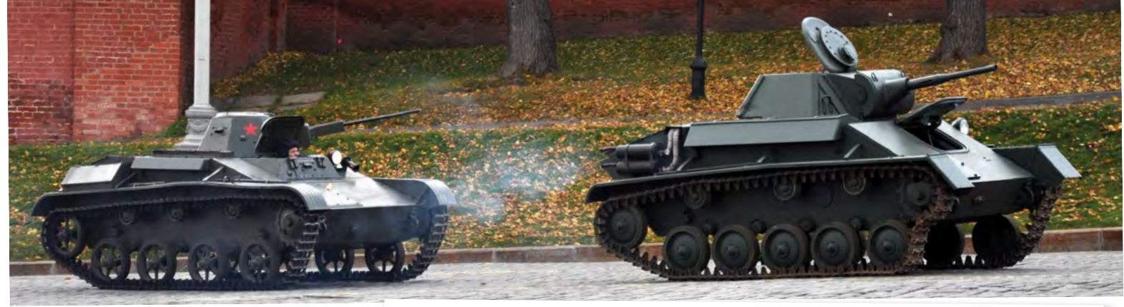
Above: The T-70 (right) was the production replacement for the T-60 (left) with only one year separating their respective service acceptances. The T-70 (actually two of them) was making its public debut on Red Square. Left: An FAI armoured car escapes the consequences of T-34 engine-start-ups! The FAI-M consisted of the earlier FAI hull and turret mounted on the later (and longer) GAZ-M1 chassis, hence the curious notch rear. Right: A BA-10A medium armoured car leads an FAI light armoured car across Red Square.
