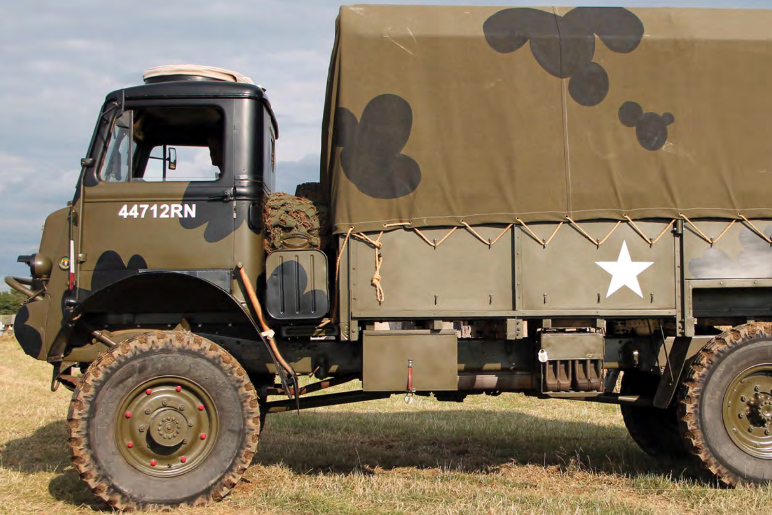
Although it now carries QLD type bodywork, this Bedford actually started out life as a QLR before losing the rear body soon after being demobbed.
