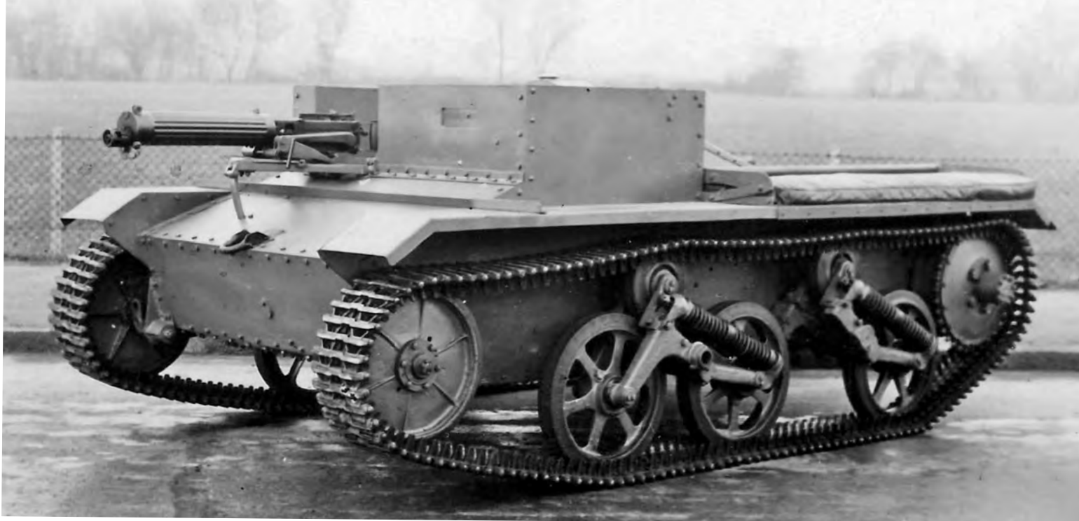
Above: Vickers-Armstrongs D50, the very first vehicle in the Carrier family. Note that the driver is seated on the left, and that the leading suspension unit is reversed.
