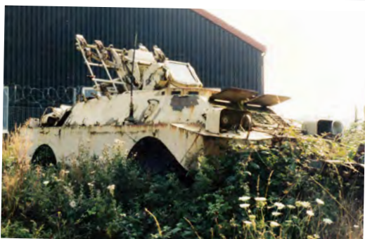
Left: A number of ex-Iraqi vehicles turned up in the compound beside the workshops at the Tank Museum, including this SA-9 Gaskin (Russian name 9K31 Strela-1), which is a derivative of the BRDM-2. Below: This pair of BMP-1 amphibious armoured personnel carriers also appeared in the October 2011 MoD tender sale held at Witham. The paintwork would suggest these are war booty, the green vehicle having been over painted at some point, presumably during evaluations.
