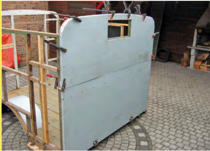
All pictures: Only the wooden frame remained of the wireless back end so with help from a local blacksmith, Jaap managed to create all the necessary panels.
