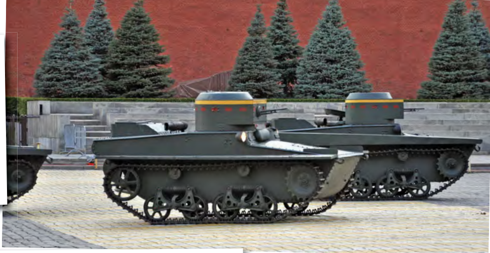
Above: Early and late T-37As, one with balsa wood floats mounted on the track guards. In fact all series production T-37s were designated T-37A.
