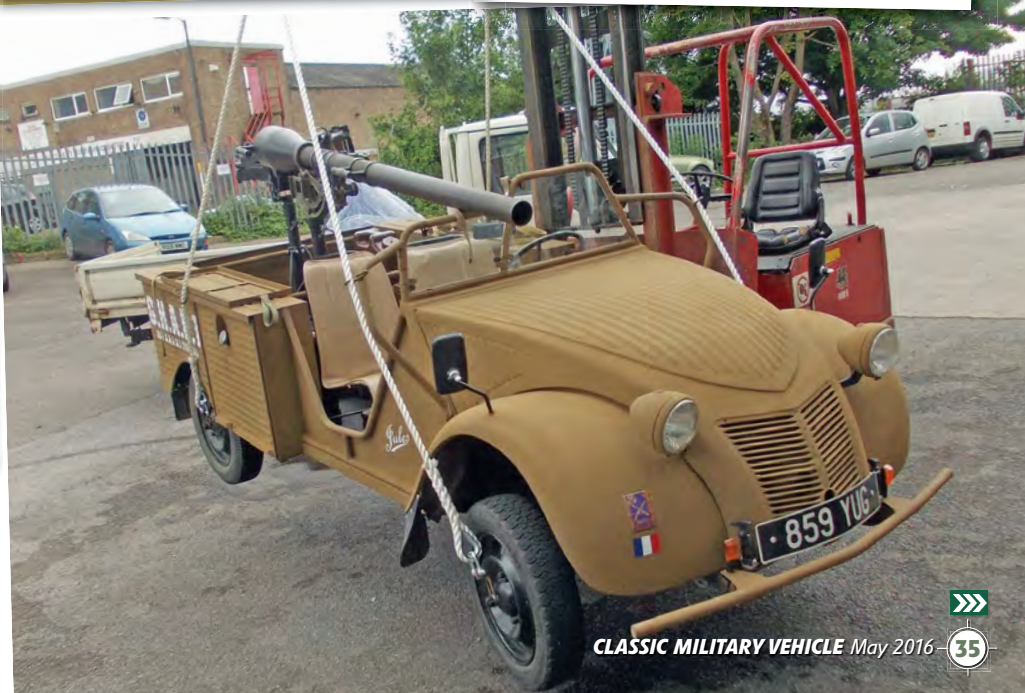
Right: A fork lift demonstrates how the vehicle would have originally been lifted. The hooks on the wheels, contrary to what the French thought, were only meant as tie-downs for when the original pickup was on deck.
