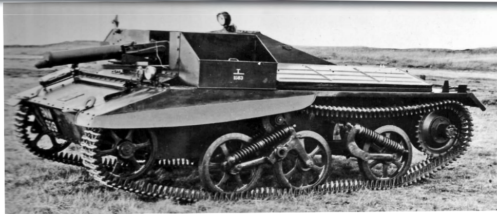
Above: Vickers-Armstrongs D50, the very first vehicle in the Carrier family. Note that the driver is seated on the left, and that the leading suspension unit is reversed.
