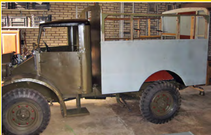
All pictures: Only the wooden frame remained of the wireless back end so with help from a local blacksmith, Jaap managed to create all the necessary panels.
