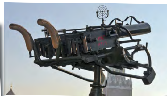
Above: The 4M anti-aircraft gun system. The quadruple 7.62mm water-cooled Maxim machine gun system was truck mounted and by all accounts rather effective.
