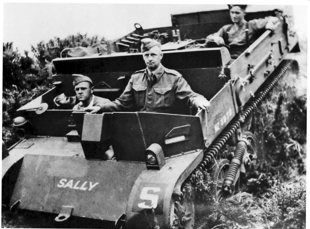
A New Zealand LP (Local Pattern) 2 Carrier. Much roomier than its British counterpart but almost identical to the Australian version and quite different from its LP1 which was essentially a mild steel copy of the British Bren Gun Carrier.
