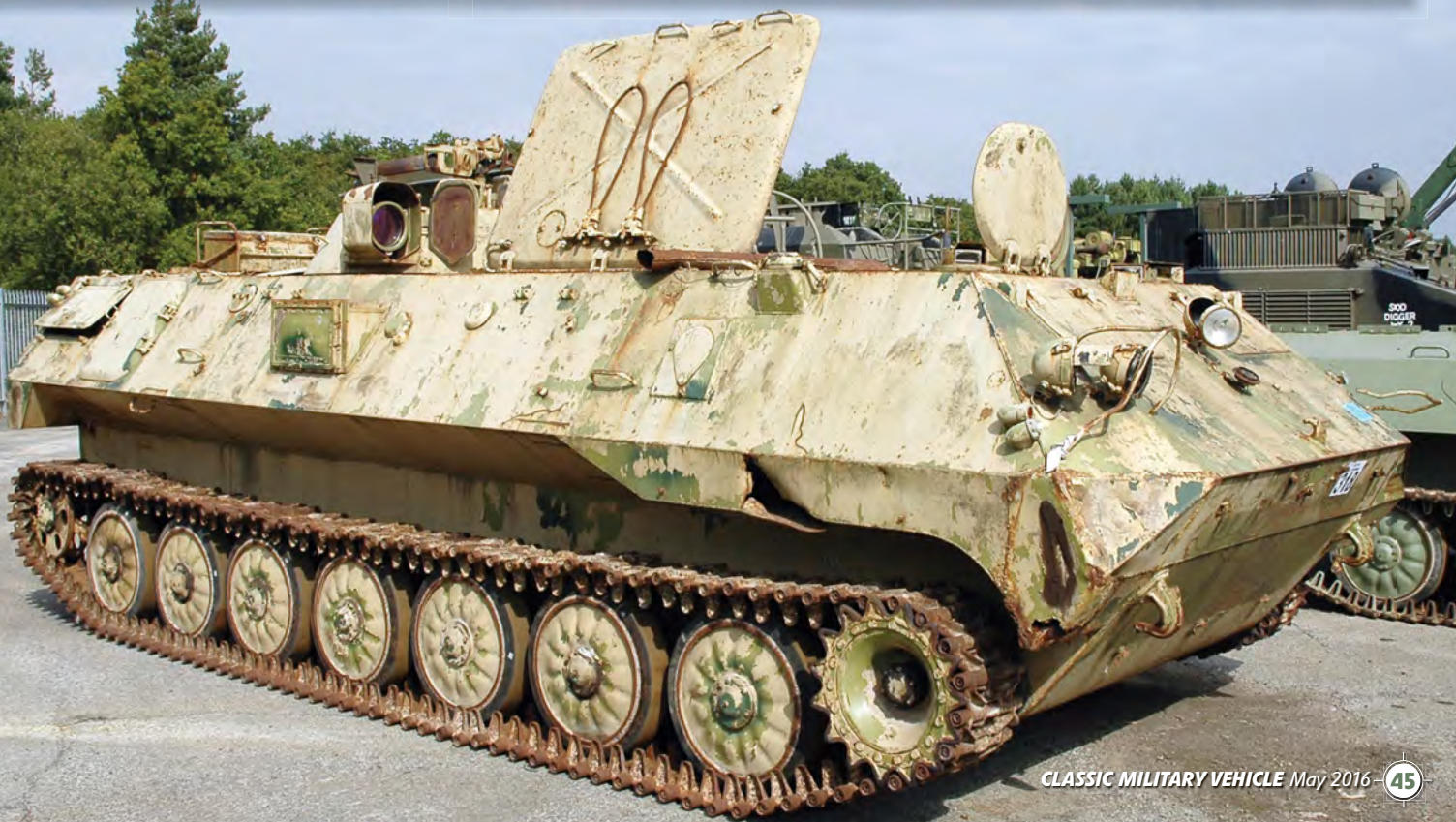
Above and below: The curious looking ACRV M1974 was offered for sale at an MoD tender sale held at Witham back in September 2007. The paintwork is, as you can see, original to the vehicle. The ACRV stands for Armoured Command and Reconnaissance Vehicle. It was based on the same basic chassis and running gear as the 2S1 122mm self-propelled howitzer.
