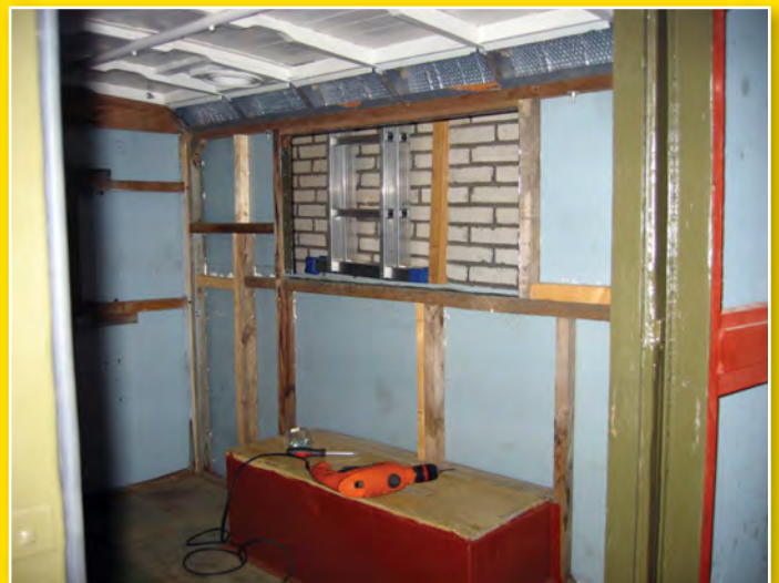
All pictures: Only the wooden frame remained of the wireless back end so with help from a local blacksmith, Jaap managed to create all the necessary panels.
