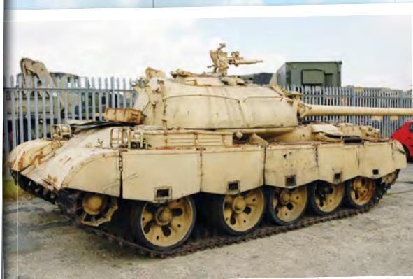
Above and right: Although this particular tank was identified in the catalogue for the sale in which it was appearing as a Russian T-62 tank, it is in fact an ex-Iraqi Army, Chinese-built Type 59, which was itself a copy of the Russian T-54 and in widespread use with the Iraqis during the Gulf War.
