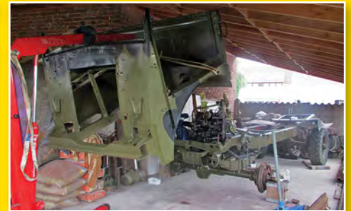
The copula on the vehicle had been left off, leaving the engine open to the elements.
