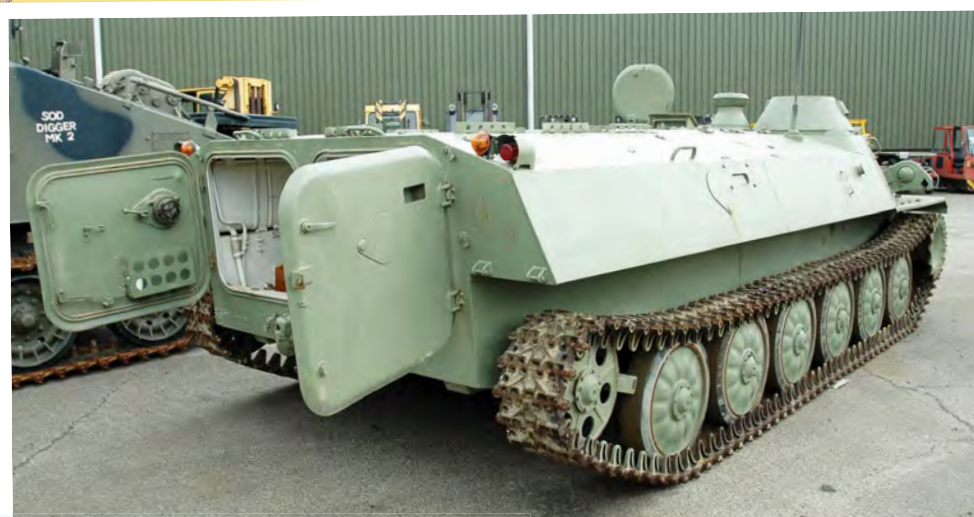
Above and right: Although this particular tank was identified in the catalogue for the sale in which it was appearing as a Russian T-62 tank, it is in fact an ex-Iraqi Army, Chinese-built Type 59, which was itself a copy of the Russian T-54 and in widespread use with the Iraqis during the Gulf War.
