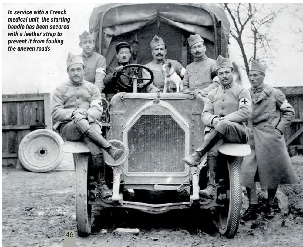
The pneumatic tyres allowed the Fiat a top speed of 36mph which is double that of a comparable size solid-tyred truck
