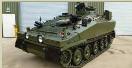
Spartan CVRT Dieselised APC , Fitted Cummins BTA 5.9ltr Turbo diesel engine, Engine power 195 hp, David Brown TN15d Epicyclic Semi-Automatic Gearbox with Neutral turn capability, Max road speed 72 km/h, Range 750 km, Manoeuvrability, Gradient 60%, Side slope 35%, Vertical step 0.5 m, Trench 2m, Fording 1m etc, Ex condition, .... Guide price from £19,995 (3 Available)
