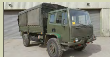
The DAF 4x4 Truck , Cargo capacity of 5000kg, Fitted Cummins 5.9 ltr Turbo Diesel, permanent 4x4, Hi Lo Ratio with Diff Lock, PAS, Air brakes, Nata style rear hitch, Engine power 145hp, Maximum road speed 89 km/h, Range 500 km, Year from 1994., ..... Guide price from £4,500 (40 Available)
