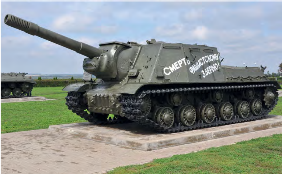
This ISU-152 Self-Propelled Howitzer is displayed as a representation of the earlier SU-152 based on the KV heavy tank The slogan reads "Death to the Fascist Beasts" which may have been more politically appropriate in 1943 than today, though maybe not...
