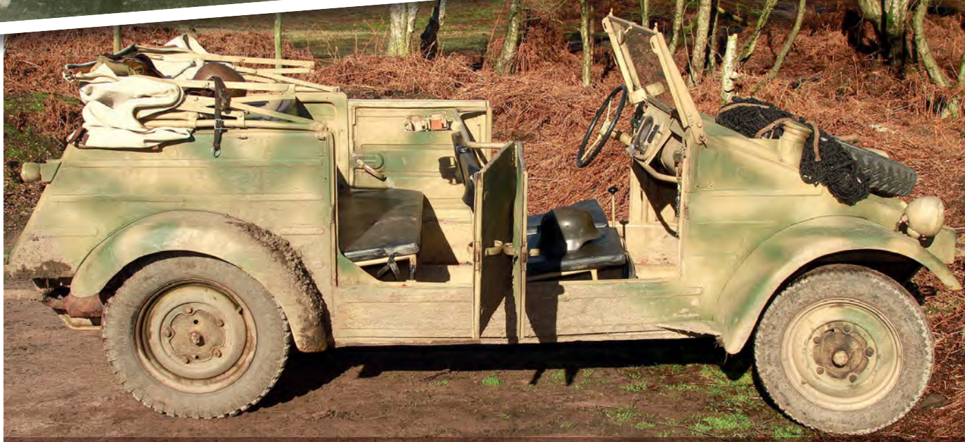
The Kübelwagen has many clever design features like the front and rear doors which share the same hinges, hung from tubular door posts which in turn connect to a transverse tubular rail for strength, all designed for space and weight saving BELOW: Proud owner Matthew has achieved what at one time he considered a vain hope; a working, authentic Kübelwagen
