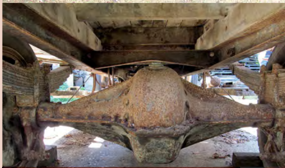
The back axle was made of two steel pressings bolted together with the date of manufacture being stamped on the case. In this instance August 2, 1917
