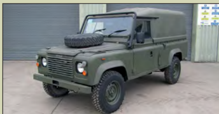
Land Rover Defender 110 Tithonus Hard Top RHD , Fitted 2500cc NAD engine LT77 5speed gear box, Transfer box with Hi Lo ratio & centre diff lock, 12 Volt electrics, Wolf style wheels, Disc brakes, Soft type steering wheel, mileage from 60,000 km, ..... Guide price from £6,250 (10 Available)
