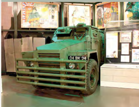
The Humber 'Pig' was originally a general purpose truck but when violence escalated in Northern Ireland in the 1970s, they were fitted with additional armour.
