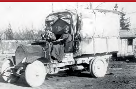
The pneumatic tyres allowed the Fiat a top speed of 36mph which is double that of a comparable size solid-tyred truck
