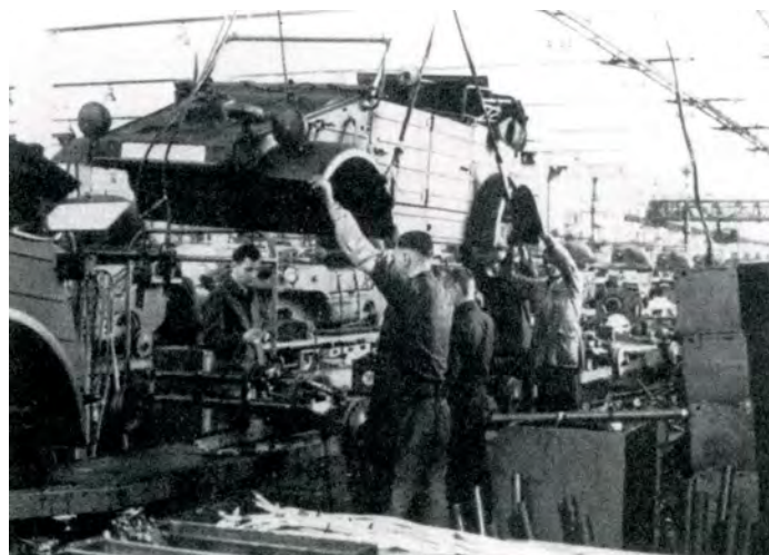
ABOVE: A body drop in the motor-industry tradition mated chassis and coachwork of the Type 82 at Fallersleben. Outside suppliers, including bodies from Ambi-Budd in Berlin, provided much of the initial content
