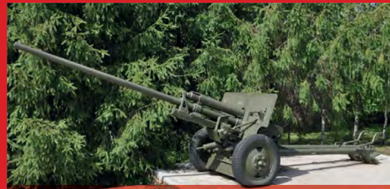
The 57mm ZiS-2 looks nearly identical to the 76 2mm ZiS-3, but was a more focused anti-tank weapon. It has a longer barrel without a muzzle brake
