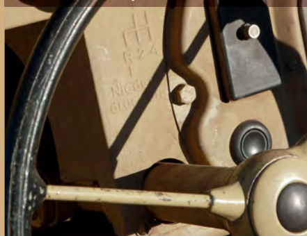
Through the later style steering wheel spokes can be seen the gearbox layout with 'Nieder drücken' instructing 'press down' for reverse gear. The wiper motor is a modern Japanese item
