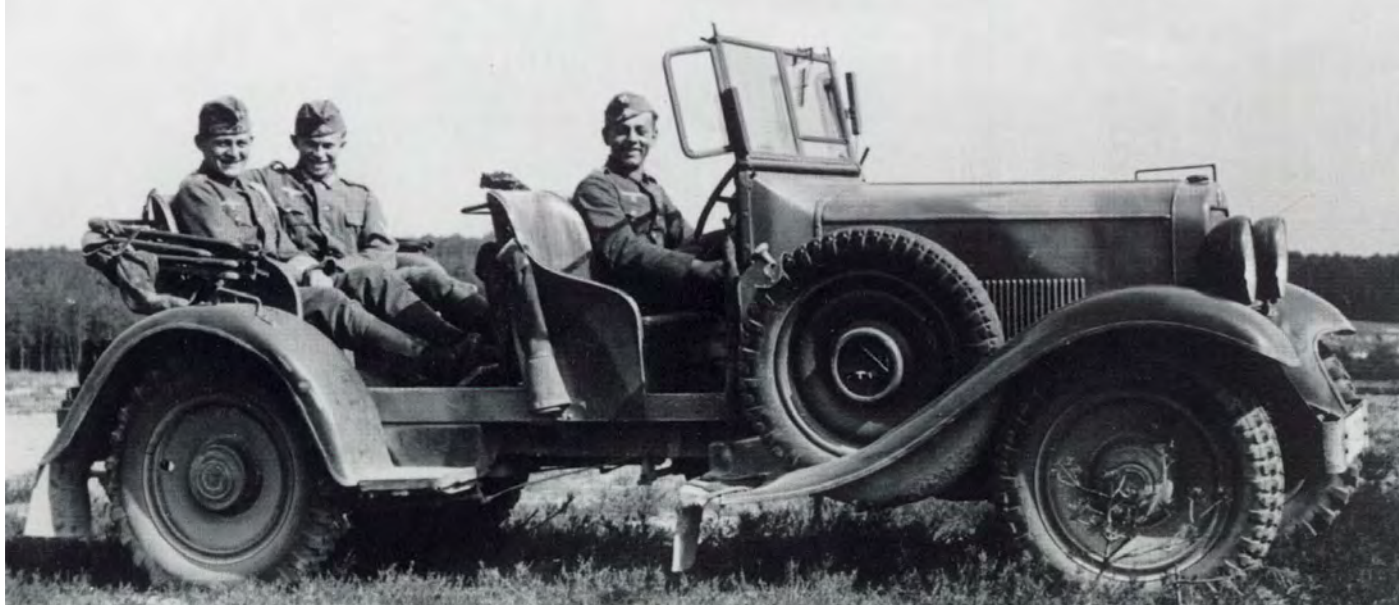
A military version of Porsche's front-engined Wanderer chassis well illustrated the origin of the term Kübelwagen as used for most German military people-carriers with their Kübel or bucket seating.
