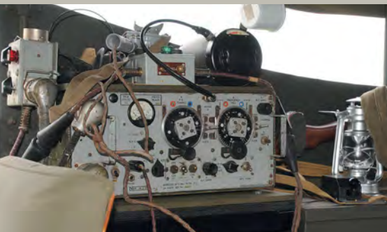
Andy has installed the Type No 19 radio set as used by the British Army and added some other items, including the hurricane lamp and tin mug to make life a bit more comfortable
