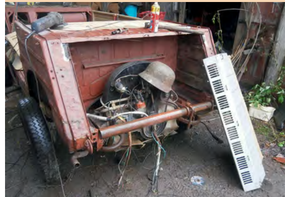
Subsequent Czech welding to the 1941 body had distorted the rear crossmember and the engine cover did not line up. An Acrow prop acts as a temporary brace while Matthew works to replace the crossmember
