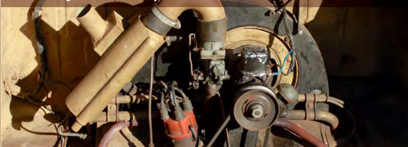
Matthew has fitted a post-war Volkswagen Typ 122 1,192cc air-cooled petrol engine though the fan housing dates from the war years
