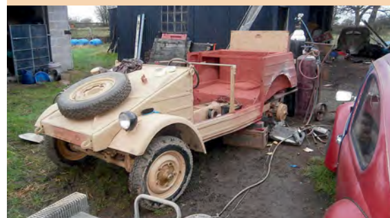
Work progresses at Matthew's workshop and a coat of 'Dunkel Gelb' is applied to the red oxide finish with which the body arrived
