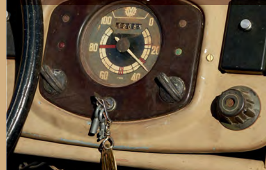
Matthew's replica dash has a Kübelwagen-style clock face distressed to look appropriately aged while genuine Bakelite controls are from a 1950s Beetle and are slightly smaller than those found on the Kübelwagen
