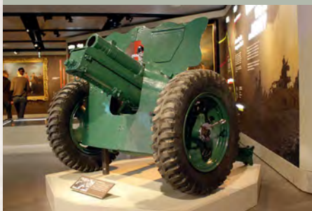
The 1944 Pack Howitzer was designed for challenging terrain and could be broken down and carried in several pieces
