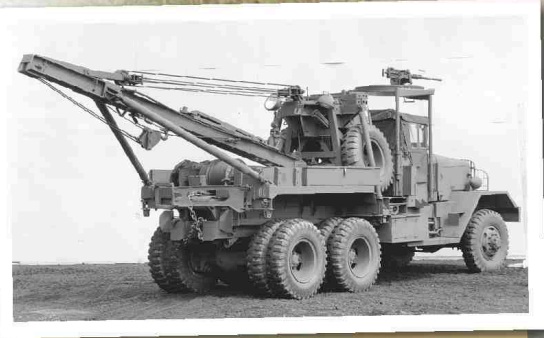
The most obvious change brought about with the introduction of the Ward LaFrance series 5 was the military-style open cab introduced with this series. Also visible just behind the cab are the three levers that control the now power-operated crane. Just to the rear of them can be seen the stabiliser legs added to each side, and the vastly different tool box and bed arrangement. Compare this to photos of earlier vehicles to see how the wreckers became much more cluttered looking. The pioneer tool rack is also visible in this view, just above the step to the cab. (National Archives)
