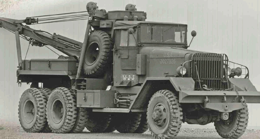
Left: This is the Kenworth version of the M1A1, almost indistinguishable from a Ward LaFrance M1A1. The whiffle tree was slightly different: notice the Kenworth whiffle tree lacks the flange across the back present on the Ward LaFrance. The tool lockers varied with manufacturer as well, although a few Ward LaFrances were built with the Kenworth tool lockers, to use excess inventory after Kenworth stopped building the trucks. (US Army)
