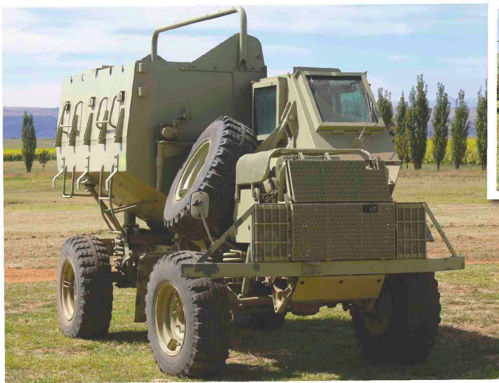
The Buffel was developed in the 1970s under the auspices of ARMSCOR (Armaments Corporation of South Africa) to meet the operational requirements for a mine protected Armoured Personnel Carrier (APC) for the South African Army. It uses a German Mercedes-Benz UNIMOG Model 416/162 series 4x4 chassis and featured a Merc engine. Around 2400 were built for the home and export markets and some are still being used by the South African Army.
