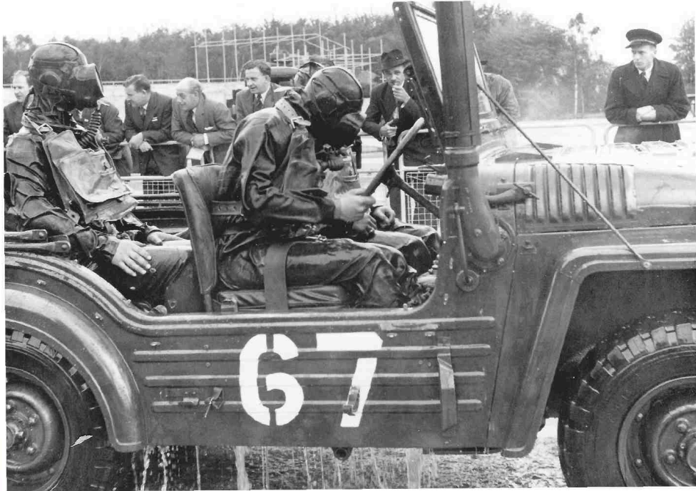
With the snorkel erected, the Champ was equipped to wade to a depth of 72in (1830mm) with a minimum of preparation, requiring the driver to stand or kneel on the seat and operate the vehicle using the hand throttle. Holes in the floor allowed water to drain from the interior. The photograph was taken at the Exhibition of British Military Vehicles at Chertsey in 1956. (Soldier Magazine)
