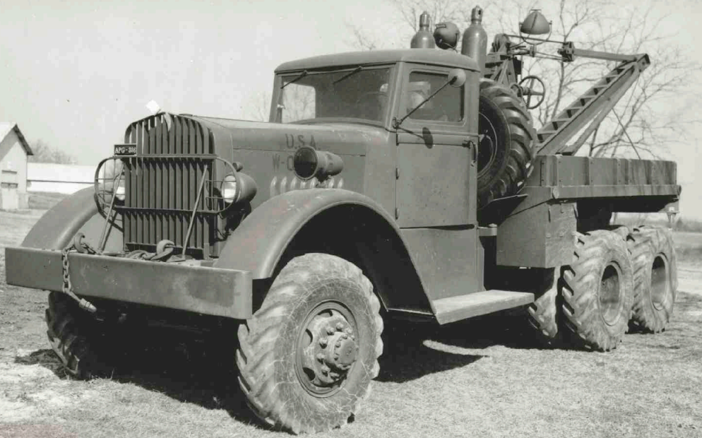
This is one of the two test examples of the famed Ward LaFrance M1 wrecker. Representing the earliest production, this photo was taken on March 18, 1941. The front-end sheet metal was an adaptation of Ward LaFrance's civilian product. The front winch is hidden between the front bumper and the radiator. One of the spare tyres, with directional tread, can be seen behind the cab. (National Archives)
