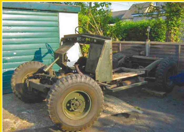
By early 2012 the Humber had been stripped back to the chassis so that the rebuild could begin.
