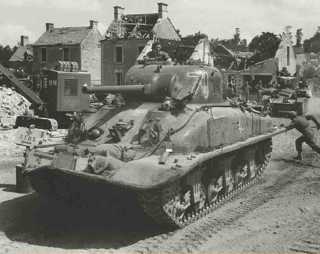
This M4A1 DD has had its screen cut off to clear away space ahead of the hull machine-gun and to reduce risk from enemy flame throwers but the lower portion has been retained as a useful space to carry stores.
