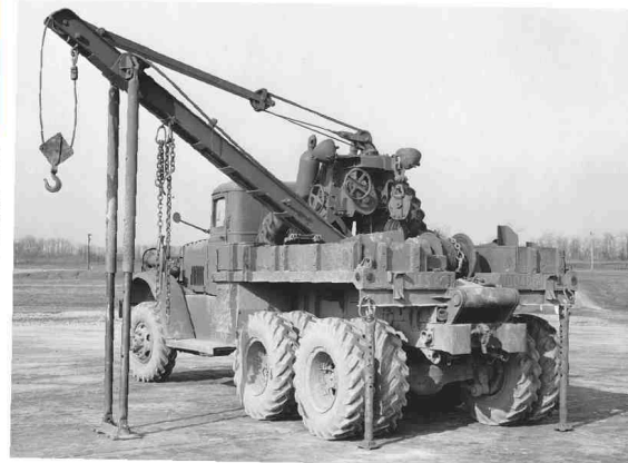
The Series 2 wreckers incorporated a much needed drag winch (a Gar Wood 5M713K, 47,000 lb capacity) on the rear of the truck, as can be seen in this April 1942 photo. In addition to the outriggers on the rear of the chassis to stabilise the truck, these wreckers had boom jacks, shown in place here, to support the outer end of the Gar Wood US5 boom during heavy lifting operations. (National Archives)
