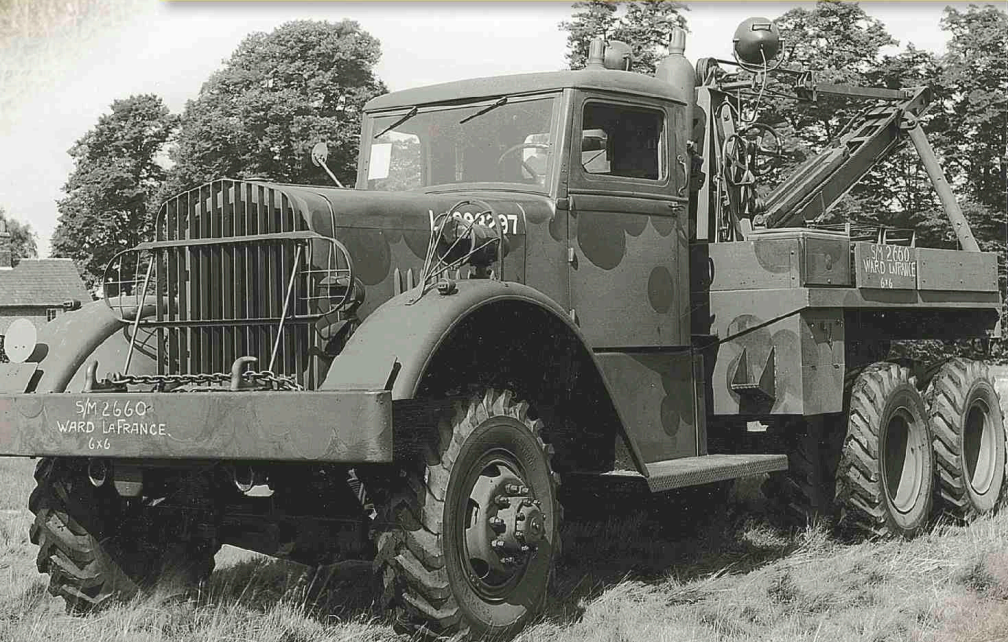
Below: The Series 3 lacked the front and rear trailer connections found on the earlier models, and the entire run of 365 was supplied to the British as Lend-Lease items. These trucks also had the British style lighting, including the spotlight illuminating the white-painted rear differential cover, creating a blackout tail light.
