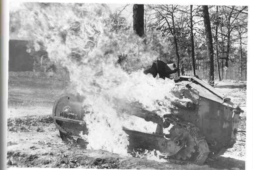
Above: The US Army copied the Renault FT-17, fitting a Buda engine, and dubbing the result '6-ton tank, M1917'. It was planned that 4400 examples would be constructed, but, by November 1918, just 64 had been completed, with only 10 sent to Europe. Just 1100 or so were eventually constructed. The tracks were modified in 1931 and a new engine fitted, changing the designation to M1917A1. This fiercely-burning example was photographed as late as 1941, demonstrating the effects of the 'Molotov cocktail' at Atlanta, Georgia. (Warehouse Collection) Below: The bicycle in the background would suggest that this is a post-war picture, but it does show how the rear skid of the Renault FT-17 supports the tank when crossing trenches and ditches. (Warehouse Collection)
