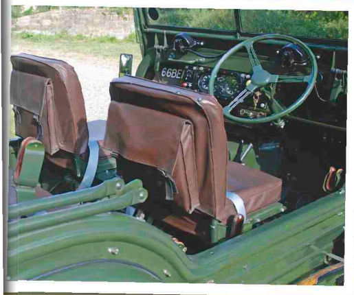
The driver's compartment showing the slight angle at which the steering wheel is presented to the driver, and the standardised instrument panel; although of the same period, the switch panel to the left of the instruments is not original. The windscreen wipers are vacuum operated. (Warehouse Collection)
