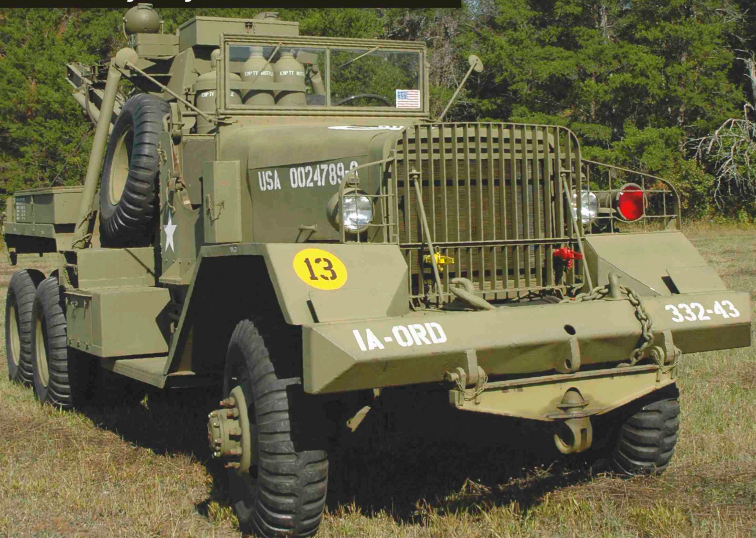
The M1A1 was America's heavy wrecker during WW2. Its chisel-shaped bumper and towering grille display a down-to-business styling typical of heavy vehicles of the era. This restored example is from the collection of the late Kevin Kronlund, Spooner, WI, USA. (David Doyle)
