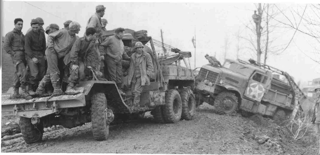
Every available man is standing on the front end of an M1A1 to help it get more front-end traction while attempting to free a mired 6-ton 6x6 pontoon bridge truck. The whiffle tree is of the Ward LaFrance type with the raised flange around the edges. Note the chains on the rear set of tyres of the wrecker, and the telephone linemen in the trees, watching the proceedings. (National Archives)
