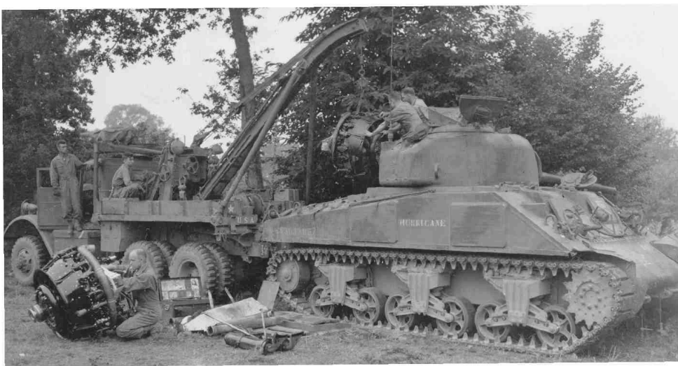
The Series 4 Ward LaFrance Model 1000 is readily identifiable by the curved boom of the Gar Wood US5G crane, in place of the US5 straight boomed crane used previously. Although the boom was still manually operated, these trucks had a dual-ratio swinger gear for the boom, the operating wheel being moved between shafts on the driver's side of the crane A-frame to select speed. Inside the cab the obvious change was the introduction of individual military instruments in place of the civilian type used previously. This example was photographed near Le Teilleul, France, on 16 August 1944. (National Archives)
