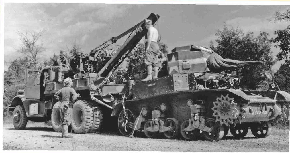
The US military's Heavy Wrecking Truck was designed not only to tow wheeled vehicles, but also to recover and tow fully track laying vehicles. A robust chassis and a wrecker bed equipped with a crane, torch set and an array of tools made these trucks a go-anywhere repair shop. Here, a Series 2 Ward LaFrance tows a disabled M3A1 Stuart light tank down a dusty Tennessee road during the October 1942 manoeuvres. (National Archives via Jim Gilmore)
