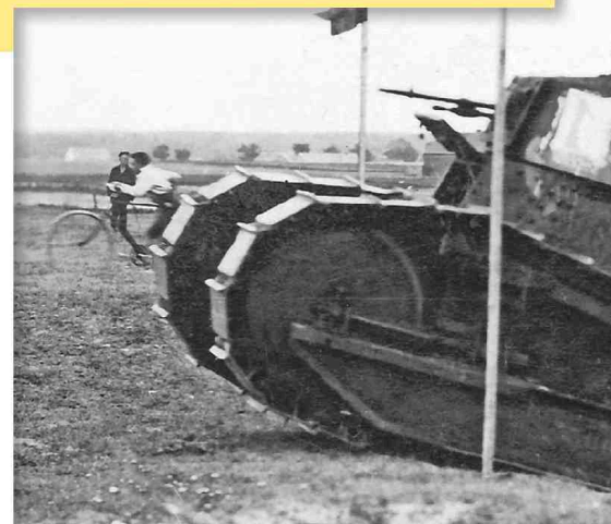
Above: The US Army copied the Renault FT-17, fitting a Buda engine, and dubbing the result '6-ton tank, M1917'. It was planned that 4400 examples would be constructed, but, by November 1918, just 64 had been completed, with only 10 sent to Europe. Just 1100 or so were eventually constructed. The tracks were modified in 1931 and a new engine fitted, changing the designation to M1917A1. This fiercely-burning example was photographed as late as 1941, demonstrating the effects of the 'Molotov cocktail' at Atlanta, Georgia. (Warehouse Collection) Below: The bicycle in the background would suggest that this is a post-war picture, but it does show how the rear skid of the Renault FT-17 supports the tank when crossing trenches and ditches. (Warehouse Collection)
