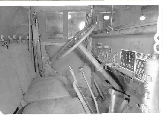
The interior of the cab of an M1A1. Partially hidden by the carbon tetrachloride fire extinguisher are, top, the cooling system draining instructions and, below, the vehicle's nomenclature plate. To the left of these plates is the shifting instructions plate. The levers are, left to right, the hand brake, transmission gearshift, front axle declutching lever, and transfer case shift lever. An M1903 Springfield rifle is in the universal bracket. (US Army)
