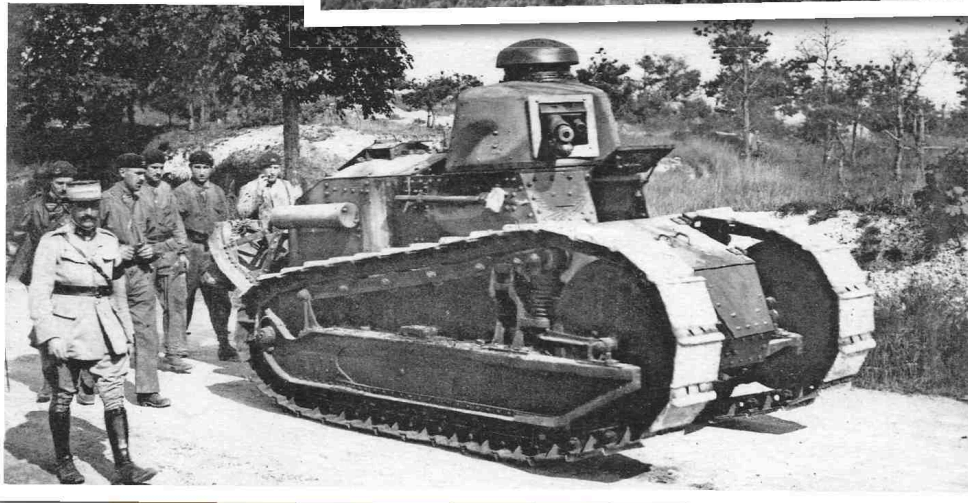
The diminutive size of the Renault FT-17 is apparent in this picture postcard view which shows the tank advancing at walking pace. Top speed of the Renault was almost 5mph (7.7km/h) and the range, on hard surfaces, was 21 miles (35km). The tail skids, clearly visible at the rear, were removable. (Warehouse Collection)
