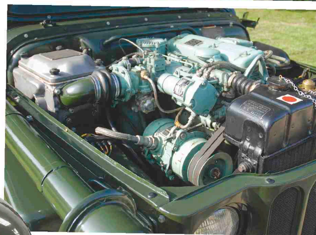
Above: Under the bonnet, the massive proportions of the Rolls-Royce B40 engine are apparent. Note the air filter and the lowered snorkel, intended for deep-water wading. The photograph also shows the Solex side-draught carburettor, the curiously-placed coil, and the huge dynamo. All of the engine intakes are sealed below the waterline to allow wading; the electrical equipment is both radio-screened and waterproofed. (Warehouse Collection)
