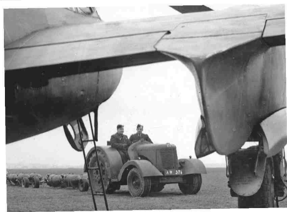
Above: Based on the agricultural tractor that David Brown had introduced in 1939, and which was later designated VAK-1, the David Brown VIG-1/100 entered service with the RAF as a light aircraft tractor in 1941. The VIG-1 was perfectly capable of providing a drawbar pull of 2,500 lb (1,136kg) and, in its later VIG-1/462 configuration, a torque converter was used to replace the clutch, giving a smoother take-off under heavy loads. There was a 5-ton chain-driven winch at the rear. Total production amounted to around 1,350 vehicles.
