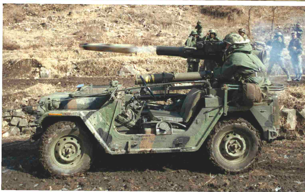
M151A2 mounting the US Army's TOW (tube-launched, optically tracked, wire-guided) missile system. The photograph was taken during the joint South Korean/US training exercise 'Team Spirit' in 1984. (US Department of Defense)
