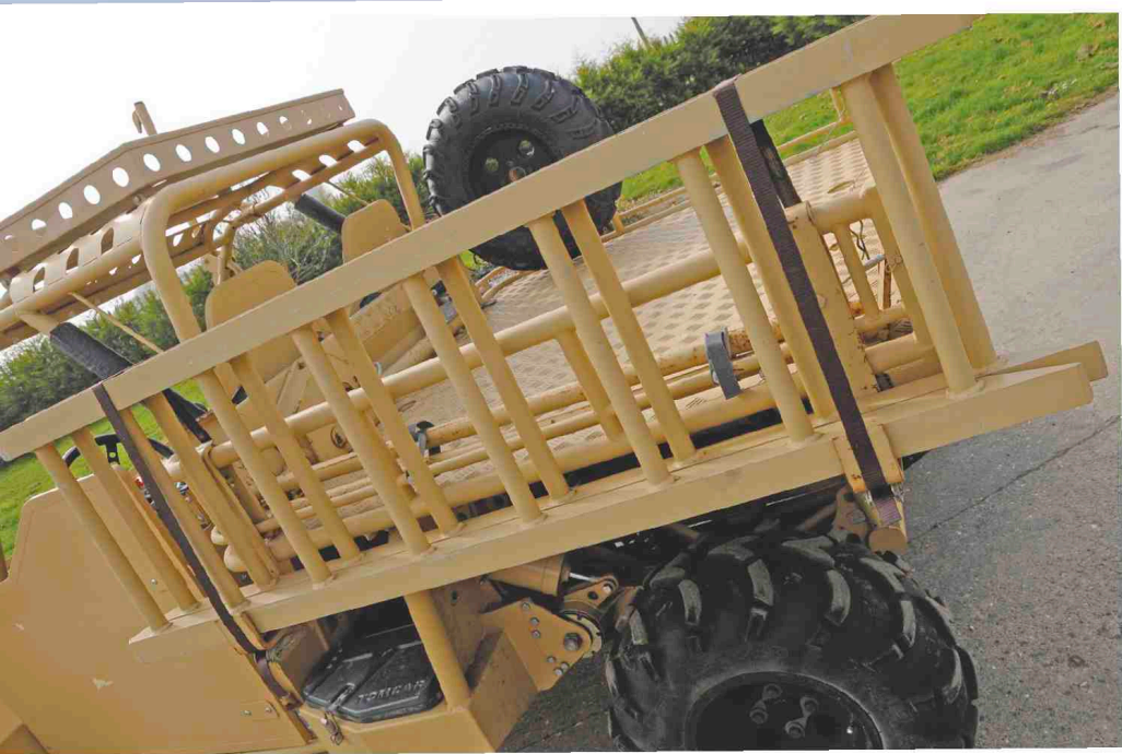
Rear was designed to carry pallets of combat supplies as well as casualties.
