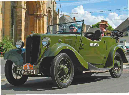
Above: One of the smallest military vehicles on show but also one of the most interesting was this 1935 Morris C8 radio car. This is the only example known to exist, with many being lost during the retreat from Dunkirk in 1940. The strange set-up in the car sees there being no passenger seat with just one back seat for the operator of the radio set which can also be found behind the driver. Right: A nice selection of American built half tracks seen at Camp Arizona near Carentan. Below: This 1944 GMC CCKW Bolster Truck had made the trip to Normandy all the way from Leek in Staffordshire. Although the vehicle owner also has the Pontoon trailer to match it was decided that it would be best to leave it at home for this journey. Still the vehicle is certainly something different with this example being restored around six years ago now with the paintwork being taken all the way back to the bare metal.
