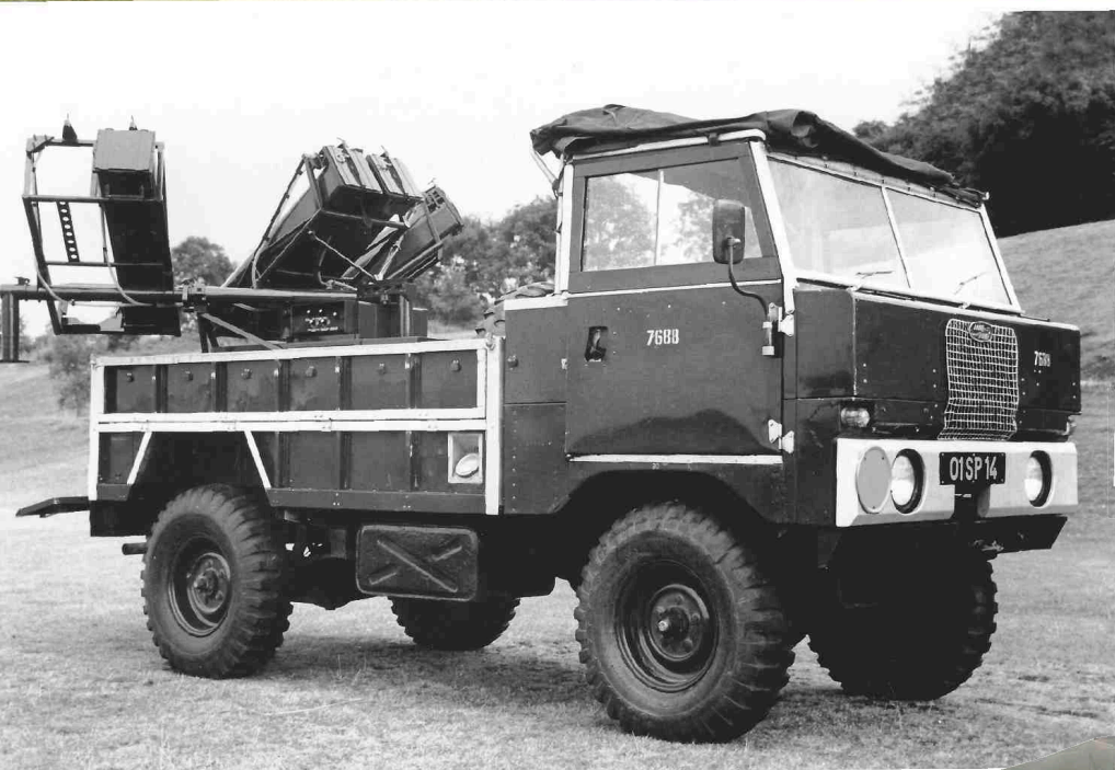
Above: One of the five early prototypes was used as a trials vehicle for the BAC Beeswing battery missile system, deploying four Swingfire wire-guided anti-tank missiles in a rotating mount. (British Aircraft Corporation) Right: Illustration taken from GSR 3463, dating from June 1968. The general appearance of the vehicle matches that of the early prototypes but note the front-mounted winch; when a winch was fitted to production vehicles it was mounted under the chassis. (Warehouse Collection)
