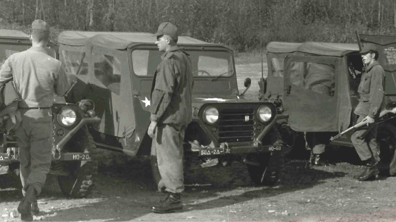
Line-up of brand-new M151A1 variants. The M151A1 can be recognised by the small turn indicators mounted on the tops of the front mudguards; the original M151 had no indicators. (Warehouse Collection)
