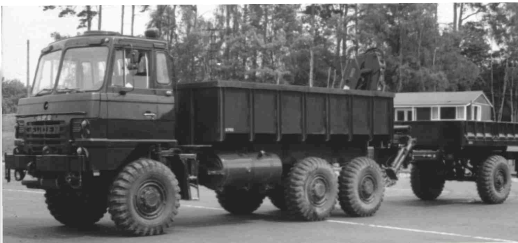
This is the engineering model of the Foden Medium Mobility Load Carrier with its powered axle trailer which was eventually shelved. MVEE had been involved in another unsuccessful study of a powered axle trailer towed by the Land Rover 1 Tonne. (TMB)
