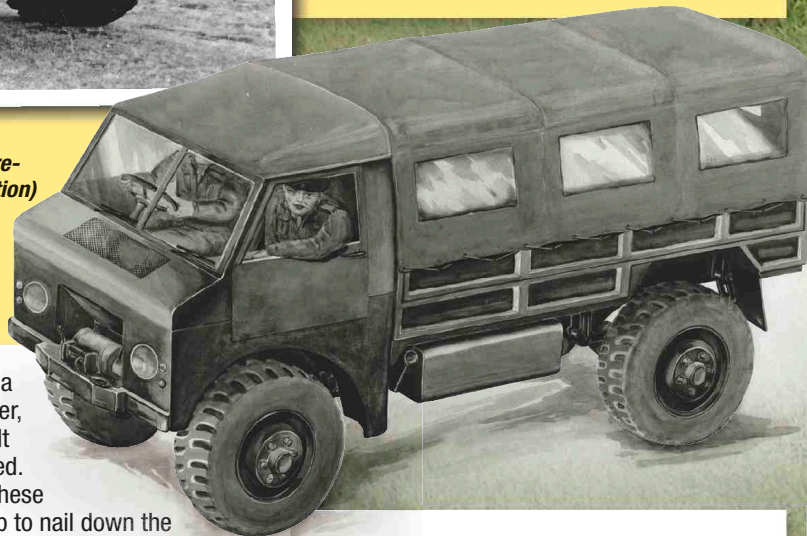
Above: This early prototype communications vehicle, which forms part of the Dunsfold Collection, nicely illustrates the short boxy front extension, presumably required to accommodate the radiator for the six-cylinder Rover engine. (Warehouse Collection)
