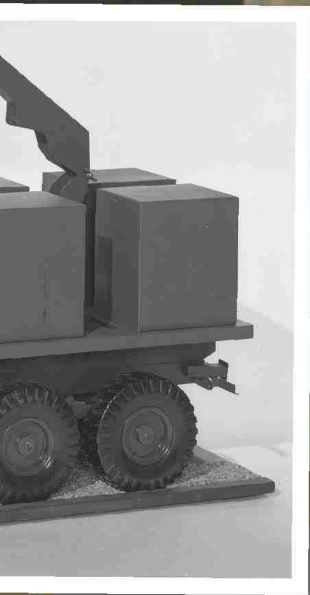
Left: The FH70 Tractor model is an AEC Militant Mark 3 (0870) carrying a crew compartment and four NATO ammunition pallets. The body on the Foden would also have a locker at the rear for carrying various tools associated with emplacing, servicing and firing the gun. (TMB)
