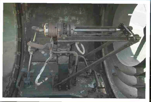
Above: The business end of the searchlight in daylight giving a good view of the carbon rod (horizontal item in the middle) which is consumed during use. The mechanism feeds the rod into the tip. Left: Rick holding the steering/aiming arms of the 90cm searchlight with the 18/24kw generator in the background.
