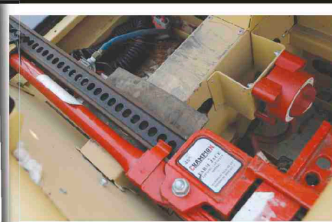
Above and below: An air compressor sits behind the front seats, alongside a 48in farm jack.
