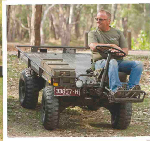
Below: Rod Mills on his recently imported M274 A5 Mule. Weighing only 900 lb, it's great fun for zipping around the Corowa site.
