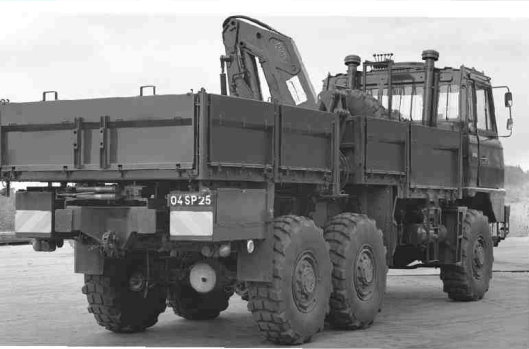
FH70 Tractor although here it is seen rigged as a Limber. It is fitted with steel dropsides and note the mid-mounted Atlas crane. (TMB)
