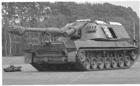
Above: A fully laden prototype FH70 tractor towing a mock-up of the FH70 gun during trials at Chertsey. The mock-up gun appears to use the real trails and wheels of an FH70 and only a simulated gun has been added. (TMB) Left: SP70 was the sister project to FH70. It mounted the same ordnance on a Leopard-based chassis but in a specially built turret. One of its more obvious problems was loading ammunition up to a turret at turret ring height! (TMB)
