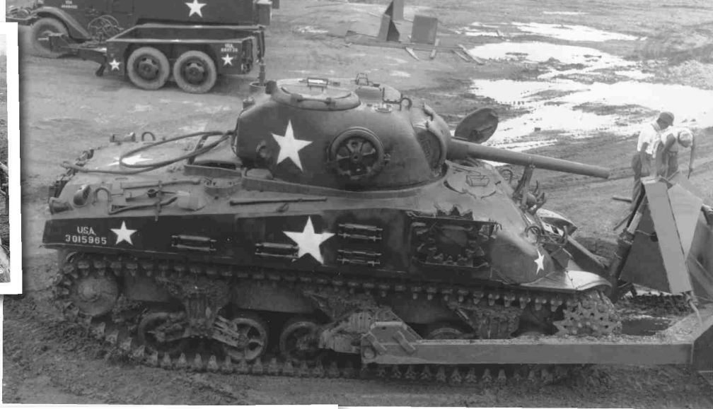
Above: The M1 continued to be used by the US Army well beyond the end of WW2. This example mounted on a composite-hull M4A3, was photographed in Korea on 2 August 1950. The lift cylinder and surrounding armour are shown to good advantage. Although suspension lock outs had been recommended as soon as the dozer attachments were fielded in 1944, they did not become part of the kit. Hence, this vehicle exhibits the characteristic slight nose down stance of tankdozers. Left: With the advent of the M4A3E8, the M1 blade had to be redesigned. The result was the M1A1, shown here. Other than the mounting and a 14in increase in width, it differed little from the earlier model.
