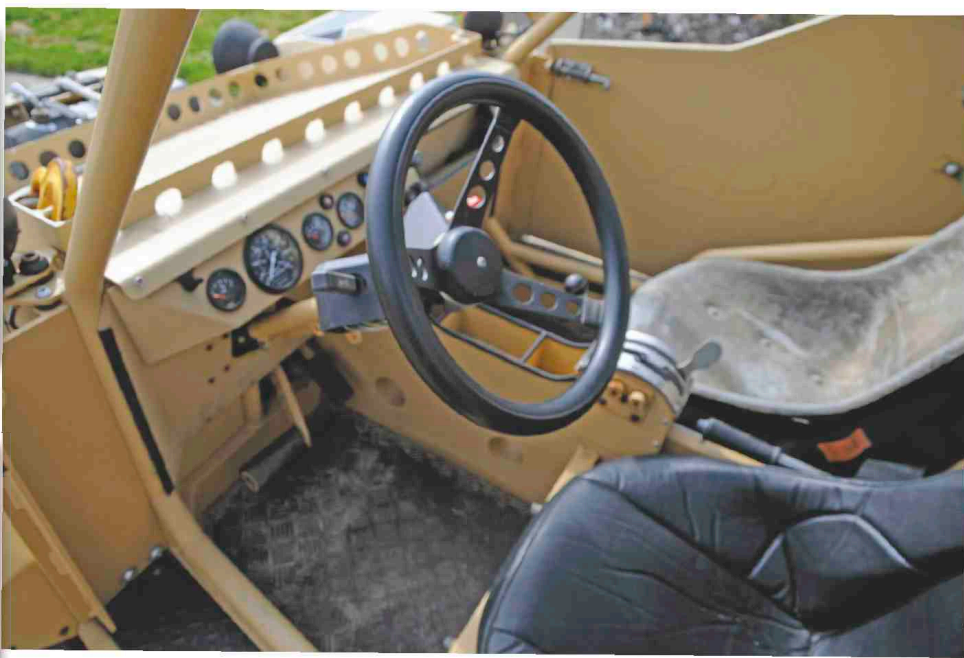
Above: Springer offers seating for two – based on the US Tomcar, all are left-hand drive. Left: Three modes are provided on the drive train. The top mode delivers high speed and low torque while lower mode gives more torque and less speed. The middle mode delivers a combination of speed and cross-country capability.
