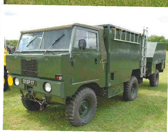
Above: This early prototype communications vehicle, which forms part of the Dunsfold Collection, nicely illustrates the short boxy front extension, presumably required to accommodate the radiator for the six-cylinder Rover engine. (Warehouse Collection)
