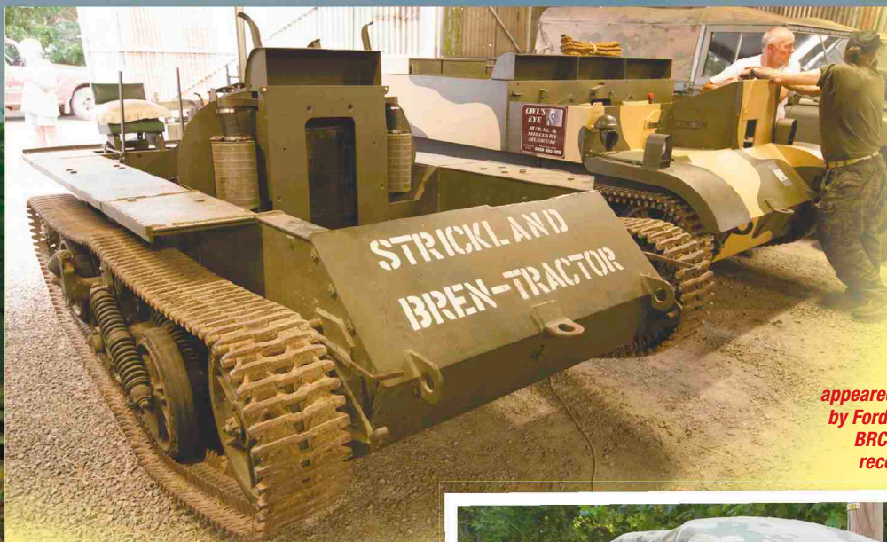
Above: A very rare Strickland Bren-gun carrier conversion used by farmers due to a lack of tractors after WW2.
