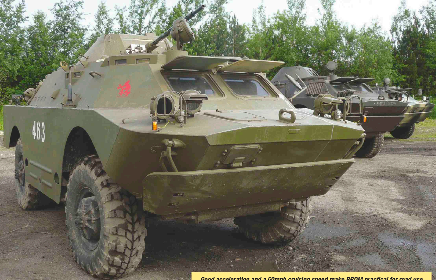
Good acceleration and a 50mph cruising speed make BRDM practical for road use.
