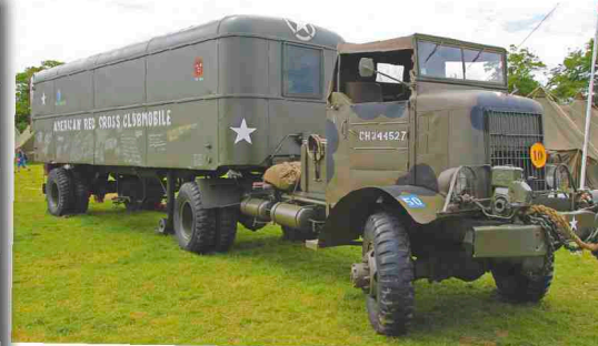
Above: The Autocar U-7144-T Tractor, 4-ton, 4x4, such as this one pictured, was very similar to the Federal 94x43 tractor units, with them both serving their purpose during WW2 with great vigour. This fine example, despite the British Mickey Mouse colour scheme, is seen with a load which it would have been expected to haul during WW2.
