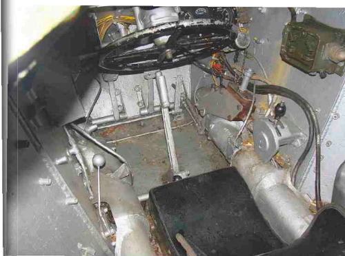
Lack of hatch glazing in Ferret makes a balaclava an essential bit of kit during winter although lots of owners retro-fit windows.
