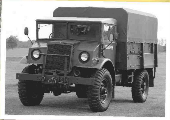
Below: Thousands of Canadian Military Pattern (CMP) trucks were produced to a common design, and with a range of bodies, by the Ford Motor Company of Canada and General Motors Products of Canada across the weight range 8cwt to 3-tons, and with 4x2, 4x4, 6x4 and 6x6 drive-lines. The photograph shows the 4x4 Ford 15cwt truck designated F15A, fitted with a general-service (GS) steel body. (Warehouse Collection)
