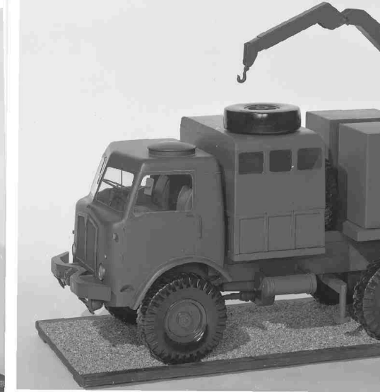
Left: The initial model for the FH70 Limber produced at MVEE. It shows an AEC Militant Mark 3 (0880) chassis carrying eight NATO ammunition pallets in much the same way the Foden would in due course. (TMB)
