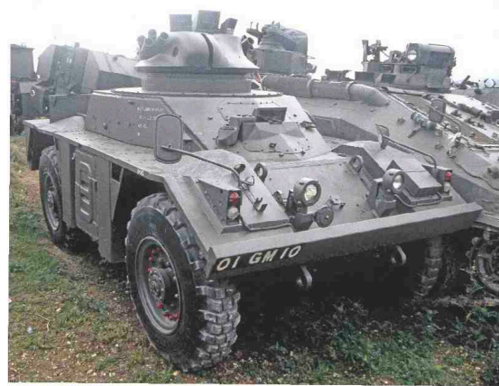
This is the Polecat, with a Peak Engineering GPMG turret fitted to a collar over the Fox turret ring. A similar vehicle was displayed at the British Army Equipment Exhibition in 1976. Note that this vehicle still has the asset code of a CVR(W) Fox stenciled on the hull side.
