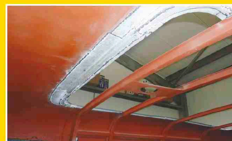
Above and below: A new channel is fabricated for the roof insert.
