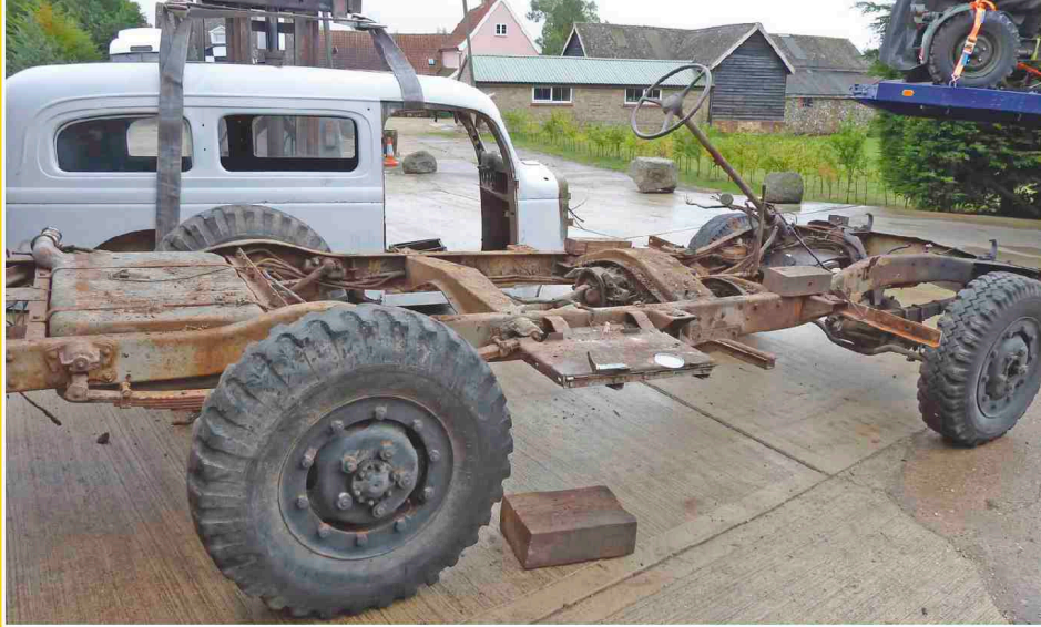
With the body off and engine removed, the chassis could be sandblasted.
