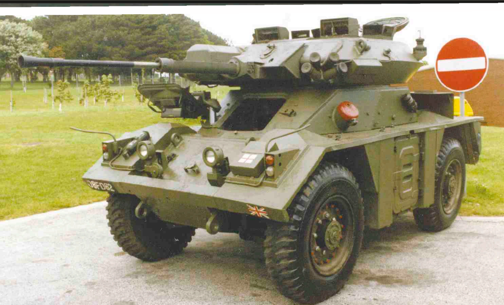
08FD62 at the Gunnery School, Lulworth, after the flotation screen was removed. This vehicle was used for instructional purposes and therefore appears rather bare.
