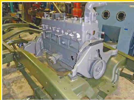
The engine required no more than new gaskets, cleaning and painting.
