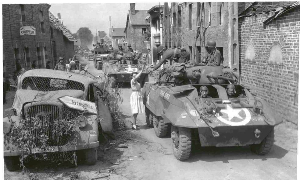
This M8 belonging to the HQ Troop of the 42nd Cavalry Reconnaissance Squadron (Mechanized) is not fitted with the .50cal machine-gun mount widely adopted. It is shown in Brehal, near Avranches, on 2 August 1944 (National Archives)
