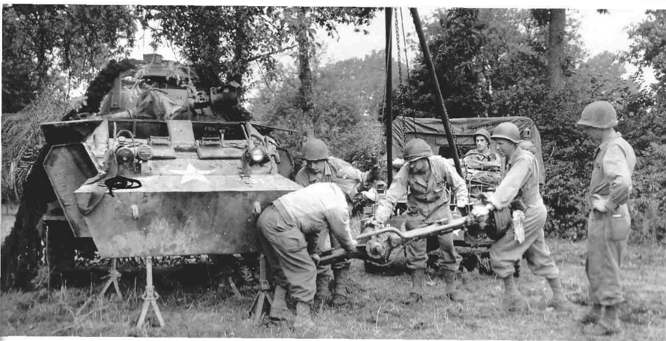
Above: Field repairs in Normandy. With the front of their M8 supported on four heavy-duty axle stands, the crew manhandle the front axle with the help of an A-frame attached to a Dodge weapons carrier. (National Archives) Below: Rows of M8s and M20s destined for the Free French forces photographed at Casablanca in October 1943. (ECPAD)
