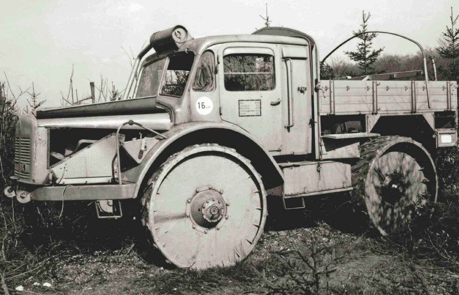
Above: An RSO evaluated by the US Army in April 1945. The air cleaner is positioned over the windscreen.
