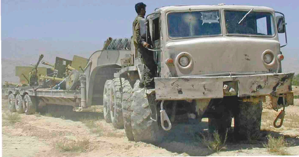
MAZ 8x8s have been equally at home in desert heat. This trailer is the 40-tonne capacity ChMZAP-5208 three-axle unit.
