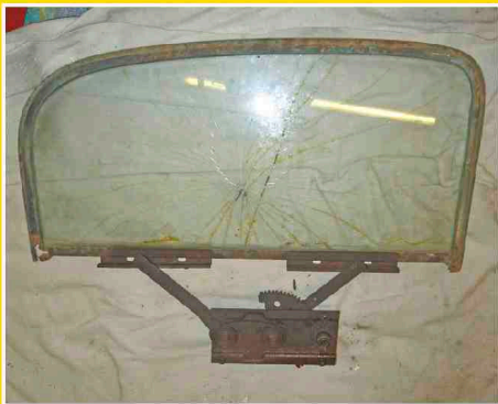
The window winders were specific to the Carryall and needed unseizing. All the glass had to be replaced.
