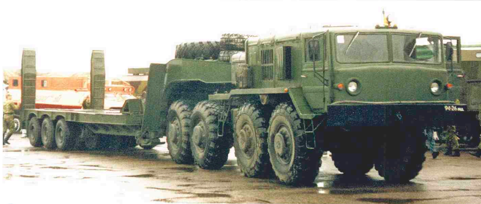
Above: The 537G tractor incorporated a winch (located behind the engine compartment) for recovering damaged armoured fighting vehicles.
