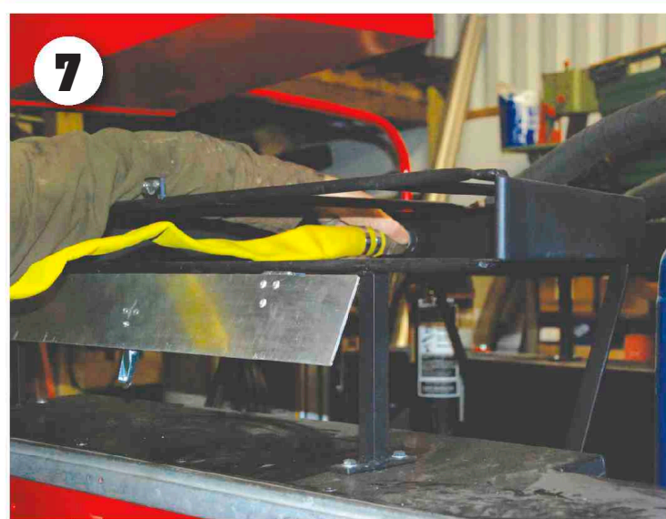
7 The hose was simply screwed onto the fitting at the rear of the rack and then folded in a serpentine fashion so that it could be run out rapidly when attending a fire.
