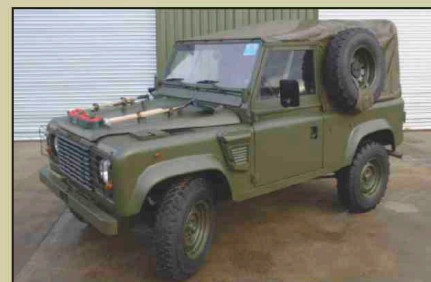
Land Rover Wolf 90 300Tdi Hard Top RHD , Fitted 300Tdi engine, 5 speed R380 gearbox, Hi/Low transfer box with centre diff lock, full FFR installation kit, 24-volt electrics, PAS, front and rear disc brakes etc, Mileage from 45110km, Guide price from £8,250 (6 Available)
