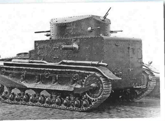
T39 viewed from the rear showing the arrangement of Hotchkiss machine guns in the turret. Compare the exhaust pipe with the one visible on the wheel-cum-track Mk I. Notice also the rear access door and the smaller side doors.
