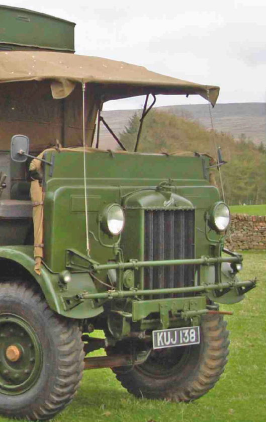
This IGL8 originally carried a Coles petrol-electric crane, but it was beyond saving so the original restorer fitted a radio body of unknown origin instead.
