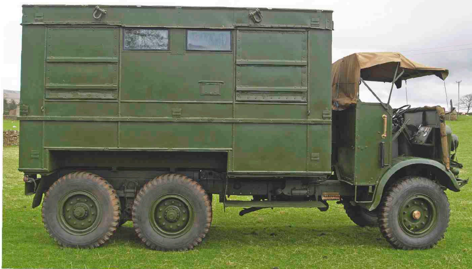
This IGL8 originally carried a Coles petrol-electric crane, but it was beyond saving so the original restorer fitted a radio body of unknown origin instead.
