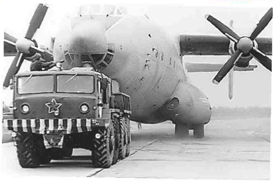
A 537L drawbar tractor for towing aircraft weighing up to 200 tonnes.
