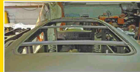
Above and below: A new channel is fabricated for the roof insert.
