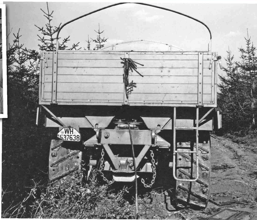
Above: This rear view shows the winch mounted under the load bed and the small spade which was lowered to anchor the vehicle when winching. You can also see holes in the wheel rim into which additional spikes could be fitted. Below: The storage box between the wheels contained additional cleats and spikes for the wheels.
