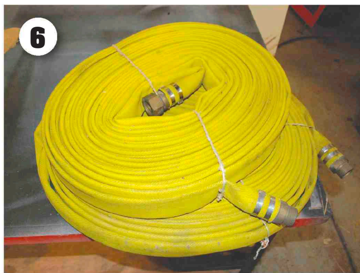
6 A Merryweather Layflat fire hose ready for fitting. The hoses were obtained via contacts with the Museum of RAF Fire-Fighting at RAF Scampton.
