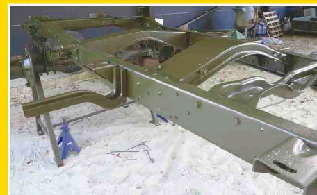
Five hours of sandblasting, three coats of red oxide and several of olive drab later...
