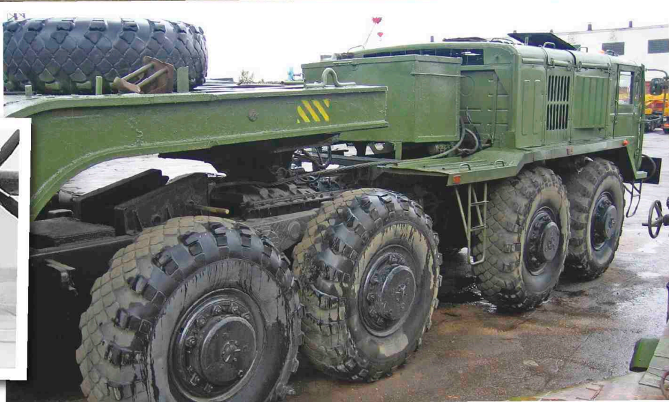
MAZ 537 tractors typically hauled 50-tonne two-axle, 40-tonne three-axle or 60-tonne four-axle trailers.
