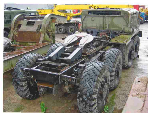
With a springless equaliser suspension system, the rear bogie of the fifth-wheel 537 tractor has a capacity of almost 30 tonnes.
