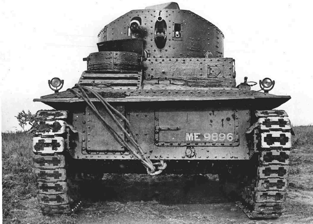
A Medium Mk IA later in life, having become a Mk IA*. The Hotchkiss guns have been eliminated and replaced by another water-cooled Vickers alongside the main gun, complete with a box to catch spent rounds. Up on top of the turret you can just make out the upper part of a 'bishop's mitre' cupola. Notice also, low down in the front of the hull, the location for the starting crank handle.
