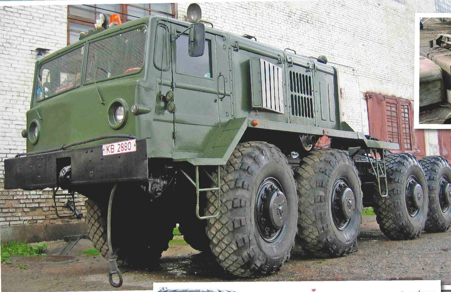
Above: Produced by the thousand, the MAZ 537 was the world's first heavy military semi-trailer tractor with independent suspension.
