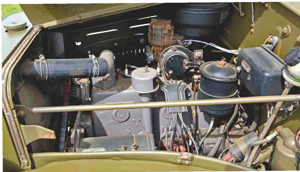
A Plymouth P20 engine from the fifties has replaced the original Dodge T214.
