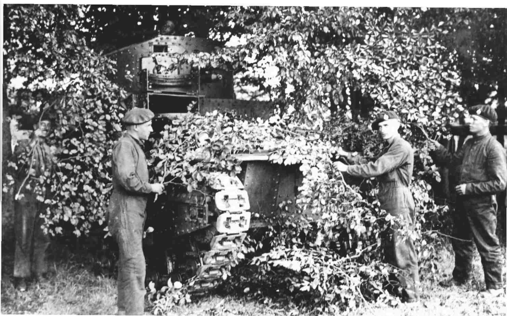
This photo shows a Mk I being camouflaged by its crew during an exercise. However it gives us an excellent view of the way that the driver's hood opens up. Just visible above it is one of the air-cooled Hotchkiss machine guns in its mounting.
