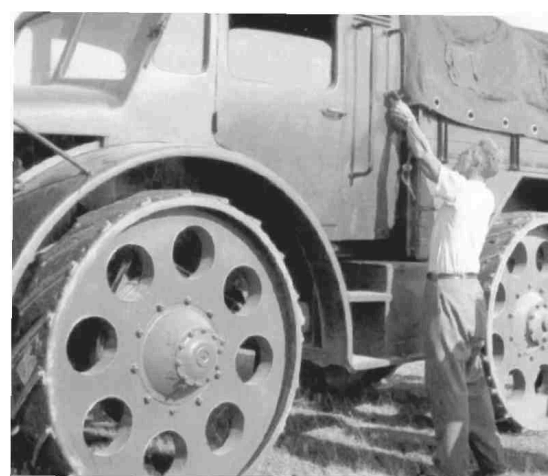
Above: This is the prototype Type 175 RSO. Photos show that in addition to the solid wheels fitted to the RSO examined by the US Army, there were also perforated (as here) and spoked types used.
