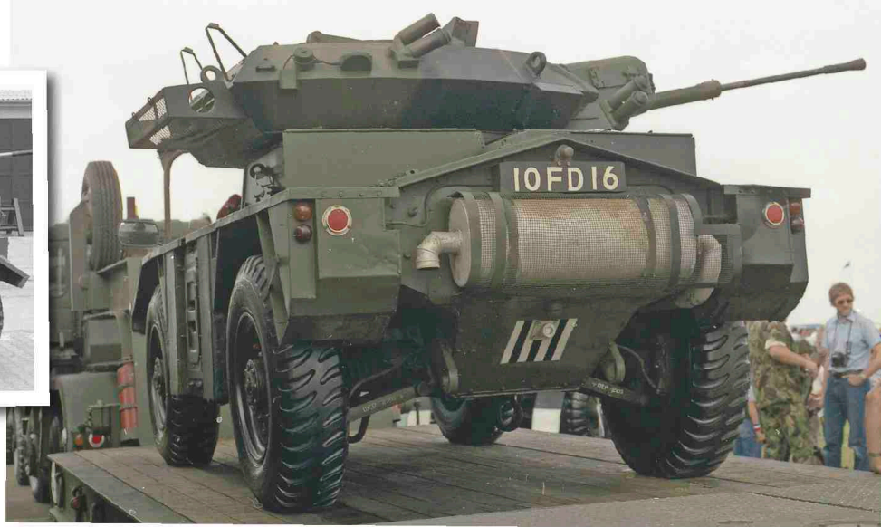
Above: This photograph gives a good view of the suspension arms and the rear exhaust. The vehicle was with the Infantry Display Team at IAS Middle Wallop in 1986. (FMW)
