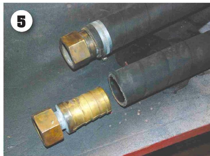
5 The hoses are made up of lengths of coolant hose fitted with BSP (British Standard Pipe) threaded couplings at the ends. They were then secured in place with jubilee clips.
