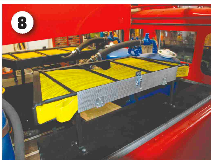
8 The finished racks complete with hoses. So far the correct powder nozzles that attached to the end of the hoses have not been found, so the hunt for these elusive pieces of equipment continues. Note that the rear quarter-light windows in the cab are still to be fitted.
