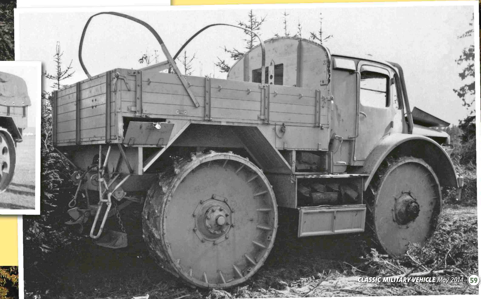
Above: This rear view shows the winch mounted under the load bed and the small spade which was lowered to anchor the vehicle when winching. You can also see holes in the wheel rim into which additional spikes could be fitted. Below: The storage box between the wheels contained additional cleats and spikes for the wheels.
