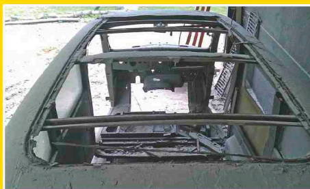
The original canvas and Masonite roof insert had been replaced by a metal panel welded and screwed in.
