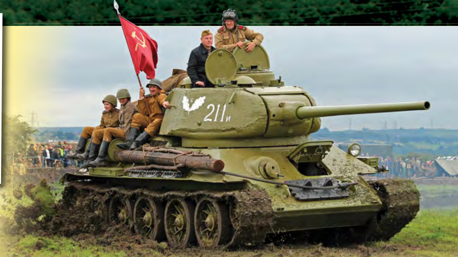
Above: Nearly 30,000 examples of the T34-85 were produced between 1941 and 1945, with this example being one of the later models rolling off the production line in Gorki as the war drew to a close. Following WW2 it spent time in Eastern Europe, being found in Czechoslovakia and imported into the UK in January 2013. This example of the T34 carries a 85mm gun and is powered by a 38-litre V12 engine. Below left: Blink and you may have missed it but it was good to see this Austin K6 flatbed tucked away in a corner of the show field. Bottom: Making one of its last appearances in the UK before being purchased by an Eastern European collector was Rick Wedlock's 1944 MK6 Cromwell. Rick started the restoration in 2011 and spent just 18 months transforming it from a wreck to show-stopper. He decided to sell it in order to finance new projects.
