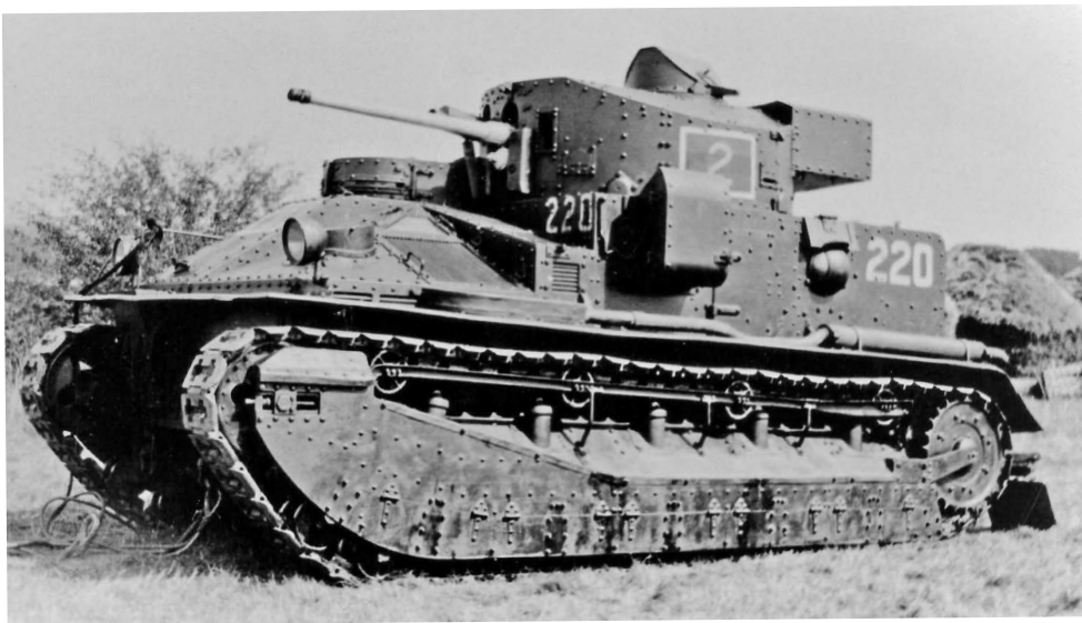
A Medium Mark II** showing the wireless extension on the back of the turret. When the gun was painted white it was normally meant to represent a Close Support tank on an exercise.
