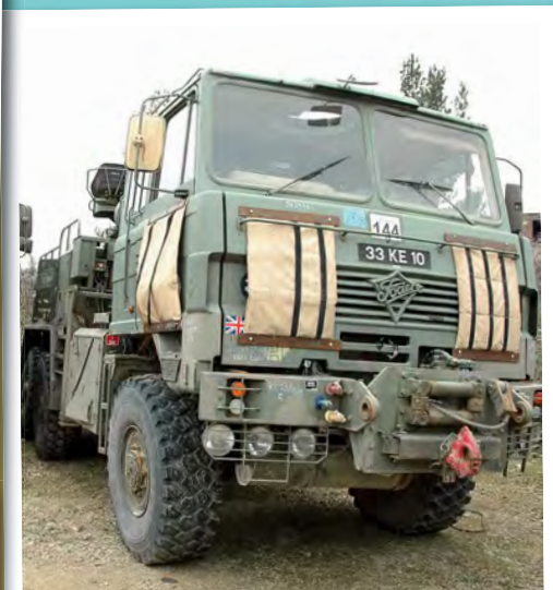
Prior to the application of officially developed and purpose-built add-on armour, some vehicle crews attempted a few DIY fixes using MAPIK panels to give themselves a little extra protection while serving in Iraq and Afghanistan.
