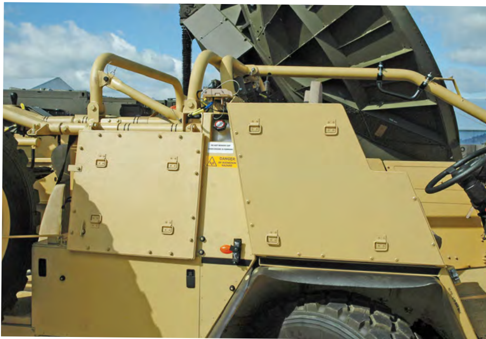
Open top vehicles being used in Iraq and Afghanistan required additional protection. These are the composite armoured door panels on a Supacat Jackal.
