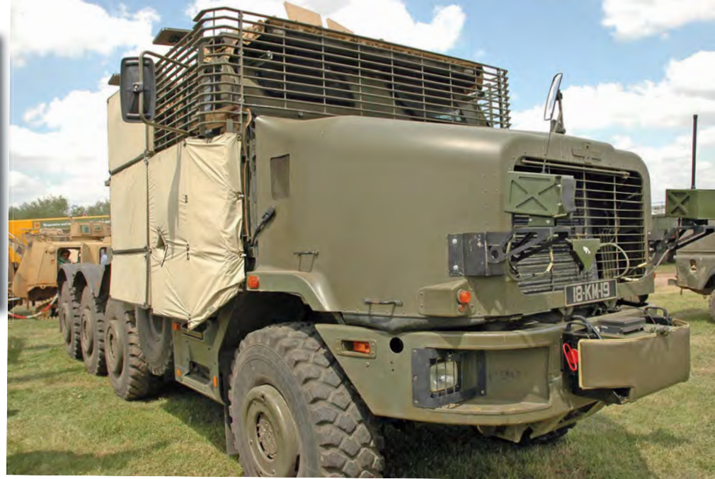
Softskins are always going to be more vulnerable to attack and the MAPIK armour system saw several development phases before being introduced on a wide range of vehicles, including this Oshkosh HET tractor unit fitted with MAPIK panels.
