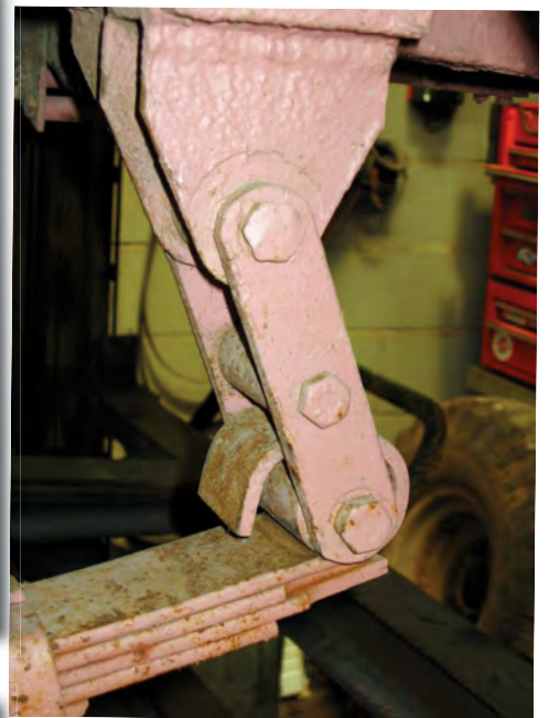
To give clearance for the large tyres, the Marshall's-built Pink Panthers had heavy-duty 'drop shackle' suspension.
