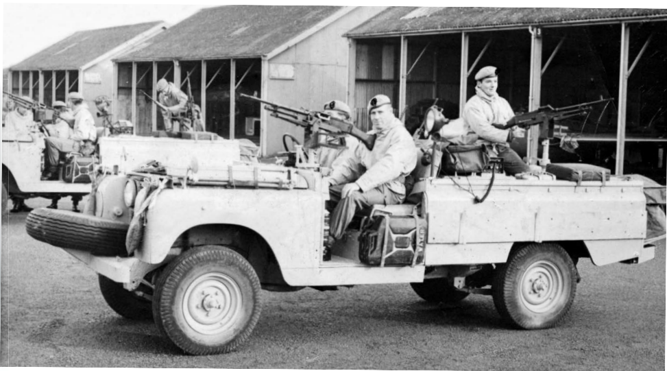
This is a unit-converted 'Pinky', dating from the mid-1960s. There are several differences from the later standardised models; note the absence of smoke grenade launchers, for example.
