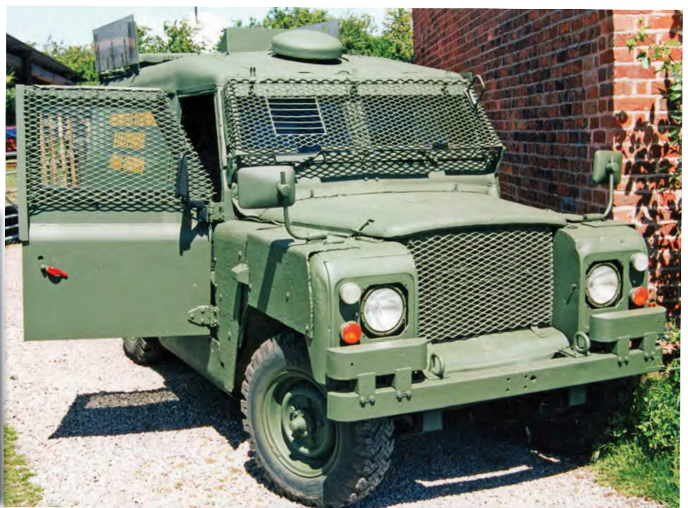
As the paramilitary factions started to use higher velocity weapons the VPK Land Rover was developed further. This is the HVVPK or High Velocity Vehicle Protection Kit Piglet, which saw many of the GRP panels being replaced by armoured steel panels.
