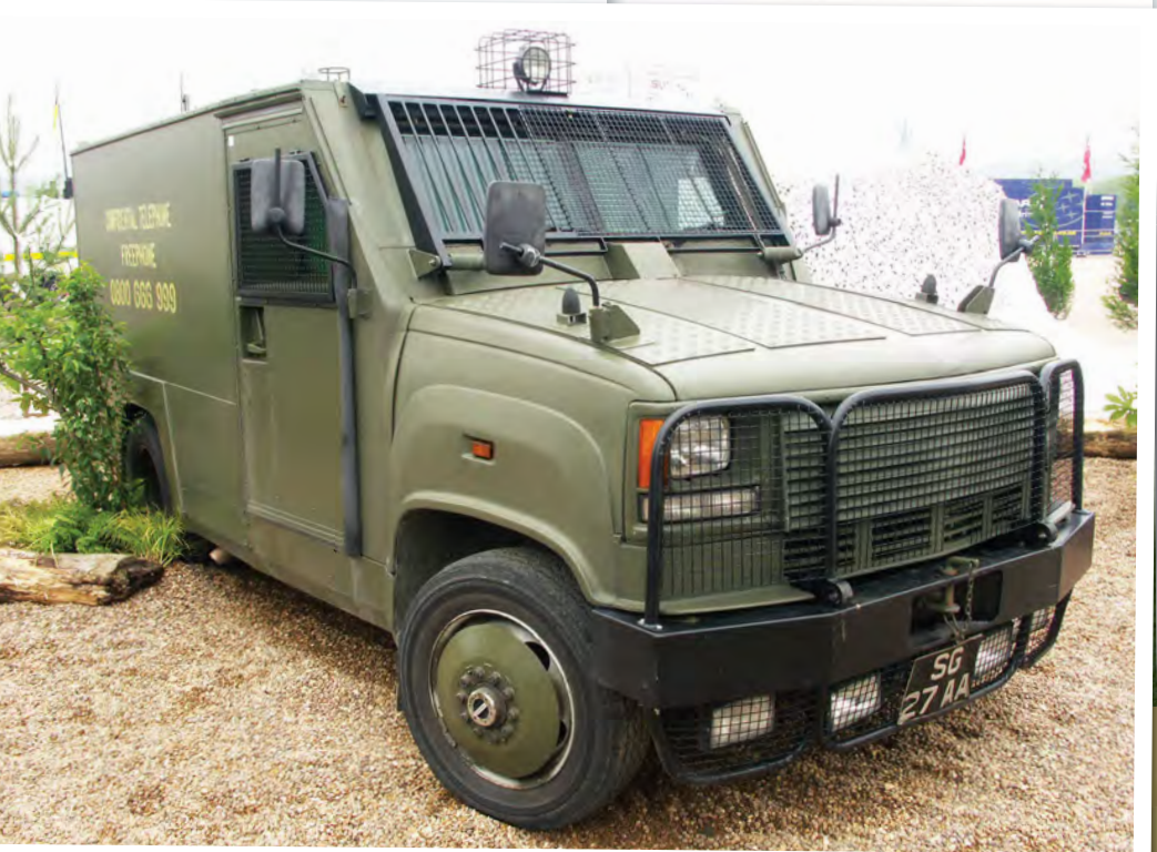
The Tavern Armoured Patrol Vehicle was used in Northern Ireland as a replacement for the older VPK Land Rovers. It had a much higher level of protection, but the base vehicle used was not ideal.
