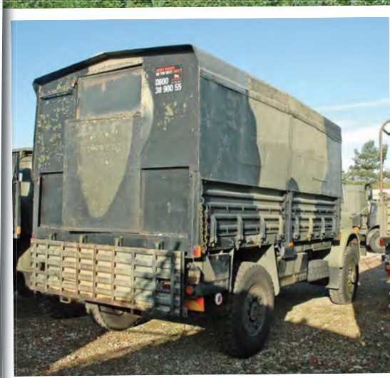
Here, a Bedford 4-tonne truck has been fitted with a protected rear cargo area.
