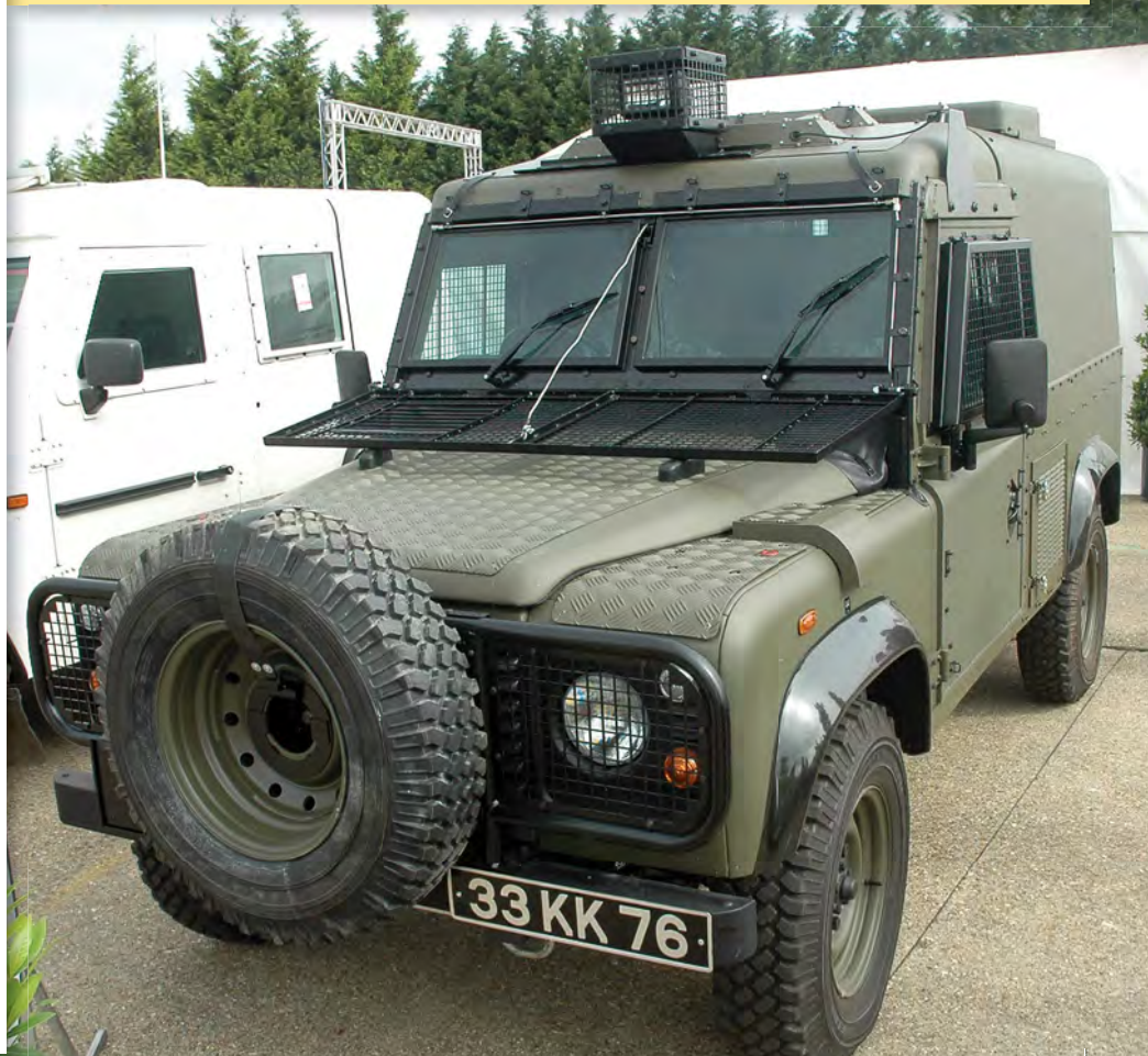
Below: The CAV-100 was developed by Courtaulds and used a new type of moulded GRP armour. It went on to serve in Northern Ireland as a replacement for the VPK Piglets.
