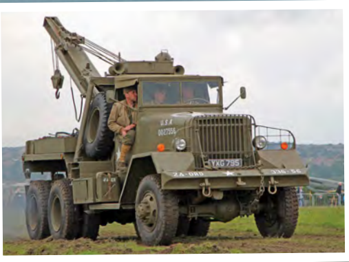
Above: This Ward La France M1A1 Heavy Wrecker is owned by Graham Booth and 2015 was the first time that it had been out on the circuit following restoration. Introduced in 1943 in order to supersede the earlier M1 series, the 5-tonne boom swing crane was installed in order to recover tanks and most heavy vehicles. Right: This may well be a post-war Czechoslovakian OT810 version from the 1950s but in essence it is the same design as the German built Sd. Kfz 251s that were produced in over 20 different varieties. The post-war version, such as this one, was fitted with a diesel engine and had other subtle changes.
