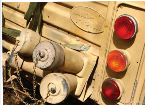
... and these are the smoke grenade launchers, also seen on the Marshall's-built Pink Panthers.
