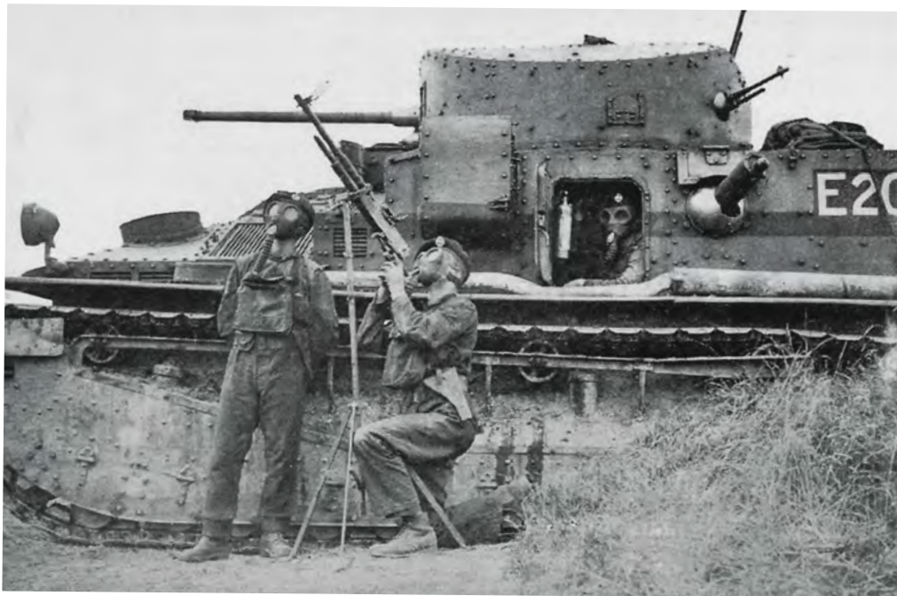
A Medium Mark II in 5th Battalion service, still painted in Mechanized Force colours and the crew wearing gas masks, posing with a Hotchkiss gun mounted for ant-aircraft defence.
