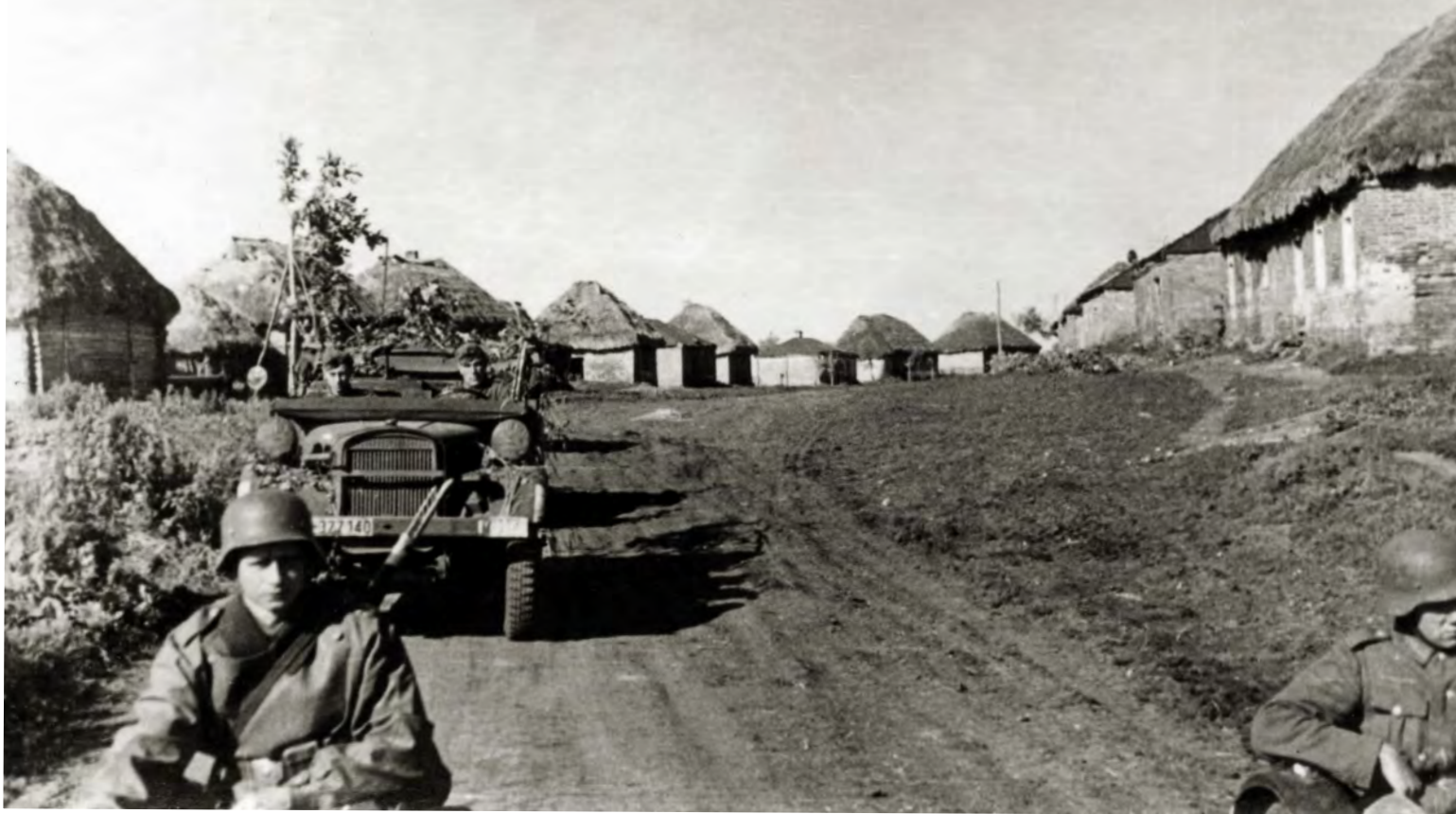
German Army motorcycles and Kübelwagen are seen here on a road passing through a typical village in the Soviet Union. The weather is dry, and the hard-packed black earth of the road through the village provides good going. The leading Kübelwagen is a Light Cross-country Car (leichter geländegängiger Personenkraftwagen) as built by BMW, Hanomag and Stoewer from 1936. The original design featured four-wheel drive and four-wheel steering. However, the latter was an absurd over-complication, and from 1940 it was dropped. From this year only Stoewer built the car, and the example seen in the photograph is a Stoewer Typ 40.
