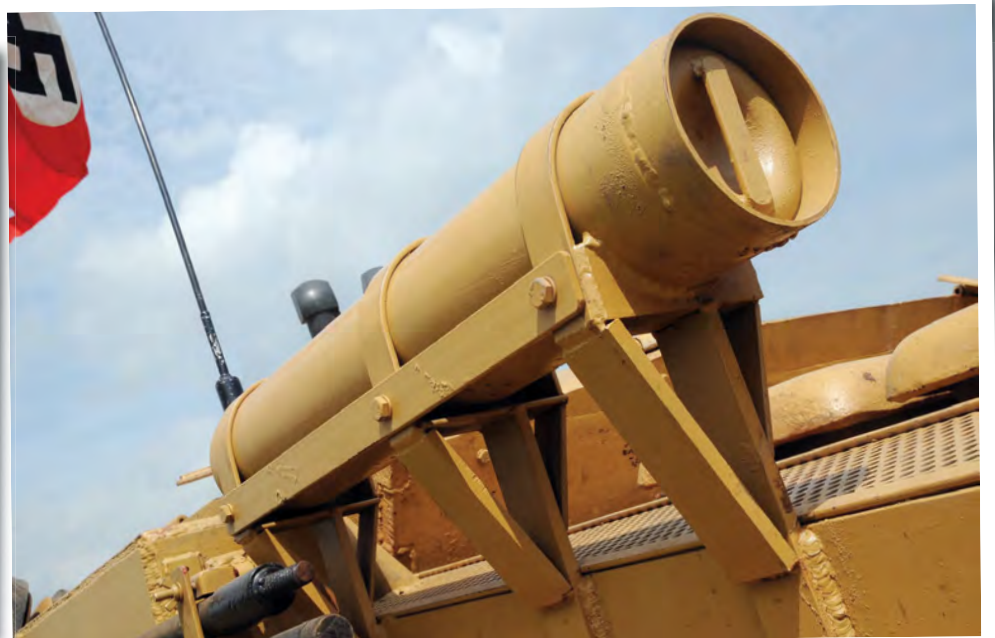
Tropical fittings included additional pre-cleaning filters, additional air intakes cut into the deck access hatches and fuel/water can racks mounted across the rear engine deck.
