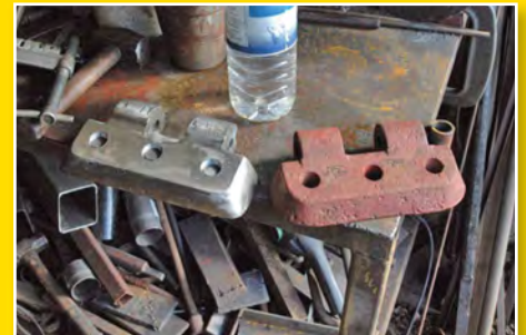
Above: Jon couldn't get the original cast steel hinges so made some himself.
