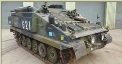
Alvis Stormer Tracked Armoured Recon Vehicle , Fitted Perkins 6-litre, 6-cylinder, Crew: Driver, Commander plus 2 pax, year 1992, low mileage, Excellent condition, ..... Guide price from £12,500 (6 Available)
