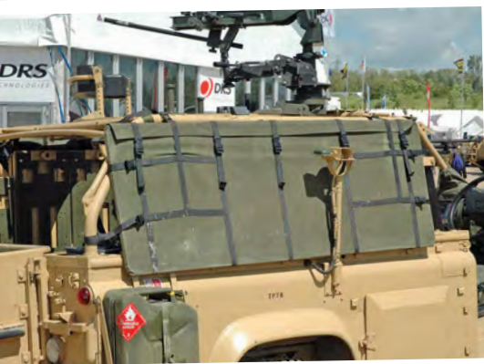
Earlier attempts to provide some sort of crew protection on the WMIK came in the form of MAPIK armour, which took the form of soft panels strapped to key areas of the vehicle.
