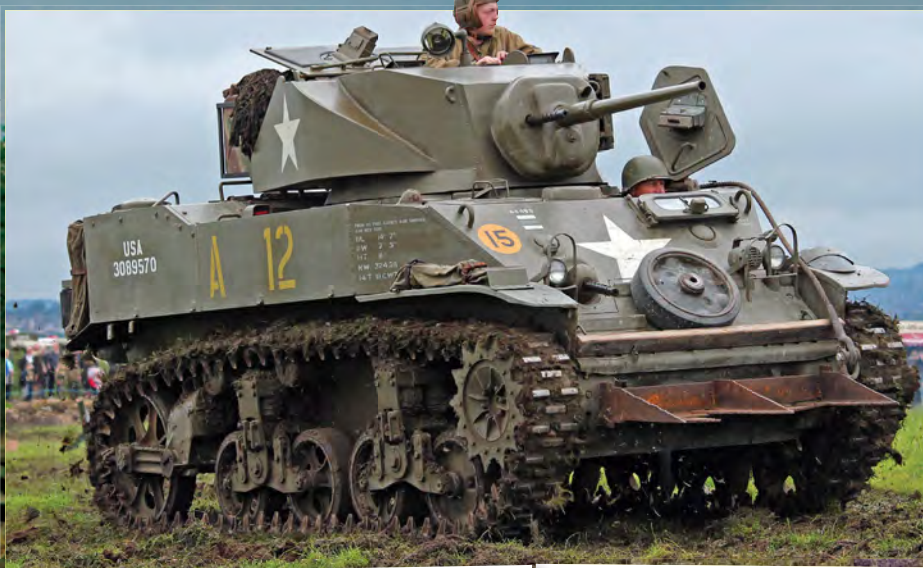
Above: One of the show organisers, Nelz, hitches a ride around the arena on this Diamond T hard cab 969 variant. Left: The M3A1 tank was first used in November 1941 in North Africa, being known as the Honey by British forces and the Stuart by the US Army. It is powered by two Cadillac V8 engines.
