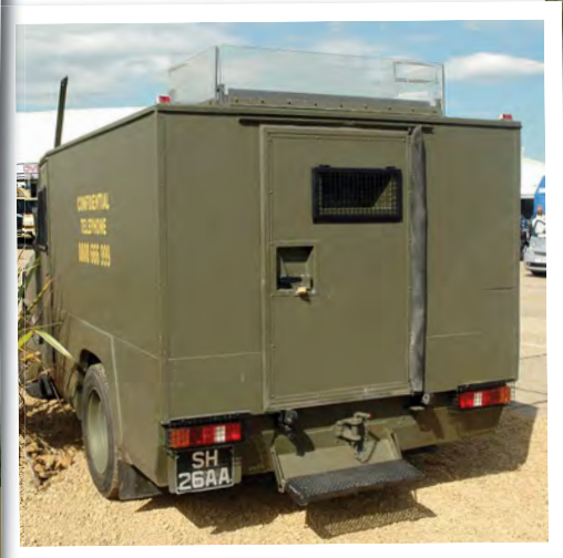
The Tavern Armoured Patrol Vehicle was used in Northern Ireland as a replacement for the older VPK Land Rovers. It had a much higher level of protection, but the base vehicle used was not ideal.
