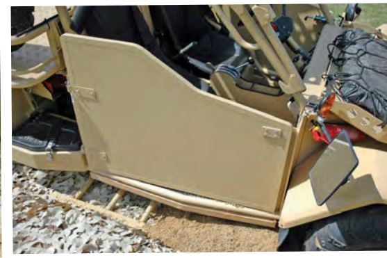
Above: Close-up of the composite armour door panel on a Springer. Additional panels were positioned behind, in front of and below the crew compartment.
