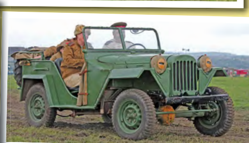
Above: The Gaz 67 was a Soviet manufactured vehicle which was influenced by the American built Bantam and Willys Jeeps and a development of the earlier designed Gaz 64. Only 718 Gaz 67s were built between September 1943 and January 1944 before the Gaz 67B was introduced.
