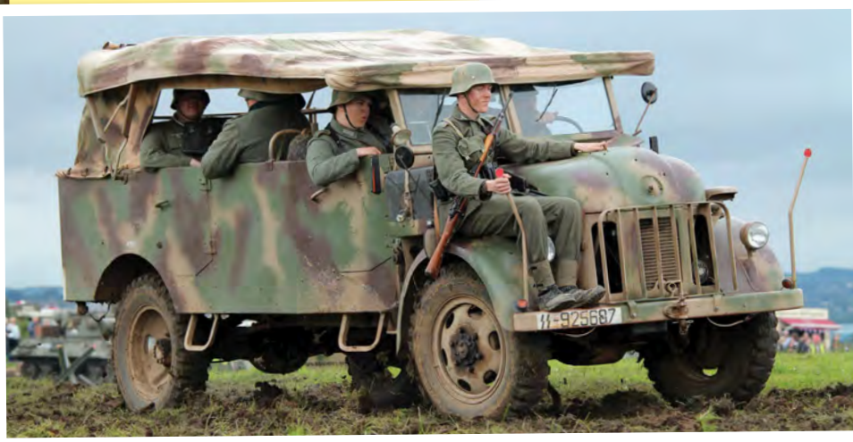
Above: Steyr built some 12,450 examples of the Steyr 1500 A from September 1941 to March 1944. It was able to carry a crew of eight men and due to its high ground clearance proved to be popular for both desert and off-road use. Right: Various battle scenarios took place at the end of both days. Below: Among the differing and interesting variants of Diamond Ts on show was this 972 Dump Truck.
