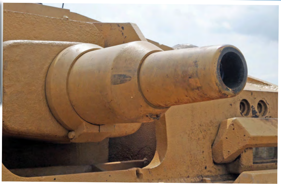
Above: Parts were acquired from as far afield as Poland, Latvia and France. Right: Gun is the 75mm short barrel as used in the Panzer IV. Above it to the left there are two holes, which are range damage, while below it is another hole (visible here) made by a Piat.
