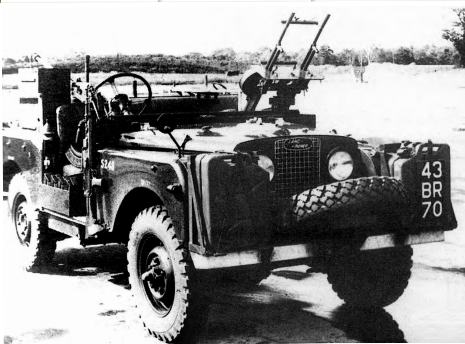
The prototype 'standardised' SAS short-wheelbase Land Rover was evaluated by FVRDE. It was converted from a standard 86-inch Mk 3 model.
