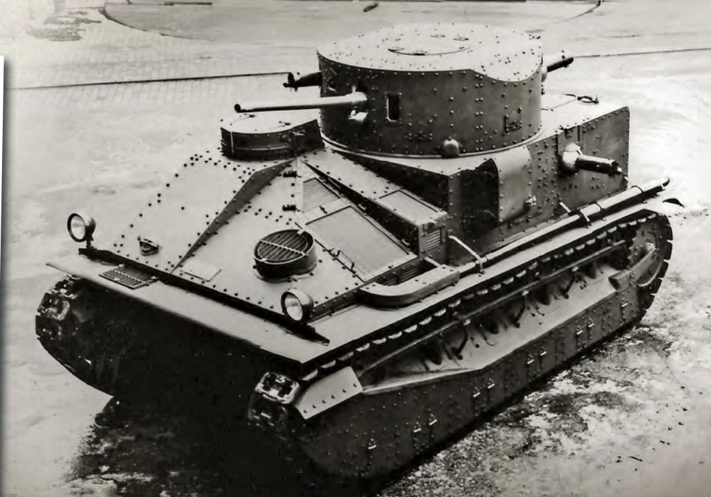
Above: Photographed at Vickers, Newcastle, one of the tanks supplied to Russia. The turret is identical to the one supplied to Australia but it's running on a Mark IIA hull. Only this one, we think, carried a three-pounder gun.
