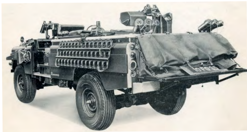
This rear view of 10 FG 35 shows the drop-down shelf at the rear, the sand channels, and the sand tyres (on 15in wheels rather than the standard 16in size used on Land Rovers).
