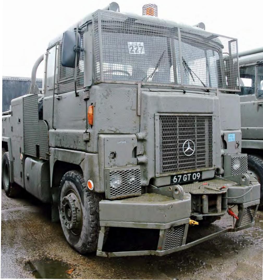
The combination of the GRP panels and steel mesh provided a reasonable level of protection for the crews, but only from low-velocity weapons, smaller blast bombs, bricks and bottles.
