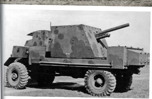
Above: A rear nearside view of a Deacon painted in camouflage colours. Notice the narrow driver's cab and the huge shield for the gun, almost a turret but open at the back and on top.
