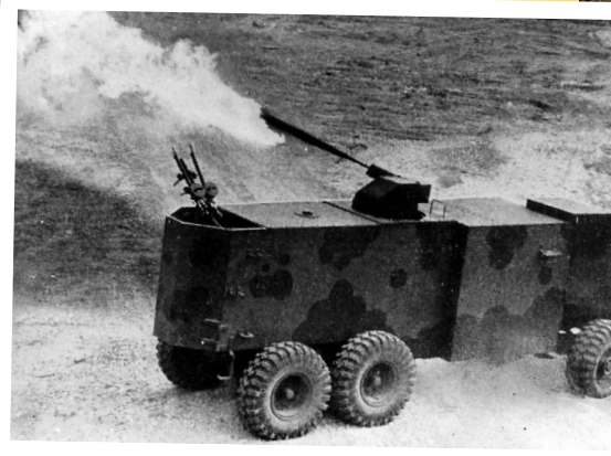
Below: The Cockatrice Mark IA which was built for the RAF on the AEC 6x6 chassis. A Spartan looking vehicle but note the two machine guns at the back for anti-aircraft use. They were never used in action because the Germans never landed.
