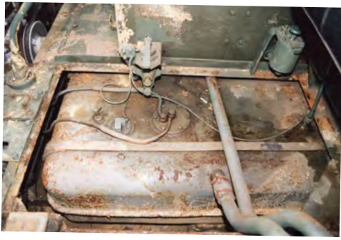
Above: Two diesel tanks are fitted, both beneath the seats in the cab. Here we see the left hand (driver's side) tank. Also visible is the tap (top centre) to change between the two tanks and the electric isolation device (top right). Right: The replica body finished off what was an already nice (and unusual) vehicle, not to mention very rare in private hands in the UK.
