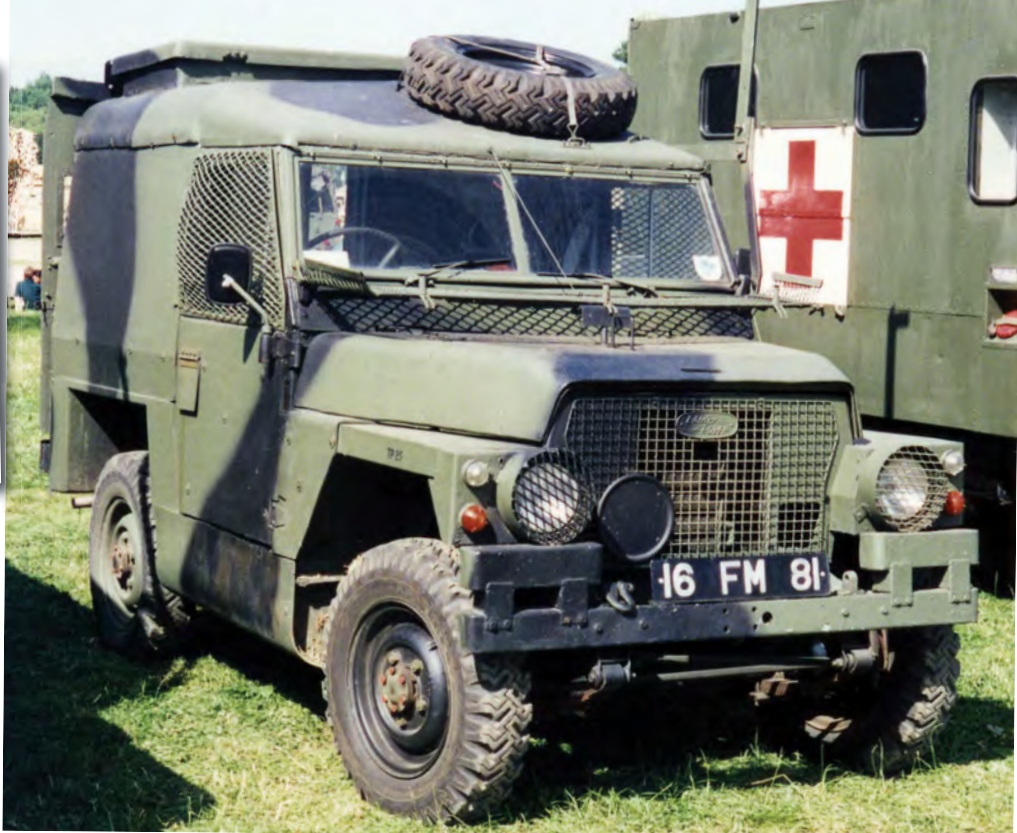
Many Lightweights that served in Northern Ireland were fitted with a VPK.
