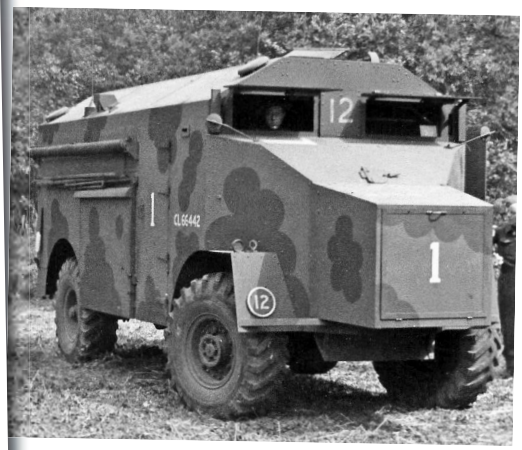
A version of the High Power Armoured Command Vehicle with an unusual nose on the front end.
