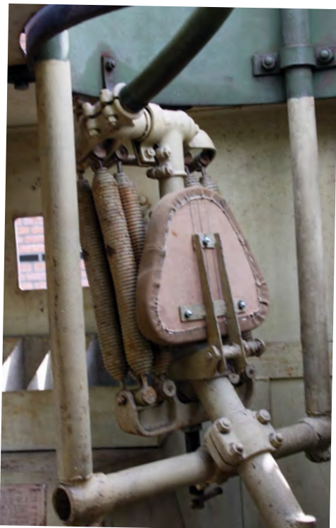
Gunner's seat helpfully tips up when not in use.
