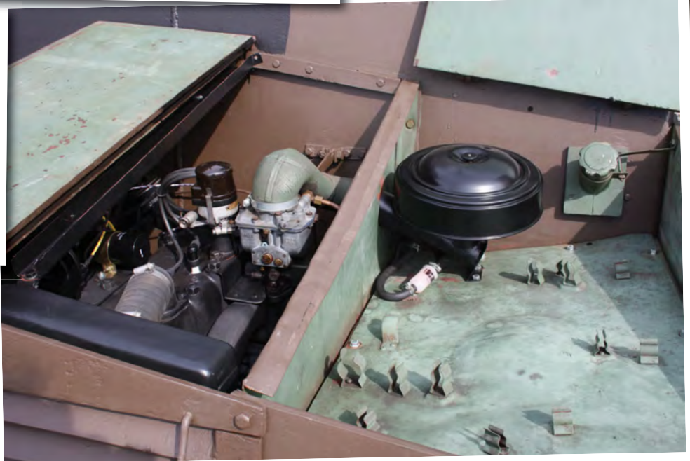
Below: Low bonnet means air cleaner has to be relocated elsewhere.
