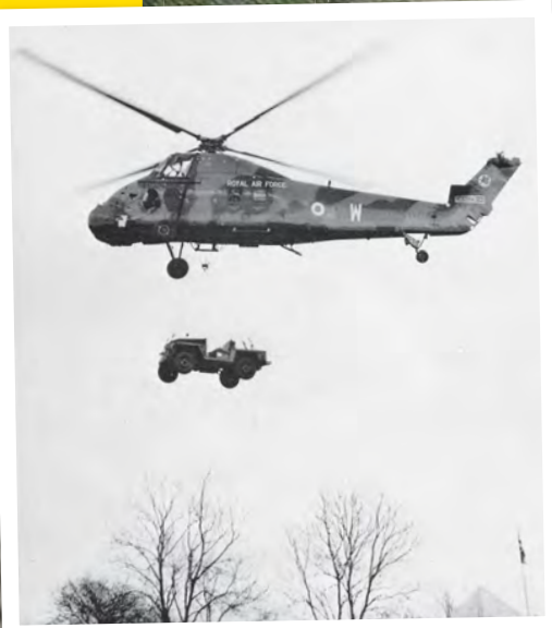
Above: The need for helicopter lifting was a major factor in the design of the Lightweight. Right: Not many Lightweights wore RAF colours, but they looked good when they did.
