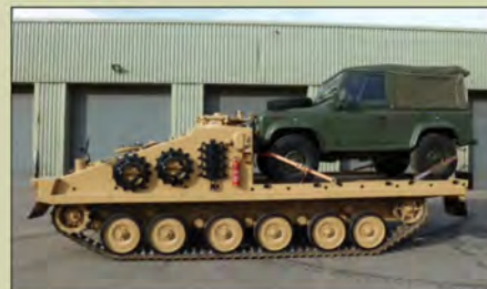
Alvis CVRT Shielder , Tracked Armoured load carrier with flat bed platform, The flat bed can be adopted for a wide range of roles such as logistic carrier, bridge layer repair / recovery and towing. Built to a high specification the vehicle hull is composed of aluminium armour to protect the crew, etc, Mileage from 500, Excellent condition, Guide price from 12,500 (4 Available) .
