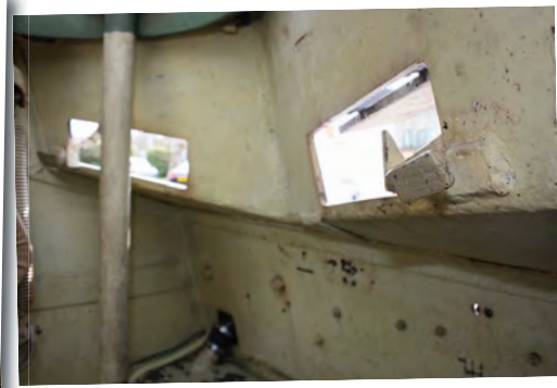
Above: Forward visibility for the driver is surprisingly good but becomes severely hindered when the dual front slots are closed. There's also a vision slot each side.
