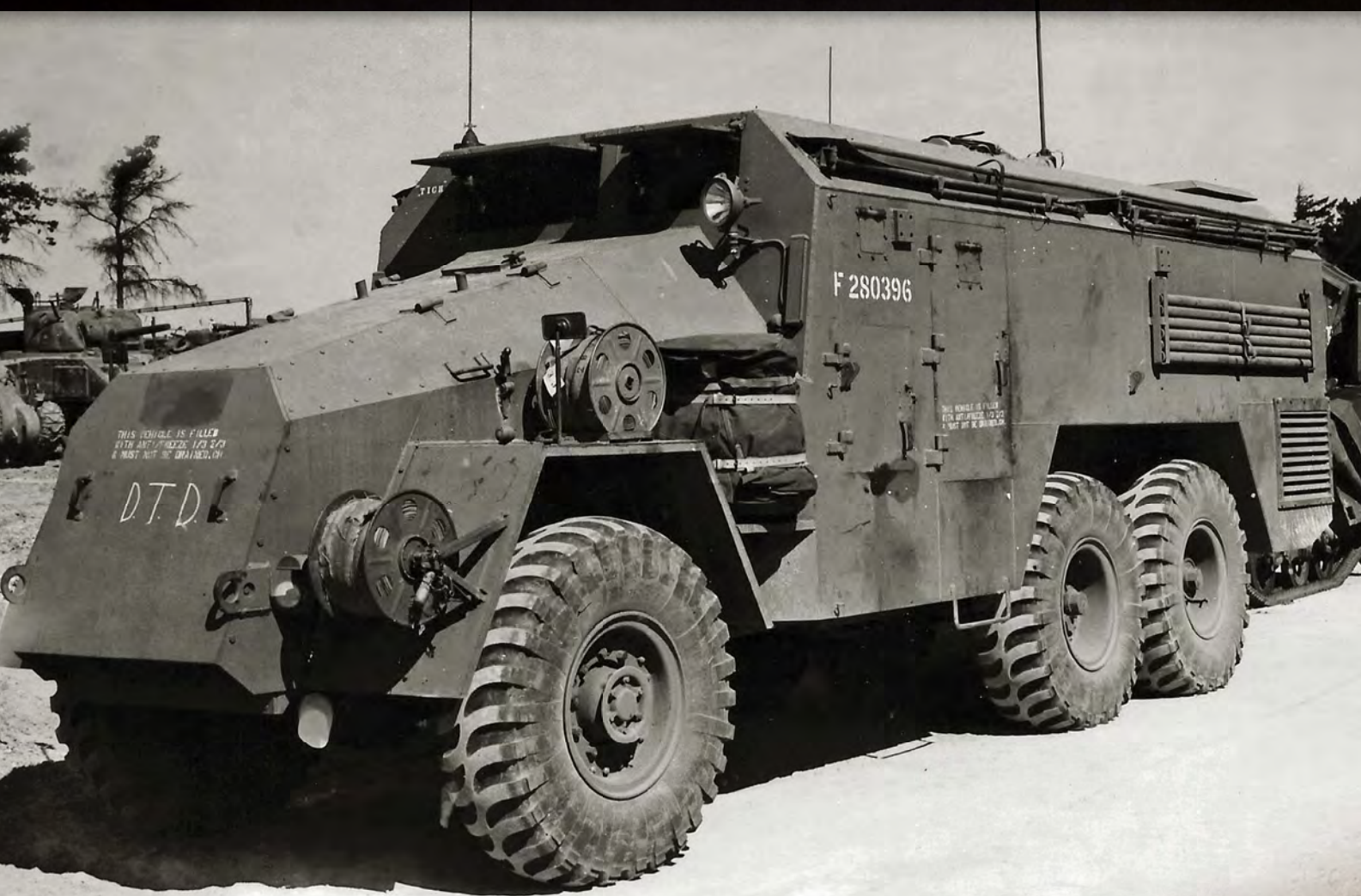
The AEC 6x6 Armoured Command Vehicle Mark I, shown with two cable reels on the nearside front mudguard. Notice the folding frames for extension tents on the roof.
