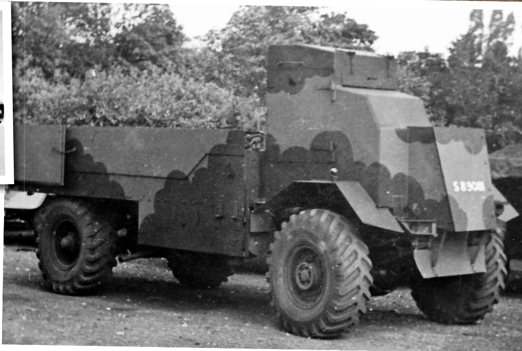
Right: The AEC Armoured Ammunition Lorry was based on the Matador but developed from the Deacon. Were they ever used?
