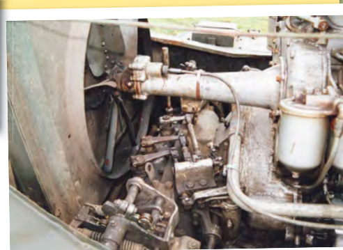
The engineering is 'agricultural' and typical of Russian-built vehicles of the time. The series of rods visible here are the gearbox linkage controls.
