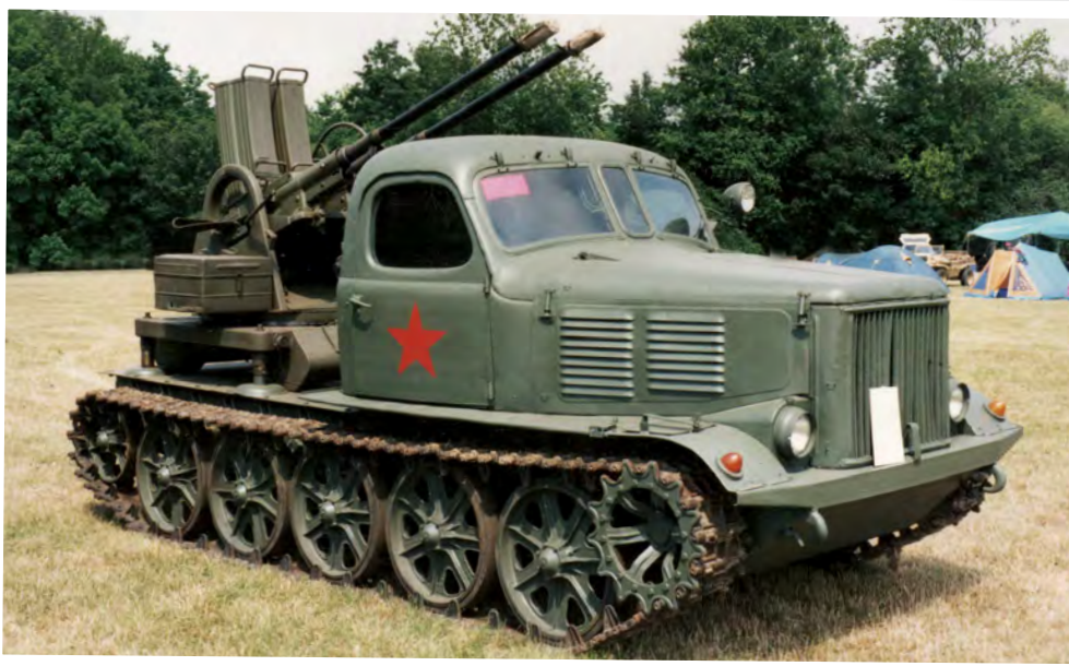
Above: Prior to Ian purchasing the AT-LM it had been owned by R&R Services in Kent, who fitted this twin barrel anti-aircraft gun to the back, though in reality it was never configured in this way while in service. Right: While checking oil levels Ian found to his surprise that the gearbox was filled with a pungent red grease, and having consulted other Russian vehicle owners he was told that it was made from whale blubber and was used rather than oil to prevent the gearbox freezing in the extreme temperatures of Siberia!
