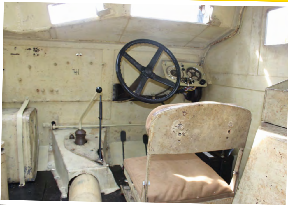
Above: Forward visibility for the driver is surprisingly good but becomes severely hindered when the dual front slots are closed. There's also a vision slot each side.
