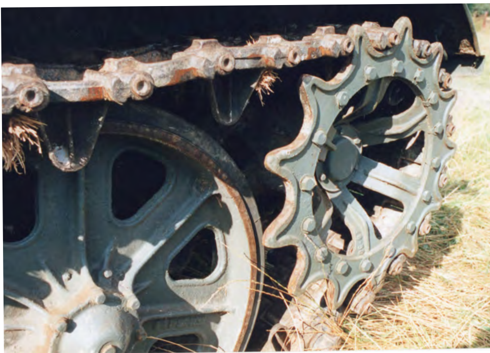
Unlike most Western-designed tracked vehicles, the AT-LM has twin guide horns that straddle either side of single roadwheels.
