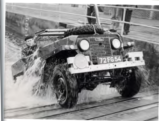
Above: The first 1500 or so Lightweights had headlights in the grille panel, like this one. Left: A full stripped-down Lightweight looked like this, although the vehicles were rarely seen in this condition.
