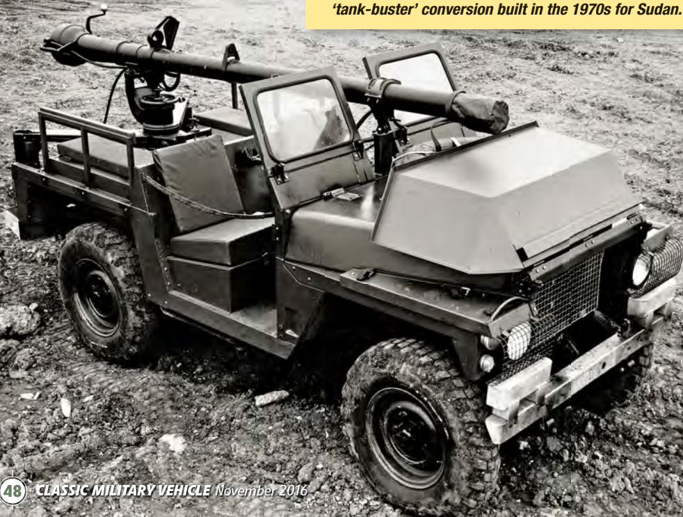
Below: There were several overseas customers for the Series III Lightweight. This was a Marshall's 106mm 'tank-buster' conversion built in the 1970s for Sudan.
