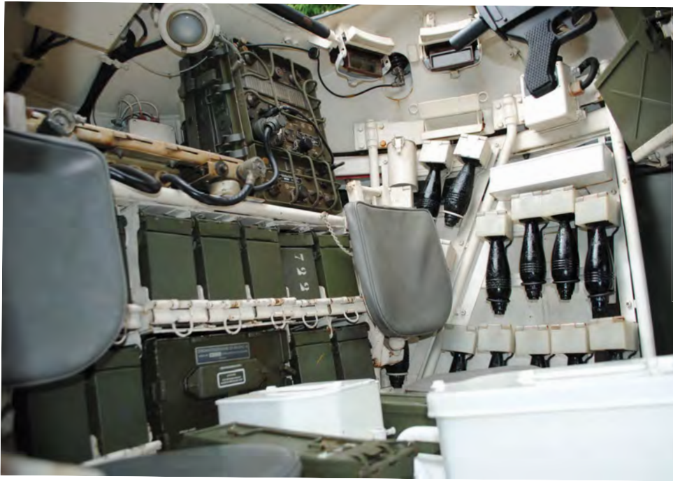
Above: The ammunition and radio inside the Panhard AML 60. Above right: Looking down into the interior of the AML 60. Right: Driver's position inside the Panhard AML 60 armoured car.
