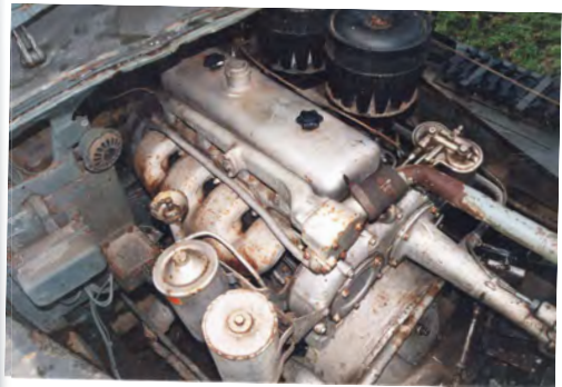
Above: The Ya-MZ-204-VKr engine is surprisingly quick, and while it was a lovely engine when running, it was a pain to get started in the cold winter months, mainly because Ian never mastered the complicated cold starting devices fitted to the engine. Right: Having driven the AT-LM around a fairly extreme off-road course at a quarry Ian can testify to the superb off-road ability of the vehicle – when he's not picking up rocks in the tracks that is!
