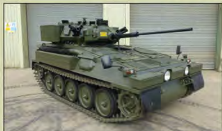
CVRT Scimitar Armoured Reconnaissance Vehicle , Fitted Cummins BTA 5.9lt Turbo diesel, Automatic Gearbox with Neutral turn capability, Maximum road speed 72 km/h, Range 750 km, etc, 820 miles, Excellent condition, Guide price £39,995 (1 Available)
