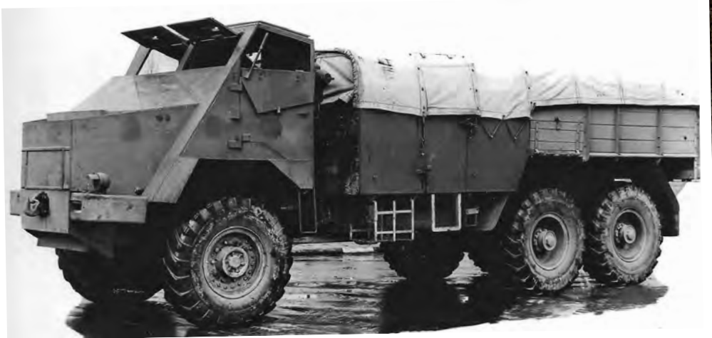
Top: The massive AEC 6x6 Armoured Gun Tractor which is thought to have been selected to tow the big 32 pounder anti-tank gun. It was never developed beyond the prototype stage.
