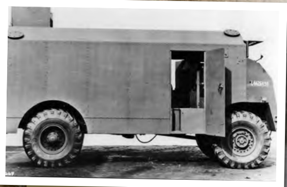
Above: The Armoured Demolition Vehicle version of the Dorchester showing the roof hatch through which a pile driver could be operated.
