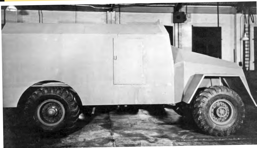
The mock-up of the proposed second version of the Matador Armoured Command Vehicle. Notice how the front end resembles the bonnet of the 6x6 version.
