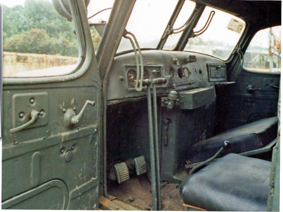
Above: One of the cold start devices involves putting a highly volatile mixture into this pump and by pumping the knob to the right you squirt the mixture into the engine. Ian tried it with Easy Start and it worked a treat on cold mornings! Right: Looking inside the cab from the driver's side we see the steering tillers, conventional clutch, brake and accelerator pedals and the rudimentary interior of the cab.
