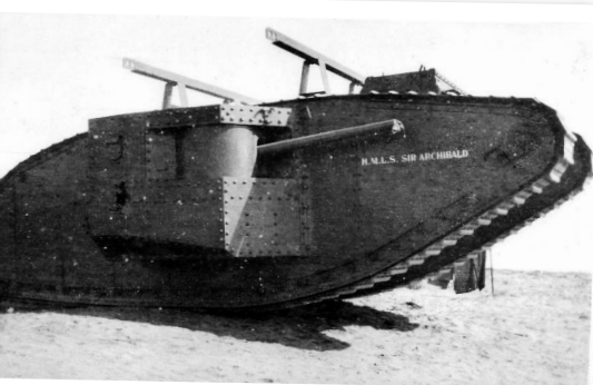
Above: The Mark I male tank 'Sir Archibald' named after General Sir Archibald Murray, photographed at Gaza. The gantries on top are used to lift off the sponsons for rail travel.
