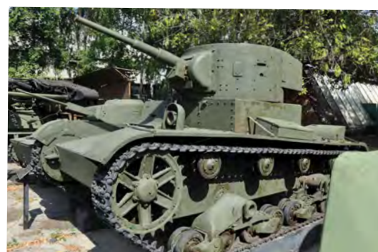
Below: The collection's 'standard' T-26 M-1933 is nothing of the sort. It is actually a TU-132 command vehicle for a tele-tank system, converted back to line tank status.
