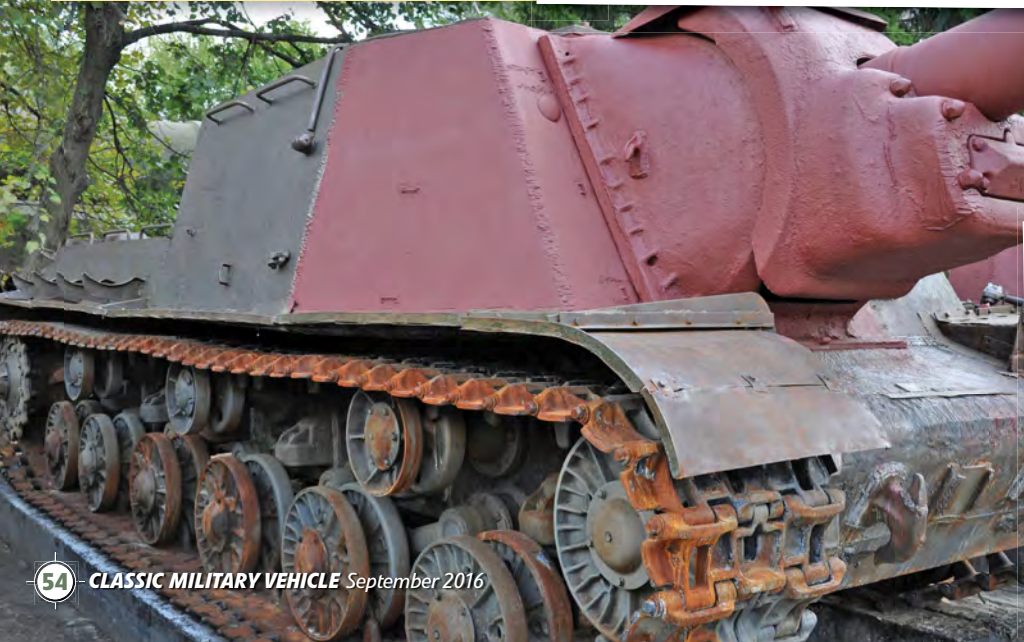
Above: This particular IS-2M also has a modified glacis with additional water sealant mounting points installed. Below: The museum's wartime ISU-152 showing the bare-metal restoration as a work in progress.
