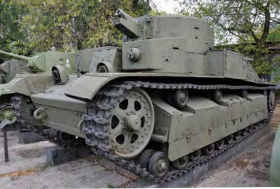
The T-28 medium tank is in poor condition, with the sheet metal track guards and other thin metal components requiring replacement.
