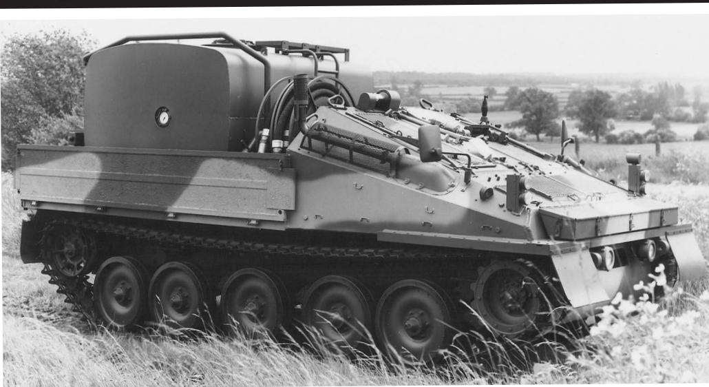
Above: The Streaker fuel tanker version could refuel vehicles in the forward areas in an emergency. Right: The fuel tanker version of the Streaker was a good idea from the logistics point of view.
