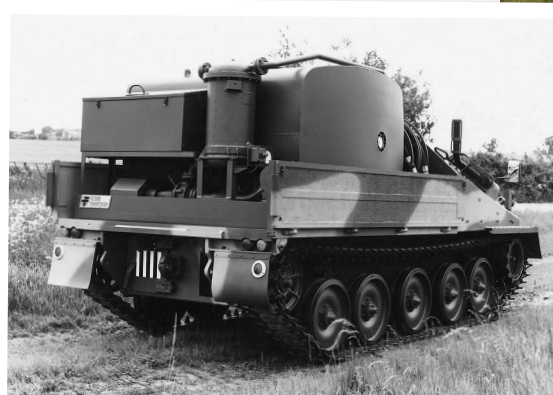
Streaker fuel tanker version could transport petrol or diesel.
