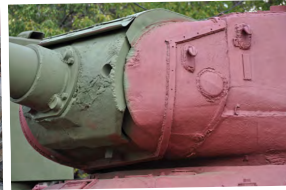
Above and below: The museum's IS-2M is also not a standard tank. It was modified for trials of OPVT-type deep-wading equipment in the early 1950s. The metal strips added to the gun mantlet, for affixing rubberised fabric waterproofing, are an obvious clue to the tank's non-standard history.
