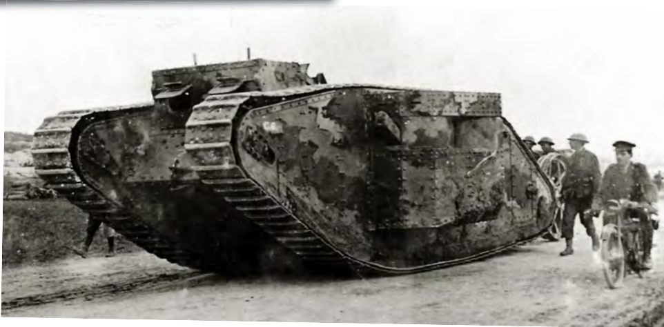
Below: C6 'Cordon Rouge', 2nd Lieutenant Allan's tank, seen on the Albert Road after the battle. It is a female tank as you can see, but notice the two tiny periscopes poking out the top of the cab.
