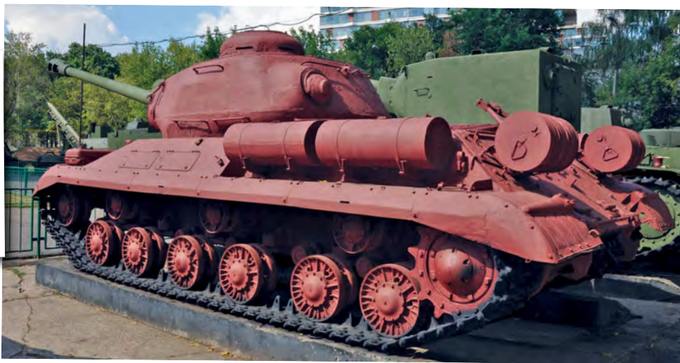
Above and below: The museum's IS-2M is also not a standard tank. It was modified for trials of OPVT-type deep-wading equipment in the early 1950s. The metal strips added to the gun mantlet, for affixing rubberised fabric waterproofing, are an obvious clue to the tank's non-standard history.
