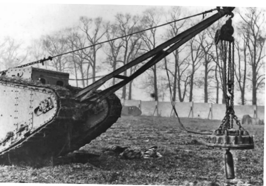
Above: Towards the end of the war, a Mark I tank fitted with a Westinghouse generator, was used to power a large Ingranic electro-magnet to lift shells from the battlefield. Tested at the Dollis Hill ground in London it did not work very well and was abandoned. Right: The only surviving Mark I tank, painted up as C19 although to be honest we don't know its identity. It is shown in a previous display at the Tank Museum.
