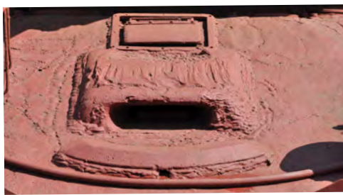
Above: This particular IS-2M also has a modified glacis with additional water sealant mounting points installed. Below: The museum's wartime ISU-152 showing the bare-metal restoration as a work in progress.
