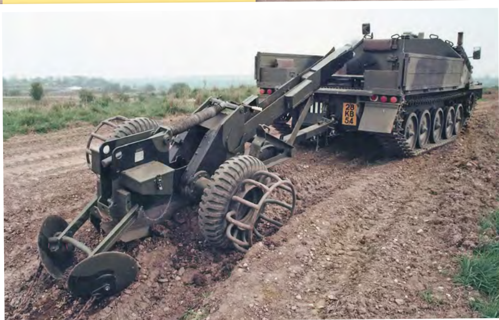
The Barmine laying version of Streaker as requested by the Royal Engineers.
