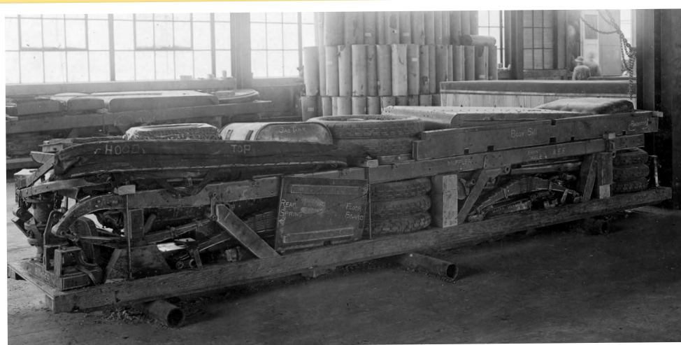
Above: Not easily identifiable as such is this completely dismantled Light Aviation which is being prepared for shipment to Europe in a crate. The parts have been labelled for the benefit of the photographer. Below: This Heavy Aviation has a couple of design differences from the other examples, having wooden spoke wheels as opposed to discs and a rather primitive cab roof which is held up by four metal poles as opposed to the more common 'pram iron' roof.
