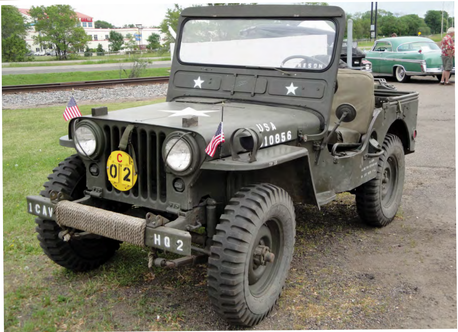
Above: Note the M38's bulging headlamps with their protective wires, and the single-pane windscreen. This fifties' gem is both affordable and practical. (Wikipedia Commons) Below right: This is a 1956 Dutch assembled M38A1 C Type. The A1 with its curvy wings and bonnet replaced the M38 in 1952.
