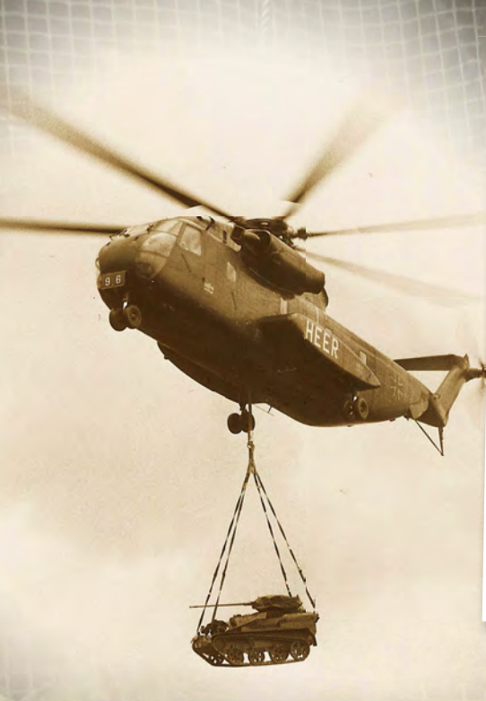
Above: A pair of Wiesel 2s deploying from a CH-57 via the rear ramp. Left: Wiesel 1 being carried by CH-57 showing ease of lift as underslung cargo.
