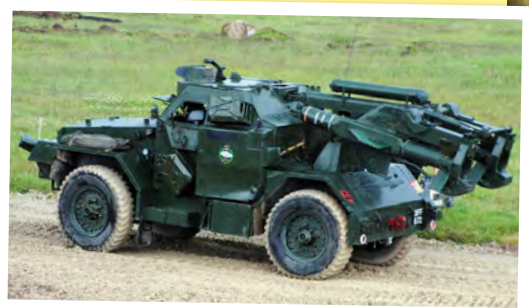
Above: The unusual Malkara version of the Humber Pig with anti-tank missiles. Left: It's hard to believe the tiny Matilda I saw service during the Dunkirk campaign in 1940. Below: The M110A1 SPG with 155mm gun puts in a good appearance.
