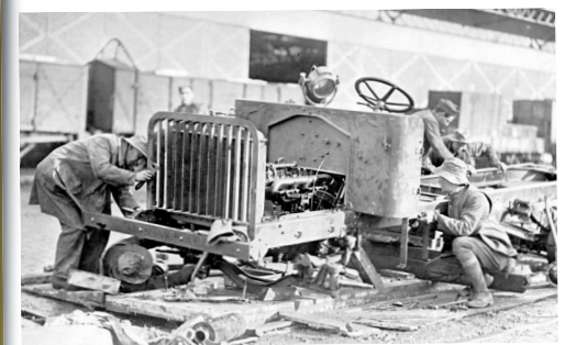
A freshly un-crated Heavy Aviation is being reassembled after having arrived in France after its long journey across the Atlantic.
