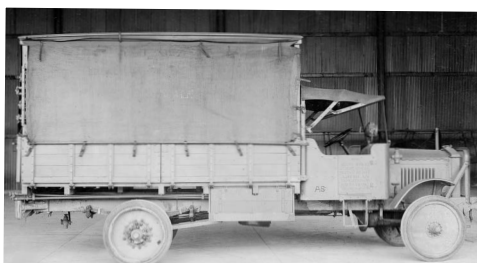
Above: The Heavy Aviation made an ideal platform for the specialist equipment required by the Air Service. This example is a field lighting set but another specific requirement by the Air Service was for mobile dark rooms to develop aerial photographs. Right: With the side screens rolled up and the sides folded down it can be seen how this truck was used to carry an engine, generator and two large drums of cable in order to power the 12 enormous lamps for airfield illumination.
