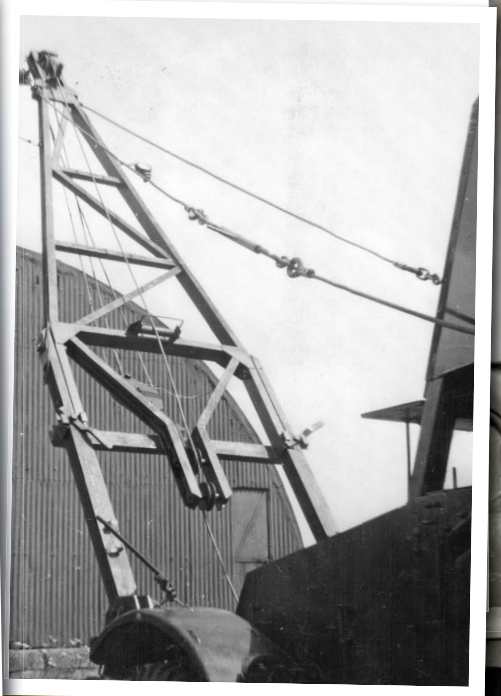
Again a detailed image of the jib here in its extended position. Note the pulley wheel and guides on the sub frame and support cables now running back to brackets welded just behind the cab doors.
