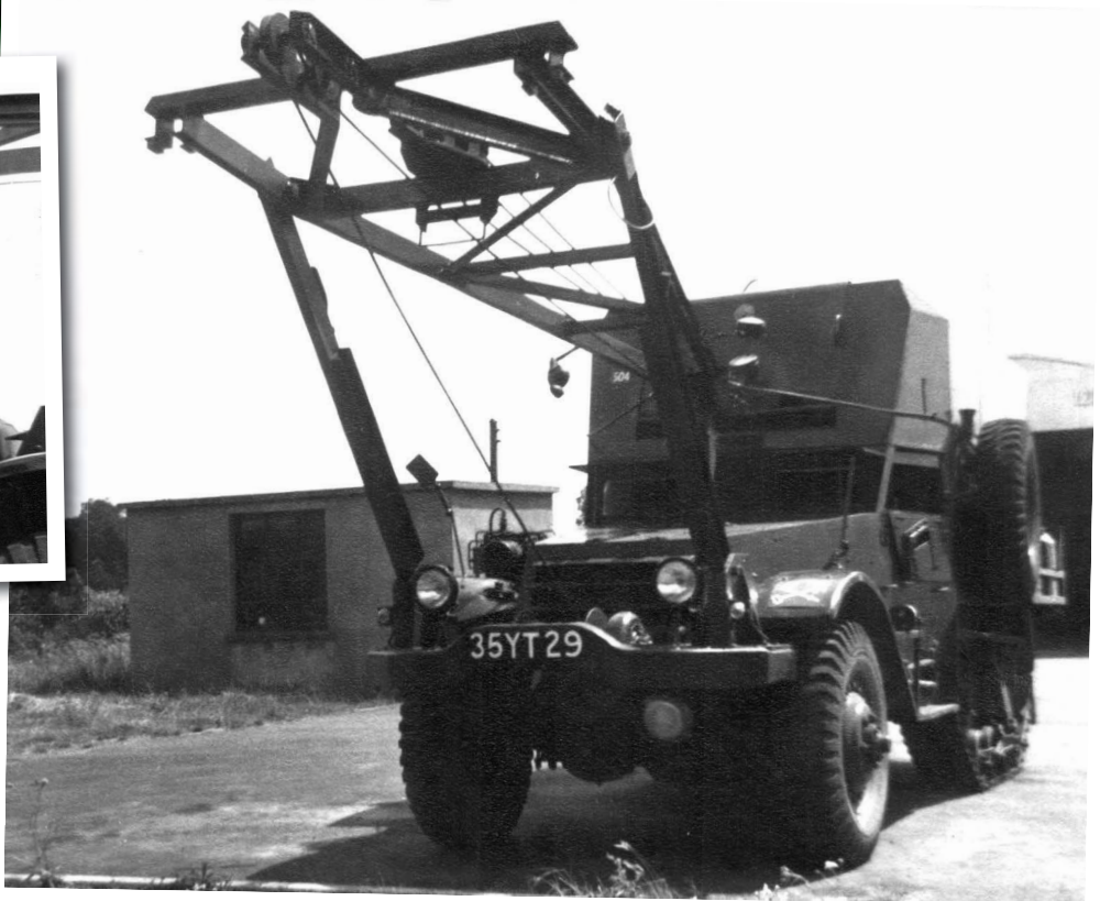
Above: This shows the closed down frame and the mounting brackets.
