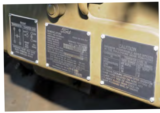
Above: The Jeep vehicle data plates are riveted to the glovebox lid. This photograph shows the correct plates for a Ford GPW.
