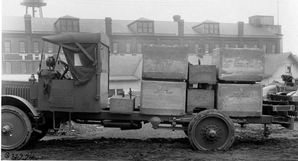
Built in Springfield Ohio by the Kelly Springfield Corp this Heavy Aviation is undergoing testing with 25,000lb of concrete and metal springs on the back. No wonder it appears to be sinking into the mud.
