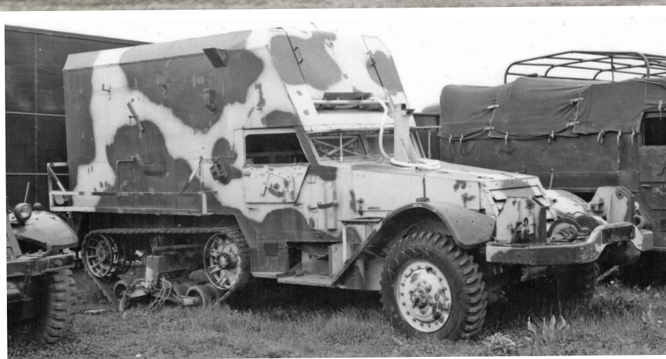
Above: Another image from Germany with a different design superstructure. This one is minus its jib. It is interesting to note the spare wheel has been mounted further back than normal. Fitters vehicles are known to have towed the 1-ton trailer but this one has a WW2 10cwt GS trailer in tow.
