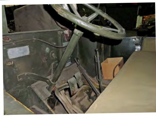
The missing wooden floor in the cab must make it a little awkward to drive. The controls are quite conventional but instead of an accelerator pedal it has a sprung metal lever which the driver has to push to the right with the side of his boot.
