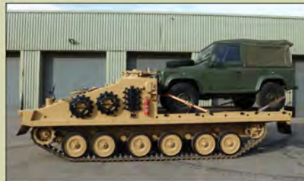
Alvis CVRT Shielder, Tracked Armoured load carrier with flat bed platform, The flat bed can be adapted for a wide range of roles such as logistic carrier, bridge layer repair / recovery and towing. Built to a high specification the vehicle hull is composed of aluminium armour to protect the crew, etc, Mileage from 500, Excellent condition, Guide price from 12,500 (4 Available).
