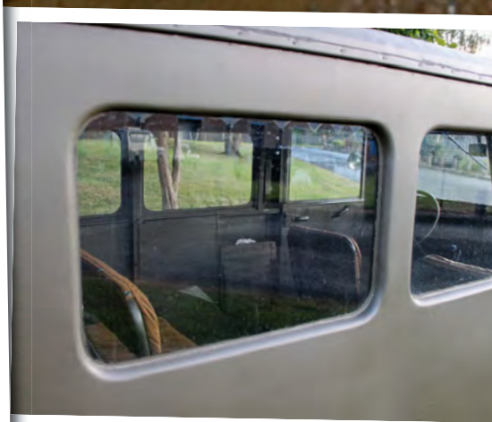
Above: The detail around the windows shows how much craftsmanship went in to the construction of the handmade aluminium rear body. Left: Both the windscreen and the door have been perfectly constructed to fit around what remains of the bulkhead belonging to the original body tub.
