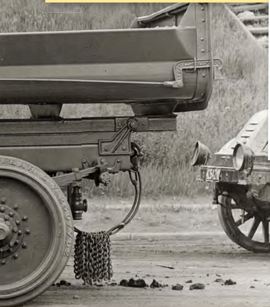
Built in Springfield Ohio by the Kelly Springfield Corp this Heavy Aviation is undergoing testing with 25,000lb of concrete and metal springs on the back. No wonder it appears to be sinking into the mud.
