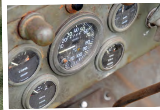
Above: Instrument panel of the M201 showing metric-calibrated Jaeger instruments. The button above the speedometer is the starter and usually has a rubber cover.
