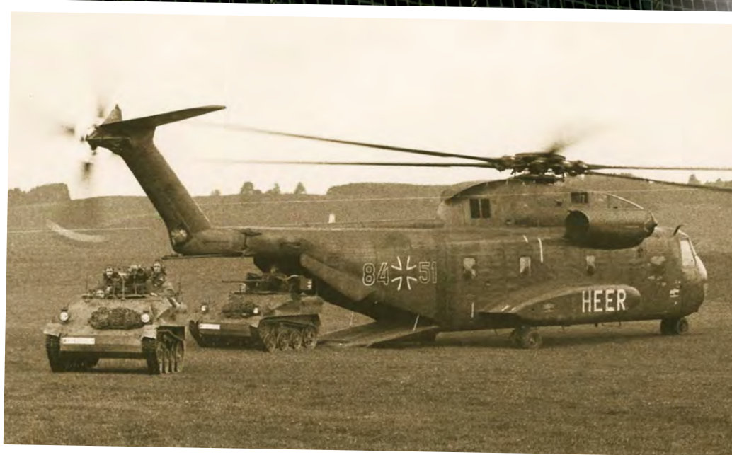
Above: A pair of Wiesel 2s deploying from a CH-57 via the rear ramp. Left: Wiesel 1 being carried by CH-57 showing ease of lift as underslung cargo.
