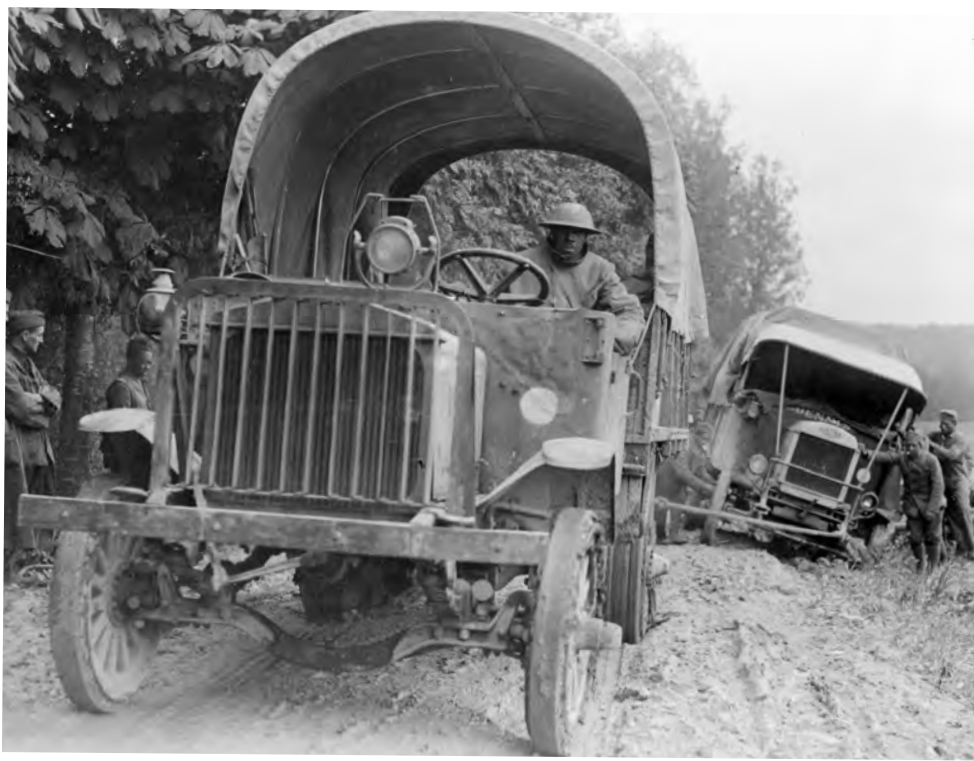
Above: One of the first trucks used by the Aviation Section of the Signal Corps was this four-wheel drive Jeffery workshop truck. The rather primitive open ring gear drive mechanism of the Jeffery suffered very badly in the dusty conditions and many had to be abandoned. Left: Photographed in October 1918 at Beauchamps this Heavy Aviation is towing a stuck British-built Dennis out of a ditch.
