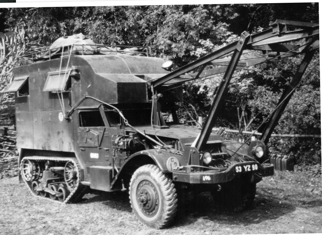
A more sophisticated superstructure has been fitted to this half-track with roof railings to accommodate extra crew stowage. The chore horse generator can clearly be observed in this image.
