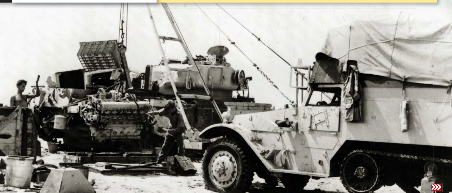
Above: Here you can see the early tubular frame jib from a different angle. This one is in operation in Germany (BAOR). Repairs appear to be the order of the day on this Centurion. Note the extensive camouflage draped over the half-track's superstructure. Below: This photo shows the early tubular steel frame design in operation with its wire supports fixed to brackets welded to the rear of the bonnet sides. This image to my knowledge was taken in Aden and shows the replacing of a Centurion MBT power pack.
