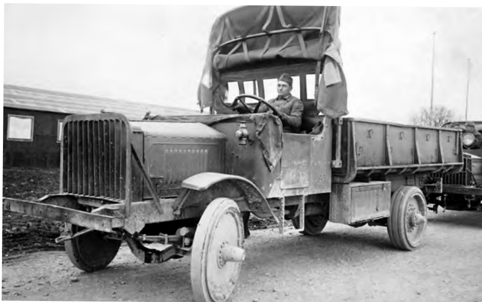
The only lighting, the paraffin side lamps made by Adlake, look rather incongruous on such a large truck. The metal body is another product of Budd, but is a non-tipping version which would require emptying by hand.
