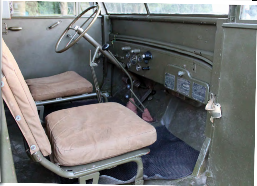
The original driver and passenger seats were adapted and retained and much of the original dash board remains as original with the exception of the relocation of the hand brake.
