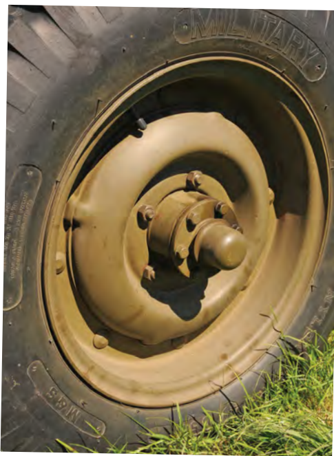
The distinctive two-piece combat wheel was fitted to all Willys MB Jeeps after serial number MB120700 and all Ford GPWs.
