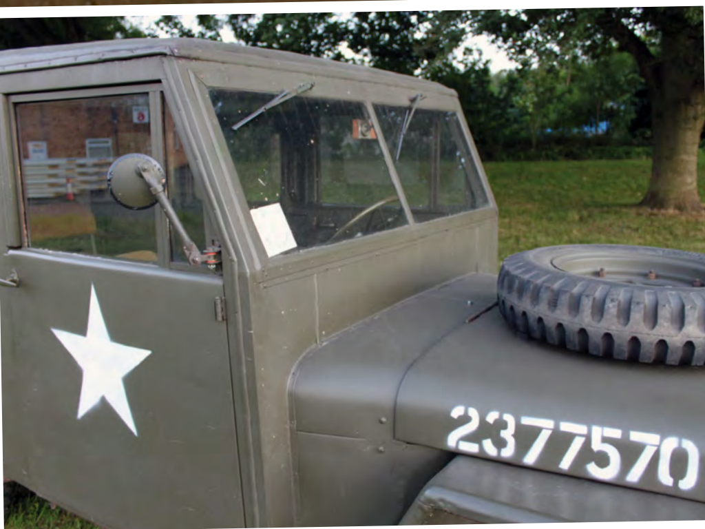
Above: The detail around the windows shows how much craftsmanship went in to the construction of the handmade aluminium rear body. Left: Both the windscreen and the door have been perfectly constructed to fit around what remains of the bulkhead belonging to the original body tub.
