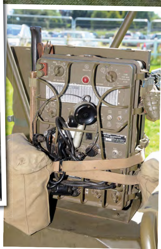
Right: A period-correct WW2 radio set is a popular Jeep accessory; typical sets include US Signal Corps radio stations SCR-510 or SCR-610, but there are many others. The photograph shows the so-called 'angry 9', a man-pack transmitter/receiver that was used during the Korean War.
