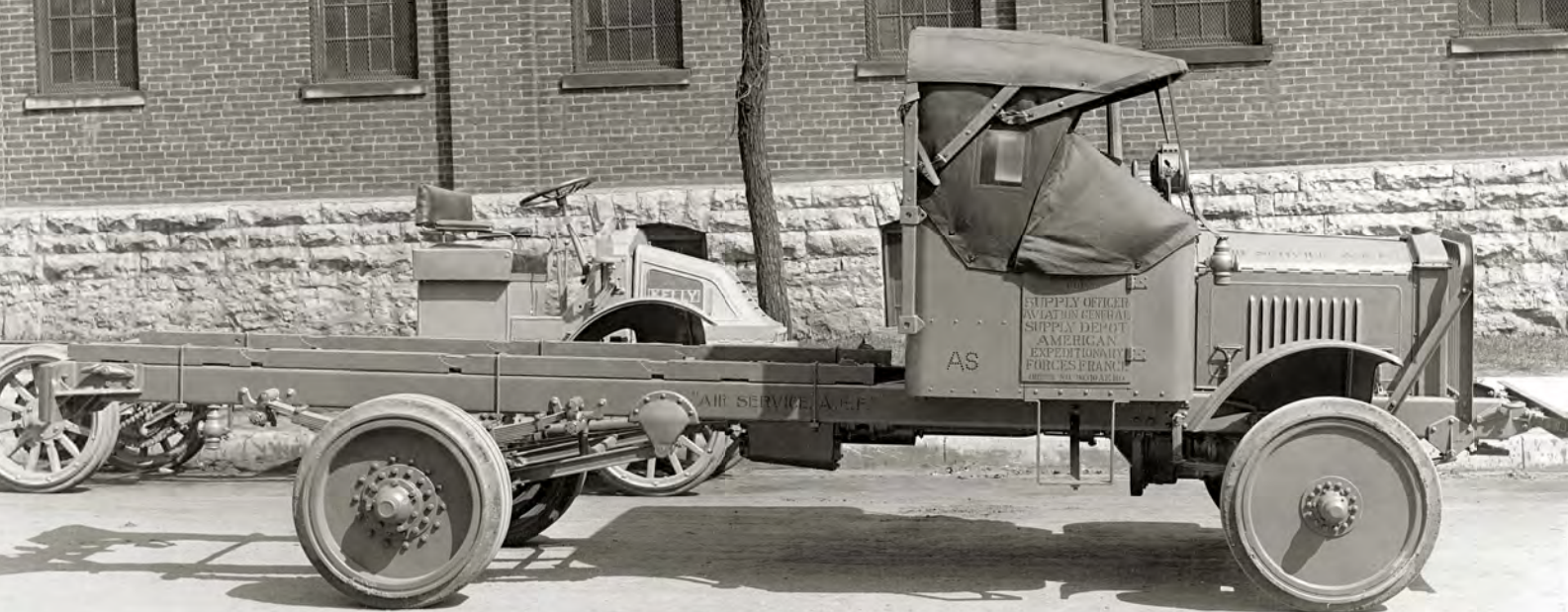
Above: Another example built by Kelly Springfield. It clearly shows the letters 'AS' drilled into the side of the cab to help prevent it being misappropriated. A problem more commonly associated with Jeeps and GMC trucks in WW2.
