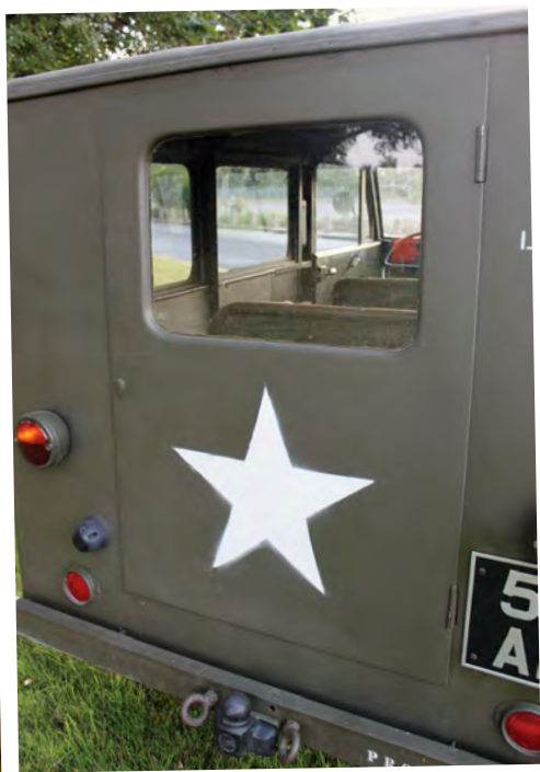
The rear door is also exquisitely made and despite having no seal as such, the perfect fit lets in very little water!
